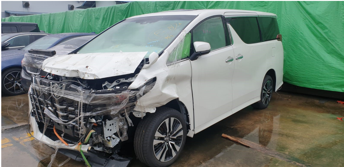
Photo 1 shows the front left body of the Motor Car (photograph provided to me). The Motor Car was observed to have sustained damage at its frontal body. The front bumper, front bumper reinforcement, front bumper centre lower grille, front bumper left lower grille chrome moulding, front bumper left lower grille, radiator grille, front emblem, front left headlamp, front bonnet, front bonnet chrome moulding, front bonnet lock, front bonnet hinges, front left fog lamp, front undercover, front sensors, front support panel, front support panel top garnish, front left fender and front left fender inner shield were amongst the body parts that were observed to have been damaged. The extent of damage to the frontal body of the Motor Car suggests possible damage to its aircon condenser and radiator.
