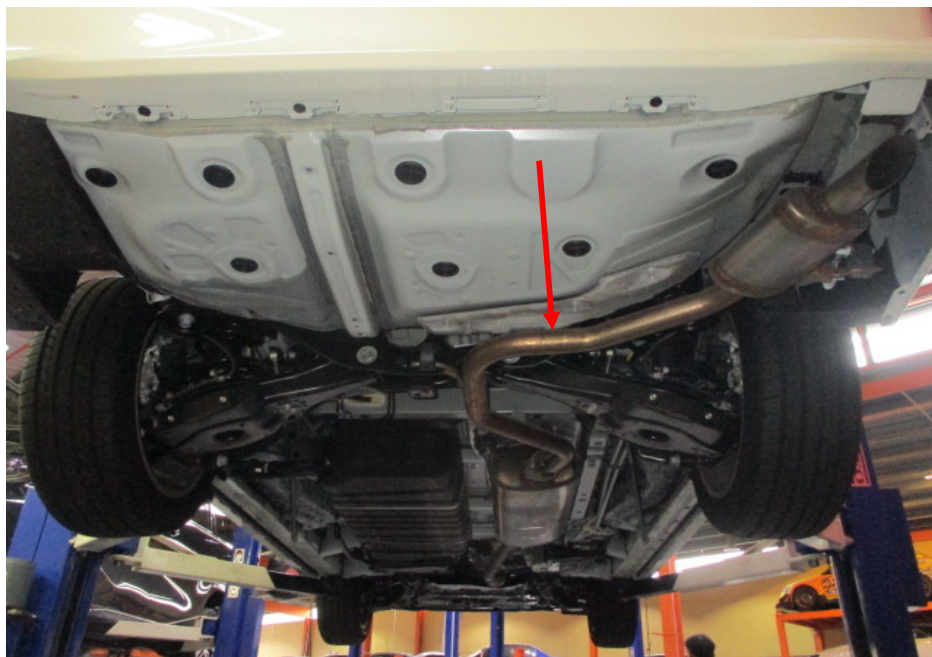
Photo 26 shows a general view of the rear section of the Motor Car's exhaust system. My examination of the Motor Car's exhaust system revealed no sign(s) or indication(s) of any cut or weld marks along its exhaust pipe (arrowed), on its catalytic converter, on its centre resonator box and on its rear muffler.
