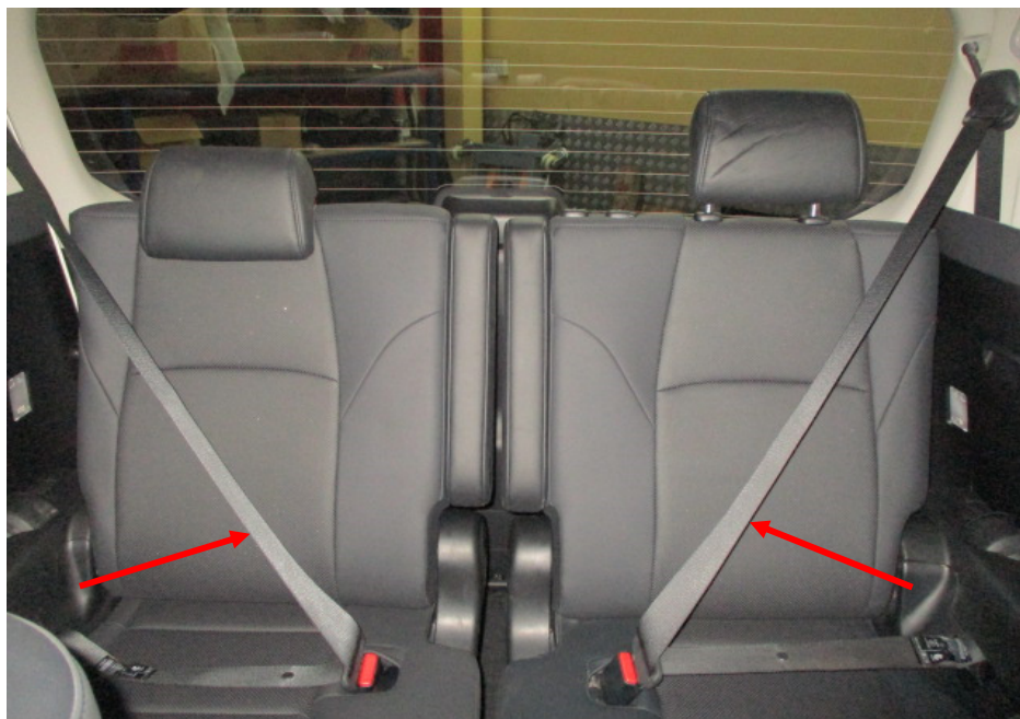
Photo 18 shows the rear seats at the 2 nd row of the Motor Car. All the seats of the Motor Car were secured via seat rails to the floorboard. They were also fitted with a retractable seat belt reel and a pre-tensioner. The seat belts (arrowed) were tested and were able to be fastened into the respective pre-tensions that were fitted on the side of each individual seat.
