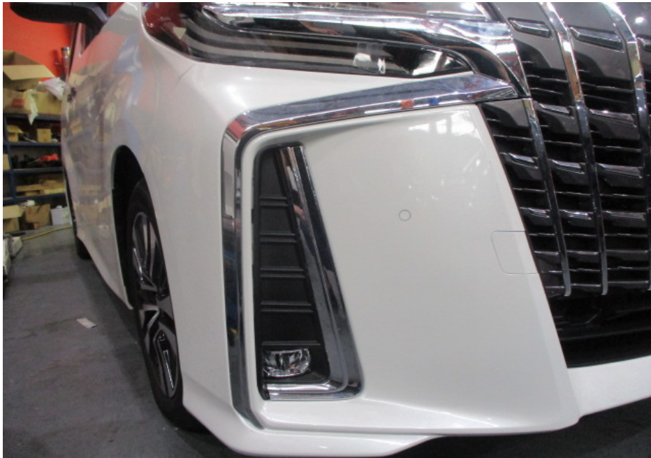
Photo 10 shows a closer view of the Motor Car's front bumper, front bumper right lower grille chrome moulding, front bumper right lower grille and front right fog lamp. The body parts at the frontal body of the Motor Car were visually examined and it was observed that the repair/restoration works carried out to the damaged area of the Motor Car (refer to photograph 2 above) were reasonably adequate and in order.
