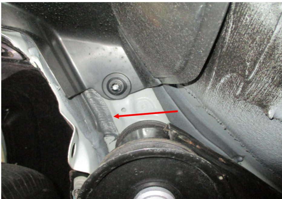
Photo 29 shows the chassis/structural body at the underside rear left of the Motor Car. The original factory sealant (arrowed) at the joints along the chassis/structural body was observed to be untouched. In general, I had found no work was carried out on the chassis/structural body of the Motor Car. The chassis/structural body of the Motor Car was originally fitted
