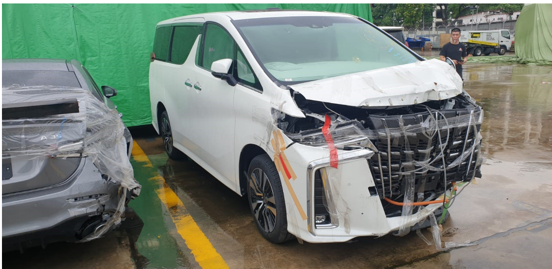
Photo 2 shows the front right body of the Motor Car (photograph provided to me). The Motor Car was observed to have sustained damage at its frontal body. The front bumper, front bumper centre lower grille, front bumper right lower grille chrome moulding, radiator grille, front emblem, front right headlamp, front bonnet, front bonnet chrome moulding, front bonnet lock, front bonnet hinges, front support panel, front support panel top garnish and front right fender were amongst the body parts that were observed to have been damaged. The extent of damage suggests possible damage to the aircon condenser and radiator of the Motor Car. The photographs provided appear to also show the Motor Car's airbags not deployed.
