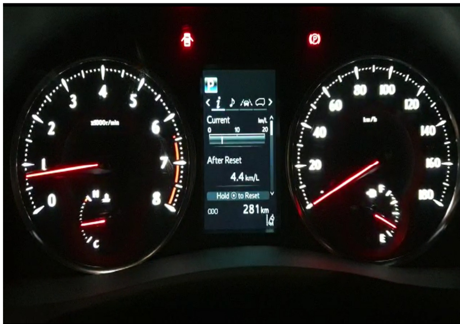
Photo 20 shows the respective warning lights no longer illuminated, indicating that there is no fault detected to the ABS, SRS, EPS, VSC and various pre-collision systems of the Motor Car during the self-test. These electronic systems were hence in working condition at the time of my inspection.
