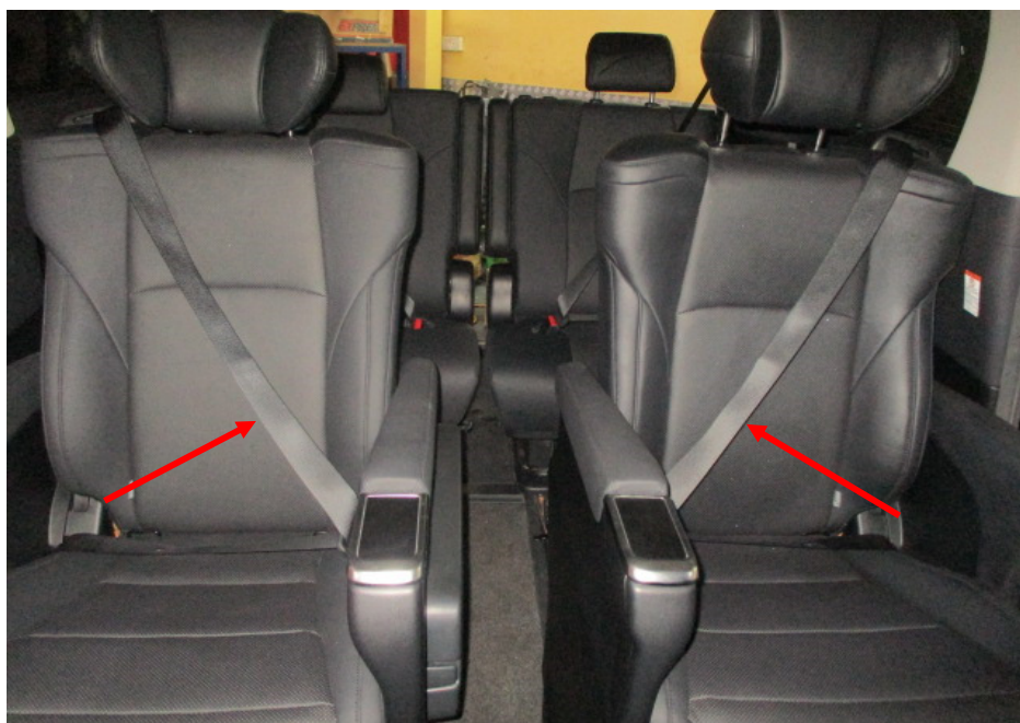
Photo 17 shows the rear seats at the 1 st row of the Motor Car. All the seats of the Motor Car were secured via seat rails to the floorboard. They were also fitted with a retractable seat belt reel and a pre-tensioner. The seat belts (arrowed) were tested and were able to be fastened into the respective pre-tensions that were fitted on the side of each individual seat.
