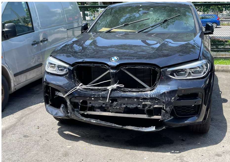
Photo 1 shows the frontal body of the Motor Car (photograph provided to me). The photographs provided to me had showed damage to the frontal portion of the Motor Car. Body parts damaged include the front bumper, front bumper centre lower grille, front bumper right lower grille, front bumper reinforcement, front radar unit, front sensors, front right day running light, front left day running light, front radiator grilles and front bonnet amongst others.
