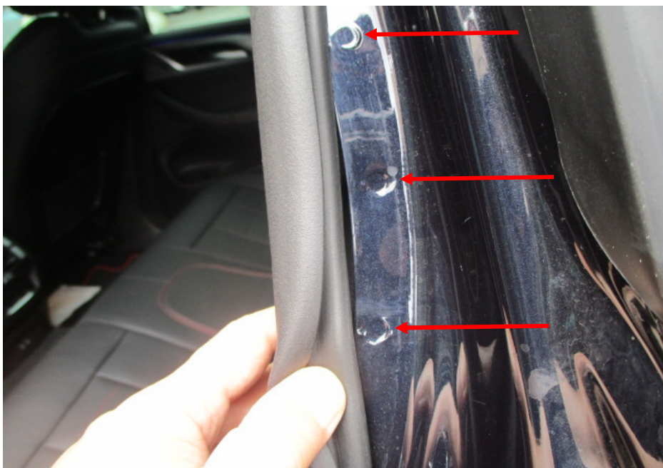
Photo 32 shows the left side "C" pillar of the Motor Car. I did not find any weld marks other than original spot weld marks (arrowed) on the left side "C" pillar of the Motor Car which, indicates that there was no re-welding works carried out. In general, I had found all the non-detachable body panels of the Motor Car to be originally fitted at the time of my inspection.
