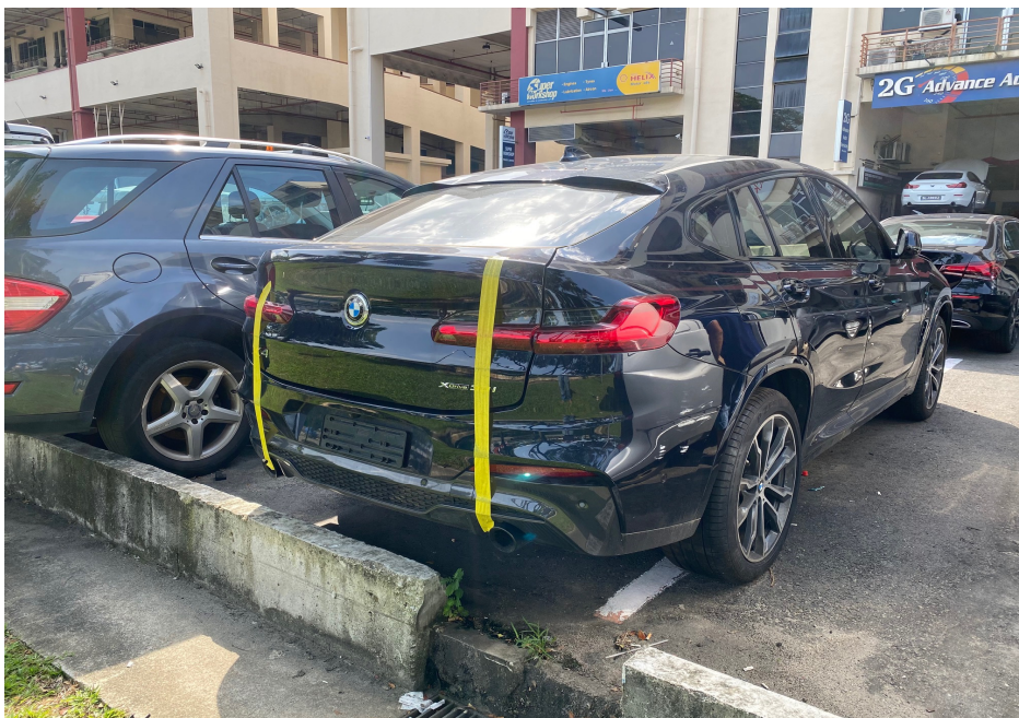
Photo 2 shows the rear right body of the Motor Car (photograph provided to me). Apart for the frontal portion, I had also observed damage to the Motor Car's rear right portion. The rear bumper and rear right fender were observed to be with relatively minor damage.
