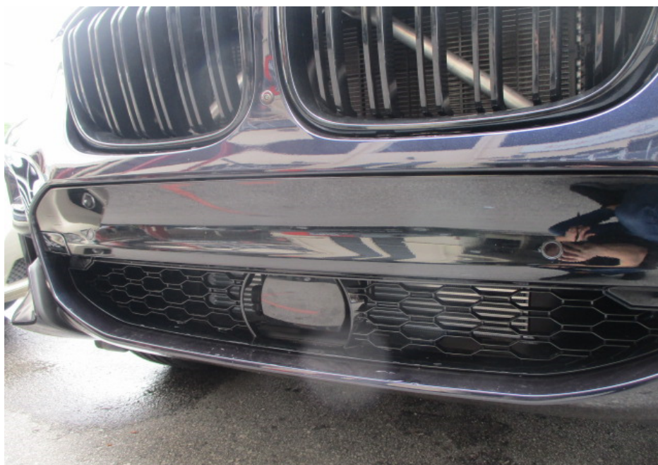
Photo 10 shows a closer view of the Motor Car's front bumper centre lower grille, front radar unit and front radiator grilles at the time of my inspection. The body parts at the frontal portion of the Motor Car were visually examined and it was observed that the repair/restoration works carried out to the damaged area of the Motor Car (refer to photograph 1 above) were reasonably adequate and in order.
