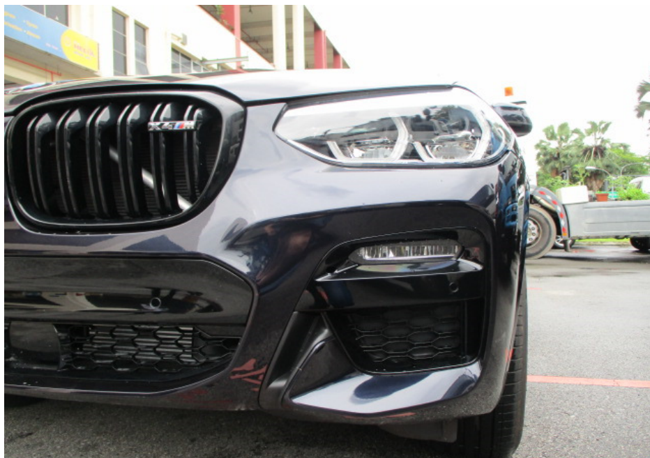
Photo 9 shows a closer view of the Motor Car's front bumper, front left lower grille, front left day running light and front left headlamp at the time of my inspection. The body parts at the frontal portion of the Motor Car were visually examined and it was observed that the repair/restoration works carried out to the damaged area of the Motor Car (refer to photograph 1 above) were reasonably adequate and in order.
