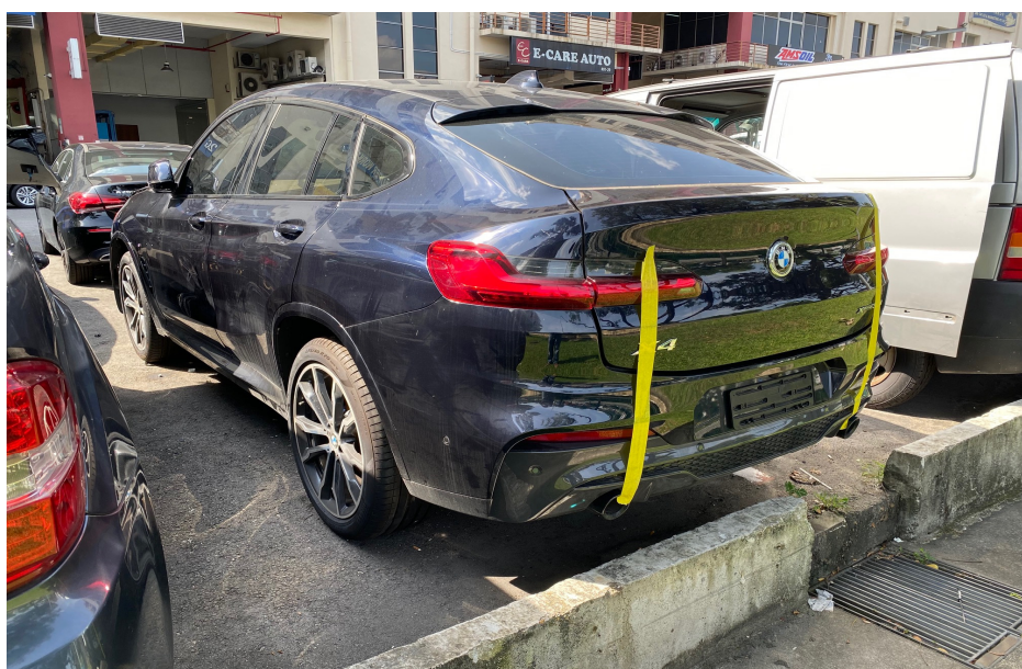
Photo 4 shows the rear left body of the Motor Car (photograph provided to me). Apart for the frontal portion and rear right portion, there was no physical damage observed to other areas of the Motor Car. The airbags of the Motor Car were also not deployed as seen from the photographs that were provided to me.
