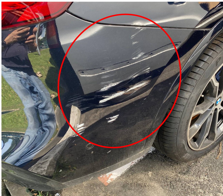
Photo 3 shows a closer view of the damage (circled) at the rear right portion of the Motor Car (photograph provided to me). The rear bumper and rear right fender of the Motor Car were observed to be with relatively minor damage.
