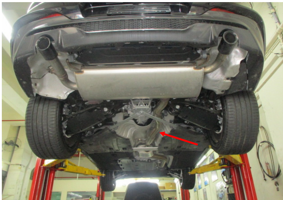
Photo 25 shows the rear section of the Motor Car's exhaust system. My examination of the Motor Car's exhaust system revealed no sign(s) or indication(s) of any cut or weld marks along its exhaust pipes (arrowed), on its rear muffler, on its centre resonator box and on its catalytic converter.
