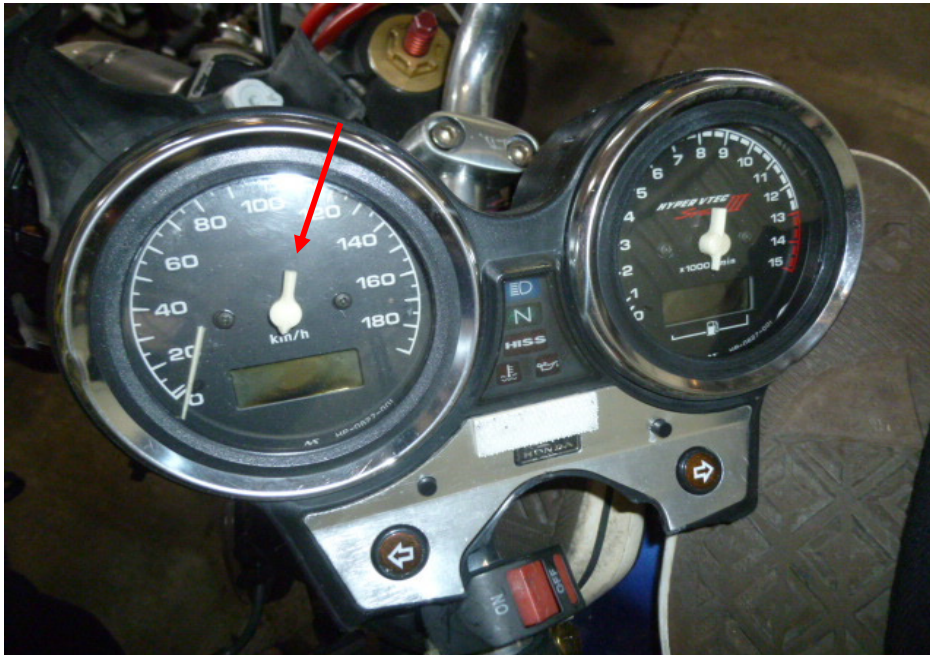
Photo 7 shows the damaged speedometer of the Motorcycle as a result of the accident (arrowed).
