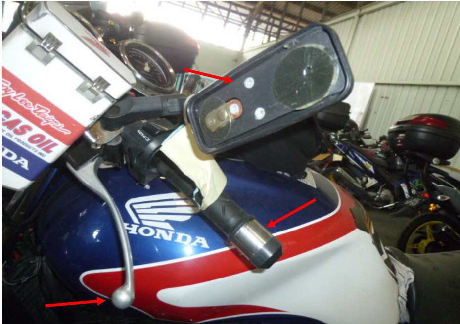
Photo 11 shows a closer view of the clutch lever, left side mirror and left handlebar end (arrowed) which were amongst the body parts at the front body of the Motorcycle that had sustained damage as a result of the accident.
