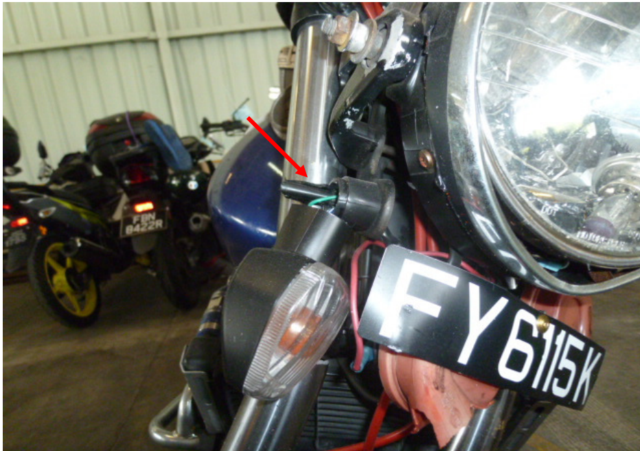
Photo 13 shows the broken right front signal lamp (arrowed) of the Motorcycle as a result of the accident.
