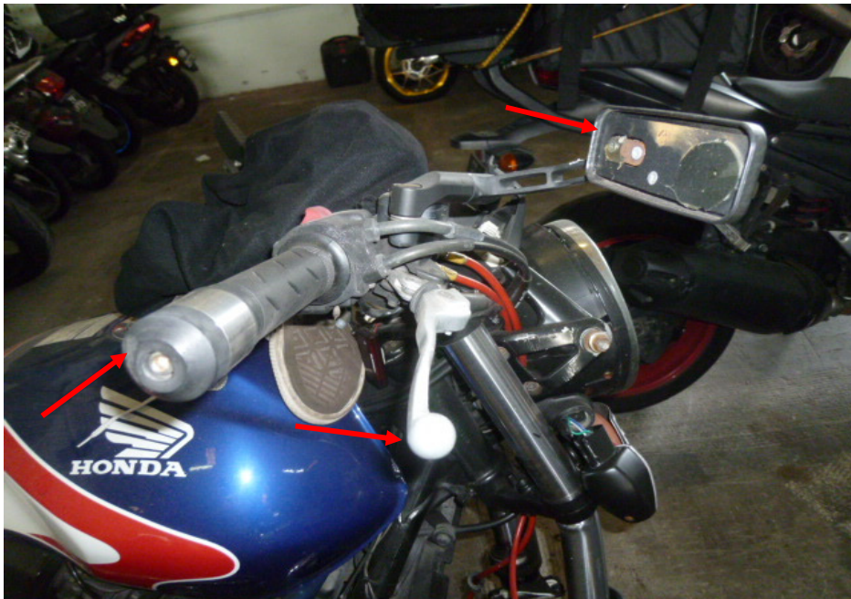
Photo 6 shows a closer view of the front brake lever, right side mirror and right handlebar end (arrowed) which were amongst the body parts at the front body of the Motorcycle that had sustained damage as a result of the accident.
