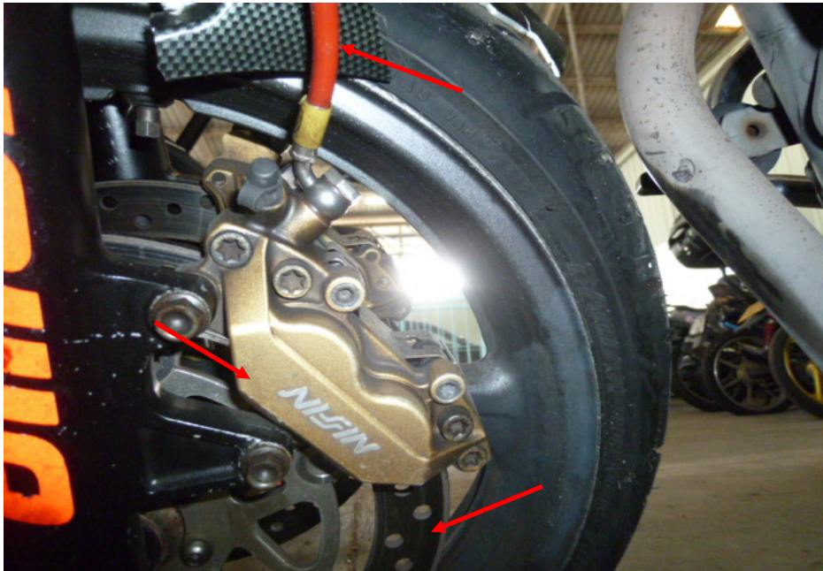
Photo 22 shows a close up view of the front brake caliper, front brake disc and front brake hose (arrowed) at the left side of the Motorcycle's front wheel, which are all part of the components in the hydraulic front brake system of the Motorcycle. Our visual checks of these various components had revealed all to be intact with no visible damage. No leakage of brake fluid was also observed.
