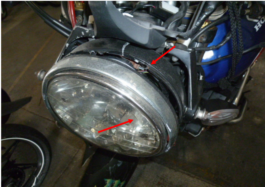
Photo 4 shows a closer view of the cracked headlight cover and scratched headlight (arrowed) of the Motorcycle as a result of the accident.
