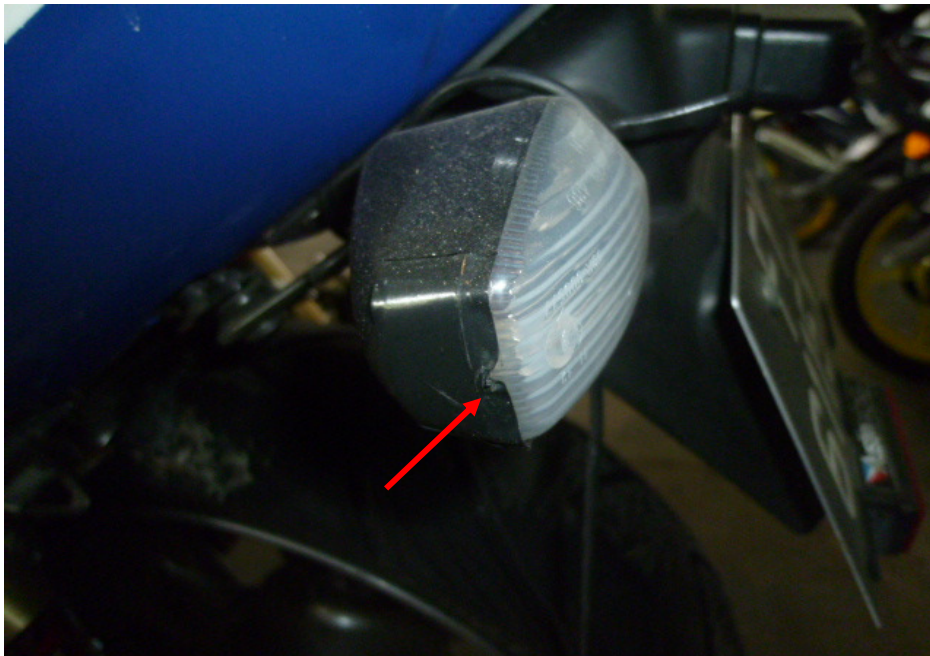
Photo 12 shows a closer view of the grazed left rear signal lamp (arrowed) of the Motorcycle as a result of the accident.
