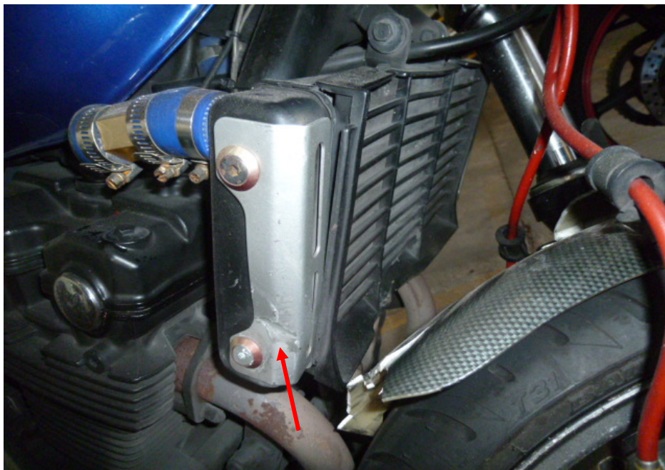
Photo 10 shows a closer view of the deformed radiator (arrowed) of the Motorcycle as a result of the accident.
