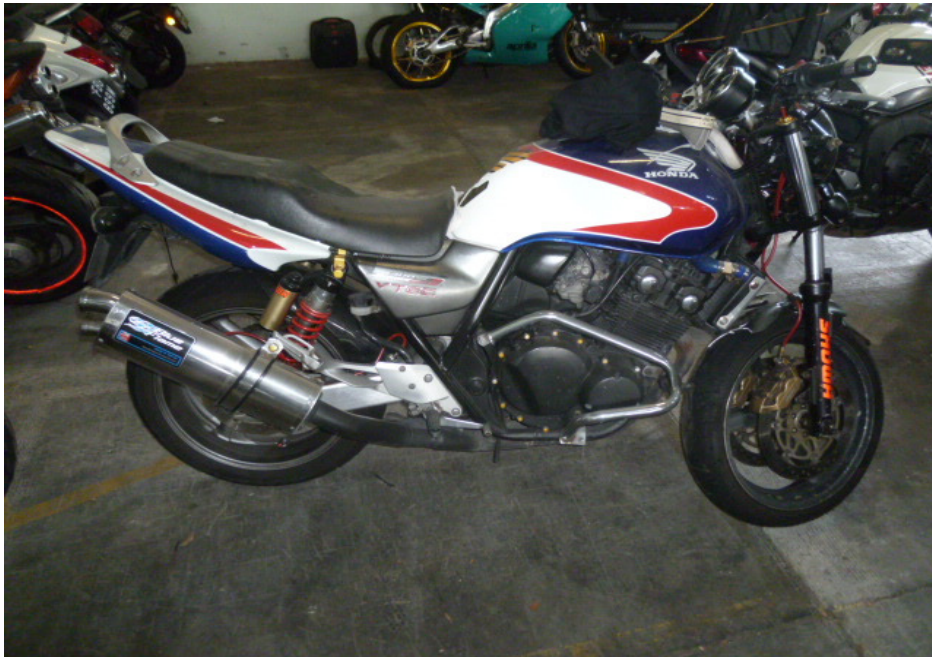
Photo 3 shows a general view of the right body of the Motorcycle at the time of our inspection. The Motorcycle was observed to have sustained damages all around. The body parts that were found to have been damaged include its speedometer gauge, headlight cover, headlight, front forks, front mudguard, radiator, right handlebar end, right side mirror, front brake lever, petrol tank, right front signal lamp, left front footrest and left rear signal lamp, amongst others.
