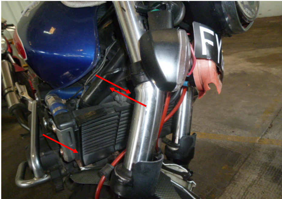
Photo 20 shows the right front fork of the Motorcycle. The right front fork (arrowed) was observed to be bent inwards as a result of the accident. We were hence not able to conduct any tests on the steering system of the Motorcycle.
