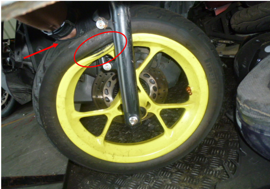
Photo 16 shows the bent front wheel rim (circled) and deflated front tyre (arrowed) of the Motorcycle at the time of our inspection.
