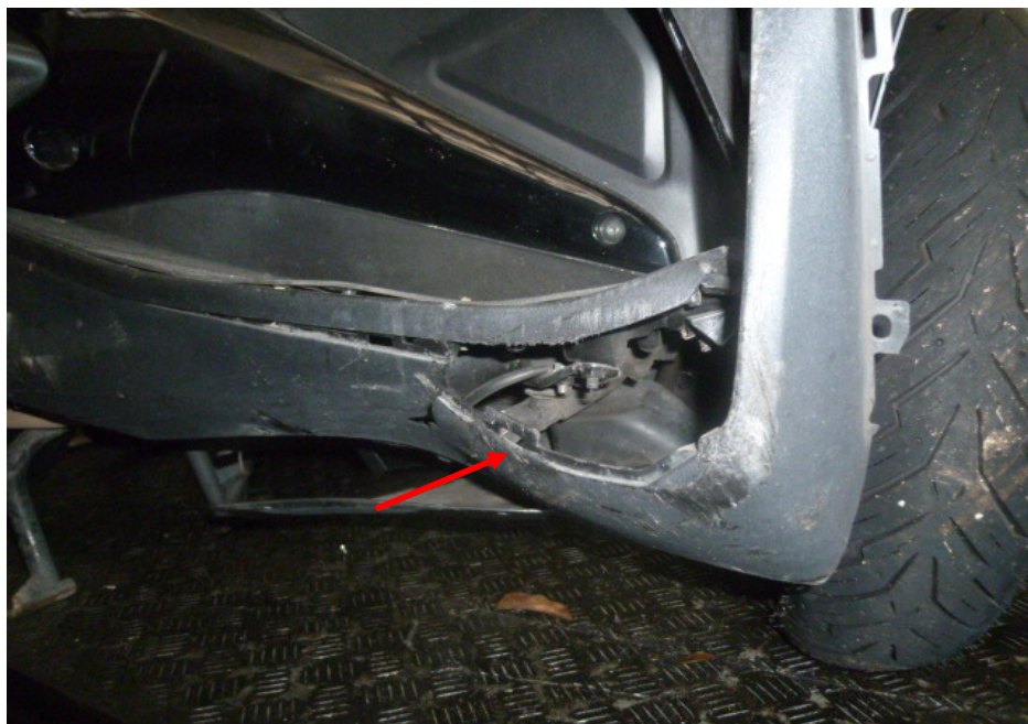
Photo 11 shows a closer view of the cracked right lower side cover of the Motorcycle as a result of the accident (arrowed).
