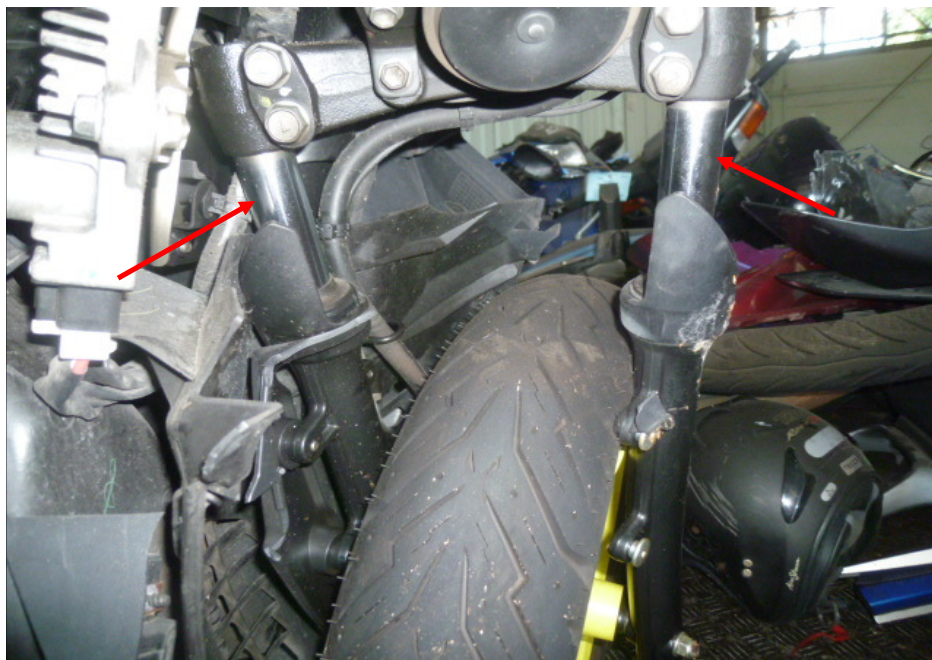
Photo 23 shows the front fork assembly of the Motorcycle. The front forks were observed to be bent (arrowed) as a result of the accident. We were hence not able to conduct any tests on the steering system of the Motorcycle.
