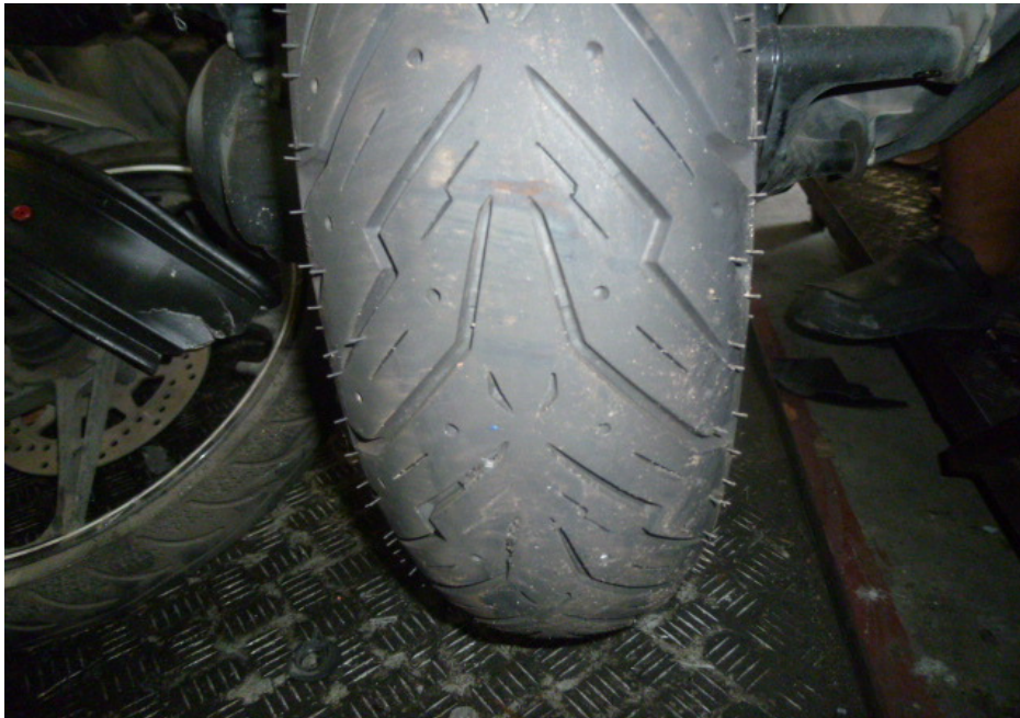
Photo 17 shows the condition of the Motorcycle's rear tyre. The rear tyre was observed to be in serviceable condition with remaining tread depth of approximately 6mm. The tyre was also observed to be sufficiently inflated for vehicular operation. We did not observe any tear, burst mark(s) and/or punctured hole(s) on the sidewalls as well as across the tread of the rear tyre.
