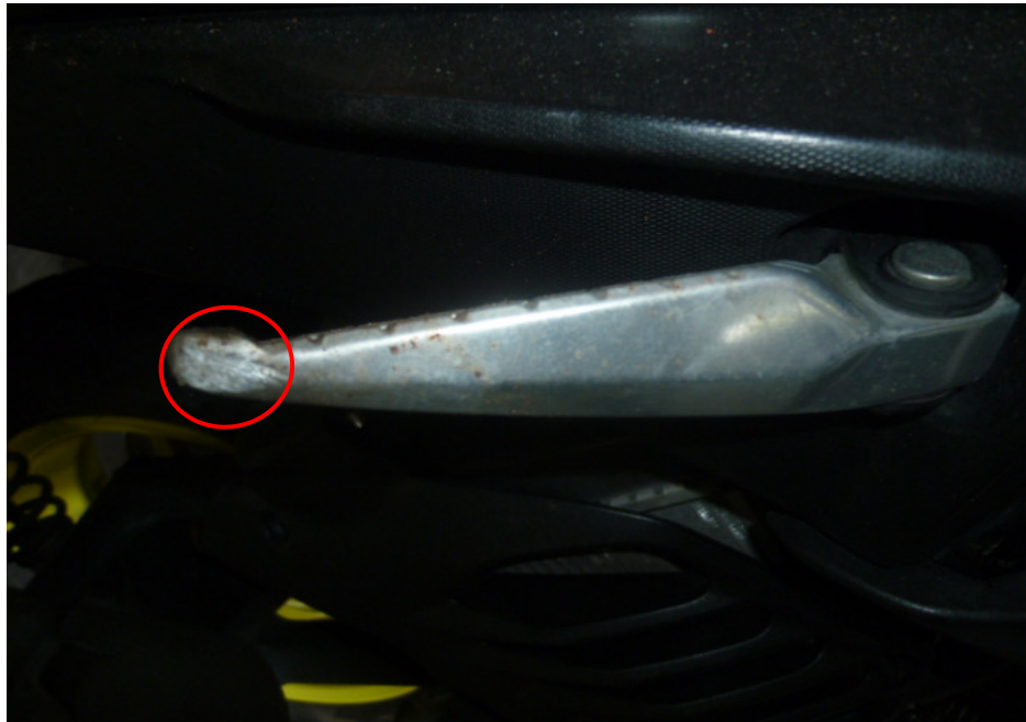
Photo 13 shows a closer view of the grazed left pillion foot peg of the Motorcycle at the time of our inspection (circled).
