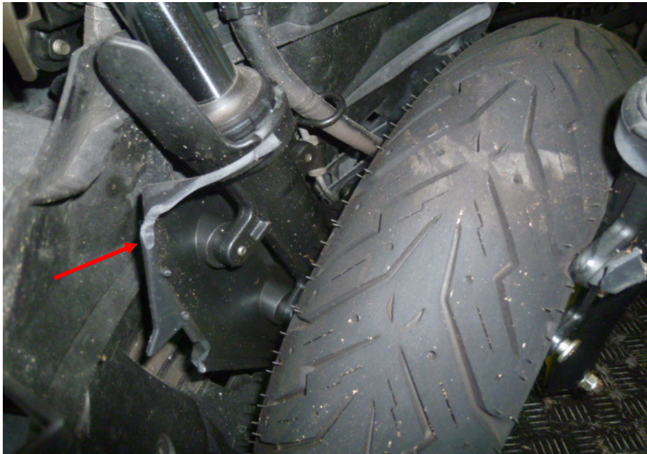
Photo 7 shows a closer view of the cracked front mudguard which was amongst the body parts at the front body of the Motorcycle that had sustained damage as a result of the accident (arrowed).
