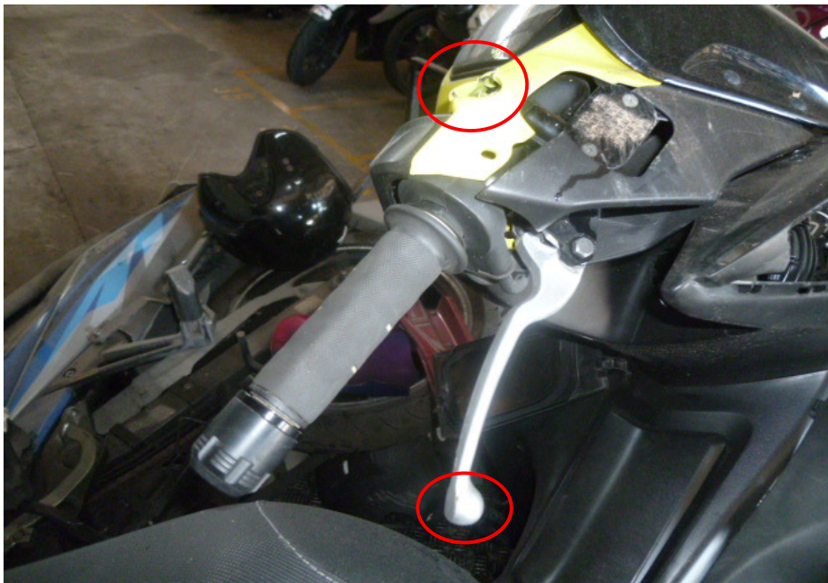
Photo 8 shows a closer view of the missing right side mirror and front brake lever of the Motorcycle which were observed to be damaged due to the accident (circled).
