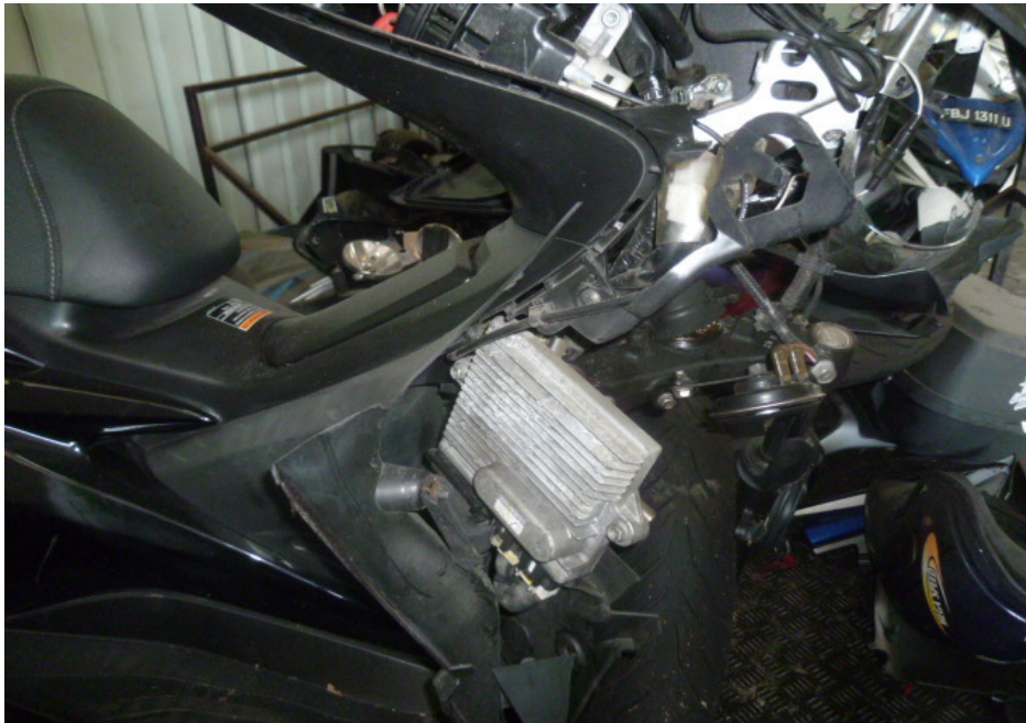
Photo 9 shows the missing right side cowling of the Motorcycle as a result of the accident.
