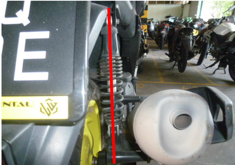
Photo 22 shows the right shock absorber of the Motorcycle which was found to be intact without any misalignment.
