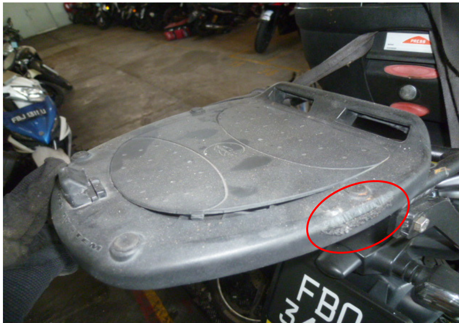
Photo 14 shows a closer view of the top box rack of the Motorcycle which had sustained damages of grazing nature due to the accident (circled).
