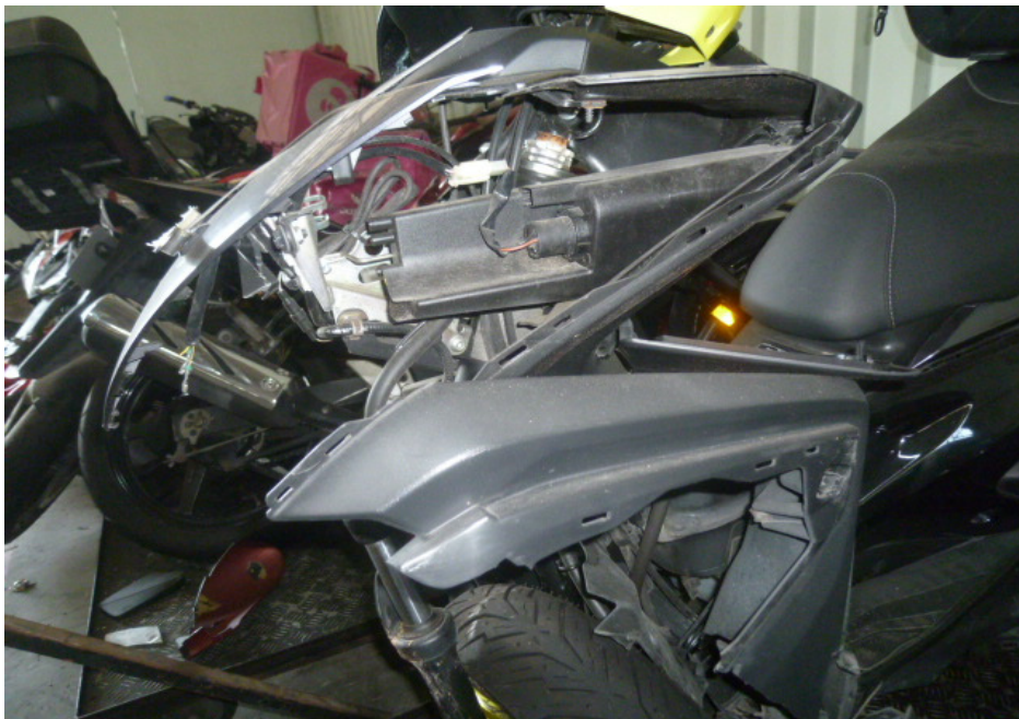
Photo 10 shows the broken left side cowling of the Motorcycle as a result of the accident.
