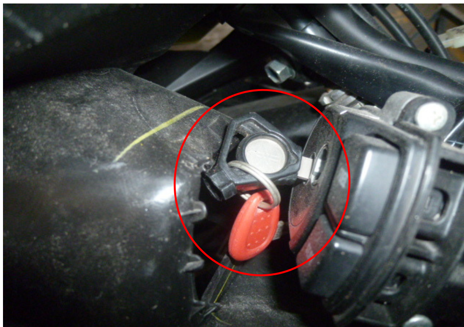
Photo 1 shows the jammed key in the ignition of the Motorcycle as a result of the accident (circled).
