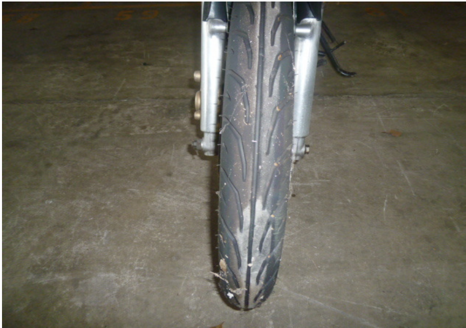
Photo 12 shows the front tyre of the Motorcycle at the time of our inspection. The front tyre was observed to be in serviceable condition with remaining tread depth of approximately 7mm. The tyre was also observed to be sufficiently inflated for vehicular operation. We did not observe any tear, burst mark(s) and/or punctured hole(s) on the sidewalls as well as across the tread of the front tyre.
