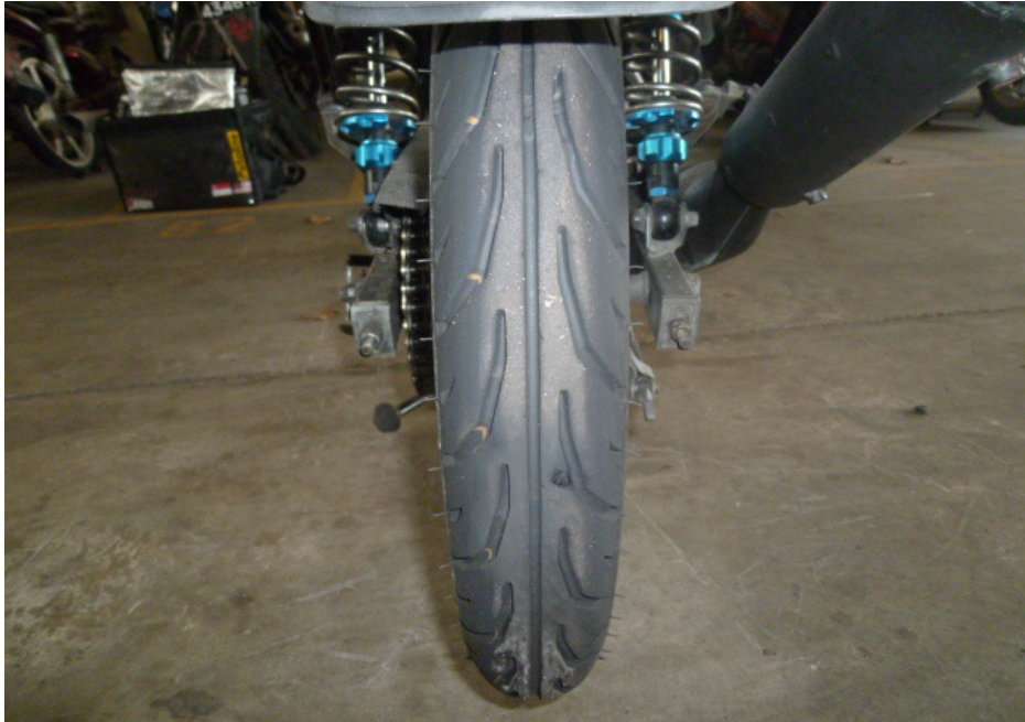
Photo 13 shows the condition of the Motorcycle's rear tyre. The rear tyre was observed to be in serviceable condition with remaining tread depth of approximately 5mm. The tyre was also observed to be sufficiently inflated for vehicular operation. We did not observe any tear, burst mark(s) and/or punctured hole(s) on the sidewalls as well as across the tread of the rear tyre.
