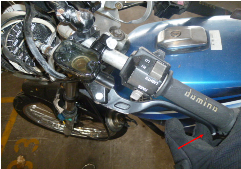
Photo 20 shows the clutch lever being depressed. There was some resistance felt (spongy like feel) upon pressing the clutch lever (arrowed). This would indicate that there is no leakage of pressure/vacuum in the hydraulic clutch system.
