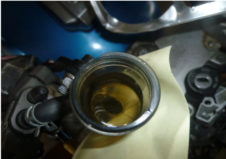
Photo 23 shows the brake fluid reservoir for the front brake of the Motorcycle. The brake fluid was found to be of sufficient level for operating purposes and without any contamination.
