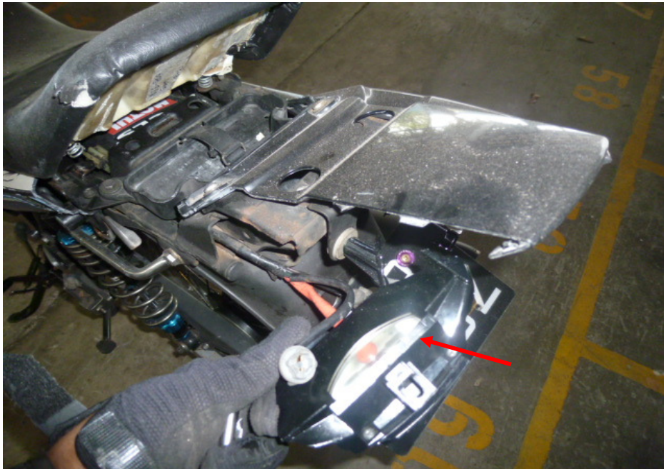
Photo 11 shows the broken tail light assembly of the Motorcycle as a result of the accident (arrowed).
