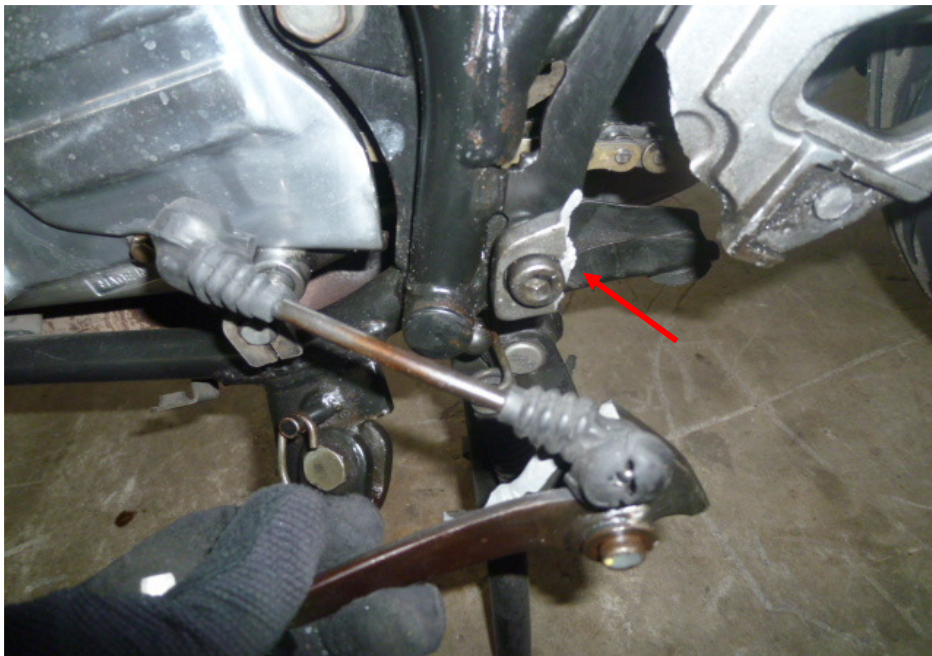
Photo 8 shows the broken left front footrest bracket (arrowed) of the Motorcycle as a result of the accident.
