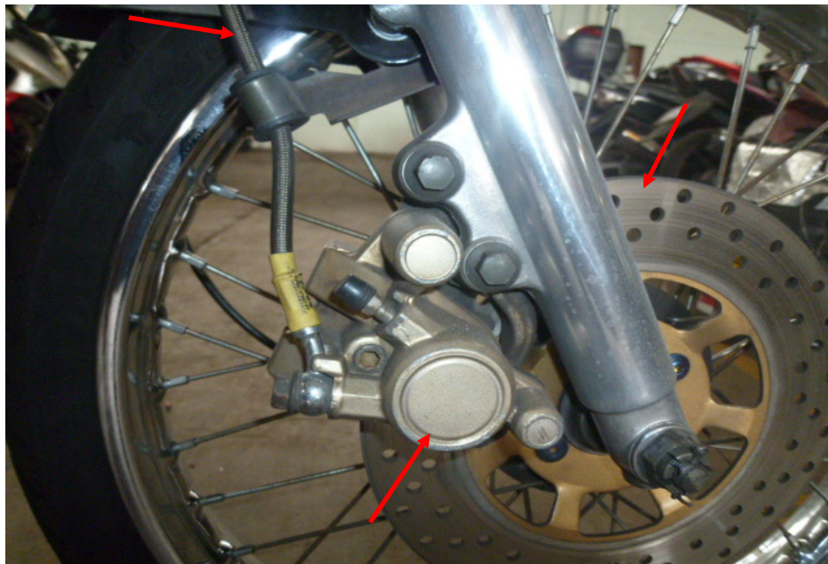
Photo 21 shows a close up view of the front brake caliper, front brake disc and front brake hose (arrowed) of the Motorcycle, which are all part of the components in the hydraulic front brake system of the Motorcycle. Our visual checks of the front brake caliper and front brake disc had revealed all to be intact with no visible damage. However we observed a leakage of brake fluid along the front brake hose.
