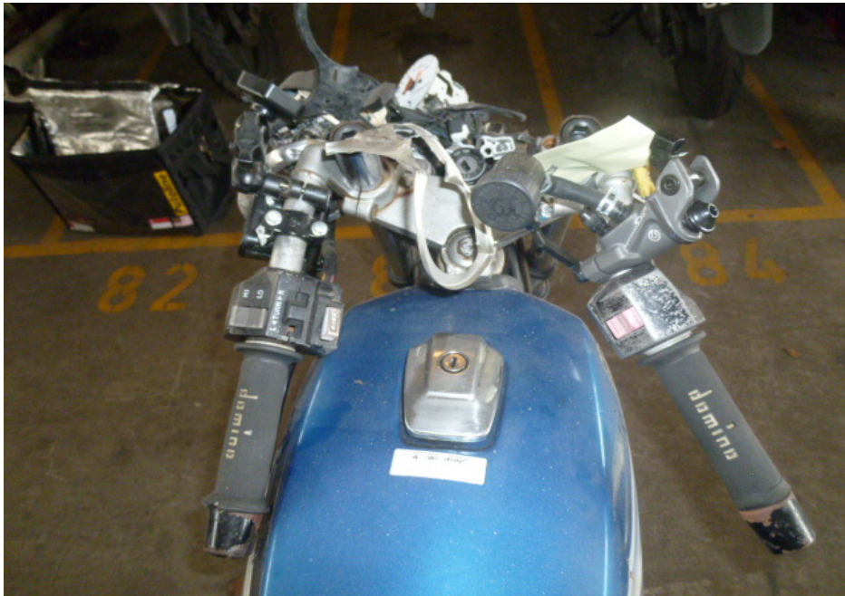
Photo 5 shows a close up view of the handlebars, side mirrors, front brake lever, clutch lever and handlebar ends of the Motorcycle. These parts were amongst the body parts of the Motorcycle which were damaged as a result of the accident.
