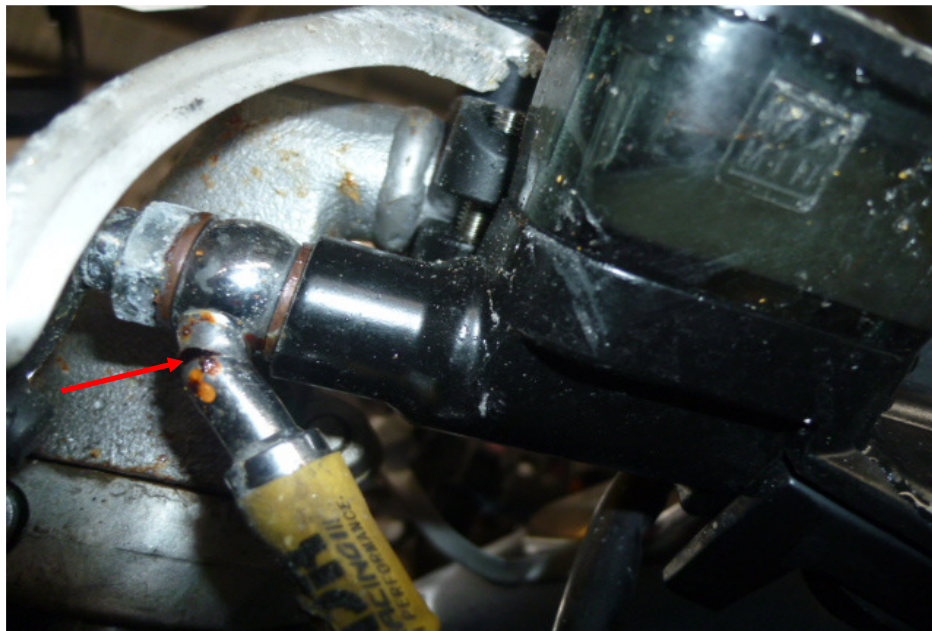
Photo 22 shows the front brake reservoir of the Motorcycle. We observed a leakage of brake fluid along the front brake hose. This was from the respective front brake fluid reservoir to the front brake caliper of the Motorcycle. Upon closer examination, we found that the front brake hose was cut as a result of the accident (arrowed).
