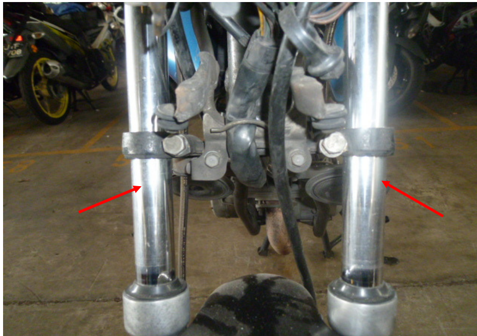
Photo 18 shows the front fork assembly of the Motorcycle. The front forks were observed to be bent inwards as a result of the accident (arrowed). We were hence not able to conduct any tests on the steering system of the Motorcycle.
