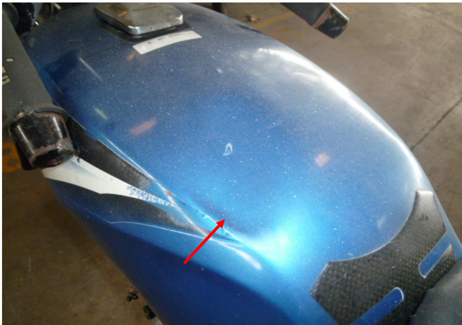
Photo 6 shows a closer view of the petrol tank, which was amongst the body parts of the Motorcycle that had sustained damage as a result of the accident (arrowed).
