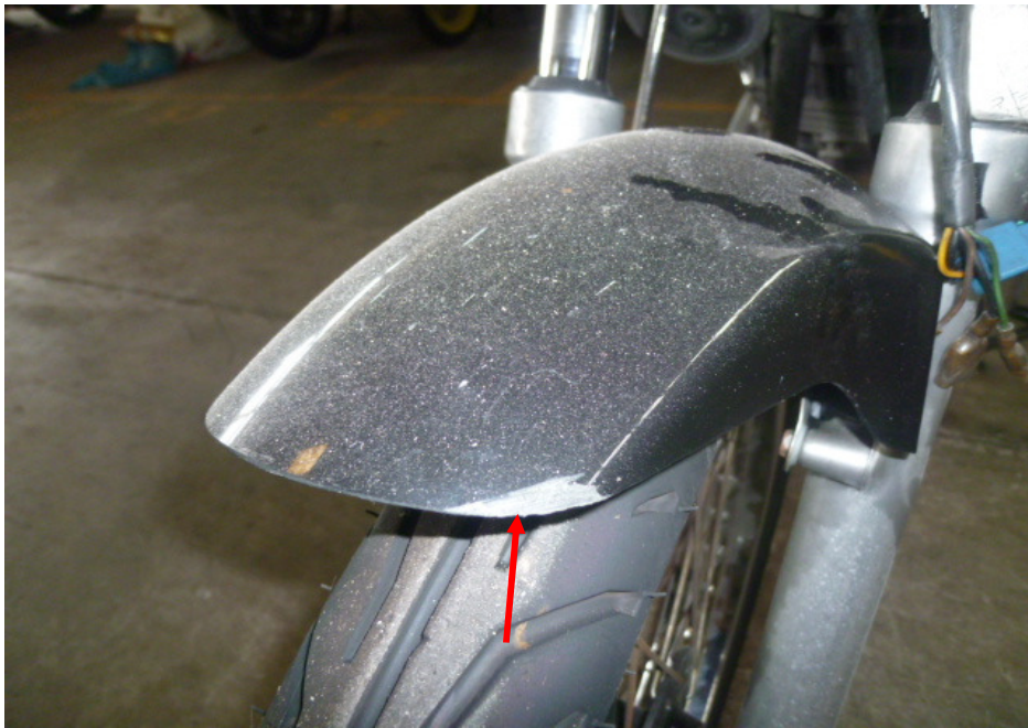
Photo 7 shows a closer view of the front mudguard (arrowed) which was amongst the body parts of the Motorcycle that had sustained damage as a result of the accident.
