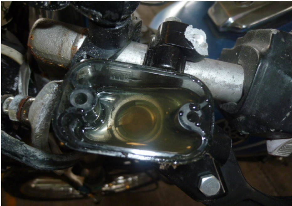
Photo 19 shows the hydraulic clutch fluid reservoir for the hydraulic clutch system of the Motorcycle. The hydraulic clutch fluid was observed to be of sufficient level for operational purposes and without any contamination.
