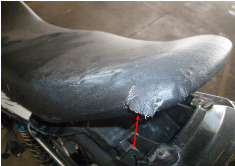
Photo 10 shows the deformed seat of the Motorcycle as a result of the accident (arrowed).
