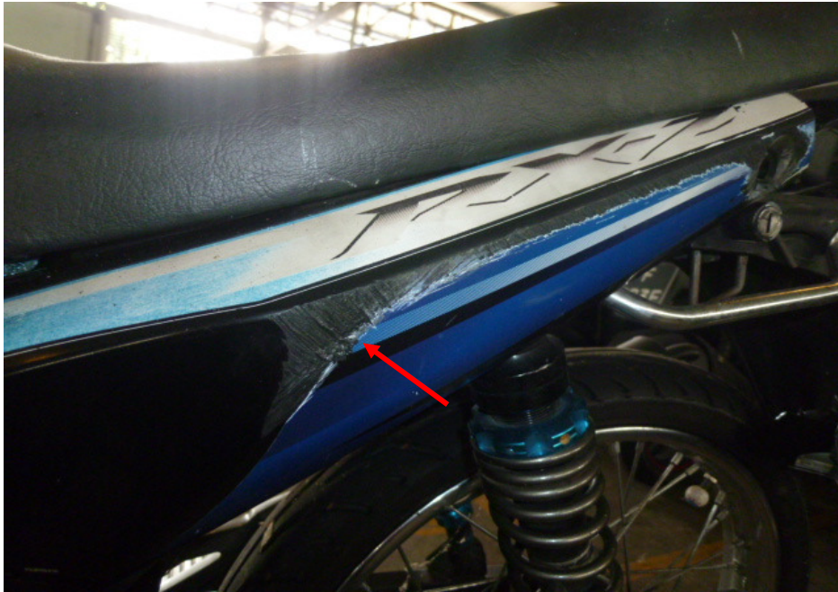
Photo 9 shows the grazed left rear side cover (arrowed) of the Motorcycle as a result of the accident.
