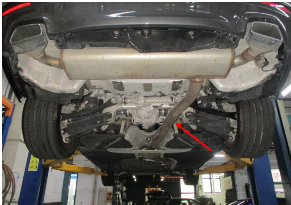
Photo 24 shows the rear section of the Motor Car's exhaust system. My examination of the Motor Car's exhaust system revealed no sign(s) or indication(s) of any cut or weld marks along its exhaust pipes (arrowed), on its centre resonator box, on its rear muffler and on its catalytic converter.
