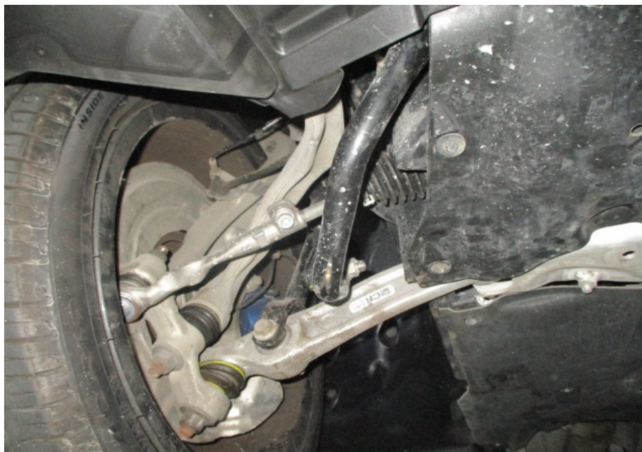
Photo 22 shows the various undercarriage components at the front right wheel of the Motor Car. The mechanical components, control arms and linkages were all found to be intact and secured in an appropriate manner.
