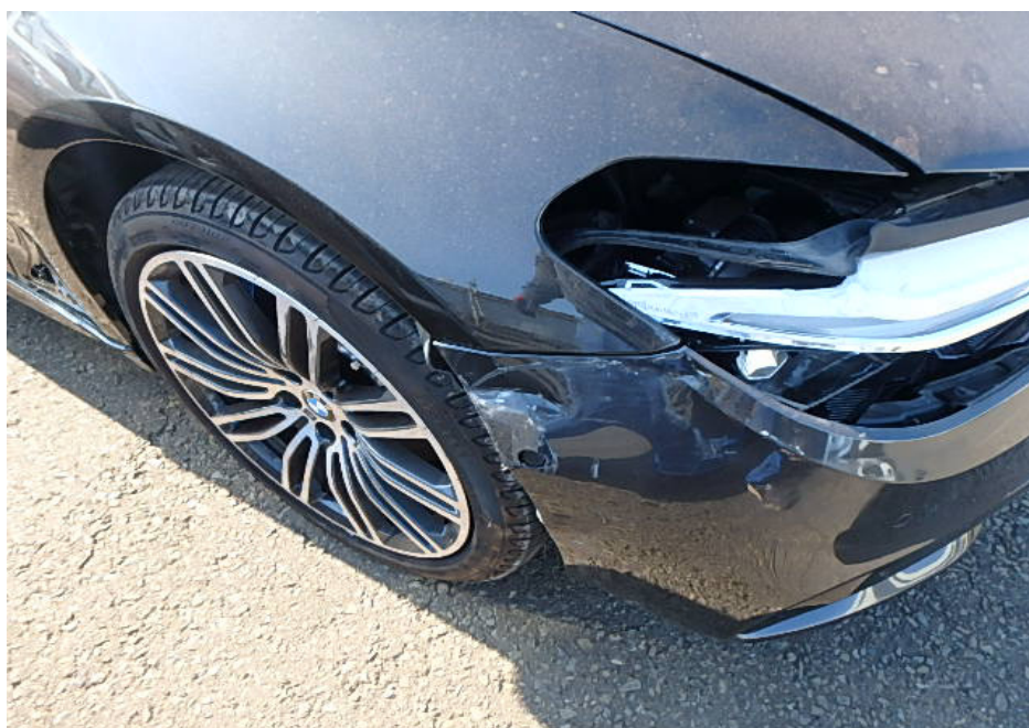
Photo 2 shows a closer view of the damage at the front right body of the Motor Car (photograph provided to me). The front bumper, front right headlamp and front right fender were observed to be damaged.
