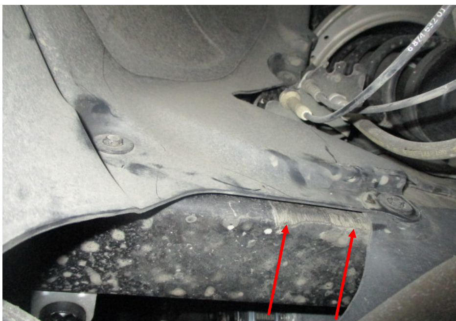
Photo 29 shows the chassis/structural body at the underside front left of the Motor Car. The original factory sealant (arrowed) at the joints along the chassis/structural body was observed to be untouched. In general, I had found no work was carried out on the chassis/structural body of the Motor Car. The chassis/structural body of the Motor Car was originally fitted.
