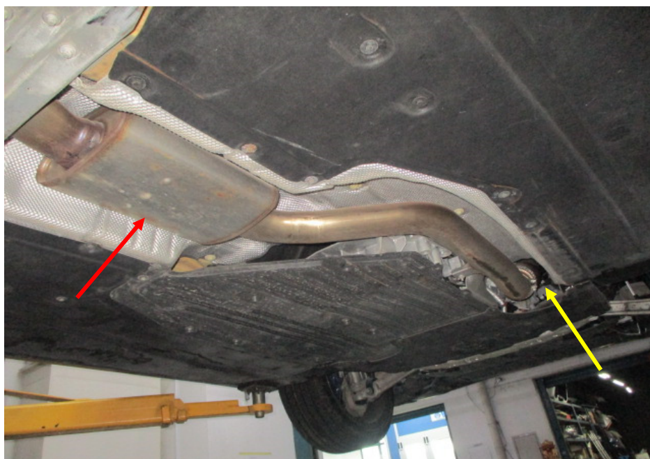
Photo 25 shows the front section of the Motor Car's exhaust system. My examination of the Motor Car's exhaust system revealed no sign(s) or indication(s) of any cut or weld marks along its exhaust pipes, on its centre resonator box (red arrow), on its rear muffler and on its catalytic converter (yellow arrow).
