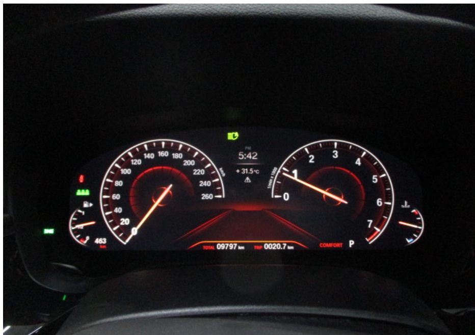
Photo 18 shows the respective warning lights no longer illuminated, indicating that there is no fault detected to the ABS, SRS, IAS, TPM and DSC systems of the Motor Car during the self-test. These electronic systems were hence in working condition at the time of my inspection.
