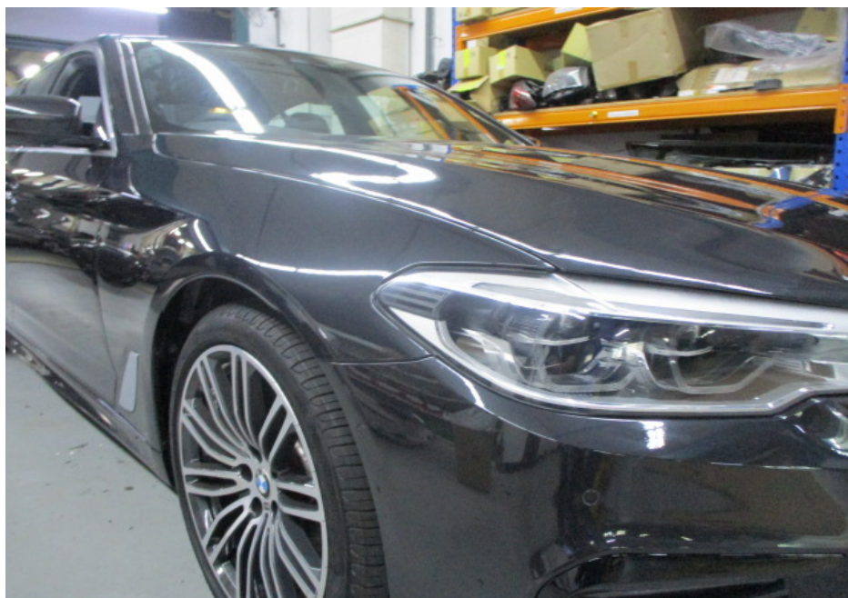
Photo 9 shows a closer view of the front bumper, front right headlamp and front right fender of the Motor Car at the time of my inspection. The body parts at the front right body of the Motor Car were visually examined and it was observed that the repair/restoration works carried out to the damaged area of the Motor Car (refer to photograph 1 & 2 above) were reasonably adequate and in order.
