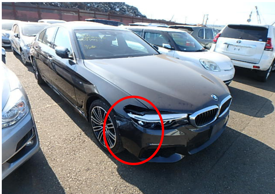
Photo 1 shows a general view of the front right body of the Motor Car (photograph provided to me). The Motor Car was observed to have sustained damage at its front right body (circled). The front bumper, front right headlamp and front right fender were observed to be damaged.
