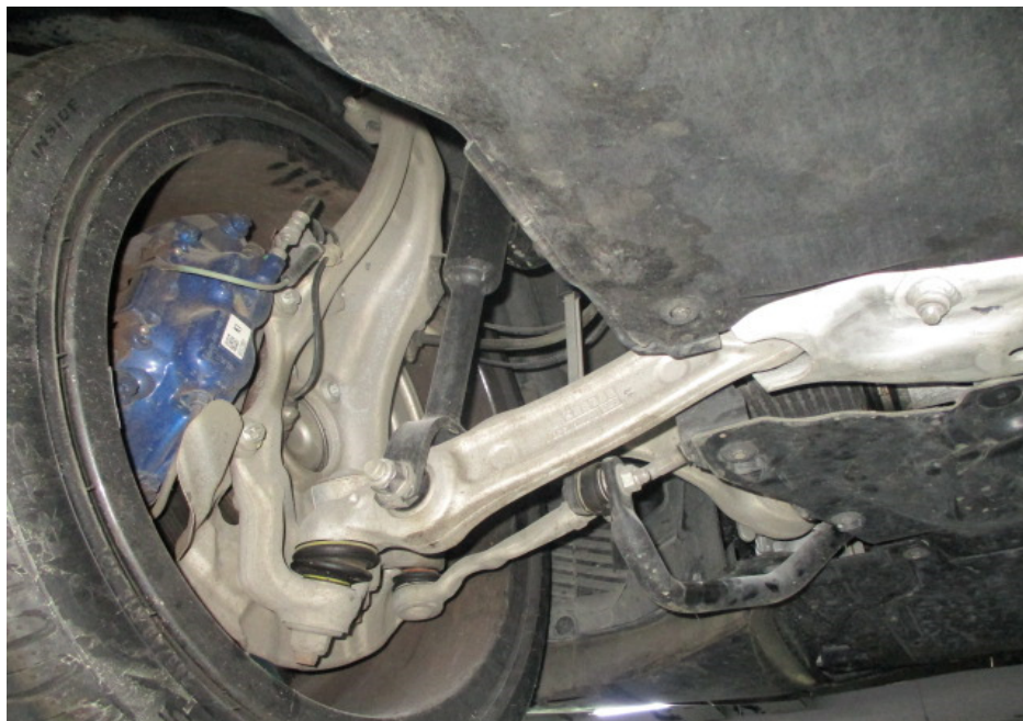
Photo 23 shows the various undercarriage components at the front left wheel of the Motor Car. The mechanical components, control arms and linkages were all found to be intact and secured in an appropriate manner. I also did not observe any fluid leak and/or fluid stain on the underside of the Motor Car.
