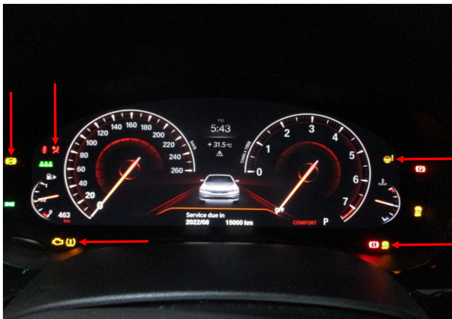
Photo 17 shows the warning lights for the various electronic safety features appearing on the instrument panel of the Motor Car during its self-test when the engine is cranked, in particular the ABS, SRS, IAS, TPM and DSC lights (arrowed).
