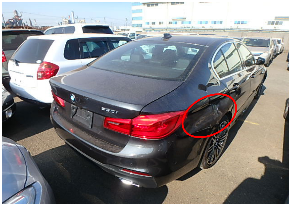
Photo 3 shows a general view of the rear right body of the Motor Car (photograph provided to me). Apart for the front right body, I had also observed damage to the Motor Car's rear right fender (circled).
