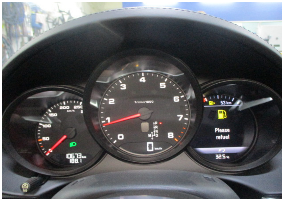
Photo 22 shows the respective warning lights no longer illuminated, indicating that there is no fault detected to the ABS, SRS, TPM and TCS systems of the Motor Car during the self-test. These electronic systems were hence in working condition at the time of my inspection.
