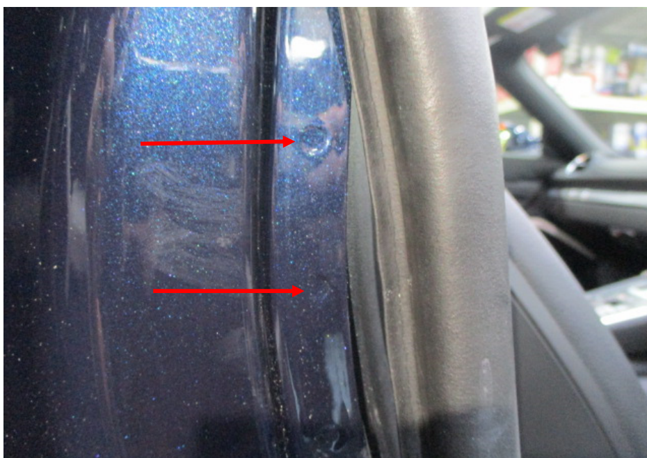
Photo 36 shows the rear right body panel of the Motor Car. I did not find any weld marks other than original spot weld marks (arrowed) on the rear right body panel of the Motor Car, which indicates that there was no re-welding works carried out. In general, I had found all the non-detachable body panels of the Motor Car to be originally fitted at the time of my inspection.
