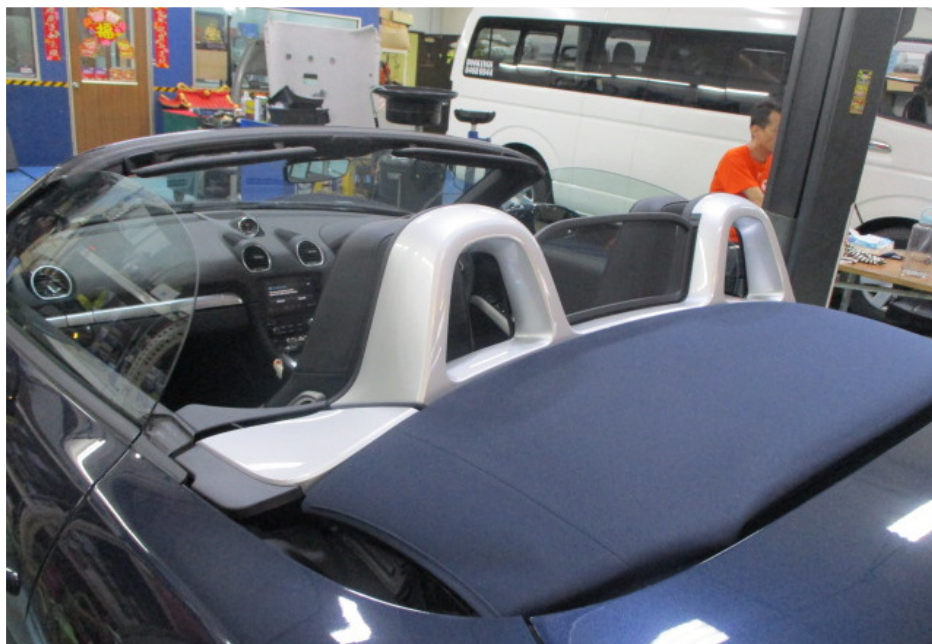
Photo 19 shows the Motor Car with its soft top roof in an open position. It was observed that as a safety feature, the soft top roof could only open and close when the Motor Car was in a stationary position. When in an open position, the soft top roof is completely folded into its rear compartment with no parts protruding out of the Motor Car's body. The soft top roof was also found adequately secured to the "A" pillar after closing.
