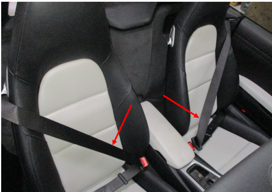
Photo 18 shows the seats of the Motor Car. All the seats of the Motor Car were secured via seat rails to the floorboard. They were also fitted with a retractable seat belt reel and a pre-tensioner. The seat belts (arrowed) were tested and were able to be fastened into the respective pre-tensions that were fitted on the side of each individual seat.
