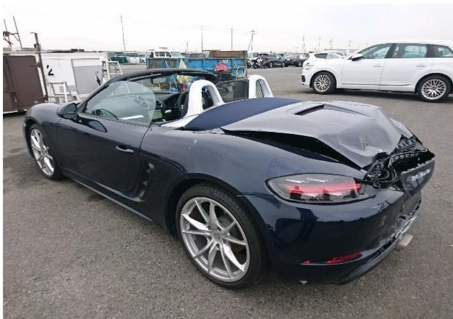
Photo 1 shows the rear left body of the Motor Car (photograph provided to me). The Motor Car was observed to have sustained damage at its rear portion. The rear bumper, rear bumper left reflector, rear bumper top centre garnish, rear bumper top lip, rear exhaust tip, rear left taillamp and rear bootlid were amongst the body parts that were observed to have been damaged.
