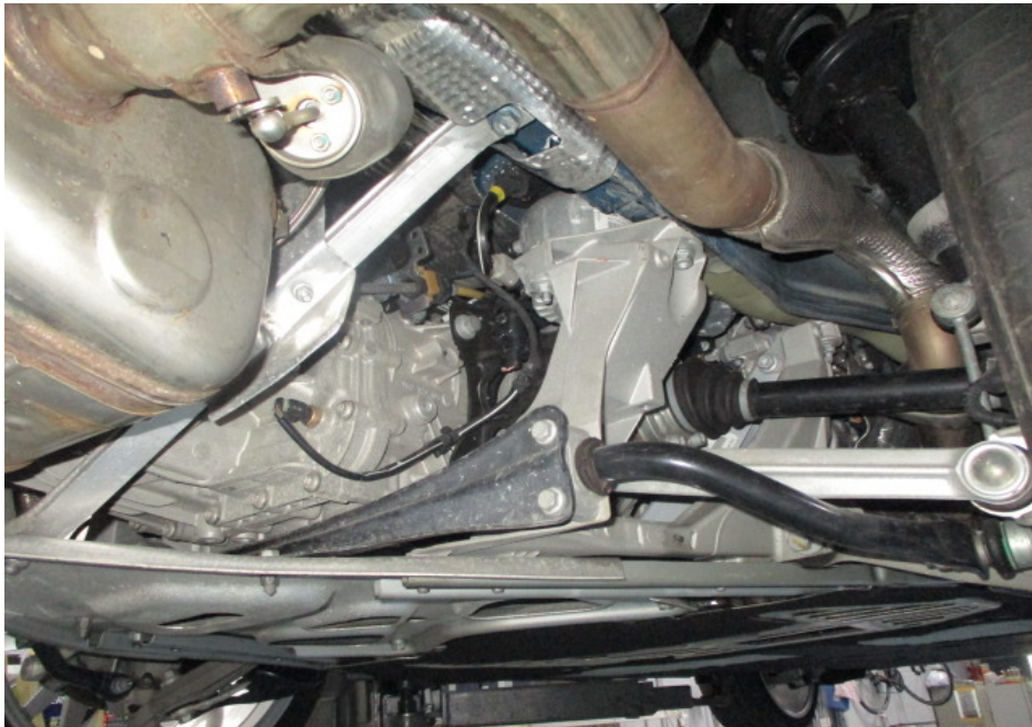
Photo 31 shows another view of the Motor Car's engine compartment. The engine compartment was at the rear underside of the Motor Car. The various parts and components inside the engine compartment were all observed to be intact and properly fitted. There was also no sign(s) or indication(s) of fluid leak and/or fluid stain found inside the engine compartment.
