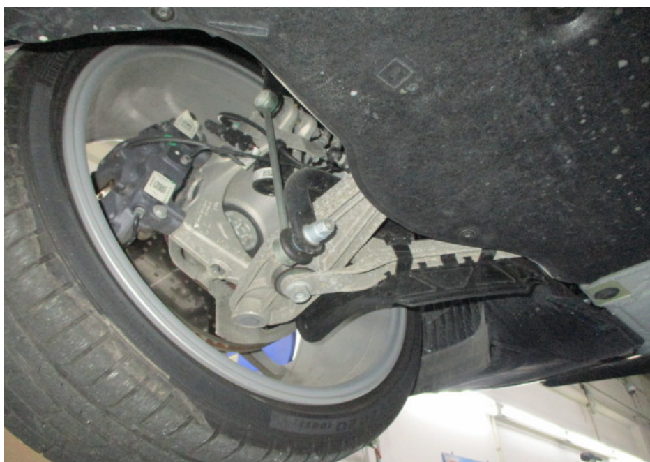
Photo 26 shows the various undercarriage components at the front left wheel of the Motor Car. The mechanical components, control arms and linkages were all found to be intact and secured in an appropriate manner.
