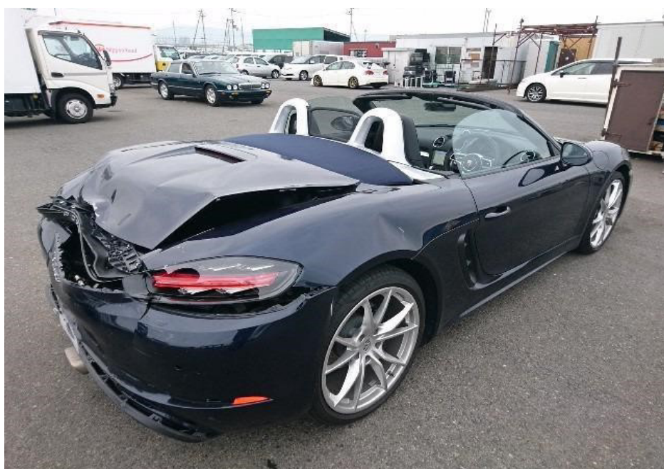
Photo 2 shows the rear right body of the Motor Car (photograph provided to me). The Motor Car was observed to have sustained damage at its rear portion. The rear bumper, rear bumper right reflector, rear bumper lower cover, rear right taillamp, rear bootlid and rear right body panel were amongst the body parts that were observed to have been damaged. As seen from the photographs, the airbags of the Motor Car were not deployed.
