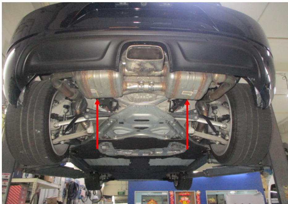
Photo 28 shows the Motor Car's rear mufflers (arrowed). My examination of the Motor Car's exhaust system revealed no sign(s) or indication(s) of any cut or weld marks along its exhaust pipes, on its catalytic converters and on its rear mufflers.
