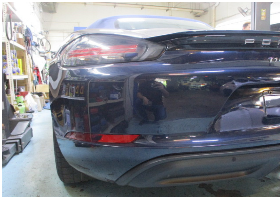
Photo 7 shows a closer view of the Motor Car's rear bumper, rear bumper left reflector, rear bumper lower cover and rear left taillamp. The body parts at the rear portion of the Motor Car were visually examined and it was observed that the repair/restoration works carried out to the damaged area of the Motor Car (refer to photograph 1 – 3 above) were reasonably adequate and in order.
