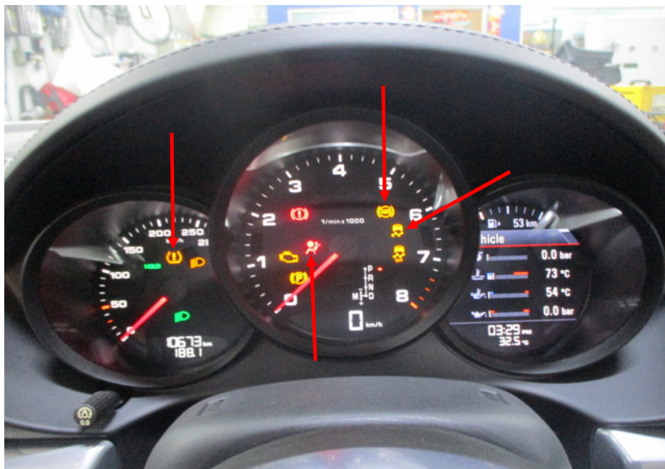
Photo 21 shows the warning lights for the various electronic safety features appearing on the instrument panel of the Motor Car during its self-test when the engine is cranked, in particular the ABS, SRS, TPM and TCS lights (arrowed).
