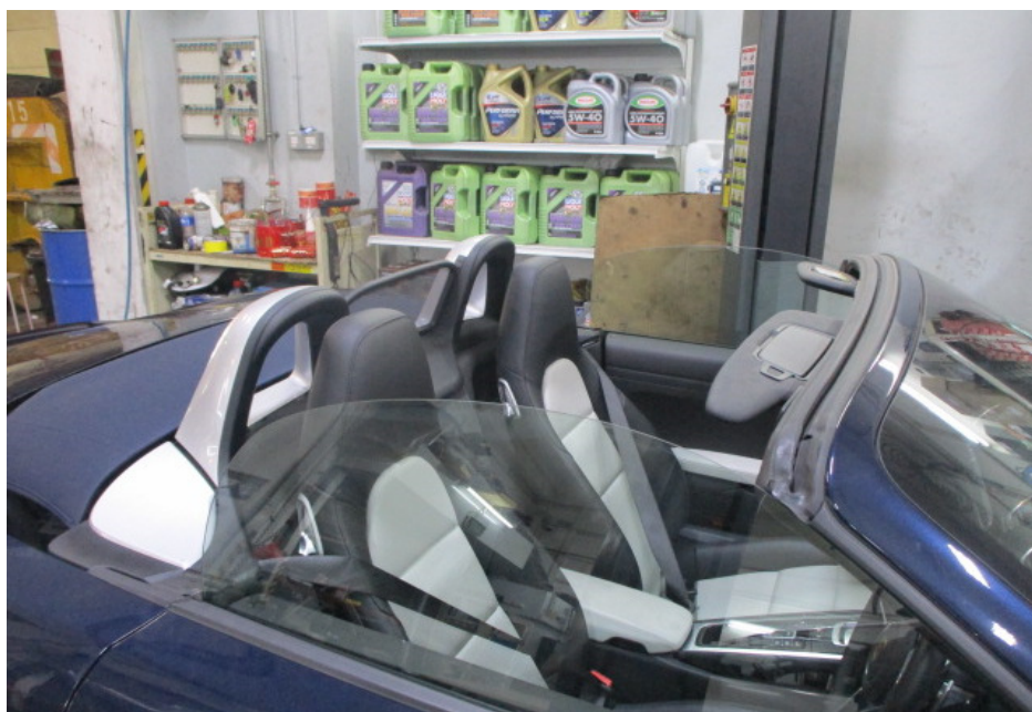
Photo 20 shows another view of the Motor Car with its soft top roof in an open position. It was observed that as a safety feature, the soft top roof could only open and close when the Motor Car was in a stationary position. When in an open position, the soft top roof is completely folded into its rear compartment with no parts protruding out of the Motor Car's body. The soft top roof was also found adequately secured to the "A" pillar after closing.
