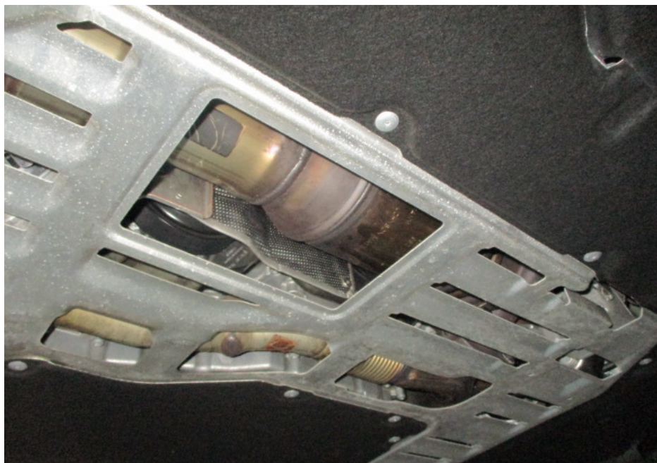
Photo 29 shows the Motor Car's catalytic converters. My examination of the Motor Car's exhaust system revealed no sign(s) or indication(s) of any cut or weld marks along its exhaust pipes, on its catalytic converters and on its rear mufflers.
