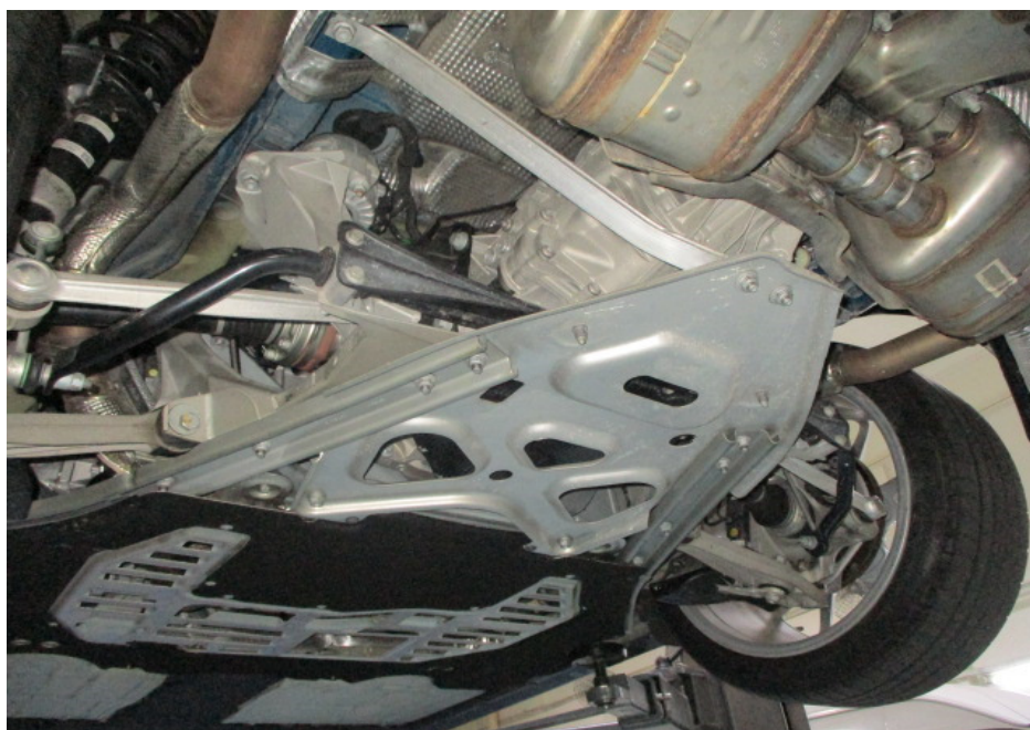
Photo 30 shows a general view of the Motor Car's engine compartment. The engine compartment was at the rear underside of the Motor Car. The various parts and components inside the engine compartment were all observed to be intact and properly fitted. There was also no sign(s) or indication(s) of fluid leak and/or fluid stain found inside the engine compartment.
