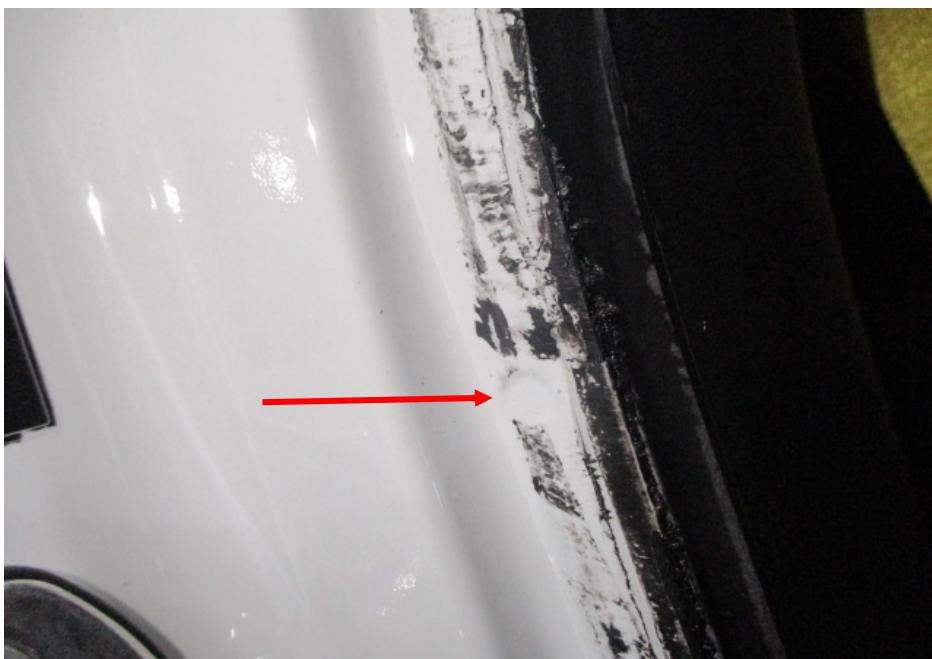
Photo 35 shows the rear right body panel of the Motor Car. I did not find any weld marks other than original spot weld marks (arrowed) on the rear right body panel of the Motor Car, which indicates that there was no re-welding works carried out. In general, I had found all the non-detachable body panels of the Motor Car to be originally fitted at the time of my inspection.
