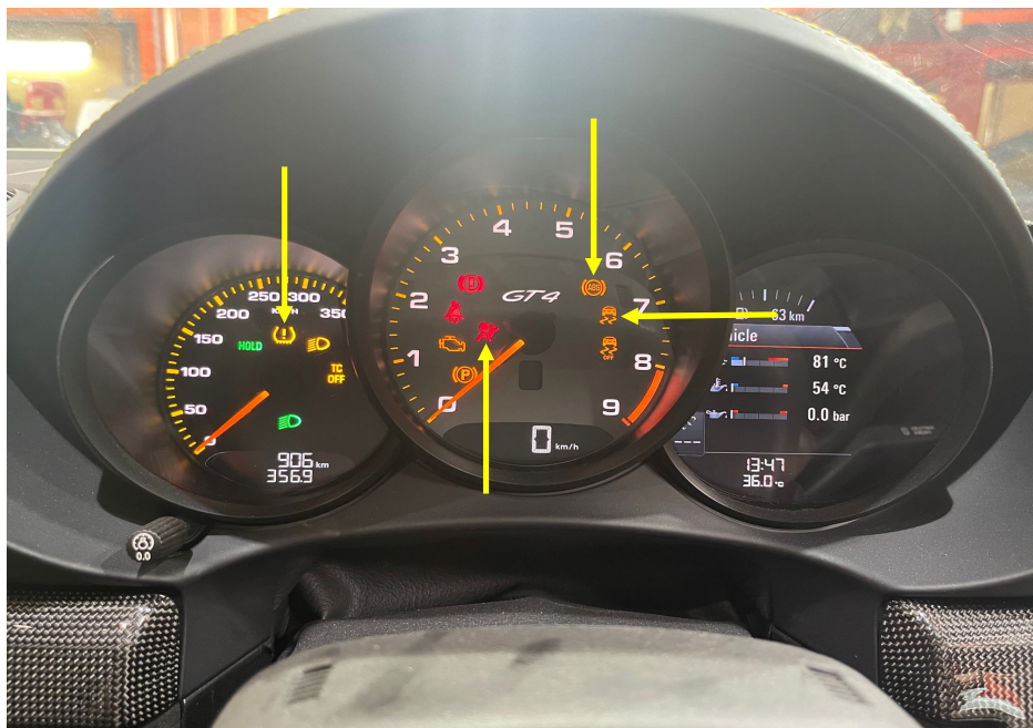
Photo 20 shows the warning lights for the various electronic safety features appearing on the instrument panel of the Motor Car during its self-test when the engine is cranked, in particular the ABS, SRS, TPM and TCS lights (arrowed).
