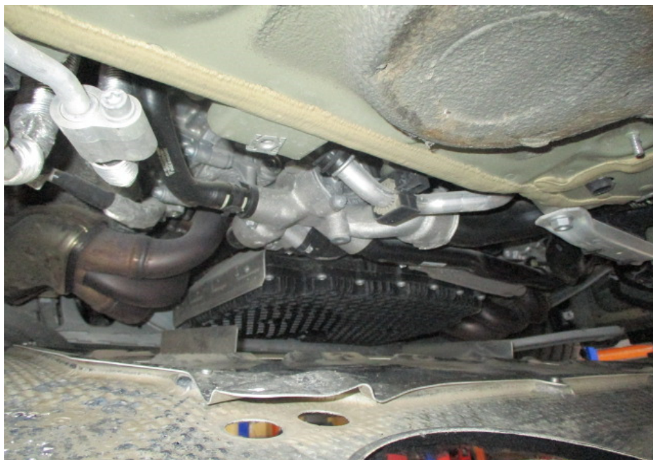
Photo 28 shows a general view of the engine compartment of the Motor Car at the time of my inspection. The engine compartment was at the rear underside of the Motor Car. The various parts and components inside the engine compartment were all observed to be intact and properly fitted. There was also no sign(s) or indication(s) of fluid leak and/or fluid stain found inside the engine compartment.
