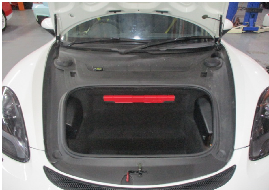
Photo 9 shows a general of the Motor Car's front bonnet compartment at the time of my inspection. All inner trims, garnishes and upholstery etc were observed to be properly fitted. The body parts at the front left portion of the Motor Car were visually examined and the repair/restoration works carried out to the damaged area of the Motor Car (refer to photograph 1 above) were found to be reasonably adequate and in order.
