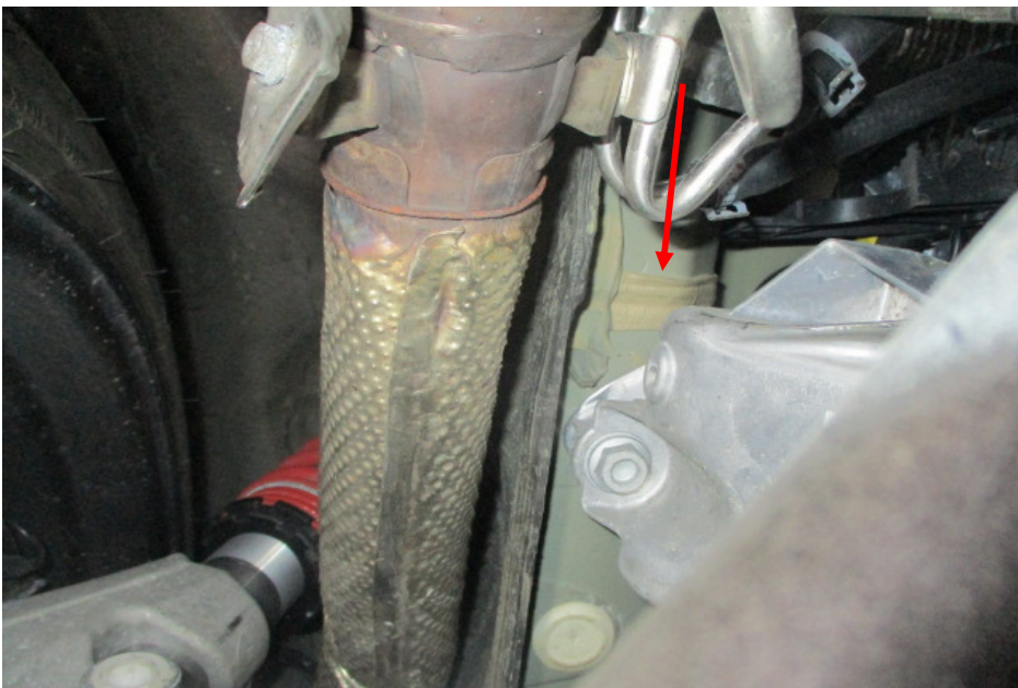
Photo 31 shows the chassis/structural body at the underside rear left of the Motor Car. I did not find any weld marks other than original spot weld marks on the chassis/structural body of the Motor Car. The original factory sealant (arrowed) at the joints along the chassis/structural body was untouched, indicating no work was done on the chassis/structural body of the Motor Car and that the chassis/structural body was originally fitted.
