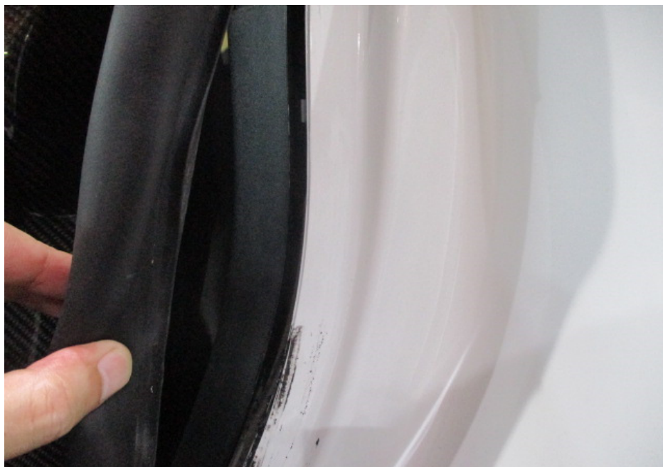
Photo 34 shows the rear left body panel of the Motor Car. I did not find any original weld marks at the rear left body panel of the Motor Car, indicating that the rear left body panel of the Motor Car was replaced. The lack of original weld marks seen was due to replacement work when the replaced rear left body panel was re-welded onto the Motor Car and smoothen for re-spraying work.
