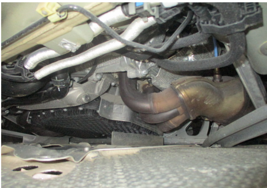
Photo 29 shows another view of the engine compartment of the Motor Car at the time of my inspection. The engine compartment was at the rear underside of the Motor Car. The various parts and components inside the engine compartment were all observed to be intact and properly fitted. There was also no sign(s) or indication(s) of fluid leak and/or fluid stain found inside the engine compartment.
