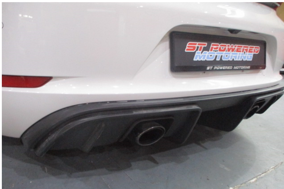
Photo 12 shows a closer view of the Motor Car's rear bumper, rear bumper left reflector, rear bumper lower diffuser and rear left exhaust at the time of my inspection. The body parts at the rear left portion of the Motor Car were visually examined and it was observed that the repair/restoration works carried out to the damaged area of the Motor Car (refer to photograph 3 above) were reasonably adequate and in order.
