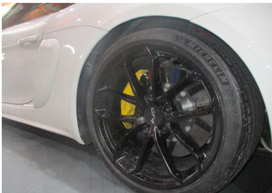
Photo 15 shows a closer view of the Motor Car's rear left wheel rim and rear left body panel at the time of my inspection. The body parts at the rear left portion of the Motor Car were visually examined and it was observed that the repair/restoration works carried out to the damaged area of the Motor Car (refer to photograph 3 above) were reasonably adequate and in order.
