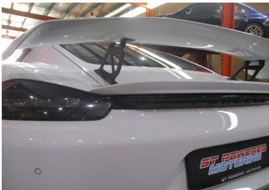
Photo 13 shows a closer view of the Motor Car's rear bumper, rear bumper top centre garnish, rear bumper top lip and rear left taillamp at the time of my inspection. The body parts at the rear left portion of the Motor Car were visually examined and it was observed that the repair/restoration works carried out to the damaged area of the Motor Car (refer to photograph 3 above) were reasonably adequate and in order.
