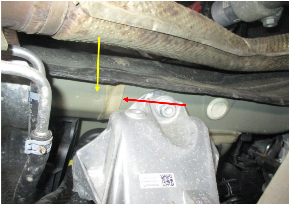
Photo 30 shows the chassis/structural body at the underside rear right of the Motor Car. I did not find any weld marks other than original spot weld marks (yellow arrow) on the chassis/structural body of the Motor Car. The original factory sealant (red arrow) at the joints along the chassis/structural body was untouched, indicating no work was done on the chassis/structural body of the Motor Car and that the chassis/structural body was originally fitted.
