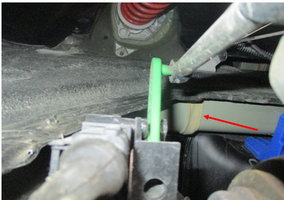
Photo 33 shows the chassis/structural body at the underside front right of the Motor Car. The original factory sealant (arrowed) at the joints along the chassis/structural body was observed to be untouched. In general, I had found no work was carried out on the chassis/structural body of the Motor Car. The chassis/structural body of the Motor Car was originally fitted.
