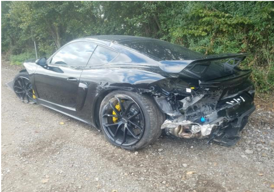
Photo 3 shows the rear left body of the Motor Car (photograph provided to me). Apart for the front left portion, the Motor Car had also sustained damage at its rear left portion. The rear bumper, rear bumper lower diffuser, rear bumper reinforcement, rear bumper left reflector, rear bumper top centre garnish, rear bumper top lip, rear left exhaust, rear left exhaust heat shield, rear left taillamp, rear left body panel, rear left body panel inner shield and rear left wheel rim were amongst the body parts that were observed to have been damaged.
