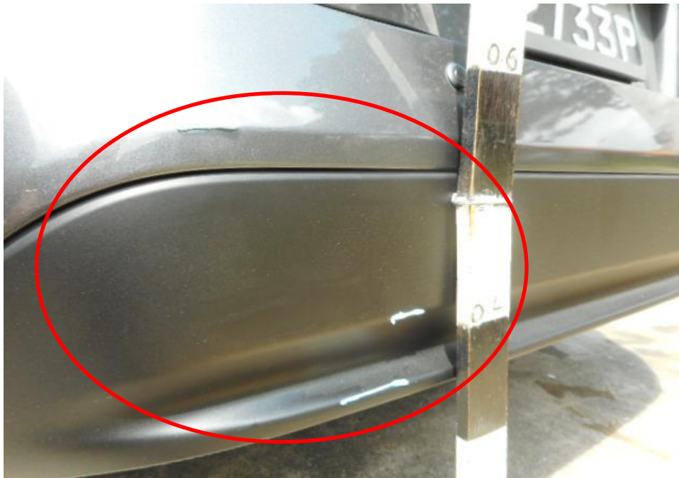
Photo 2 shows the close up view of the rear left portion of Toyota at the time of inspection. The rear bumper (circled) had been damaged.
