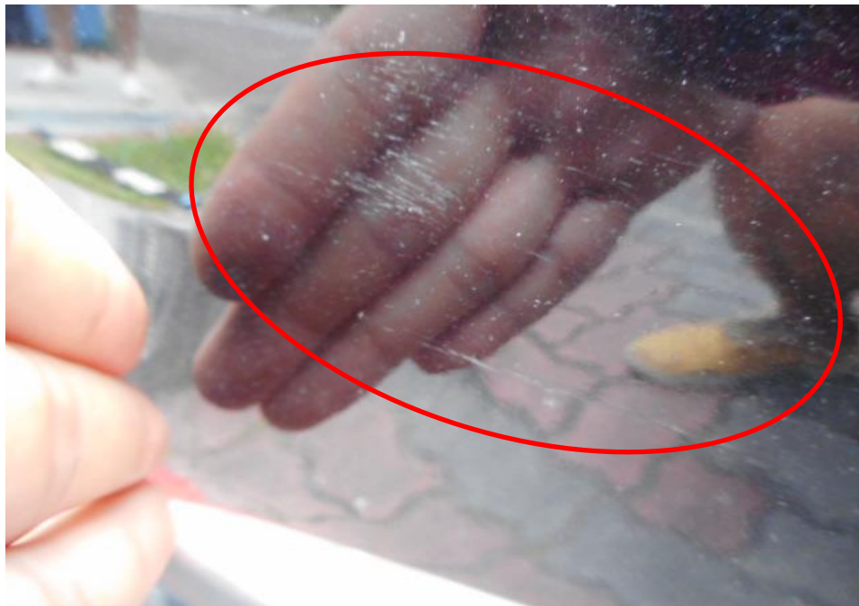
Photo 6 shows the close up view of the front right portion of Kia at the time of inspection. The front bumper right portion (circled) had paint scratch marks.
