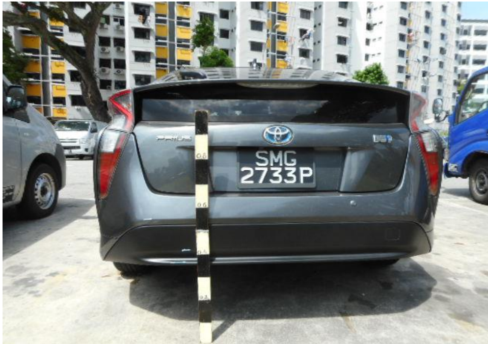
Photo 9 shows the general view of the height measurement being conducted on the rear portion of Toyota. The height above ground level of where the scratches of the rear bumper left portion, was at, 38cm, 42cm and 54cm respectively.
