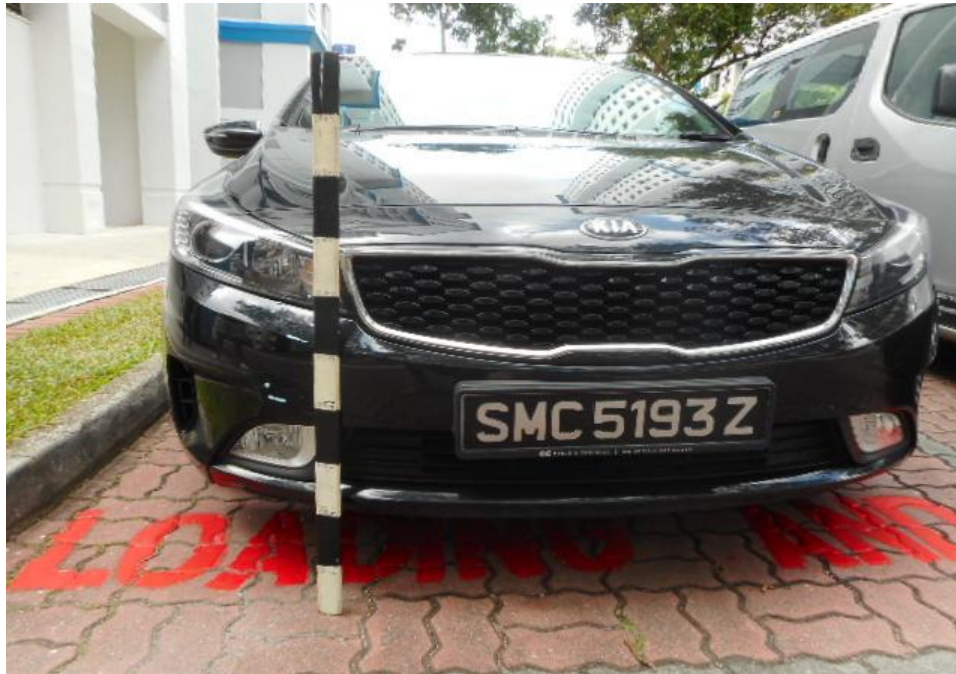
Photo 10 shows a general view of the height measurement being conducted on the front portion of Kia. The front bumper right portion where is the, was measured to be at 42cm, 45cm and 52cm above ground level.
