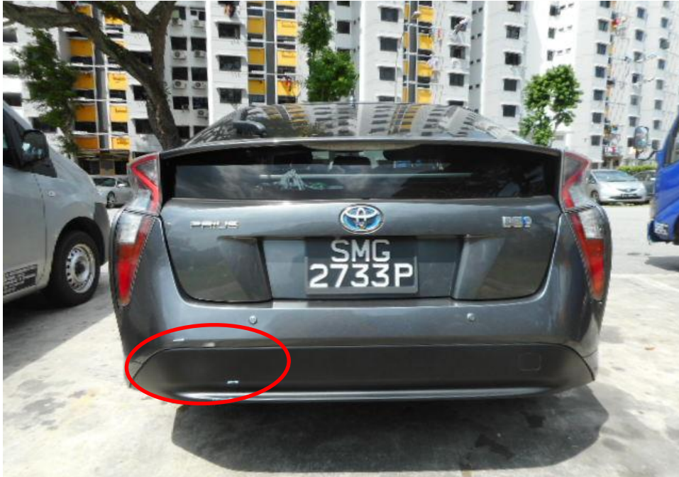
Photo 1 shows the general view of the rear portion of Toyota at the time of inspection. The rear bumper (circled) had been damaged.
