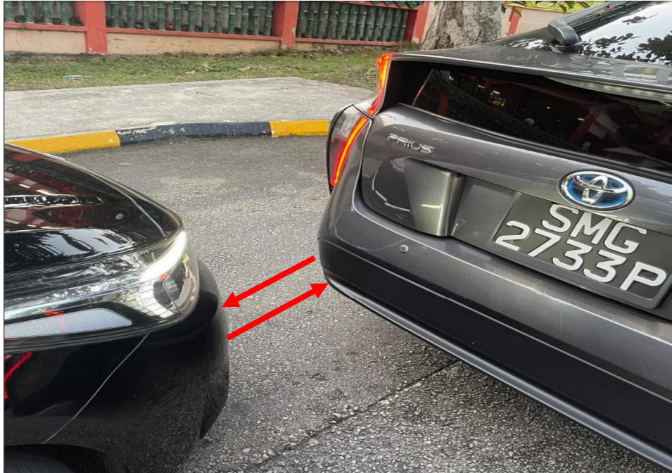
Photo 7 shows a general view of the Kia behind the Toyota. The Kia's front bumper right portion is directly behind the Toyota's rear bumper left portion. These is likely the area where the damages might have been at on the Toyota and the Kia (arrowed).
