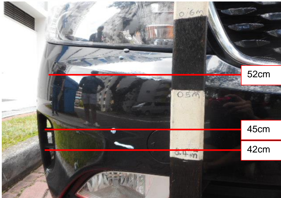
Photo 12 shows the close up view of the height measurement being conducted on the front bumper right portion of the Kia. The scratched marks found on the front bumper left portion was measured to be between 42cm, 45cm and 52cm above ground level.
