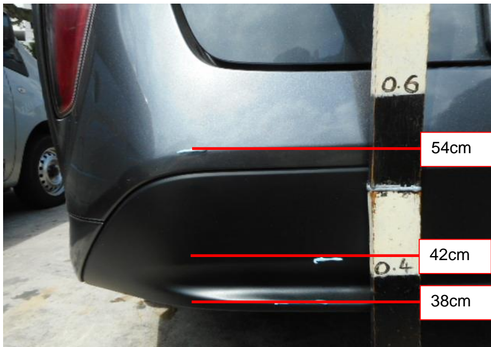
Photo 11 shows the close up view of the height measurement being conducted on the rear portion of Toyota. The height above ground level of where the damage were found on the rear bumper left portion of the Toyota was between 38cm, 42cm and 54cm.
