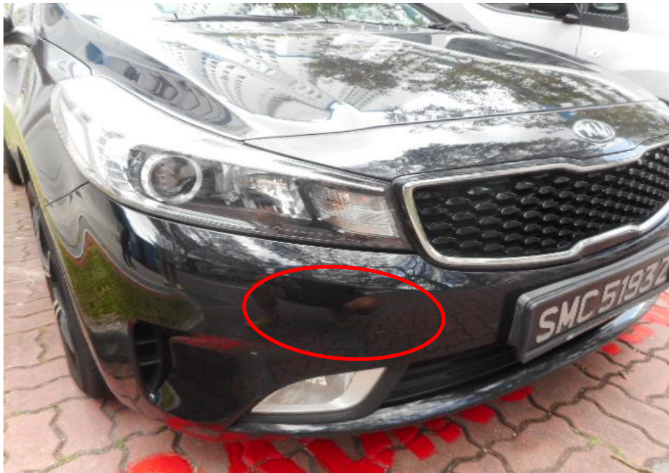
Photo 4 shows the close up view of the front right portion of Kia at the time of inspection. The front bumper right portion (circled) had paint scratch marks.
