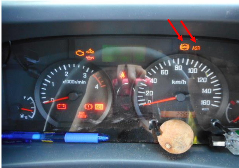
Photo 25 shows the warning light for Anti-Lock Brake System (ABS) and Traction Control System (TC) (arrowed) appearing on the instrument panel of the Motor Van during the self-test of its various electronic operating systems when its engine was cranked.
