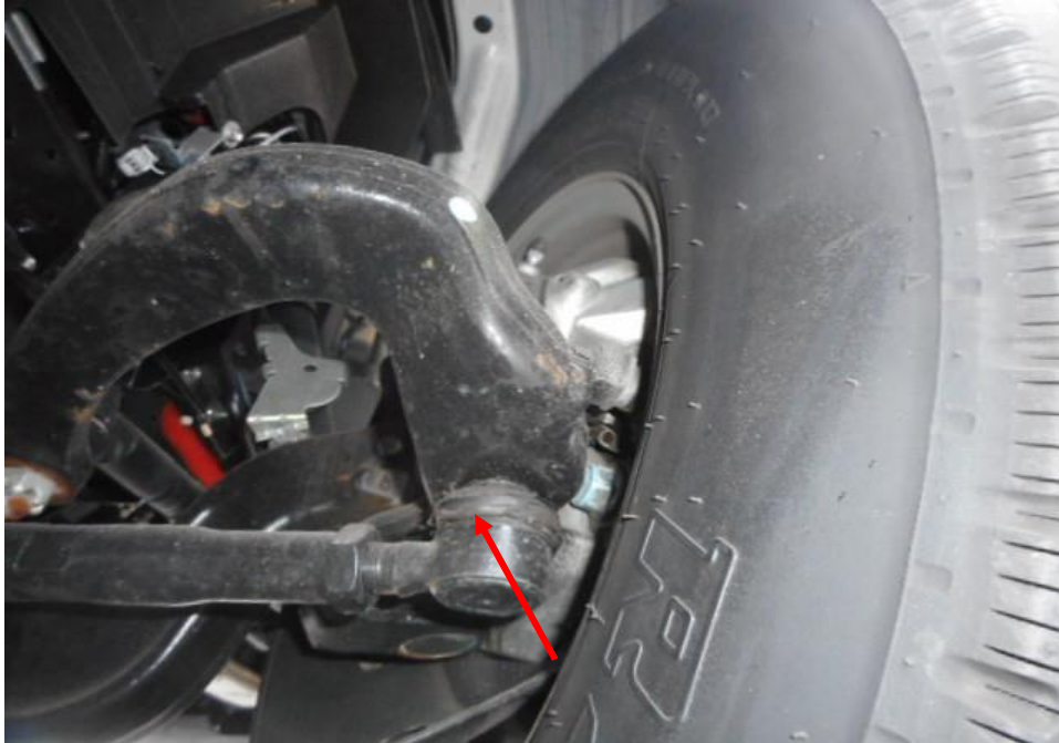
Photo 18 shows the various undercarriage components at the front right wheel of the Motor Lorry, in particular the steering tie rod end (arrowed). The various steering components were all found to be intact, suggesting that the steering system of the Motor Lorry was likely to be in serviceable condition at the material time of accident. There was also no sign of fluid stain(s) observed on the various undercarriage components.
