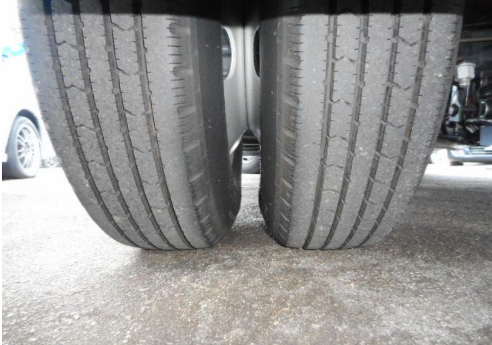
Photo 10 shows the condition of the rear left tyres of the Motor Lorry, which was observed to be in serviceable condition with remaining tread depth of approximately 7.8mm. The tyres, which were wrapped around standard steel wheel rim, were also observed to be sufficiently inflated for vehicular operation. There was also no damage found on all 6 steel wheel rims of the Motor Lorry.
