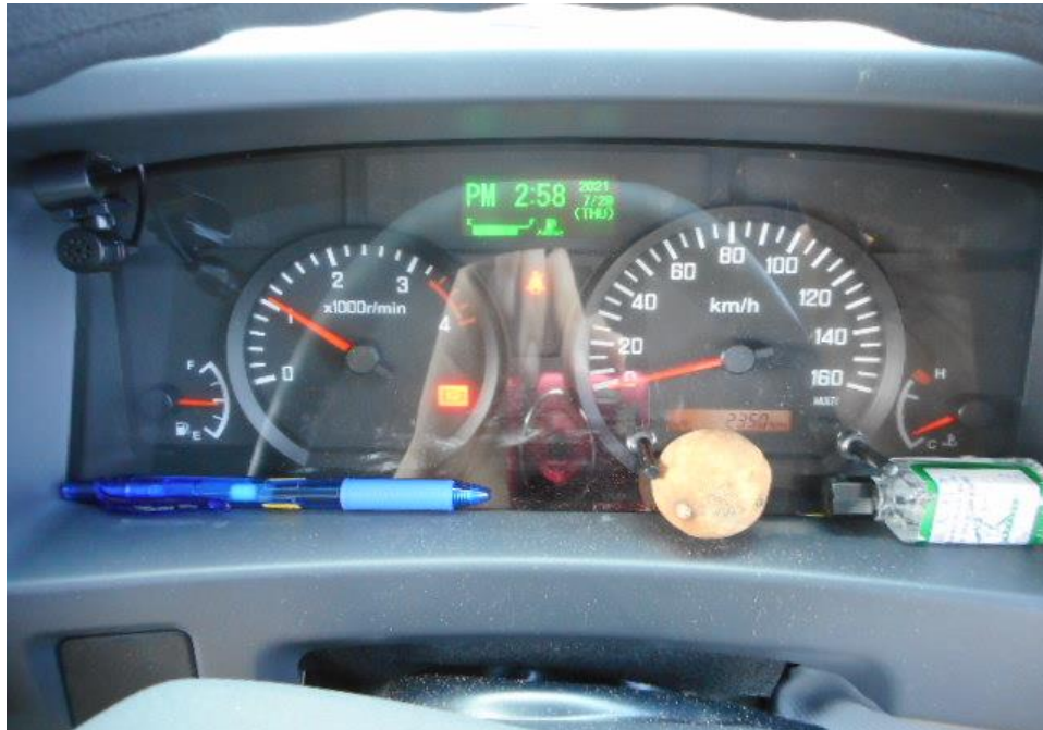
Photo 26 shows no warning lights illuminated on the instrument panel of the Motor Van after the engine was cranked. This would suggest that there was no abnormality to the electronic operating system of the Motor Van, like the ABS and TC etc.
