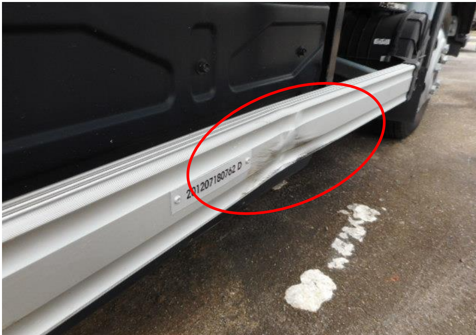
Photo 5 shows a close up view of the Motor Lorry's right portion at the time of my inspection. It appeared to have sustained damage at its right portion. Its right guard rail (circled) were damage at the time of my inspection as a result of the accident.
