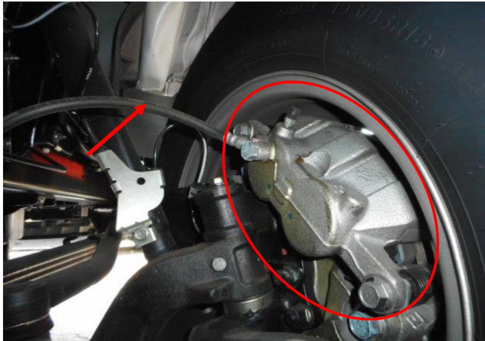
Photo 22 shows the brake hose/pipe (arrowed) at the front right wheel of the Motor Lorry. No leakage of brake fluid was observed. Visual examination of the various components of the braking system like the brake caliper (circled), brake booster, brake pedal etc had revealed all to be intact and without visible damage at the time of accident. There was also no sign of fluid stain(s) observed on the various undercarriage components.
