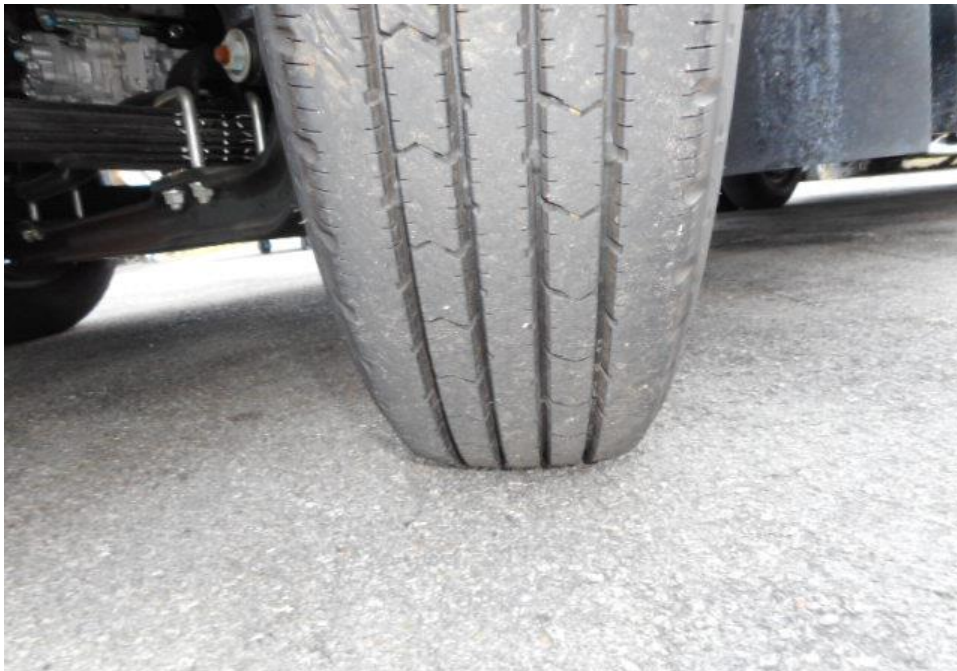
Photo 11 shows the condition of the rear right tyres of the Motor Lorry, which were observed to be in serviceable condition with remaining tread depth of approximately 6.7mm. There was also no tear, cut or burst mark(s) on the outer and the inner sidewalls as well as across the tread of the 6 tyres that were fitted on the Motor Lorry.
