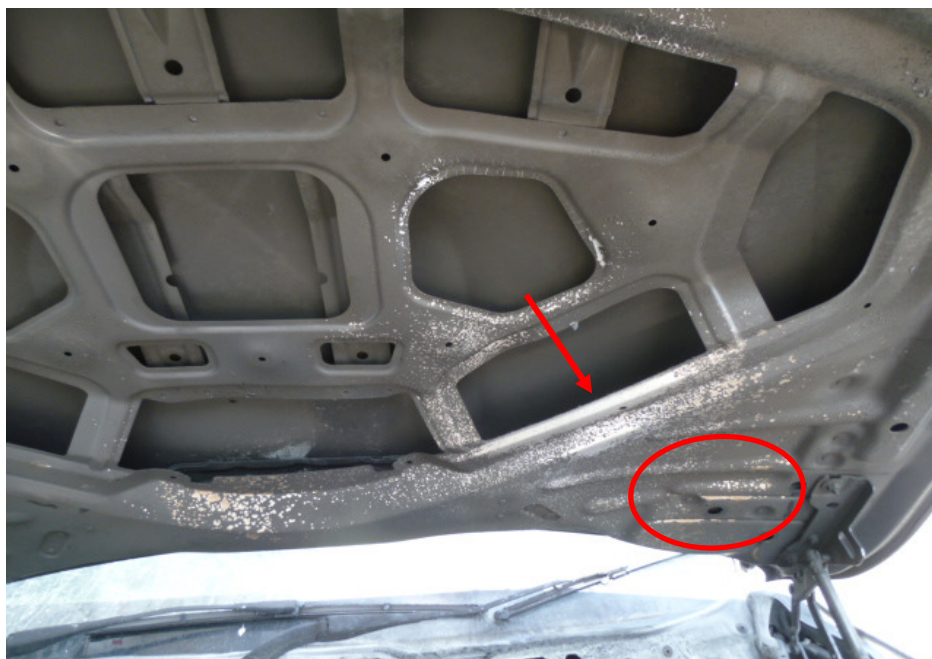
Photo 8 shows the faint whitish burn marks on the bottom left portion on the underside of the bonnet (arrowed) and the rust (circled) that had developed on the underside of the front bonnet, around the bottom left area. The development of rust is an indication that this area was exposed to prolonged exposure to high heat intensity, which had caused the steel/metal material of the front bonnet to be exposed to natural environmental condition. Hence the fire to the Insured Vehicle can be determined to have originated towards the rear left portion of the engine compartment.
