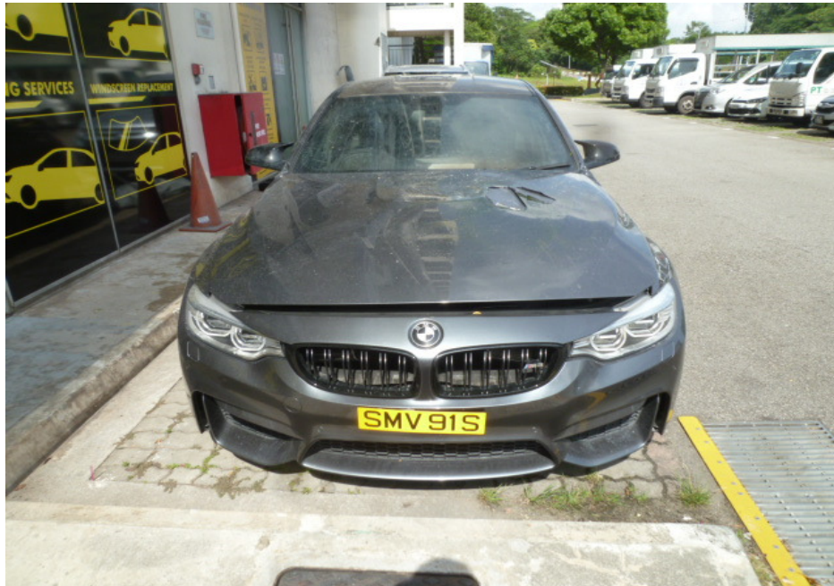
Photo 1 shows the general view of the frontal portion of the Insured Vehicle at the time of our inspection. The exterior body of the Insured Vehicle had sustained visible fire damage. This included its front windscreen and front bonnet.
