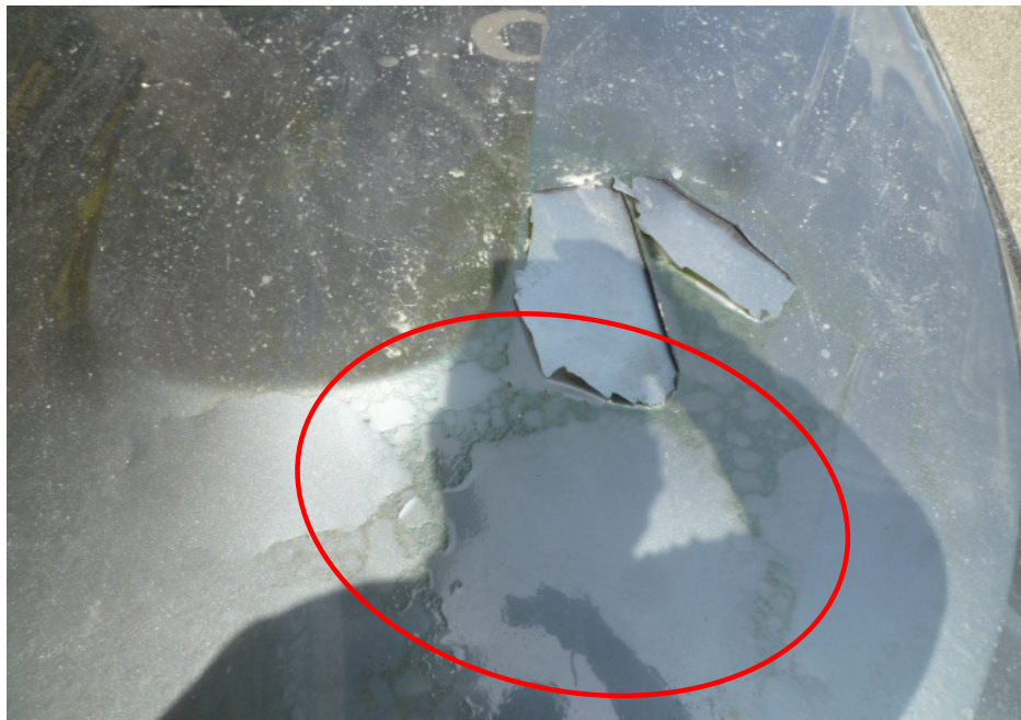
Photo 7 shows paint bubbles on the rear left portion of the front bonnet (circled).
