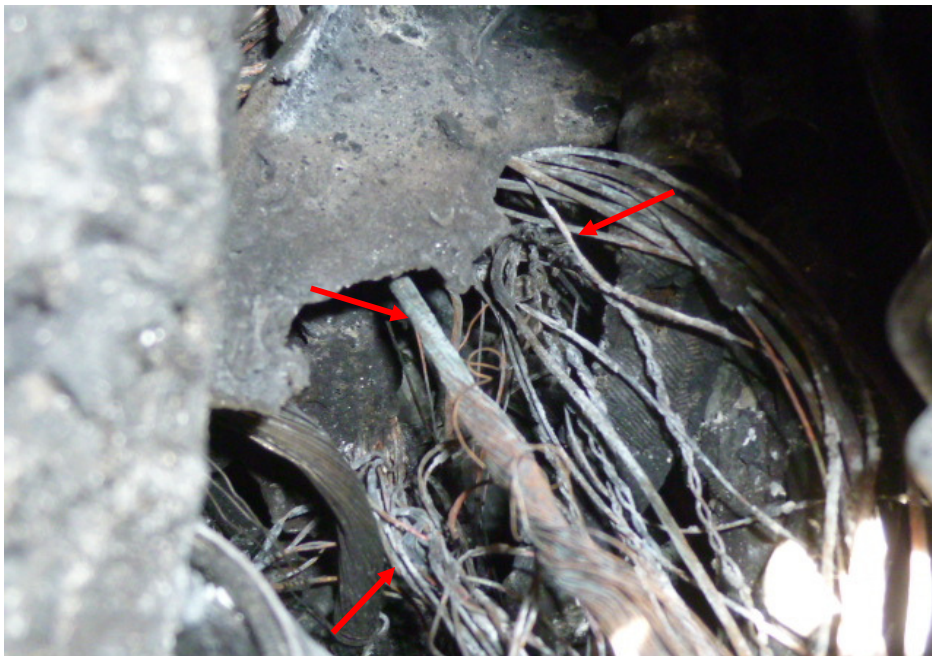
Photo 13 shows a close up view of the greenish residue found on several stretches of burnt wirings (red arrows). The presence of such greenish residue suggests occurrence of an electrical short circuit.
