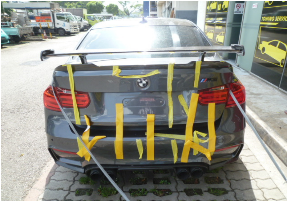
Photo 3 shows the general view of the rear portion of the Insured Vehicle at the time of our inspection. The fire damage was confined to its engine compartment. The rear portion of the Insured Vehicle was observed to be relatively unaffected by the fire.
