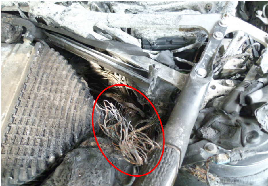
Photo 10 shows a closer view of the burnt wirings around the rear left portion of the engine compartment, which is in the immediate vicinity where the fire to the Insured Vehicle had likely started. We noticed greenish residue on several stretches of burnt wirings (circled). The presence of greenish residue indicates internal heating of copper wires, a sign of an electrical short circuit occurring. The greenish residue is normally left behind from oxidation as a result of chemical reaction involving the copper wires.
