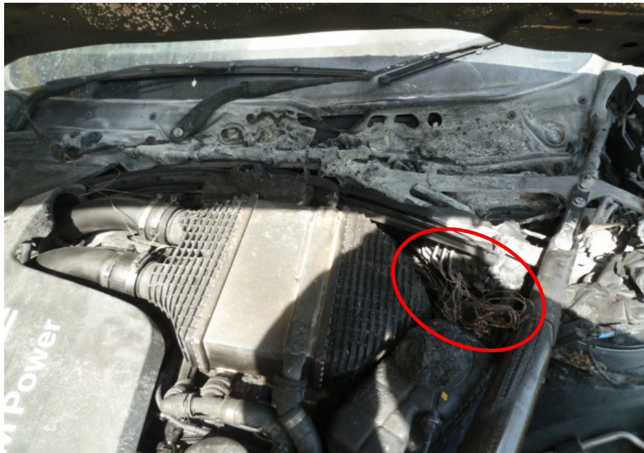
Photo 9 shows the burnt wirings around the rear left portion of the engine compartment (circled), which is in the immediate vicinity where the fire to the Insured Vehicle had likely started.
