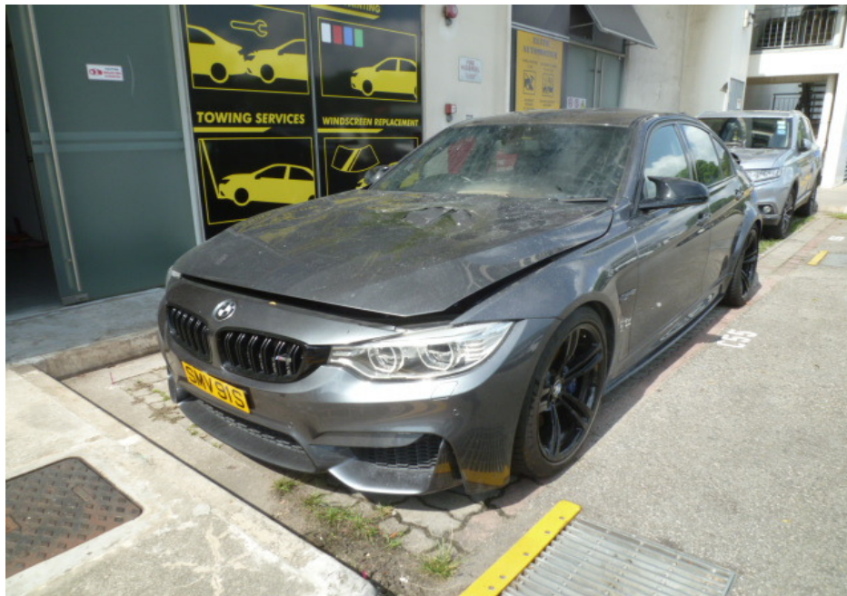
Photo 2 shows the general view of the left frontal portion of the Insured Vehicle at the time of our inspection. The exterior body of the Insured Vehicle had sustained visible fire damage. This included its front windscreen and front bonnet.
