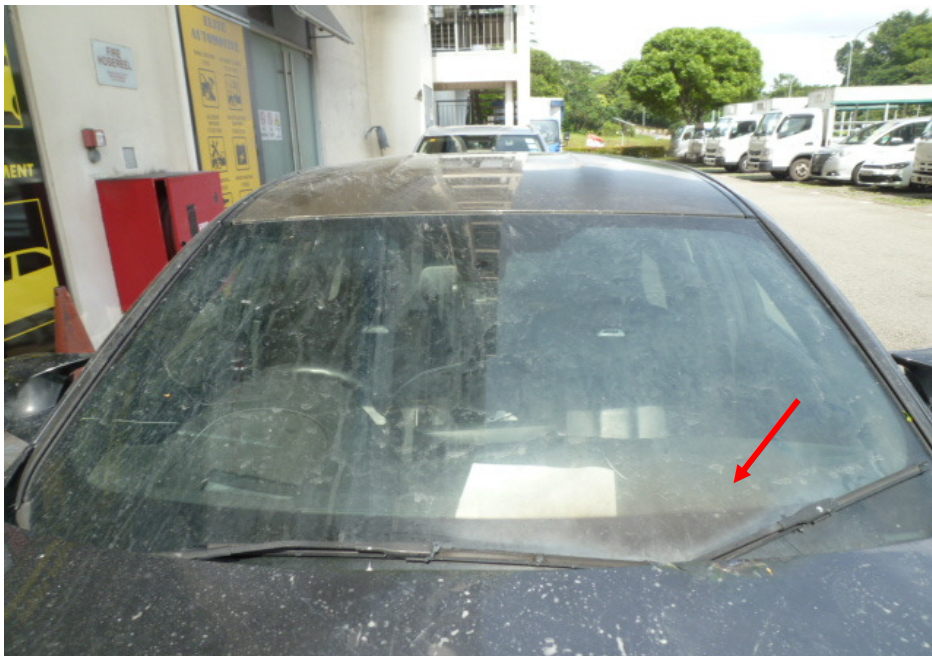
Photo 4 shows a closer view of the front windscreen of the Insured Vehicle at the time of our inspection. The front windscreen had sustained minor fire damage at the lower left portion (arrowed).
