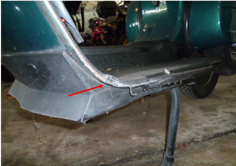
Photo 8 shows the grazed left bottom cowling (arrowed) of the Motorcycle as a result of the accident.
