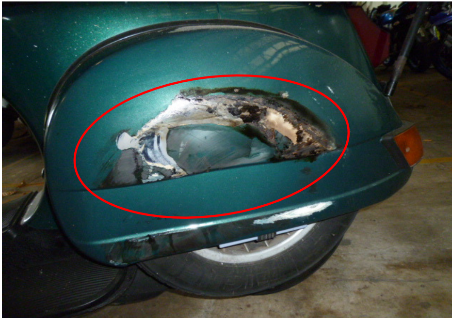
Photo 6 shows the dented left rear side cover (circled) of the Motorcycle as a result of the accident.
