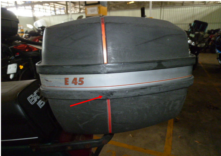
Photo 9 shows the grazed top box (arrowed) of the Motorcycle as a result of the accident.
