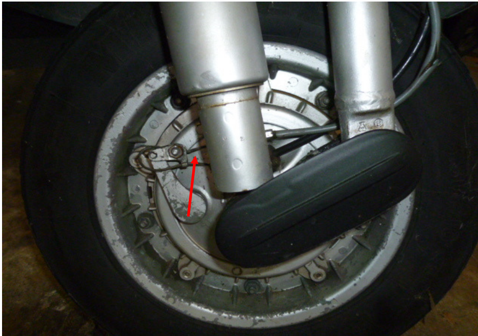
Photo 19 shows the front wheel of the Motorcycle. The type of brake system for the front wheel was of a mechanical type, controlled by the front brake lever of the Motorcycle. Our checks of the cable (arrowed), spring and drum which are all part of the components in the front brake system of the Motorcycle reveal all to be intact and without damage.
