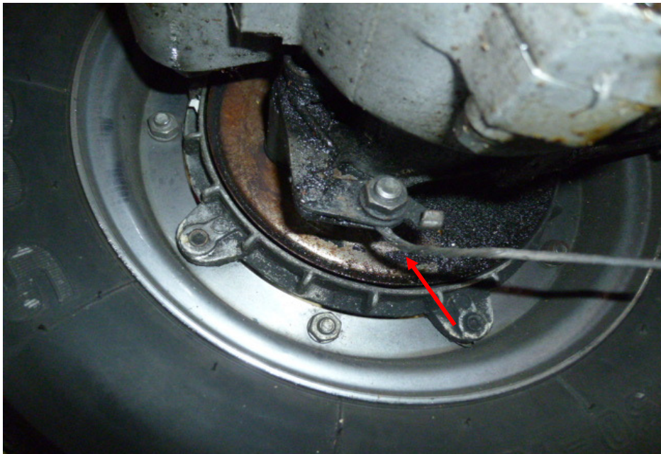
Photo 20 shows the rear wheel of the Motorcycle. The type of brake system for the rear wheel was of a mechanical type, controlled by the brake foot pedal of the Motorcycle. Our checks of the cable (arrowed), spring and drum which are all part of the components in the rear brake system of the Motorcycle reveal all to be intact and without damage.
