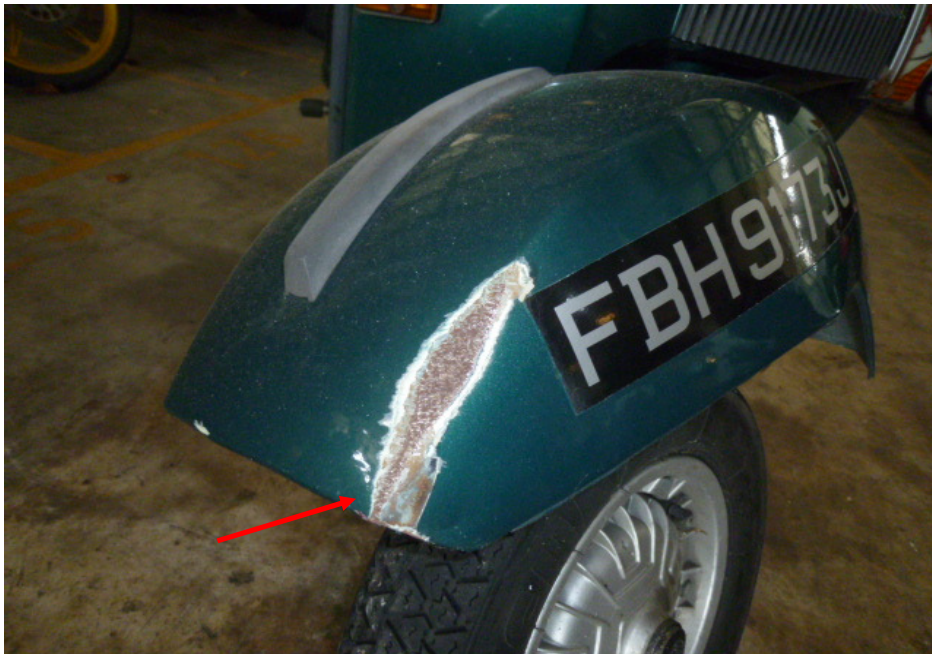
Photo 5 shows the damaged front mudguard (arrowed) of the Motorcycle. The damage sustained was again mainly of grazing nature.
