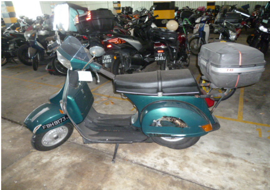
Photo 3 shows a general view of the left body of the Motorcycle at the time of our inspection. The Motorcycle was observed to have sustained damages at its left body. Amongst the body parts that were found to have been damaged include its front mudguard, left front signal lamp, left side mirror, clutch lever, left rear side cover, left bottom cowling and top box, amongst others.
