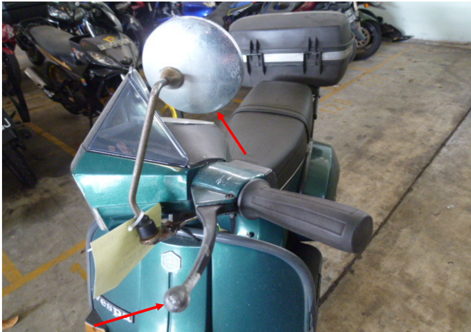
Photo 4 shows a closer view of the clutch lever and left side mirror (arrowed) which were amongst the body parts of the Motorcycle that had sustained damage as a result of the accident.
