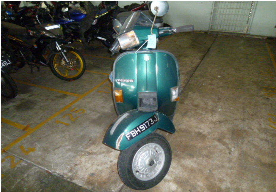
Photo 18 shows the front wheel of the Motorcycle turned towards its full right. Turning the Motorcycle's handle bar towards the left and right did not produce any abnormal free play and/or resistance. This would indicate that the steering system of the Motorcycle was in serviceable condition at the time of our inspection.
