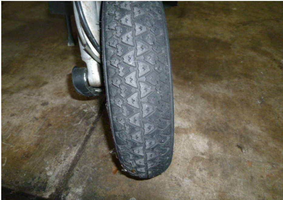
Photo 10 shows the condition of the Motorcycle's front tyre. The front tyre was observed to be in serviceable condition with remaining tread depth of approximately 3mm. There was no tear, burst mark(s) and/or punctured hole(s) on the sidewalls as well as across the tread of the front tyre.
