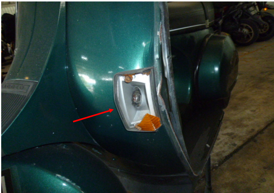
Photo 7 shows the cracked left front signal lamp (arrowed) of the Motorcycle as a result of the accident.
