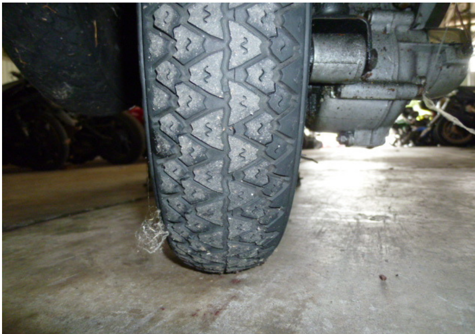
Photo 11 shows the condition of the Motorcycle's rear tyre. The rear tyre was observed to be in serviceable condition with remaining tread depth of approximately 3mm. The tyre was also observed to be sufficiently inflated for vehicular operation. We did not observe any tear, burst mark(s) and/or punctured hole(s) on the sidewalls as well as across the tread of the rear tyre.
