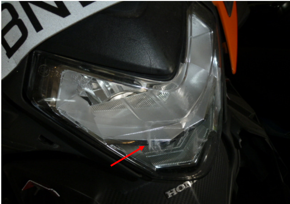
Photo 4 shows a closer view of the headlight assembly which was amongst the body parts at the front body of the Motorcycle that had sustained damage as a result of the accident (arrowed).
