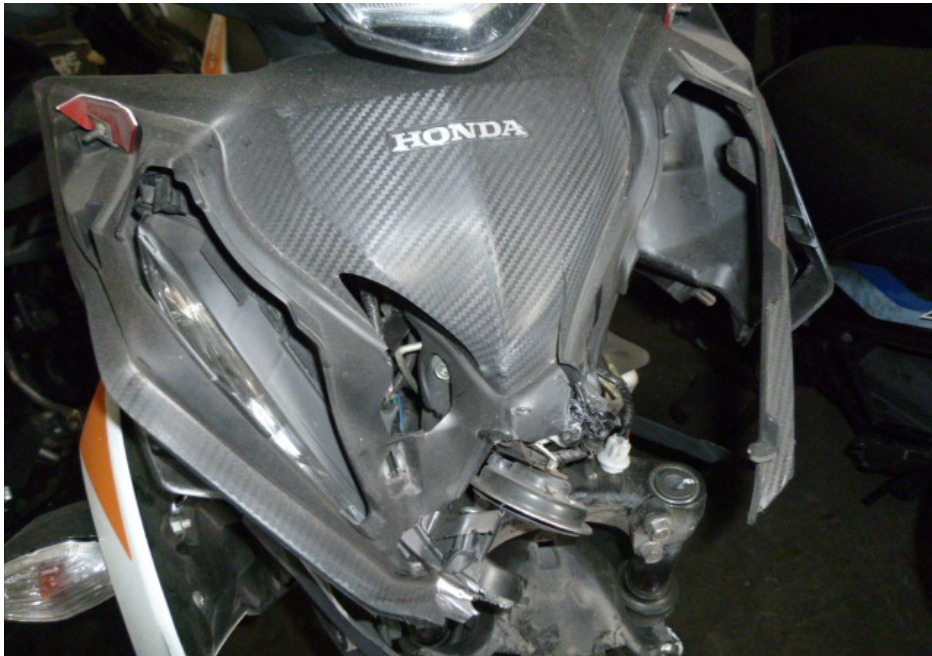
Photo 5 shows a closer view of the front cowling which was amongst the body parts at the front body of the Motorcycle that had sustained damage as a result of the accident.
