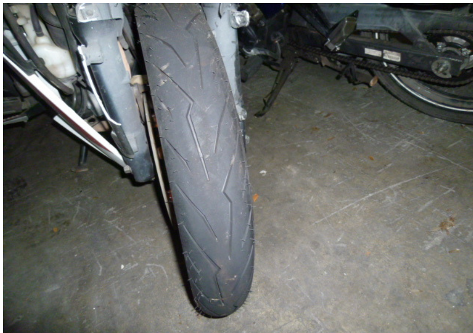
Photo 11 shows the front tyre of the Motorcycle at the time of our inspection. The pattern of the tread was clearly visible with remaining tread depth of approximately 4mm. We did not observe any tear, burst mark(s) and/or punctured hole(s) on the sidewalls as well as across the tread of the front tyre. However we did observe that the front tyre was deflated due to the broken front wheel rim.
