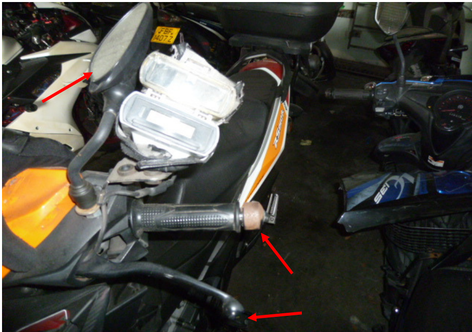
Photo 7 shows a closer view of the left side mirror, clutch lever and left handlebar end of the Motorcycle (arrowed). These parts were amongst the body parts of the Motorcycle which were damaged as a result of the accident.
