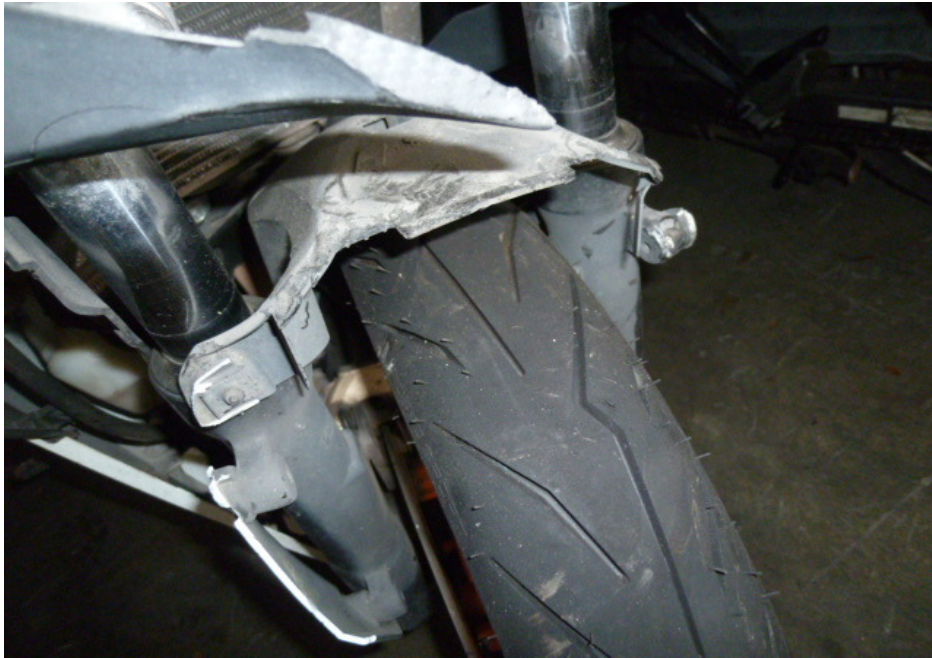
Photo 6 shows a closer view of the front mudguard which was amongst the body parts at the front body of the Motorcycle that had sustained damage as a result of the accident.
