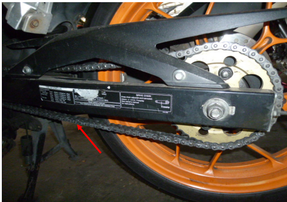
Photo 16 shows the gear chain (arrowed) of the Motorcycle, which was observed to be intact with no misalignment. It was also adequately lubricated for operating purposes. The gear chain rotates the rear wheel of the Motorcycle.
