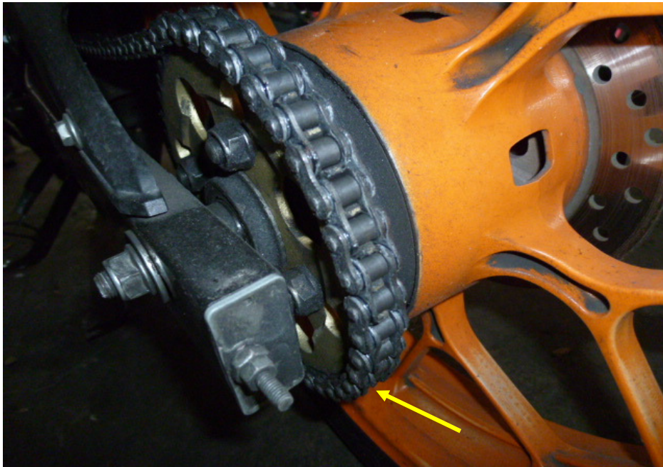
Photo 17 shows the closer view of the gear chain (arrowed) of the Motorcycle, which was observed to be intact with no misalignment. It was also adequately lubricated for operating purposes.
