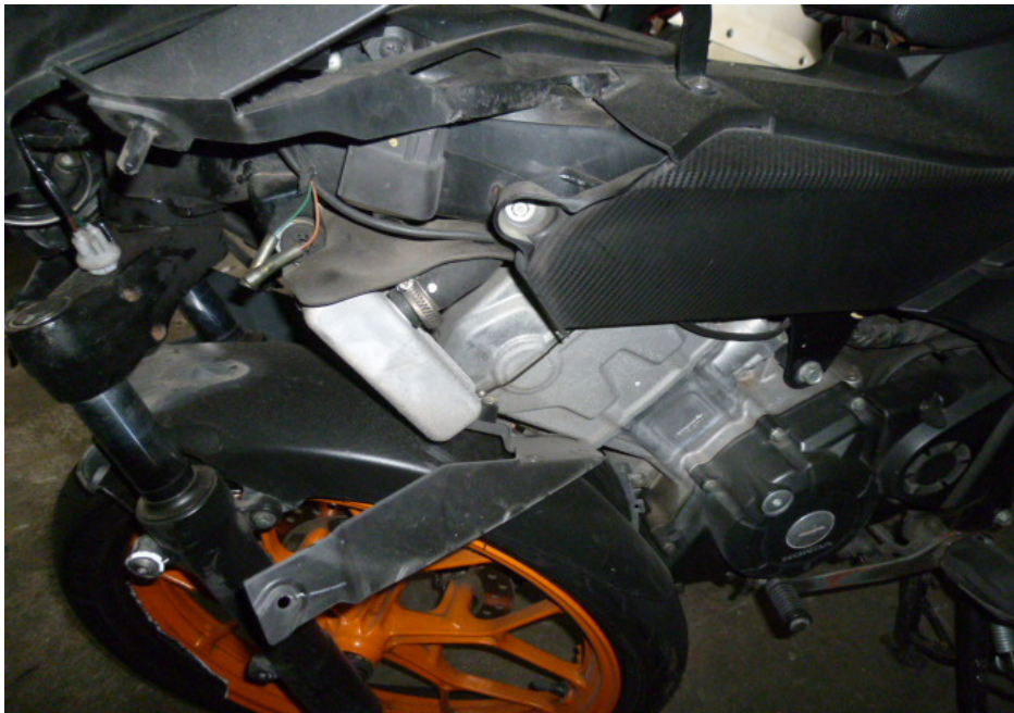
Photo 9 shows a closer view of the missing left cowling of the Motorcycle that as a result of the accident.
