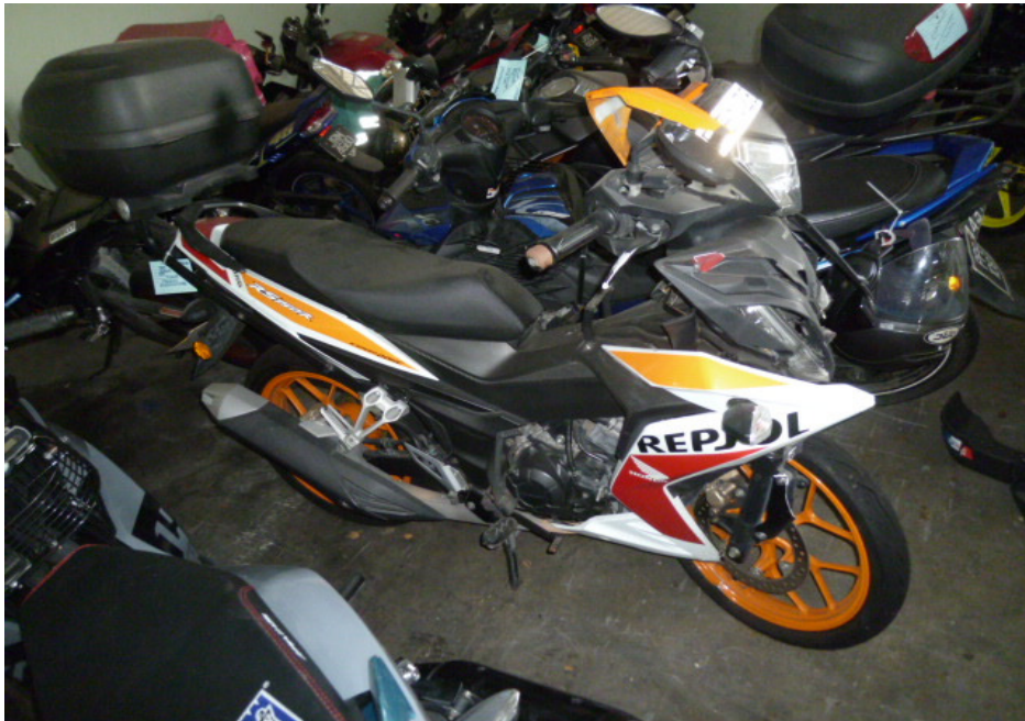
Photo 3 shows a general view of the right body of the Motorcycle at the time of our inspection. The Motorcycle had sustained damages all around. Body parts that were found to have been damaged include its headlight assembly, front cowling, front fork assembly, front wheel rim, front mudguard, left side mirror, clutch lever, side cowlings, gear shift pedal and left front footrest, amongst others.
