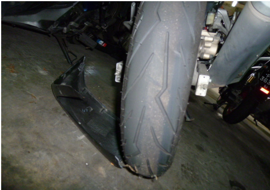
Photo 13 shows the condition of the Motorcycle's rear tyre. The pattern of the tread was clearly visible with remaining tread depth of approximately 3mm. We did not observe any tear, burst mark(s) and/or punctured hole(s) on the sidewalls as well as across the tread of the rear tyre.
