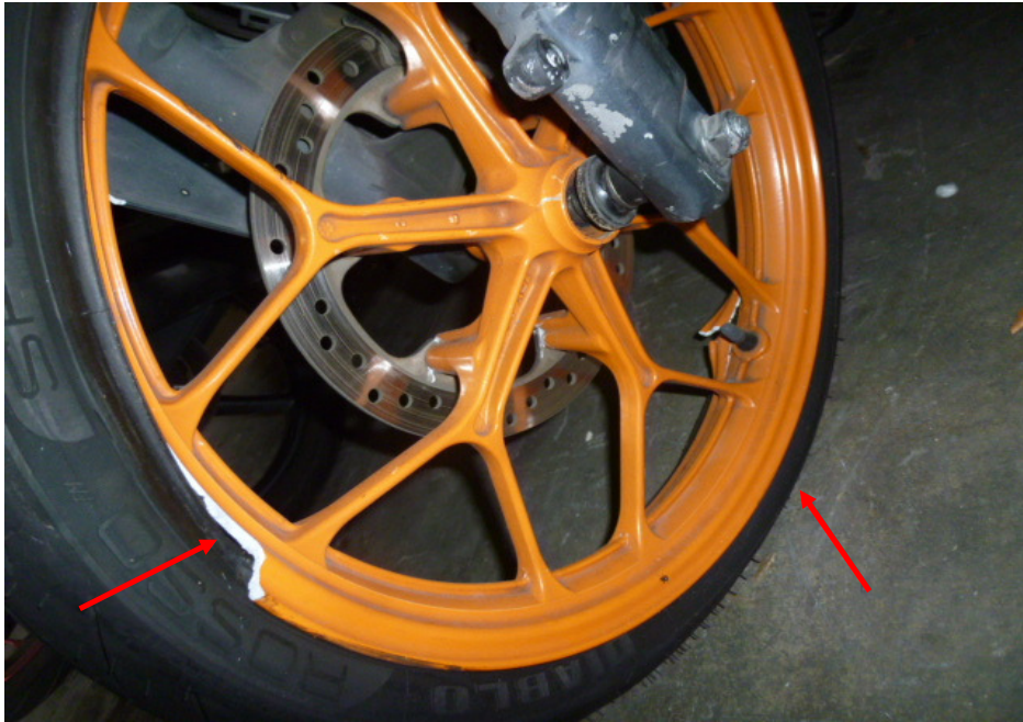
Photo 12 shows a close up view of the deflated front tyre due to the broken front wheel rim of the Motorcycle at the time of our inspection (arrowed).
