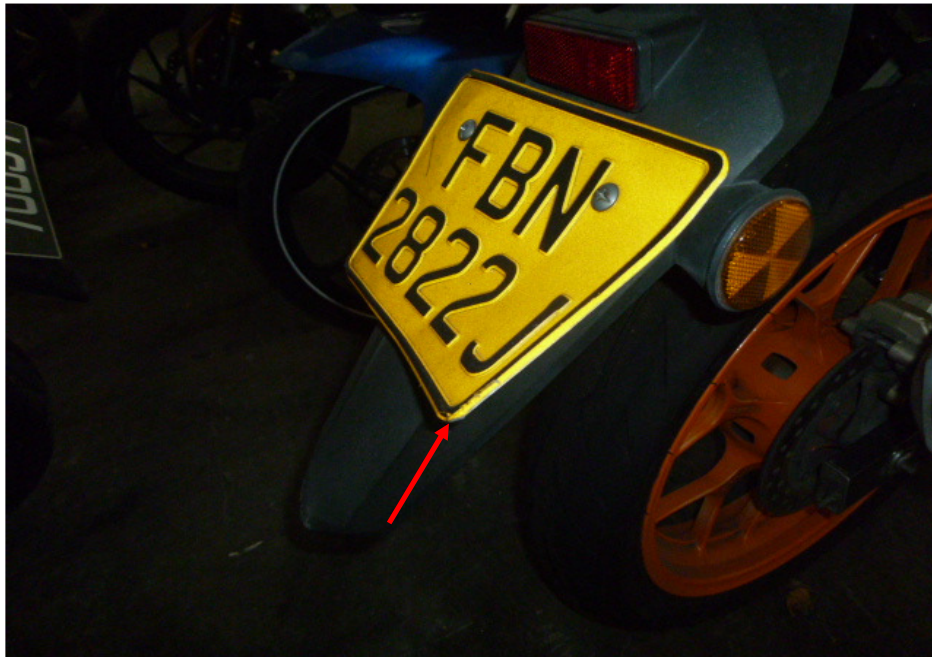
Photo 10 shows the dented rear number plate of the Motorcycle as a result of the accident (arrowed).
