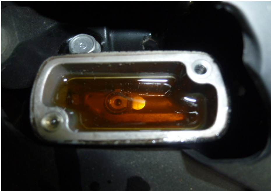
Photo 20 shows the brake fluid reservoir for the front brake of the Motorcycle. The brake fluid was observed to be of sufficient level for operational purposes and without contamination.
