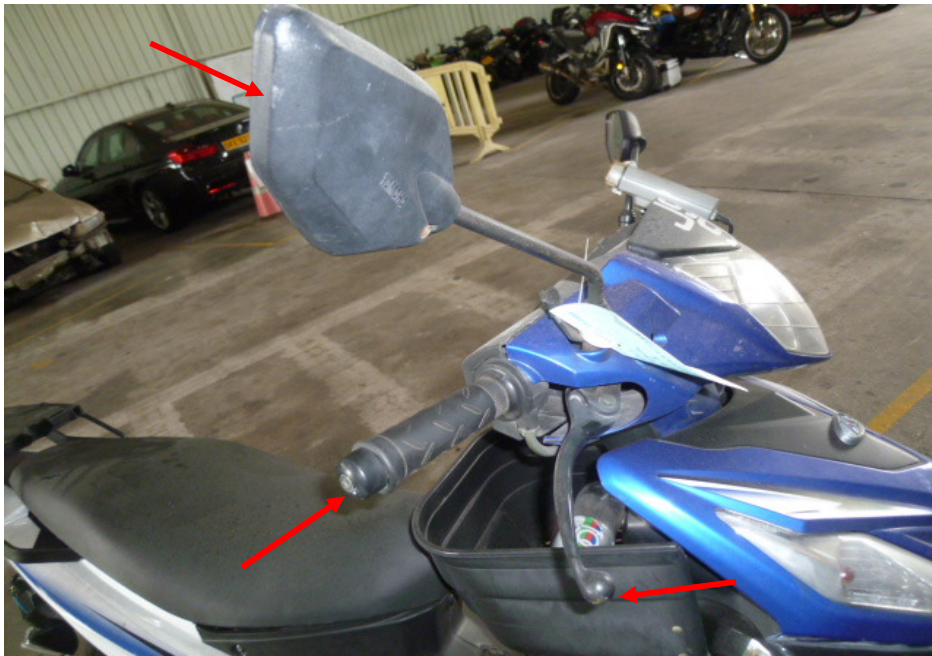
Photo 7 shows the right handlebar end, right side mirror and front brake lever (arrowed), which were amongst the body parts of the Motorcycle that had sustained damage as a result of the accident.
