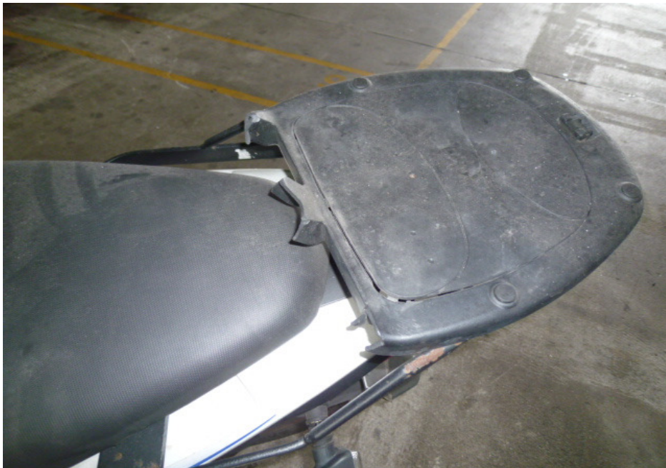
Photo 11 shows the broken top box rack of the Motorcycle as a result of the accident.
