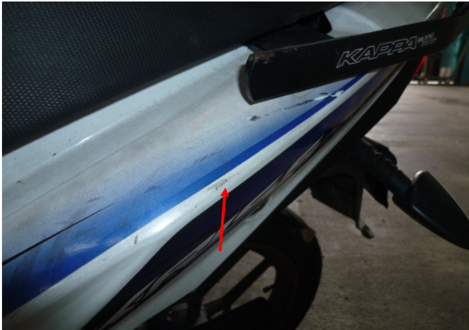
Photo 6 shows a closer view of the left rear side cover which was amongst the body parts of the Motorcycle that had sustained damage as a result of the accident (arrowed).
