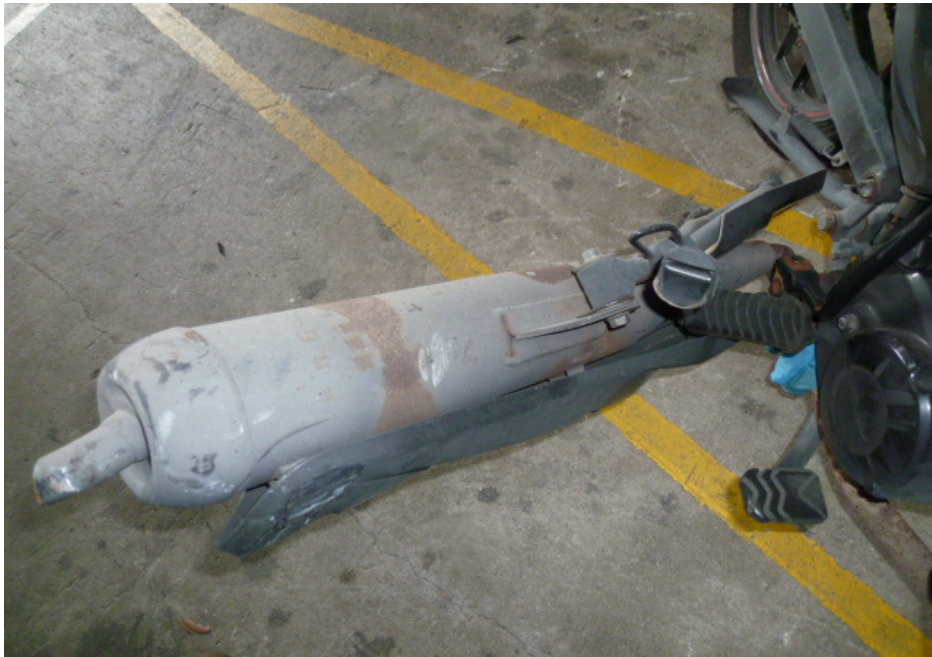
Photo 12 shows the bent exhaust muffler of the Motorcycle as a result of the accident.
