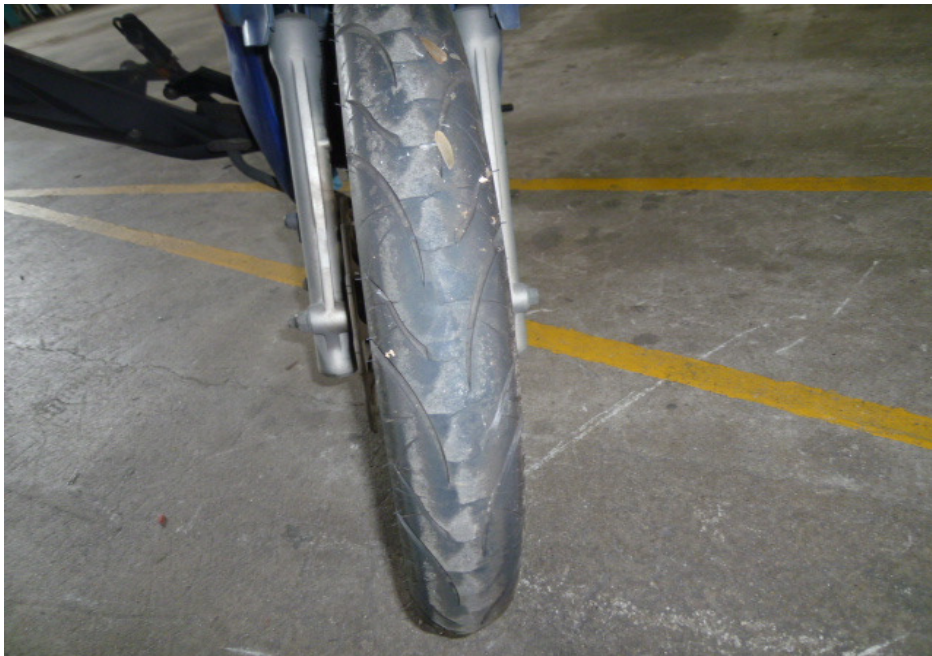
Photo 13 shows the front tyre of the Motorcycle at the time of our inspection. The front tyre was observed to be in serviceable condition with remaining tread depth of approximately 3mm. The pattern of the tread was also clearly visible. There was no tear, burst mark(s) and/or punctured hole(s) on the sidewalls as well as across the tread of the front tyre.
