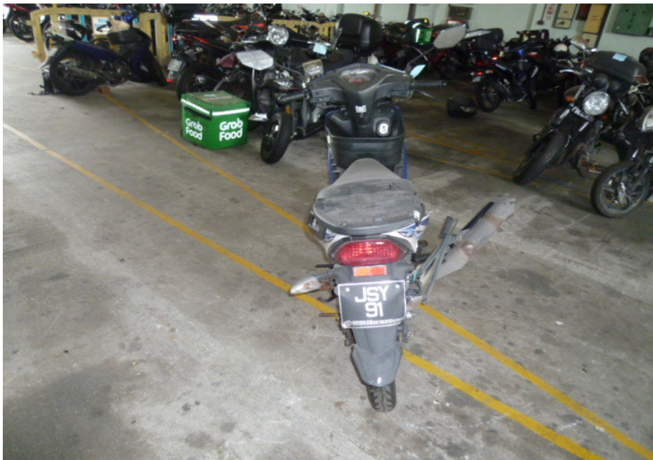
Photo 5 shows a general view of the right body of the Motorcycle at the time of our inspection. The Motorcycle was observed to have sustained damages all around. Amongst the body parts that were found to have been damaged include its front brake lever, right side mirror, right handlebar end, right pillion footpeg bracket, left pillion footpeg, left rear side cover, right rear signal lamp, top box rack, rear number plate and exhaust muffler, amongst others..
