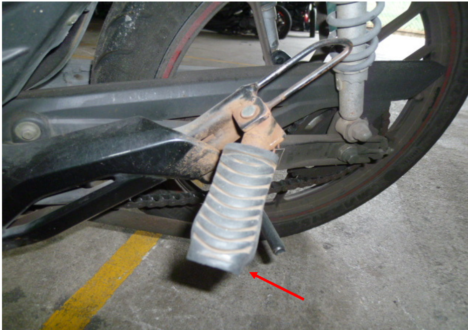
Photo 8 shows a closer view of the left pillion footpeg which was amongst the body parts of the Motorcycle that had sustained damage as a result of the accident (arrowed).
