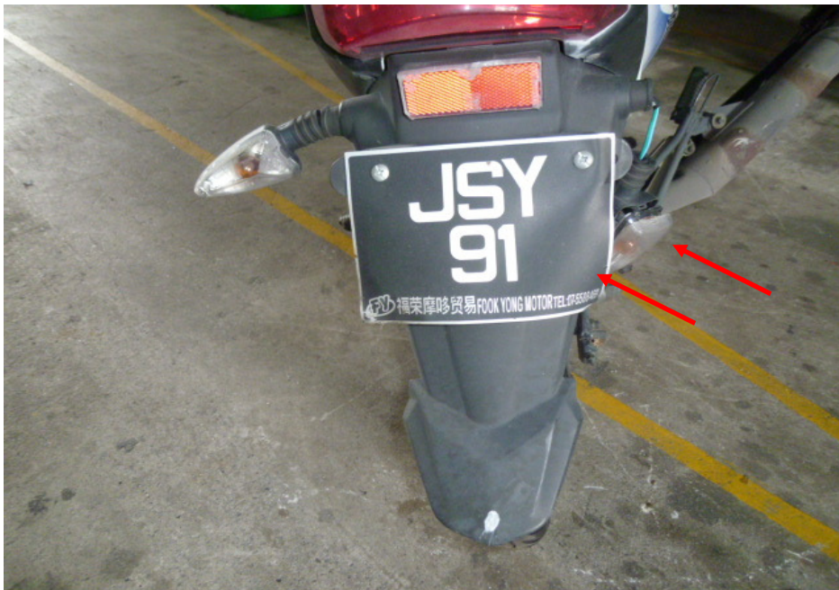
Photo 9 shows a closer view of the dented rear number plate and broken right rear signal lamp of the Motorcycle as a result of the accident (arrowed).
