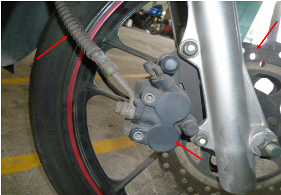
Photo 22 shows a close up view of the front brake caliper, front brake disc and front brake hose (arrowed) of the Motorcycle, which are all part of the components in the hydraulic front brake system of the Motorcycle. Our visual checks of these various components had revealed all to be intact with no visible damage. No leakage of brake fluid was also observed.
