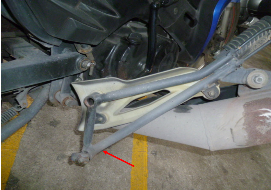
Photo 10 shows a closer view of the broken right pillion footpeg bracket (arrowed) which was amongst the body parts of the Motorcycle that had sustained damages as a result of the accident.
