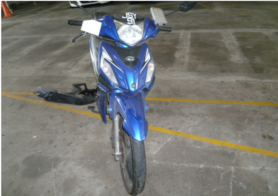
Photo 20 shows the front wheel of the Motorcycle turned towards its left. We were unable to turn the handle bar fully towards the left due to resistance most probably as a result of damages sustained during the accident.
