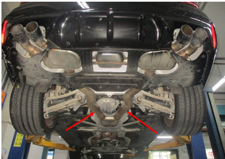
Photo 23 shows the rear section of the Motor Car's exhaust system. My examination of the Motor Car's exhaust system revealed no sign(s) or indication(s) of any cut or weld marks along its exhaust pipes (arrowed), centre resonator boxes, rear mufflers and on its catalytic converters.
