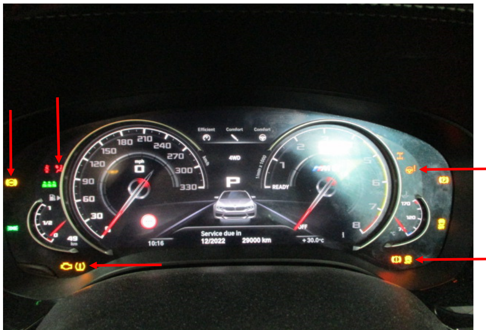
Photo 16 shows the warning lights for the various electronic safety features appearing on the instrument panel of the Motor Car during its self-test when the engine is cranked, in particular the ABS, SRS, IAS, TPM and DSC lights (arrowed).
