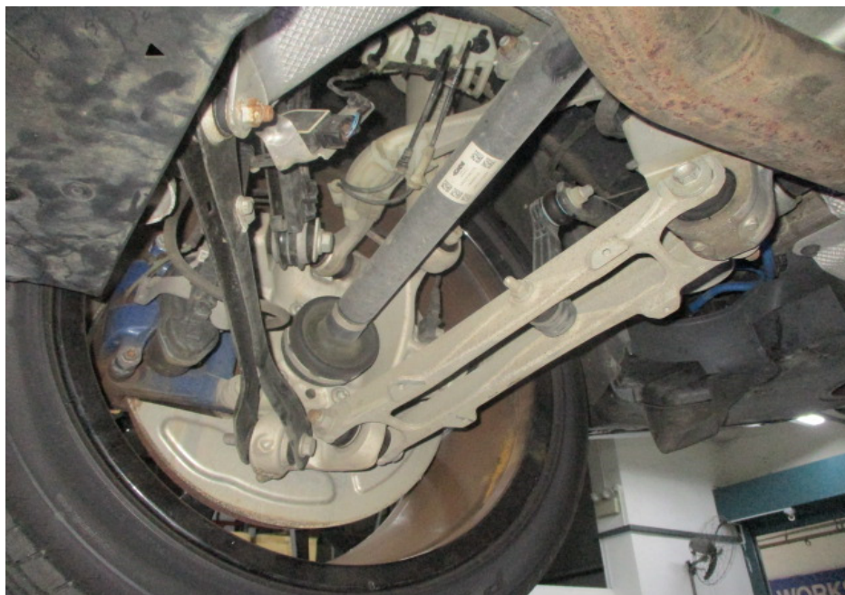
Photo 20 shows a general view of the control arms and linkages at the rear right wheel of the Motor Car. I did not observe any fluid leak and/or fluid stain on the underside of the Motor Car. All of the Motor Car's undercarriage components were observed to be intact and secured in an appropriate manner.
