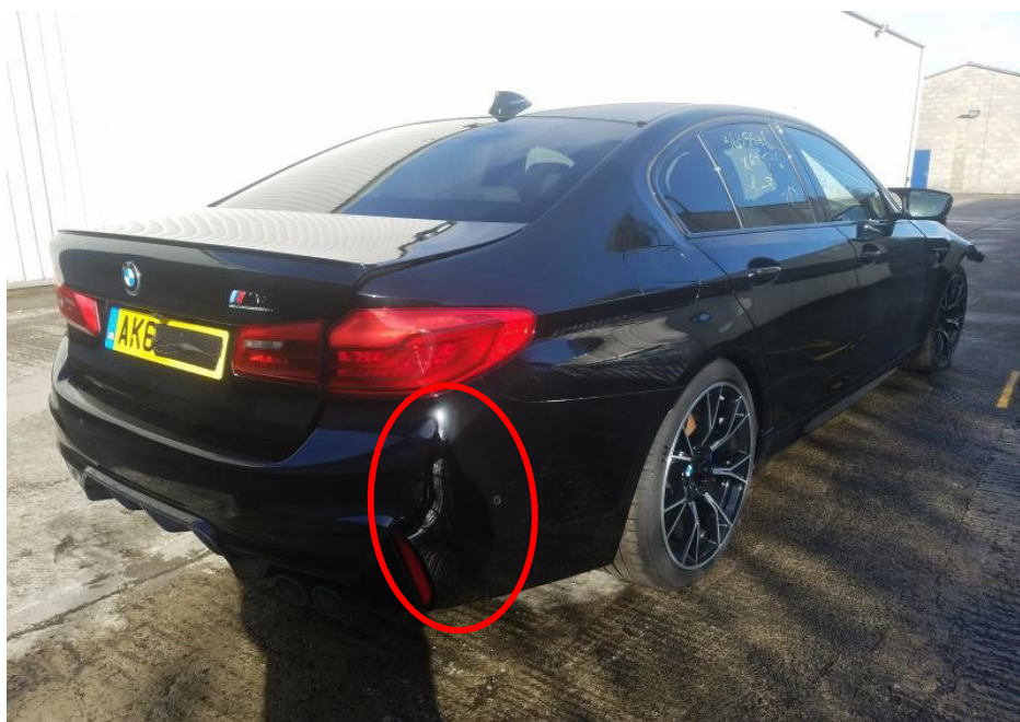
Photo 2 shows the rear right body of the Motor Car (photograph provided to me). The rear bumper of the Motor Car was also observed to be dented at its right corner area (circled).
