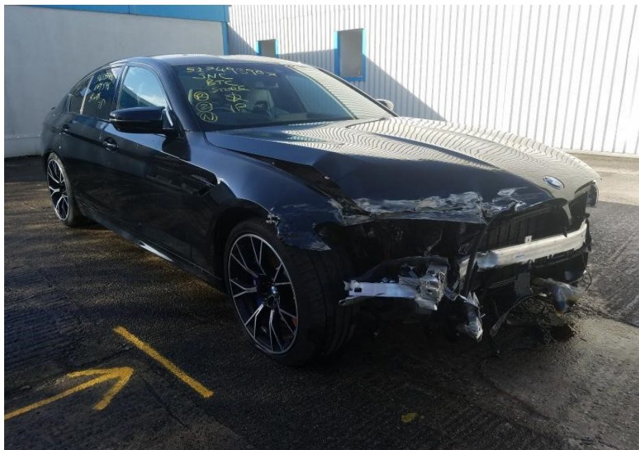
Photo 1 shows a general view of the front right body of the Motor Car (photograph provided to me). The Motor Car was observed to have sustained damage at its front right body. The front bumper and all its related parts and attachments, front bumper reinforcement, front bumper sponge, front parking sensors, radar unit, radiator grilles, front undercover, front right headlamp, front bonnet, front right fender and front right fender inner shield amongst others were observed to be damaged
