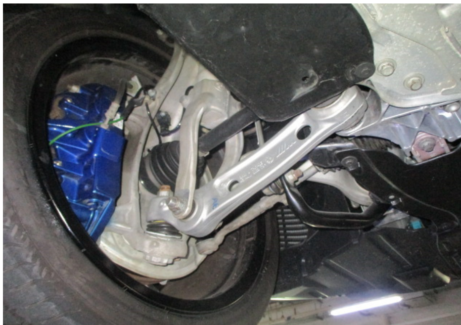
Photo 22 shows the various undercarriage components at the front left wheel of the Motor Car. The mechanical components, control arms and linkages were all found to be intact and secured in an appropriate manner. I also did not observe any fluid leak and/or fluid stain on the underside of the Motor Car.
