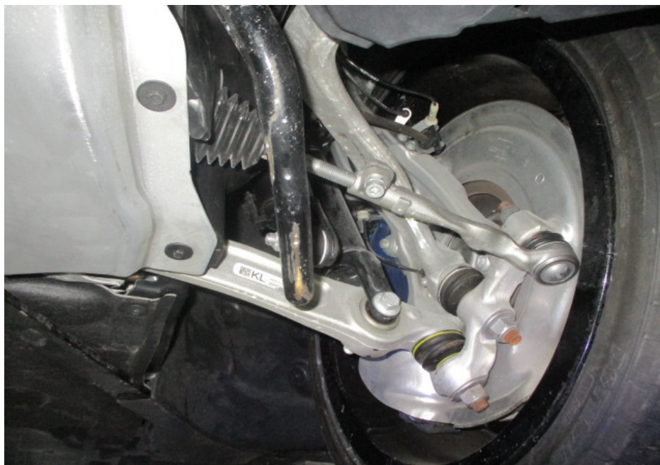
Photo 26 shows the various undercarriage components at the front left wheel of the Motor Car. The mechanical components, control arms and linkages were all found to be intact and secured in an appropriate manner. I also did not observe any fluid leak and/or fluid stain on the underside of the Motor Car.
