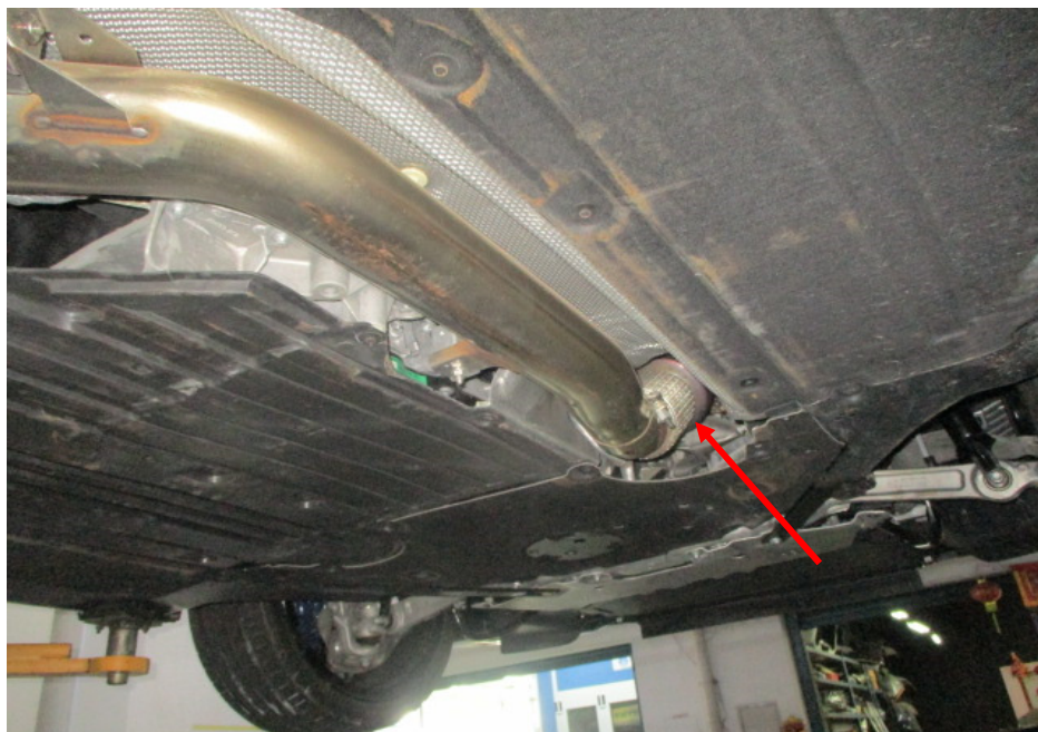
Photo 28 shows the front section of the Motor Car's exhaust system. My examination of the Motor Car's exhaust system revealed no sign(s) or indication(s) of any cut or weld marks along its exhaust pipes, centre resonator box, rear muffler and on its catalytic converter (arrowed).
