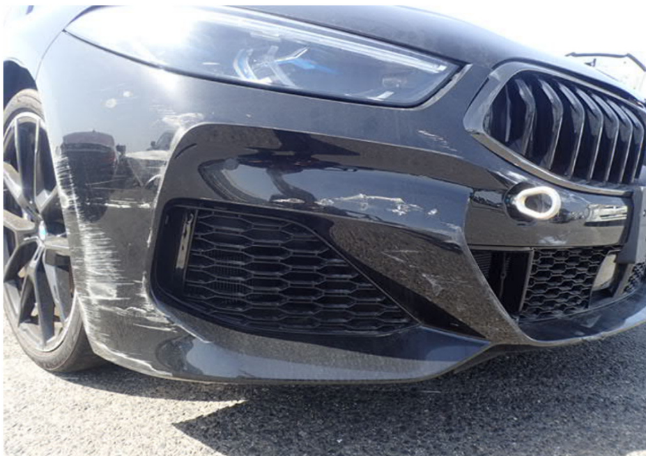
Photo 5 shows a closer view of the damage to the front bumper at the front right body of the Motor Car (photograph provided to me).
