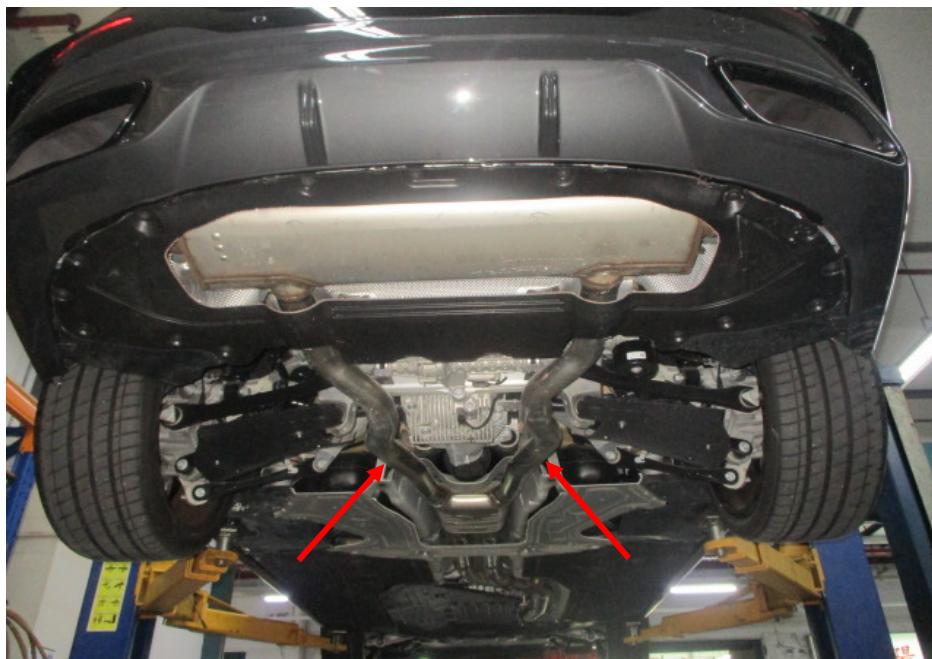
Photo 27 shows the rear section of the Motor Car's exhaust system. My examination of the Motor Car's exhaust system revealed no sign(s) or indication(s) of any cut or weld marks along its exhaust pipes (arrowed), centre resonator box, rear muffler and on its catalytic converter.
