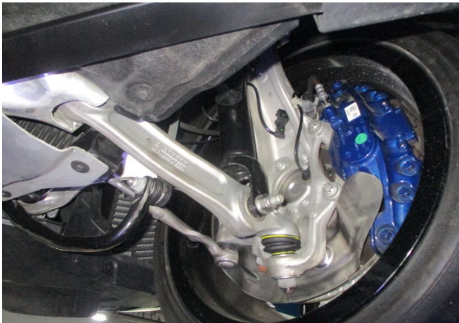
Photo 25 shows the various undercarriage components at the front right wheel of the Motor Car. The mechanical components, control arms and linkages were all found to be intact and secured in an appropriate manner.
