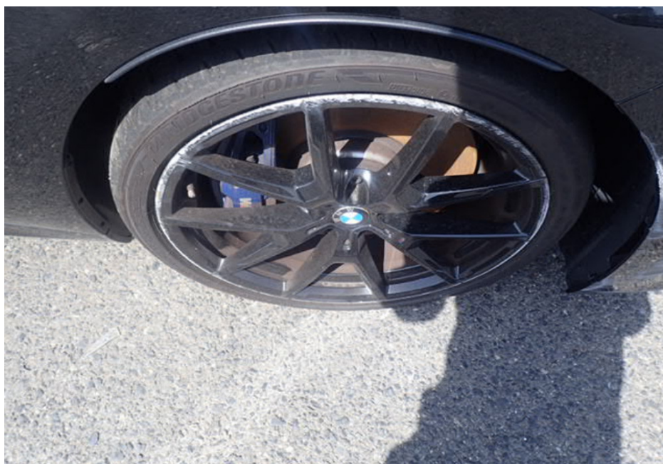
Photo 6 shows a closer view of the damage to the front right wheel rim of the Motor Car (photograph provided to me). Grazed marks were seen to the edges at the outer circumference of the front right wheel rim. The front right undercarriage parts of the Motor Car were likely to be affected as the orientation of the Motor Car's front wheels were not in the same direction (refer to photograph 1 and 4 above). Parts that may possibly have been affected include the front right lower arm, front right upper arm, front right knuckle arm, front right shock absorber and front right steering tie rod amongst others.
