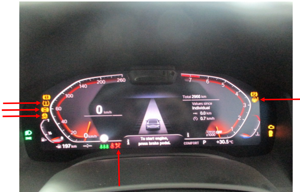
Photo 20 shows the warning lights for the various electronic safety features appearing on the instrument panel of the Motor Car during its self-test when the engine is cranked, in particular the ABS, SRS, IAS, TPM and DSC lights (arrowed).
