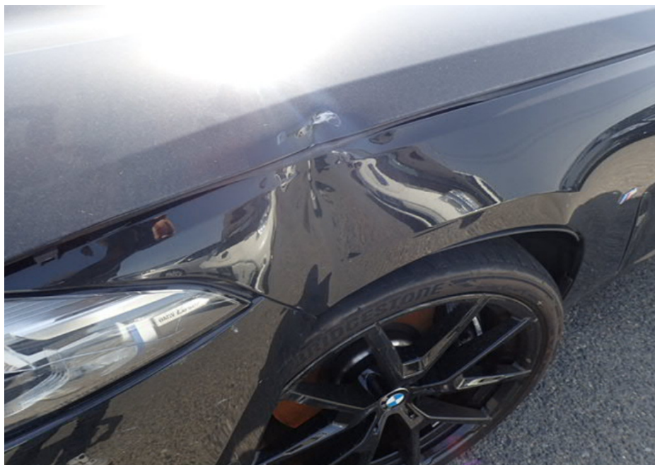
Photo 3 shows a closer view of the damage to the front left fender and front bonnet of the Motor Car (photograph provided to me).
