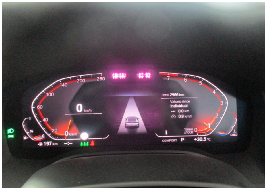
Photo 21 shows the respective warning lights no longer illuminated, indicating that there is no fault detected to the ABS, SRS, IAS, TPM and DSC systems of the Motor Car during the self-test. These electronic systems were hence in working condition at the time of my inspection.
