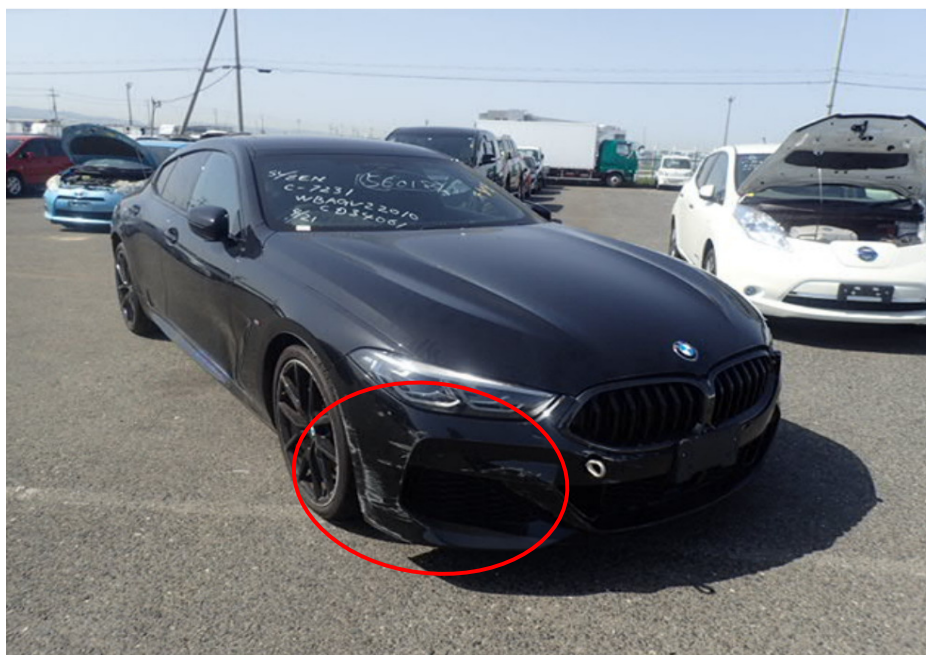
Photo 4 shows a general view of the front right body of the Motor Car (photograph provided to me). Apart for the front left body, the Motor Car had also sustained damage at its front right body (circled). The front bumper and front right wheel rim were amongst the body parts that were observed to have been damaged. The front right wheel and front left wheel (refer to photograph 1 above) were orientated in different directions, which suggests to me that there was damage to the front right undercarriage parts of the Motor Car given that the front right wheel rim was damaged (refer to photograph 6 below).
