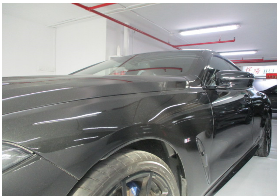
Photo 11 shows a closer view of the front bonnet and front left fender of the Motor Car at the time of my inspection. The body parts at the front left body of the Motor Car were visually examined and it was observed that the repair/restoration works carried out to the damaged area of the Motor Car (refer to photograph 3 above) were reasonably adequate and in order.
