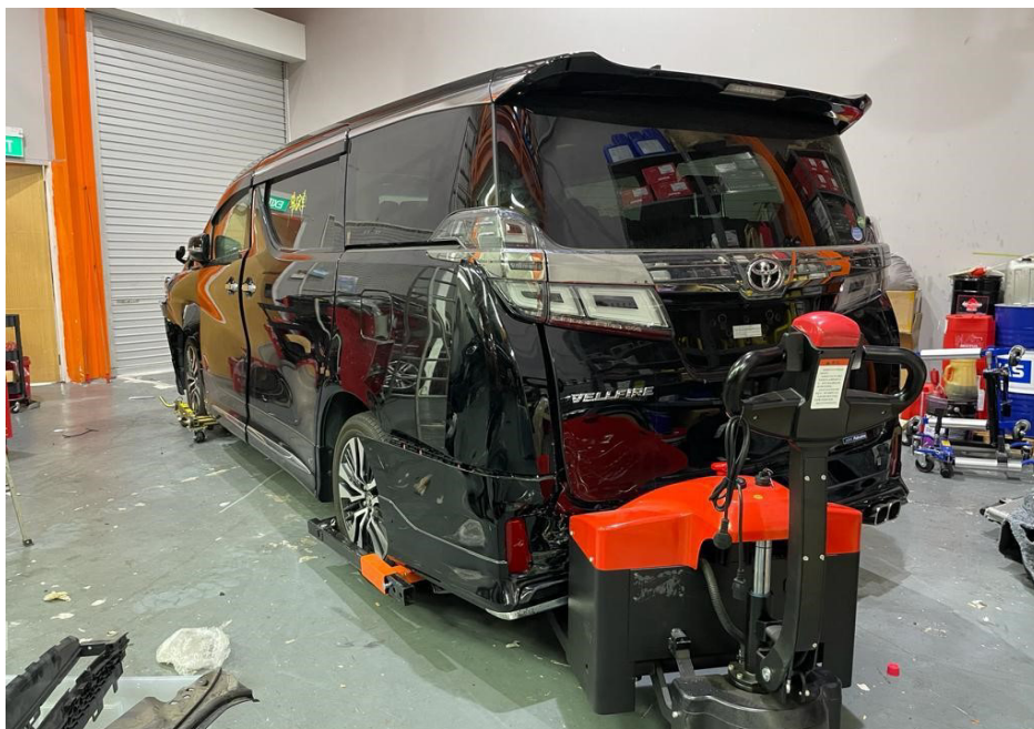
Photo 3 shows the rear left body of the Motor Car (photograph provided to me). Apart from the frontal body, the photographs provided had also showed damage to the rear left body of the Motor Car. The Motor Car's rear bumper, rear bumper lower cover, rear bumper left reflector, rear bumper left chrome moulding, rear bumper left top garnish and rear tailgate were amongst the body parts that were observed to have been damaged.
