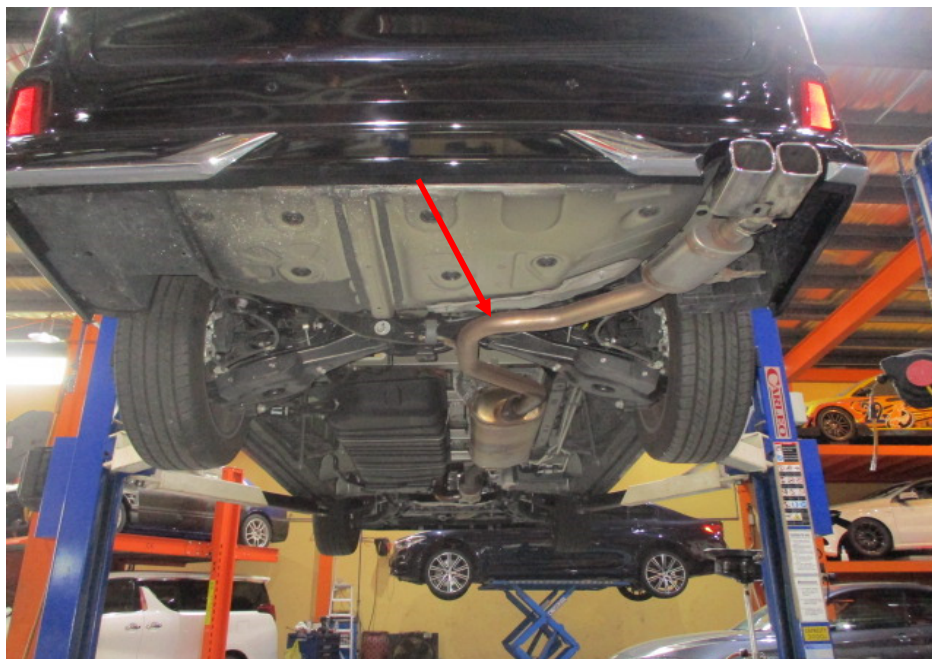
Photo 27 shows a general view of the rear section of the Motor Car's exhaust system. My examination of the Motor Car's exhaust system revealed no sign(s) or indication(s) of any cut or weld marks along its exhaust pipe (arrowed), on its catalytic converter, centre resonator box and on its rear muffler.
