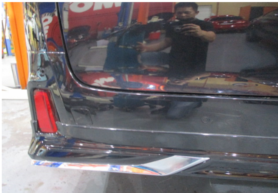
Photo 12 shows a closer view of the Motor Car's rear bumper, rear bumper lower cover, rear bumper left reflector, rear bumper left chrome moulding and rear tailgate. The body parts at the rear left body of the Motor Car were visually examined and it was observed that the repair/restoration works carried out to the damaged area of the Motor Car (refer to photograph 3 above) were reasonably adequate and in order.
