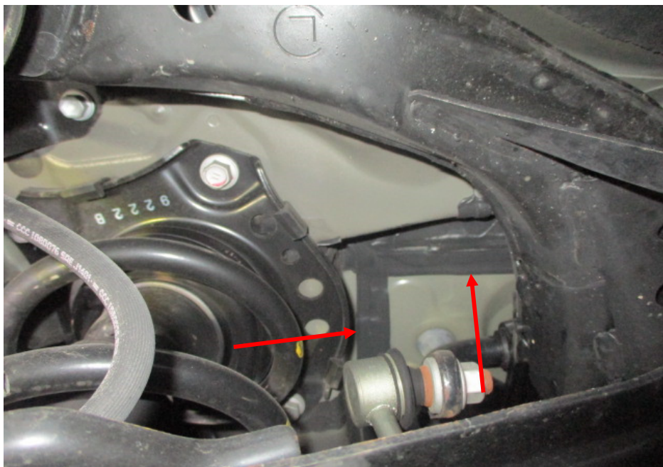
Photo 30 shows the floorboard and chassis/structural body at the underside rear left of the Motor Car. The original factory sealant (arrowed) at the joints along the floorboard was observed to be untouched. In general, I had found all the non-detachable body panels of the Motor Car to be originally fitted at the time of my inspection.
