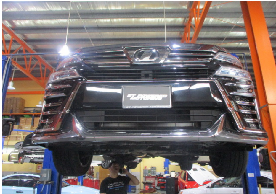
Photo 22 shows the Motor Car hoisted up for checks on its undercarriage. There was no sign(s) or indication(s) of fluid leakage and/or fluid stain(s) on the underside of the Motor Car. The undercarriage components of the Motor Car were also all observed to be intact and secured in an appropriate manner.
