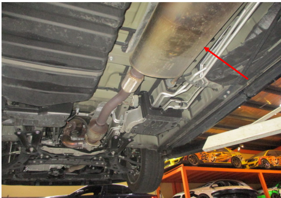
Photo 28 shows a general view of the front section of the Motor Car's exhaust system. My examination of the Motor Car's exhaust system revealed no sign(s) or indication(s) of any cut or weld marks along its exhaust pipe, on its catalytic converter, centre resonator box (arrowed) and on its rear muffler.
