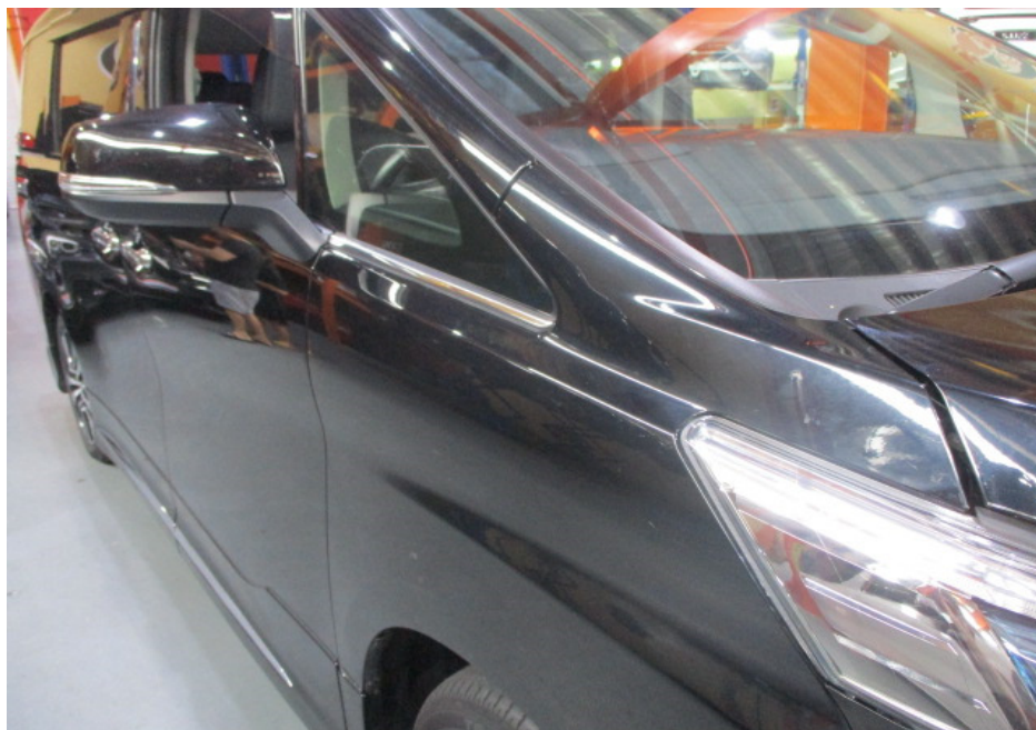
Photo 10 shows a closer view of the Motor Car's front right headlamp, front right fender and front windscreen. The body parts at the frontal body of the Motor Car were visually examined and it was observed that the repair/restoration works carried out to the damaged area of the Motor Car (refer to photograph 1 & 2 above) were reasonably adequate and in order.
