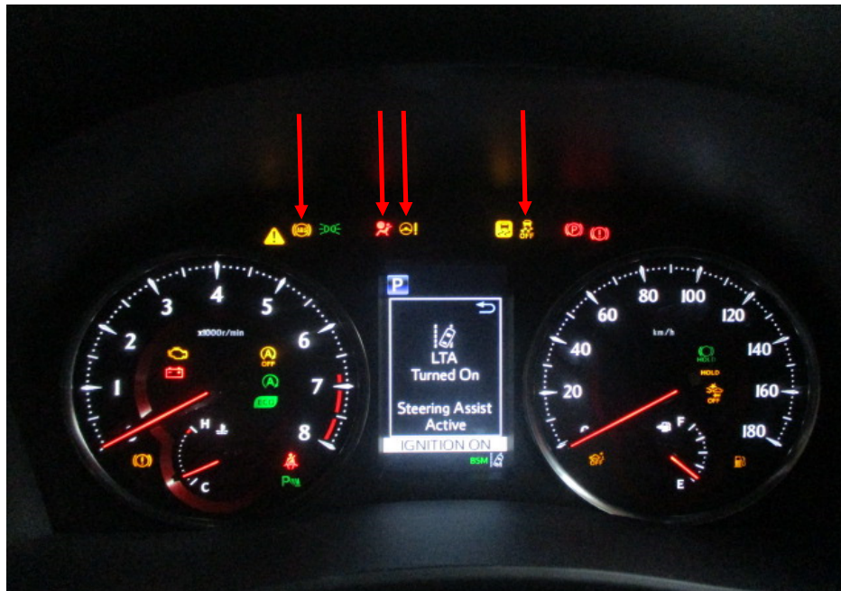
Photo 20 shows the warning lights for the various electronic safety features appearing on the instrument panel of the Motor Car during its self-test when the engine is cranked, in particular the lights for the ABS, SRS, EPS, VSC and various pre-collision systems (arrowed).
