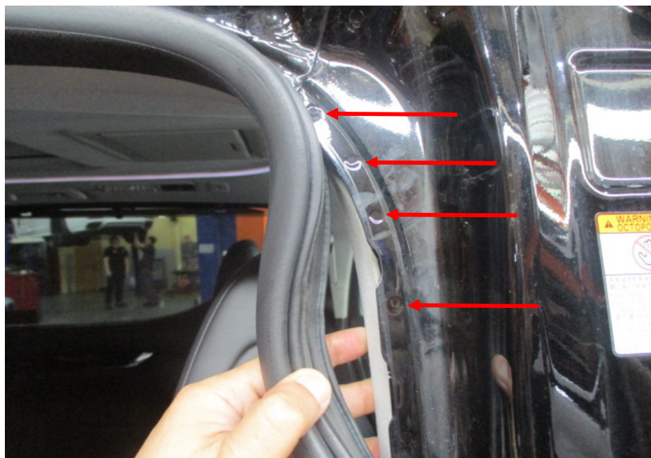
Photo 33 shows the right side centre pillar of the Motor Car. I did not find any weld marks other than original spot weld marks (arrowed) on the right side centre pillar of the Motor Car, which indicates that there was no re-welding works carried out. In general, I had found all the non-detachable body panels of the Motor Car to be originally fitted at the time of my inspection.
