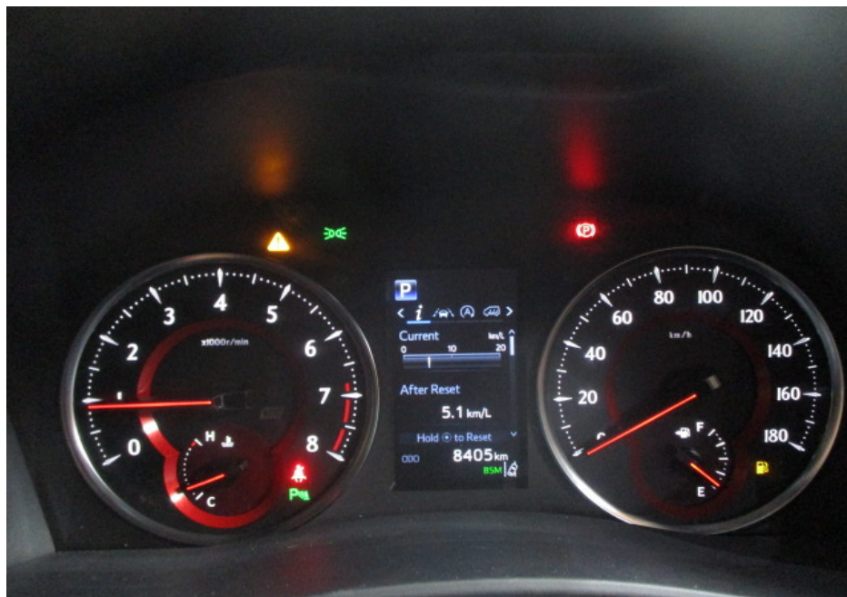
Photo 21 shows the respective warning lights no longer illuminated, indicating that there is no fault detected to the ABS, SRS, EPS, VSC and various pre-collision systems of the Motor Car during the self-test. These electronic systems were hence in working condition at the time of my inspection.
