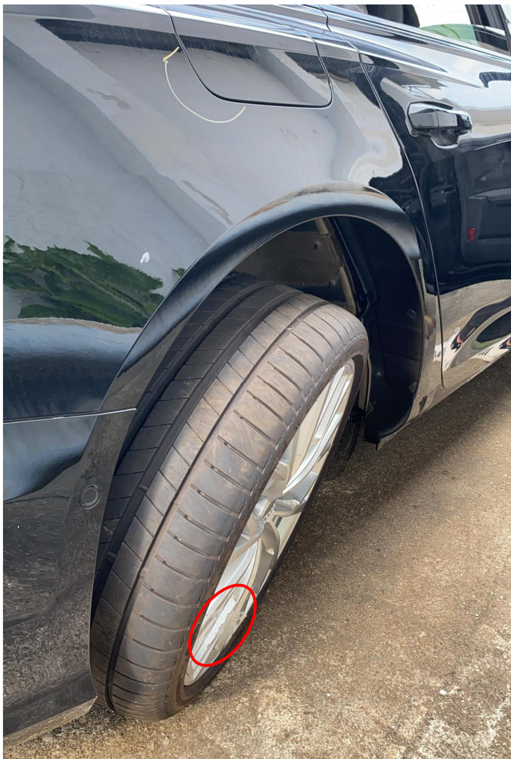
Photo 4 shows a closer view of the Motor Car's tilted rear right wheel prior to any repairs being carried out (photograph provided to me). The photographs had showed damage (circled) to the Motor Car's rear right wheel rim but not on the surrounding body parts. The tilting of the rear right wheel indicates damage to the rear right undercarriage parts like the rear right shock absorber, rear right lower arms and linkages amongst others.
