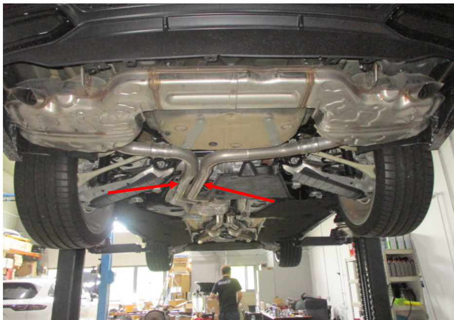
Photo 24 shows a general view of the rear section of the Motor Car's exhaust system. My examination of the Motor Car's exhaust system revealed no sign(s) or indication(s) of any cut or weld marks along its exhaust pipes (arrowed), on its catalytic converters, centre resonator boxes and on its rear mufflers.
