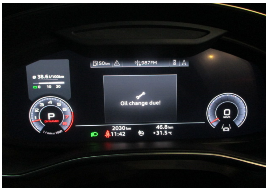
Photo 18 shows the respective warning lights no longer illuminated, indicating that there is no fault detected to the ABS, SRS, EPS, TPM and ESC systems of the Motor Car during the self-test. These electronic systems were hence in working condition at the time of my inspection.
