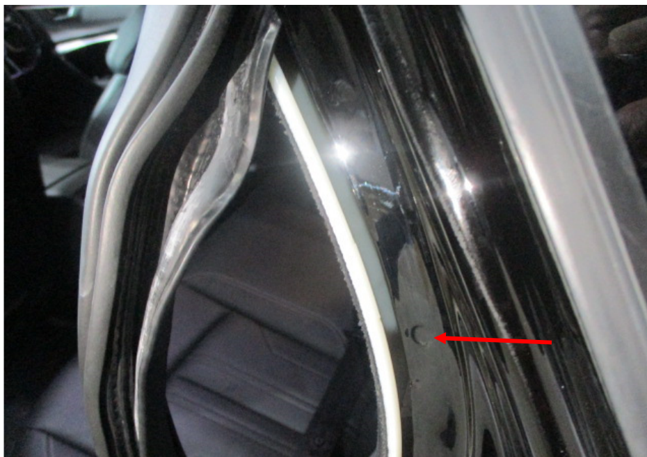
Photo 31 shows the upper section of the Motor Car's left side "C" pillar. Original weld marks (arrowed) were observed at the upper section. The lack of original weld marks at the lower section of the Motor Car's left side "C" pillar (refer to photograph 30) was due to smoothening of the lower section for re-spraying work after the left rear fender was repaired.
