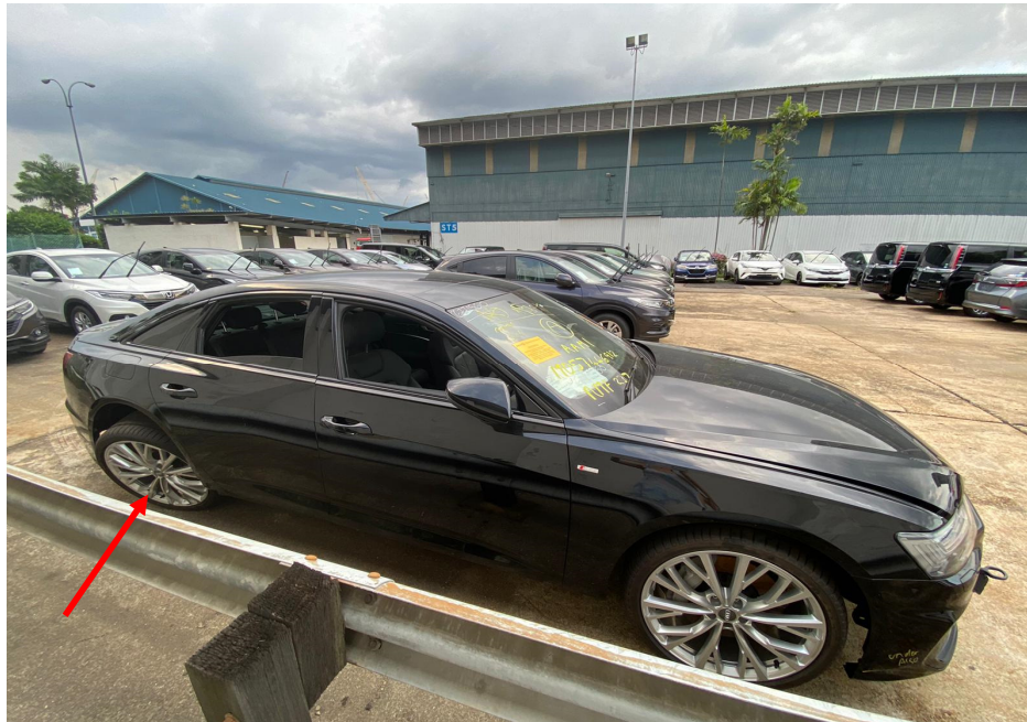
Photo 3 shows the right body of the Motor Car prior to any repairs being carried out (photograph provided to me). The rear right wheel (arrowed) of the Motor Car was observed to be tilted, which would indicate damage to the rear right undercarriage parts like the rear right shock absorber, rear right lower arms and linkages amongst others.
