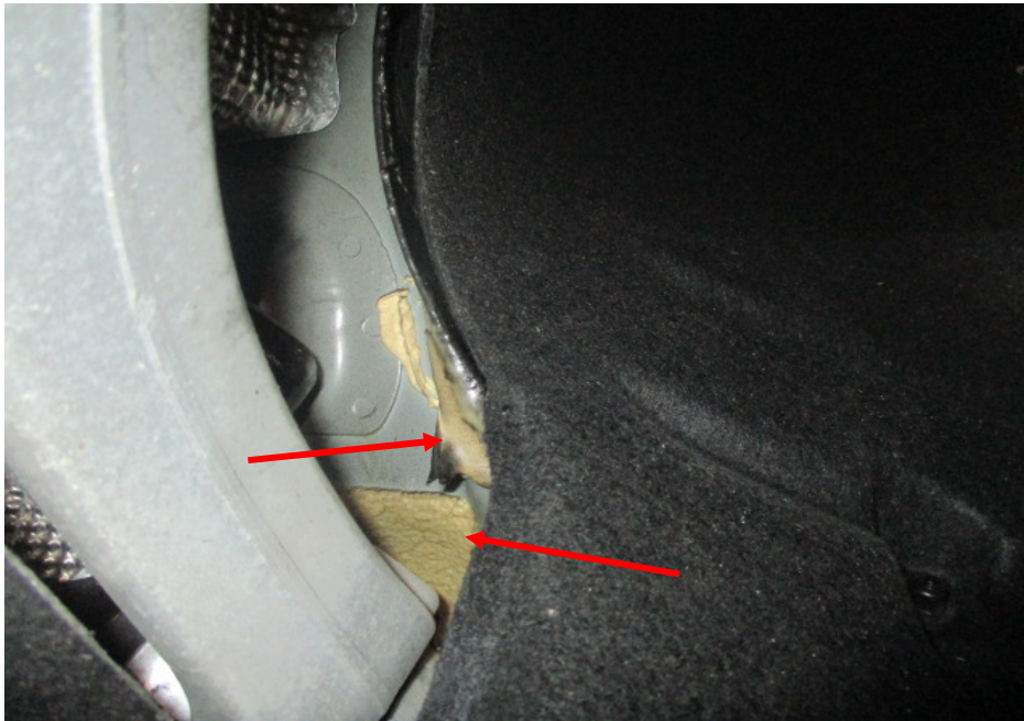
Photo 28 shows the chassis/structural body at the underside front left of the Motor Car. I did not find any weld marks other than original spot weld marks on the chassis/structural body of the Motor Car. The original factory sealant (arrowed) at the joints along the chassis/structural body was untouched, indicating no work was done on the chassis/structural body of the Motor Car and that the chassis/structural body was originally fitted.
