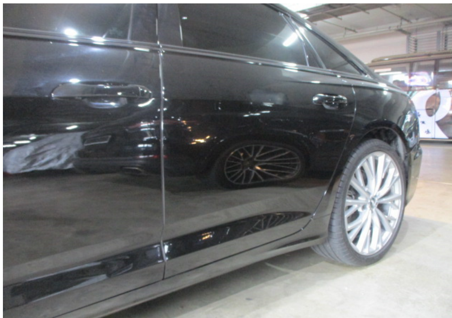
Photo 8 shows a closer view of the Motor Car's left front door, left rear door and left side rocker panel garnish. The repair/restoration works carried out to the damaged area of the Motor Car (refer to photograph 1 & 2 above) were reasonably adequate and in order.
