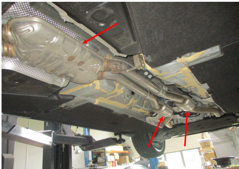
Photo 25 shows a general view of the front section of the Motor Car's exhaust system. My examination of the Motor Car's exhaust system revealed no sign(s) or indication(s) of any cut or weld marks along its exhaust pipes, on its catalytic converters, centre resonator boxes (arrowed) and on its rear mufflers.
