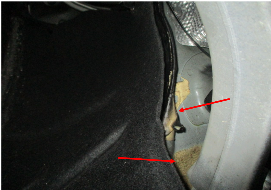
Photo 29 shows the chassis/structural body at the underside front right of the Motor Car. The original factory sealant (arrowed) at the joints along the chassis/structural body was observed to be untouched. In general, I had found no work was carried out on the chassis/structural body of the Motor Car. The chassis/structural body of the Motor Car was originally fitted.
