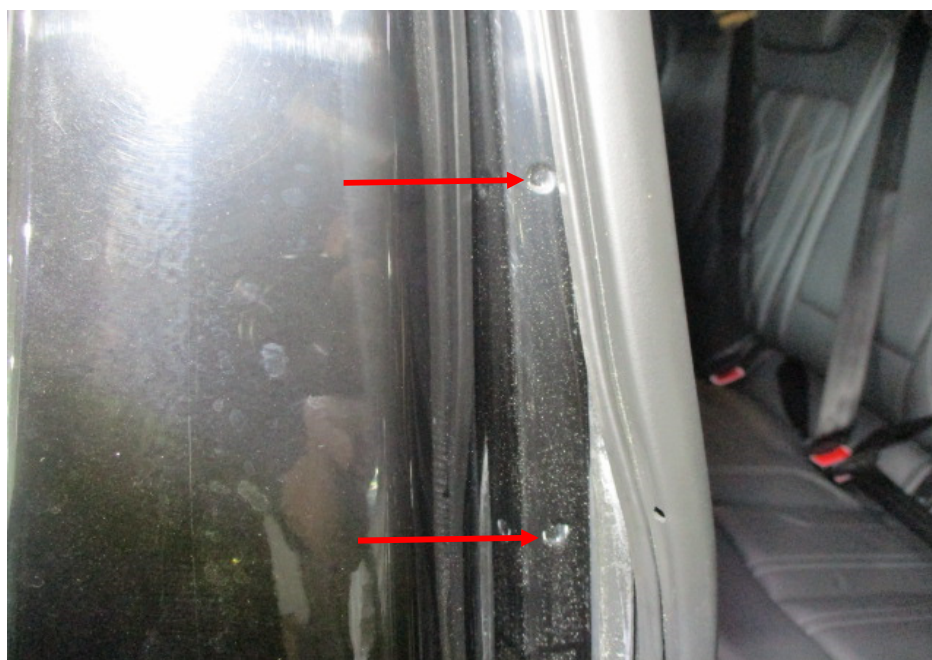
Photo 32 shows the left side "B" pillar of the Motor Car. I did not find any weld marks other than original spot weld marks (arrowed) on the left side "B" pillar of the Motor Car which, indicates that there was no re-welding works carried out. In general, I had found all the non-detachable body panels of the Motor Car to be originally fitted at the time of my inspection.
