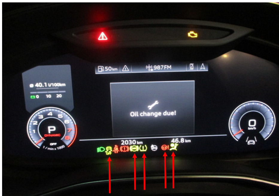
Photo 17 shows the warning lights for the various electronic safety features appearing on the instrument panel of the Motor Car during its self-test when the engine is cranked, in particular the ABS, SRS, EPS, TPM and ESC lights (arrowed).
