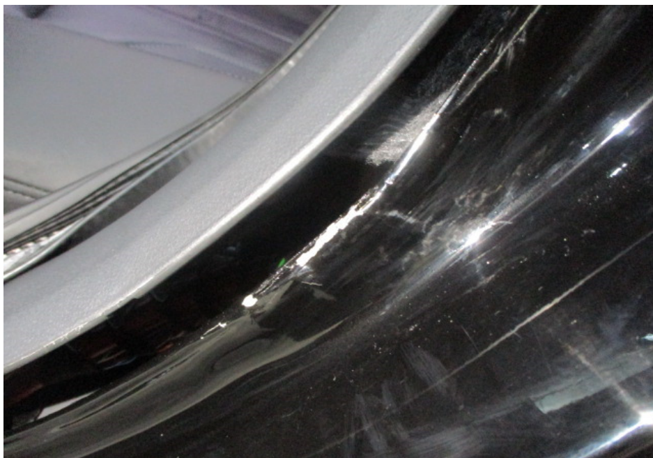
Photo 30 shows the lower section of the Motor Car's left side "C" pillar. I did not find any original weld marks at the lower section of the left side "C" pillar. Original weld marks were however found at the upper section of the left side "C" pillar (refer to photograph 31 below). The lack of original weld marks at the lower section was due to smoothening of the lower section for re-spraying work after the left rear fender was repaired.
