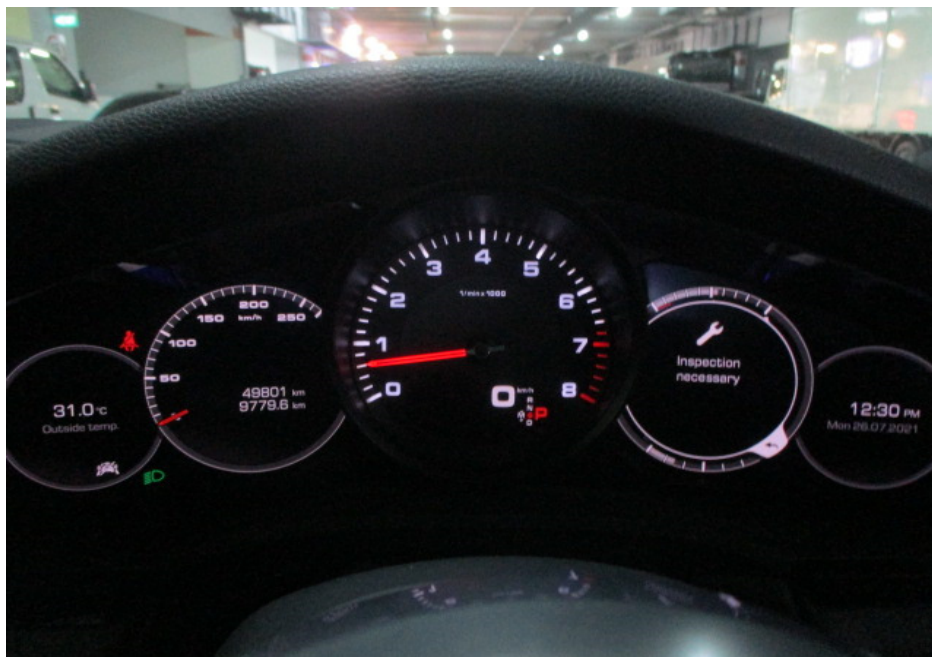
Photo 18 shows the respective warning lights no longer illuminated, indicating that there is no fault detected to the ABS, SRS, PSS, TPM and PSM systems of the Motor Car during the self-test. These electronic systems were hence in working condition at the time of my inspection.
