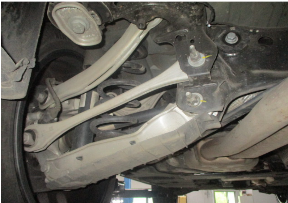
Photo 21 shows a general view of the control arms and linkages at the rear left wheel of the Motor Car. I did not observe any fluid leak and/or fluid stain on the underside of the Motor Car. All the Motor Car's undercarriage components were observed to be intact and secured in an appropriate manner.
