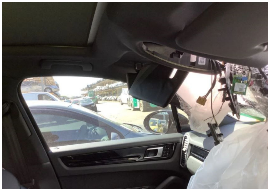
Photo 3 shows the interior compartment of the Motor Car prior to any repairs being carried out (photograph provided to me). The interior roof upholstery, interior sun visors, rear view mirror and interior top control panel were all observed to be damaged. The airbags of the Motor Car were not deployed as seen from the photographs that were provided to me.
