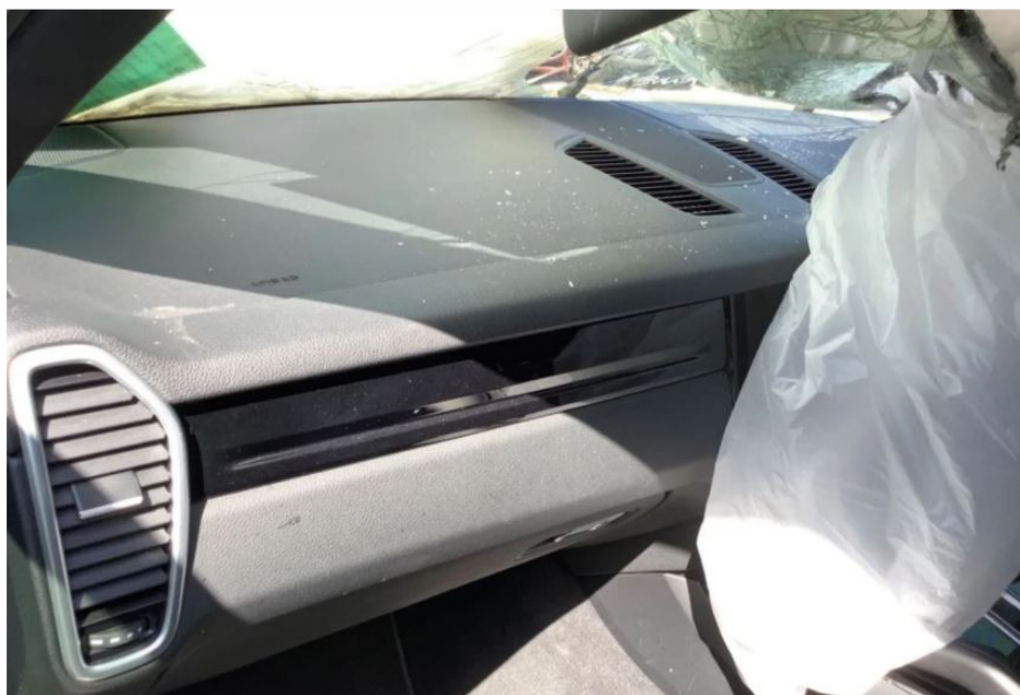
Photo 5 shows the front dashboard of the Motor Car prior to any repairs being carried out (photograph provided to me). The front dashboard did not appear to have sustain physical damage.
