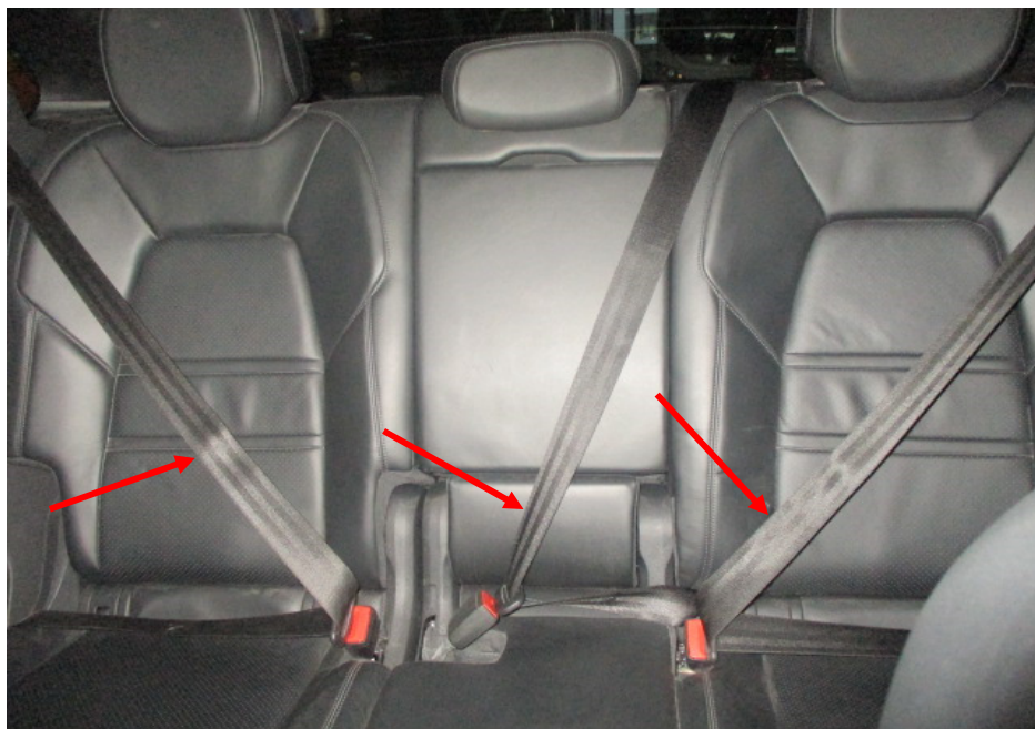
Photo 16 shows the rear seats of the Motor Car. All the seats of the Motor Car were secured via seat rails to the floorboard. They were also fitted with a retractable seat belt reel and a pre-tensioner. The seat belts (arrowed) were tested and were able to be fastened into the respective pre-tensions that were fitted on the side of each individual seat.
