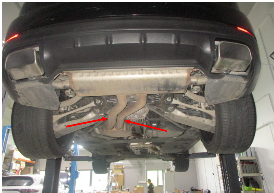
Photo 24 shows a general view of the rear section of the Motor Car's exhaust system. My examination of the Motor Car's exhaust system revealed no sign(s) or indication(s) of any cut or weld marks along its exhaust pipes (arrowed), on its catalytic converter, centre resonator boxes and on its rear muffler.
