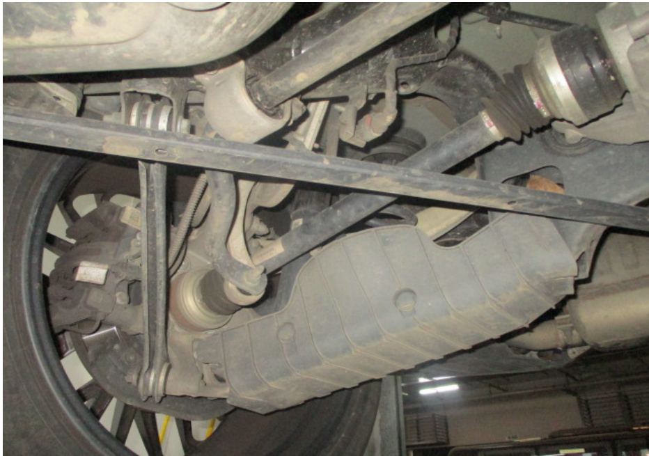
Photo 20 shows a general view of the control arms and linkages at the rear right wheel of the Motor Car. I did not observe any fluid leak and/or fluid stain on the underside of the Motor Car. All the Motor Car's undercarriage components were observed to be intact and secured in an appropriate manner.
