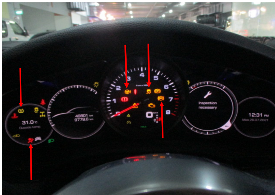
Photo 17 shows the warning lights for the various electronic safety features appearing on the instrument panel of the Motor Car during its self-test when the engine is cranked, in particular the ABS, SRS, PSS, TPM and PSM lights (arrowed).
