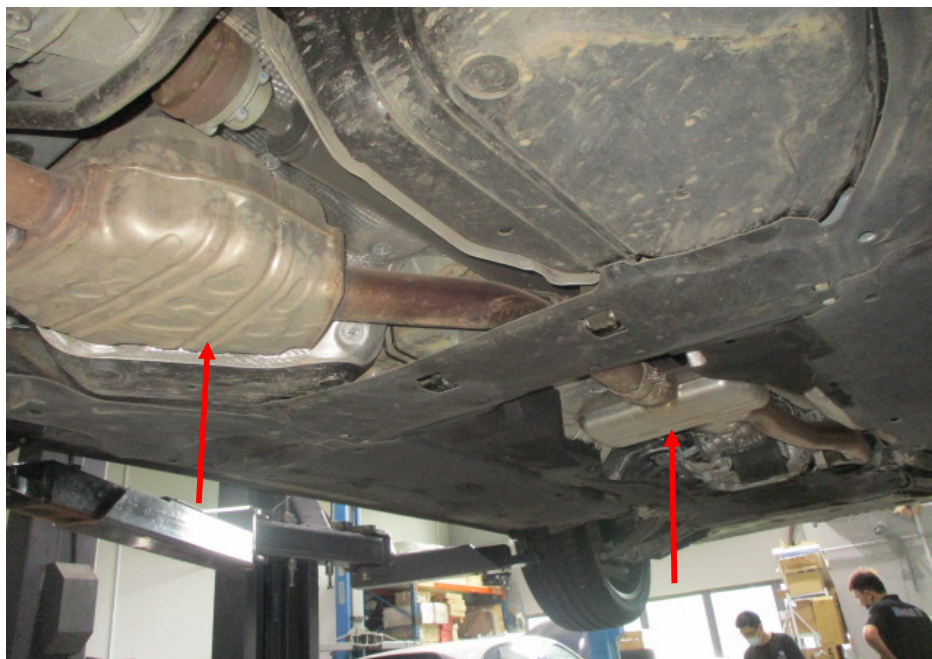
Photo 25 shows a general view of the front section of the Motor Car's exhaust system. My examination of the Motor Car's exhaust system revealed no sign(s) or indication(s) of any cut or weld marks along its exhaust pipes, on its catalytic converter, centre resonator boxes (arrowed) and on its rear muffler.
