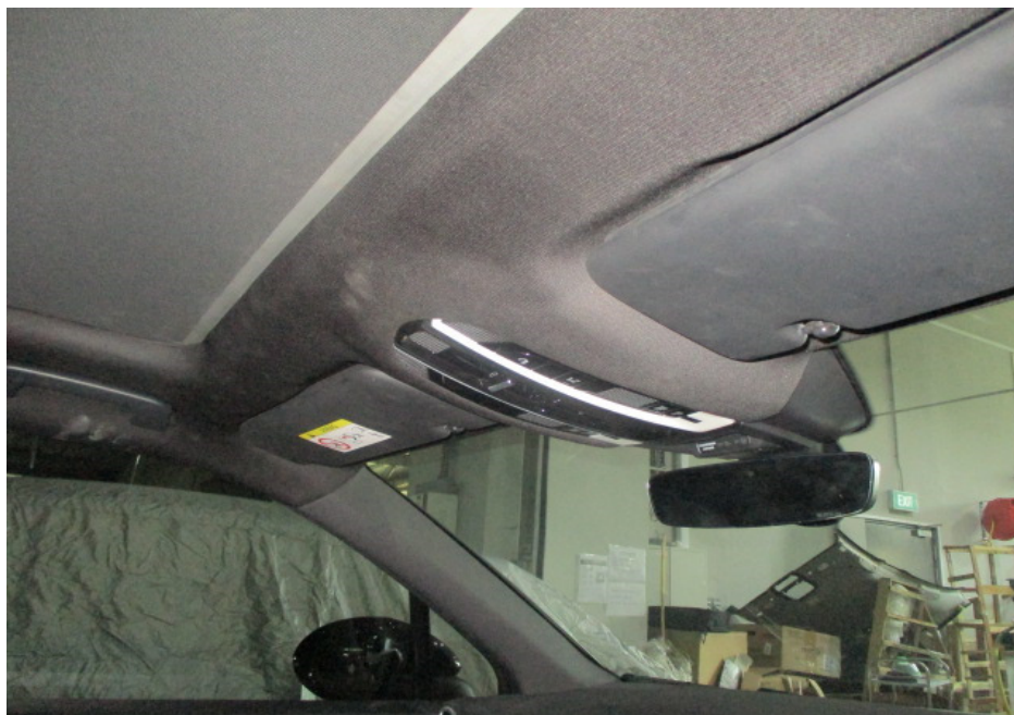
Photo 14 shows a closer view of the Motor Car's interior roof upholstery, interior sun visors, rear view mirror and interior top control panel. The repair/restoration works carried out to the damaged area of the Motor Car (refer to photograph 3 & 4 above) were reasonably adequate and in order.
