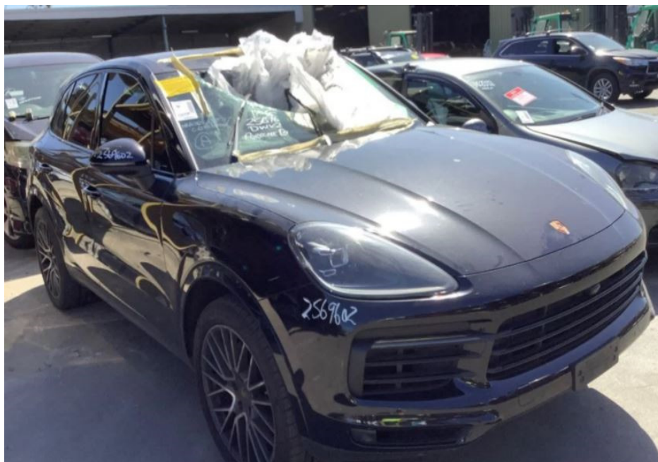
Photo 1 shows the front right body of the Motor Car prior to any repairs being carried out (photograph provided to me). The Motor Car did not appear to have sustain physical damage to its exterior body panels. Its front windscreen was however observed to be shattered.
