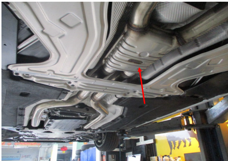
Photo 24 shows a general view of the front section of the Motor Car's exhaust system. My examination of the Motor Car's exhaust system revealed no sign(s) or indication(s) of any cut or weld marks along its exhaust pipes, on its catalytic converters, centre resonator box (arrowed) and on its rear muffler.
