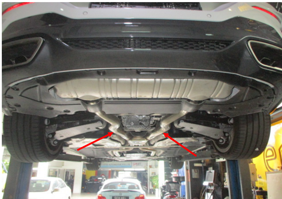
Photo 23 shows a general view of the rear section of the Motor Car's exhaust system. My examination of the Motor Car's exhaust system revealed no sign(s) or indication(s) of any cut or weld marks along its exhaust pipes (arrowed), on its catalytic converters, centre resonator box and on its rear muffler.
