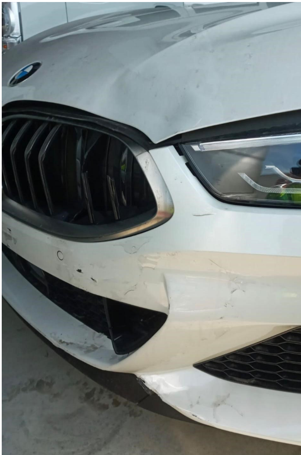
Photo 3 shows a closer view of the damage at the frontal body of the Motor Car prior to any repairs being carried out (photograph provided to me). The front bumper, front bumper centre lower grille, radiator grille and front bonnet were observed to have been damaged.
