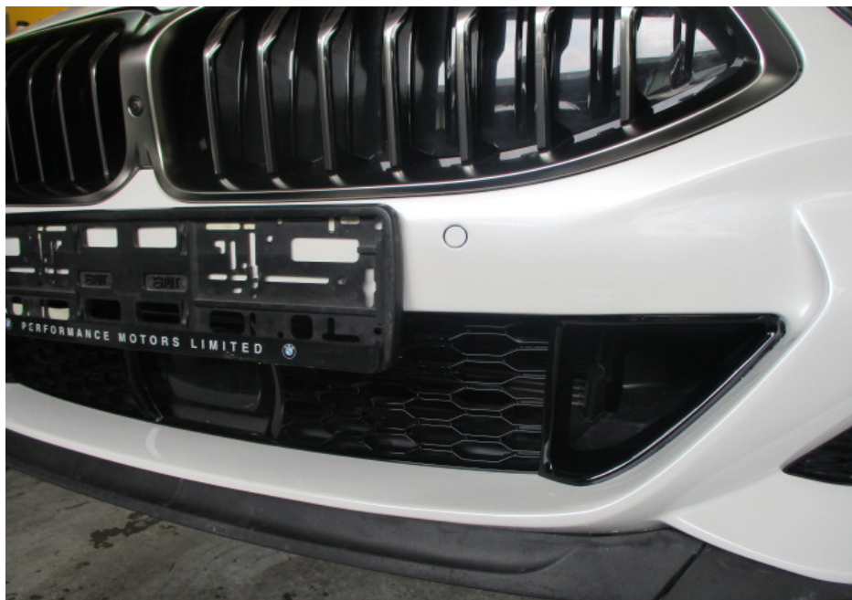
Photo 9 shows a closer view of the front bumper, front bumper centre lower grille and radiator grille of the Motor Car. The body parts at the frontal body of the Motor Car were visually examined and it was observed that the repair/restoration works carried out to the damaged area of the Motor Car (refer to photograph 2 & 3 above) were reasonably adequate and in order.
