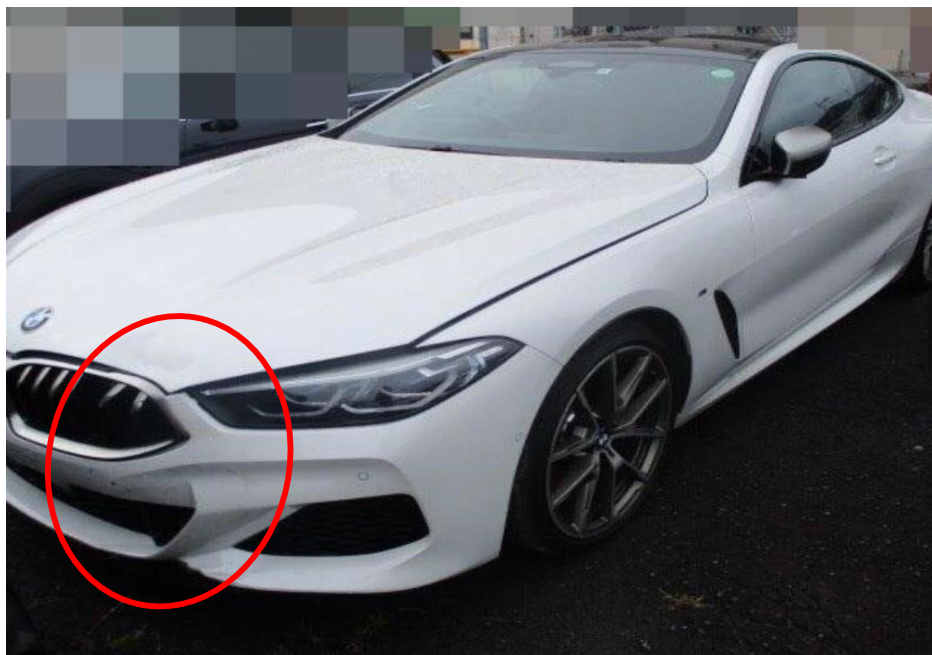
Photo 1 shows the front left body of the Motor Car prior to any repairs being carried out (photograph provided to me). The Motor Car was observed to have sustained relatively minor damage at its frontal body (circled). Body parts damaged include its front bumper, front bumper centre lower grille, radiator grille and front bonnet.
