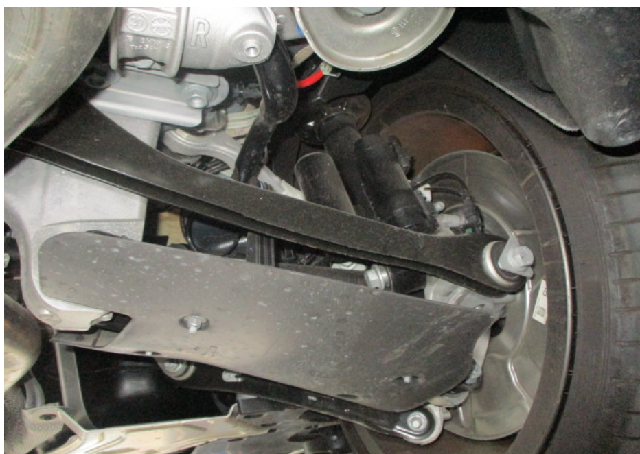
Photo 20 shows the various undercarriage components at the rear right wheel of the Motor Car. The various mechanical components, control arms and linkages were all found to be intact and secured in an appropriate manner.
