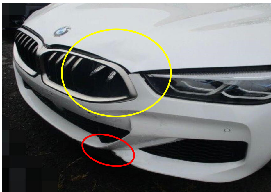
Photo 2 shows a closer view of the damage at the frontal body of the Motor Car prior to any repairs being carried out (photograph provided to me). The front bumper (red circle), radiator grille and front bonnet (yellow circle) were observed to have been damaged.
