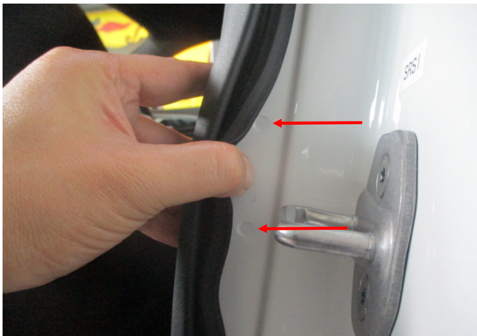
Photo 29 shows the left side rear body panel of the Motor Car. I did not find any weld marks other than original spot weld marks (arrowed) on the left side rear body panel of the Motor Car which, indicates that there was no re-welding works carried out. In general, I had found all the non-detachable body panels of the Motor Car to be originally fitted at the time of my inspection.
