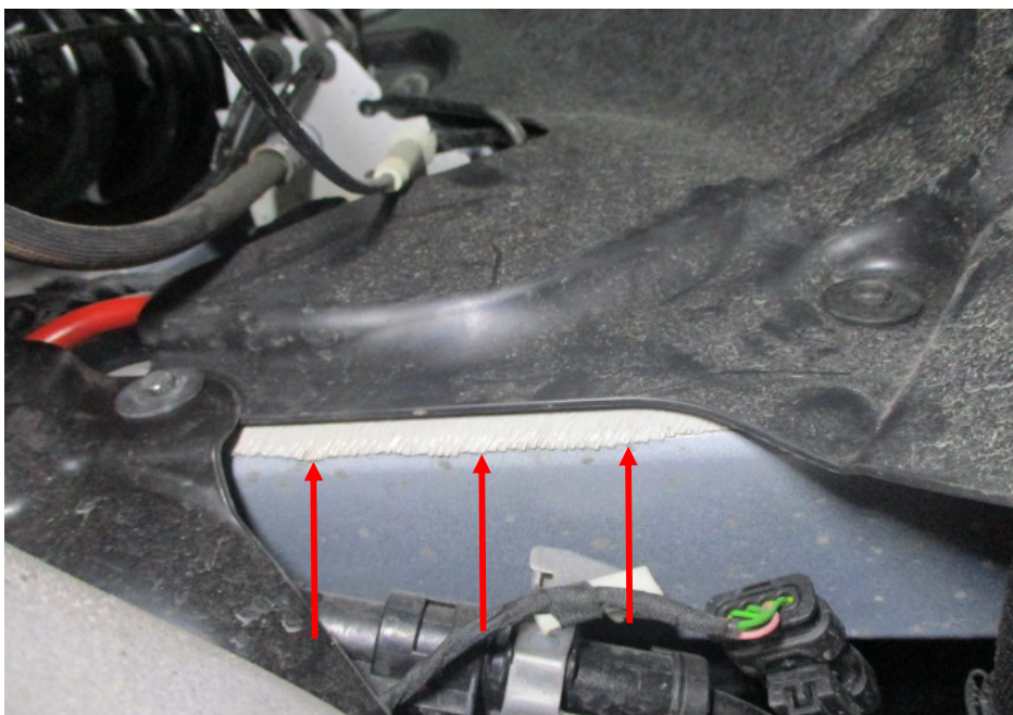
Photo 28 shows the chassis/structural body at the underside front right of the Motor Car. I did not find any weld marks other than original spot weld marks on the chassis/structural body of the Motor Car. The original factory sealant (arrowed) at the joints along the chassis/structural body was untouched, indicating no work was done on the chassis/structural body of the Motor Car and that the chassis/structural body was originally fitted.
