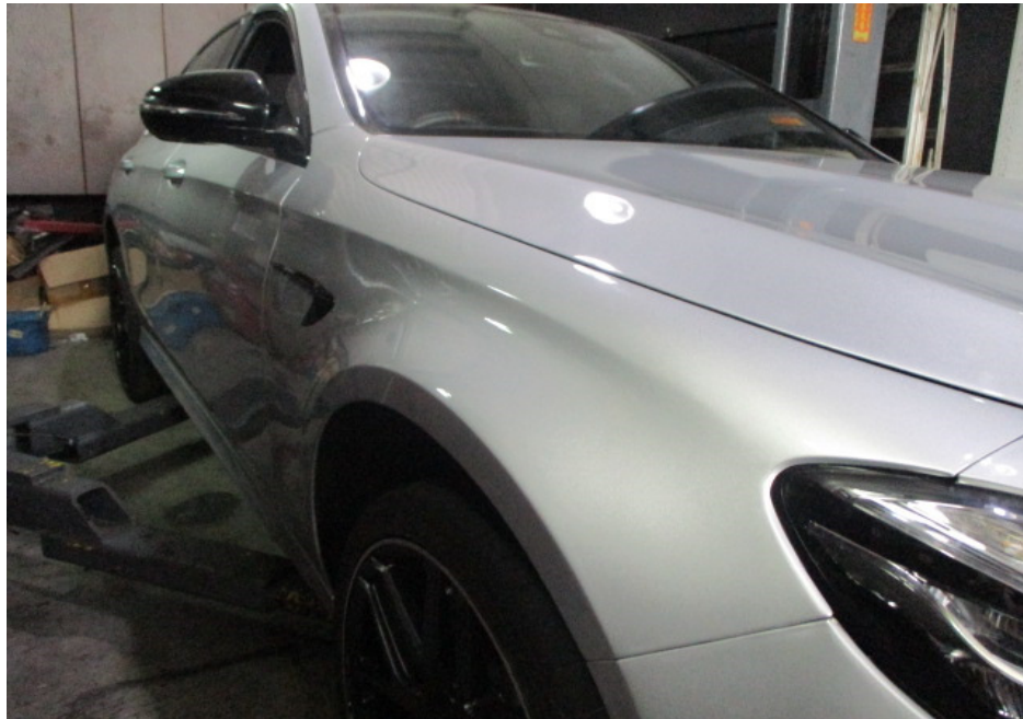
Photo 8 shows a closer view of the front right headlamp, front right fender and front bonnet of the Motor Car. The body parts at the frontal body of the Motor Car were visually examined and it was observed that the repair/restoration works carried out to the damaged area of the Motor Car (refer to photograph 3 above) were reasonably adequate and in order.
