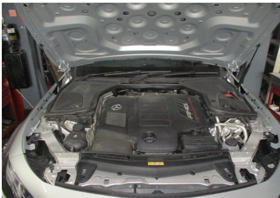
Photo 13 shows a general view of the engine compartment of the Motor Car at the time of my inspection. The various parts and components inside the engine compartment were all observed to be intact and properly fitted. There was also no sign(s) or indication(s) of fluid leak and/or fluid stain found inside the engine compartment. The repair/restoration works carried out to the various parts within the engine compartment like the front top centre panel, front headlamp top right panel, front support panel and front top air duct amongst others, were reasonably adequate and in order.
