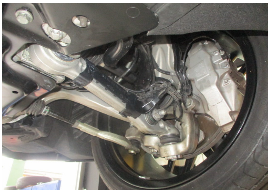
Photo 21 shows the various undercarriage components at the front right wheel of the Motor Car. The mechanical components, control arms and linkages were all found to be intact and secured in an appropriate manner.
