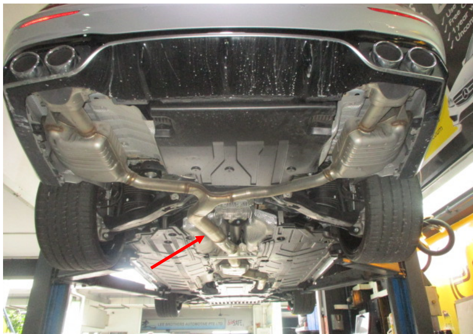
Photo 23 shows a general view of the rear section of the Motor Car's exhaust system. My examination of the Motor Car's exhaust system revealed no sign(s) or indication(s) of any cut or weld marks along its exhaust pipes (arrowed), on its catalytic converter, centre resonator box and on its rear mufflers.
