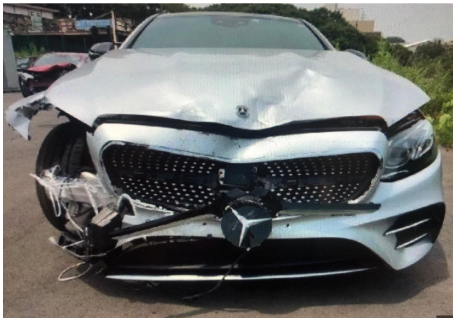
Photo 1 shows the frontal body of the Motor Car prior to any repairs being carried out (photograph provided to me). The Motor Car was observed to have sustained damage at its frontal body. Body parts damaged include its front bumper, front bumper centre garnish, front bumper centre lower grille, radiator grille, front emblem and front bonnet amongst others.
