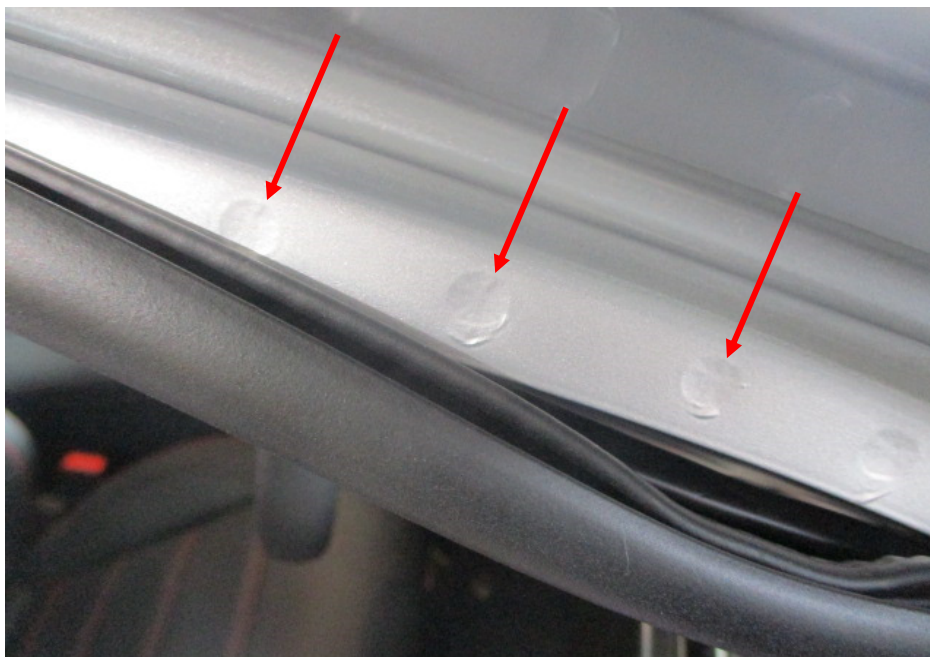
Photo 28 shows the right side "A" pillar of the Motor Car. I did not find any weld marks other than original spot weld marks (arrowed) on the right side "A" pillar of the Motor Car which, indicates that there was no re-welding works carried out. In general, I had found all the non-detachable body panels of the Motor Car to be originally fitted at the time of my inspection.
