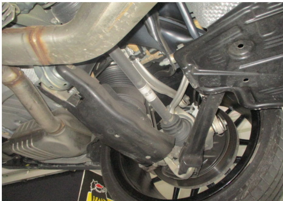
Photo 19 shows a general view of the control arms and linkages at the rear left wheel of the Motor Car. I did not observe any fluid leak and/or fluid stain on the underside of the Motor Car. All the Motor Car's undercarriage components were observed to be intact and secured in an appropriate manner.
