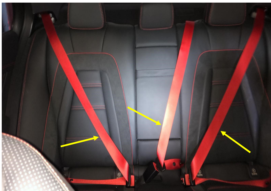
Photo 15 shows the rear seats of the Motor Car. All the seats of the Motor Car were secured via seat rails to the floorboard. They were also fitted with a retractable seat belt reel and a pre-tensioner. The seat belts (arrowed) of the Motor Car were tested and were able to be fastened into the respective pre-tensions that were fitted on the side of each individual seat.
