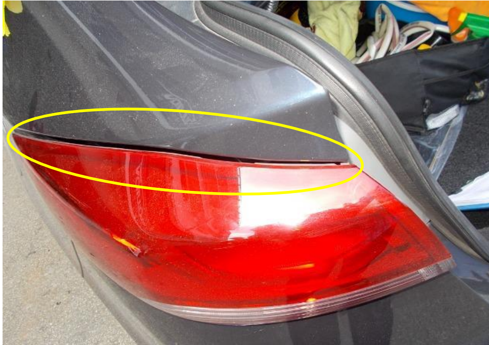
Photo 5 shows the close up view of the rear portion of Car at the time of inspection. The rear left brake lamp was observed to be misaligned (circled).
