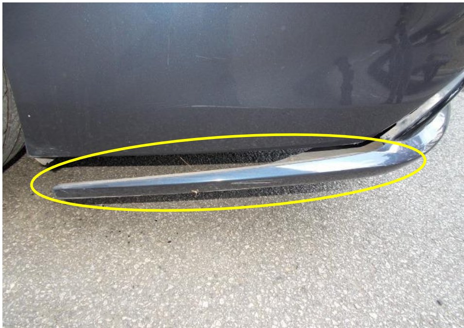
Photo 4 shows the close up view of the rear left portion of Car at the time of inspection. The rear bumper skirting had been damaged. It was also noted that it was dislodged (circled) from the rear bumper of Car.
