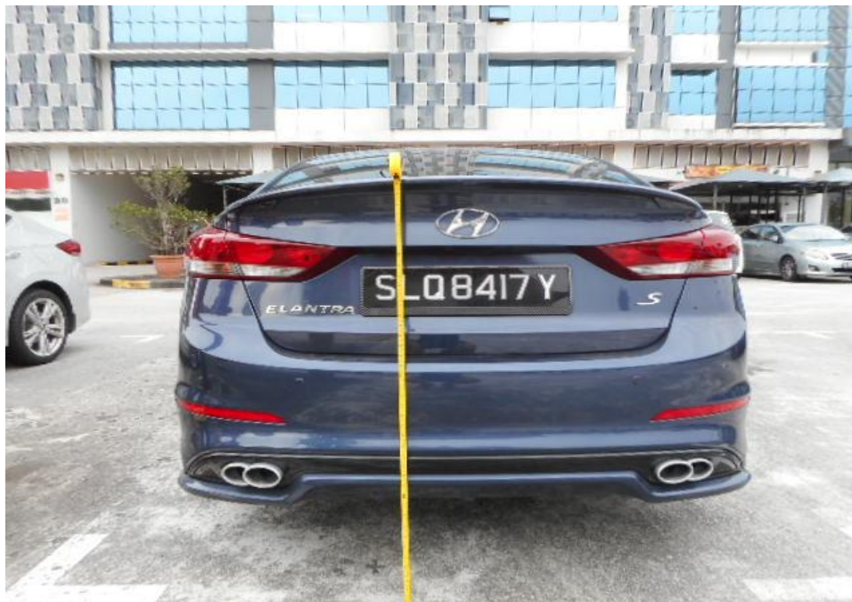
Photo 14 shows the general view of the height measurement being conducted on the rear portion of Car. The height above ground level of where the dislodgement and scratches of the rear bumper skirting, was at, 37cm to 27cm respectively.
