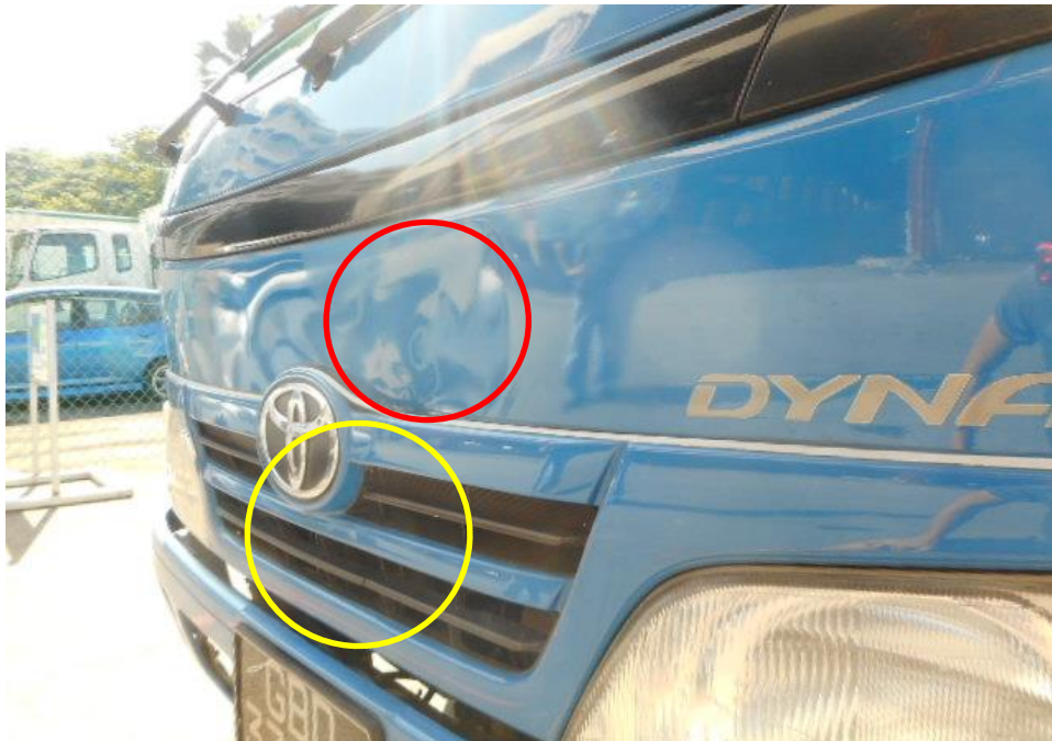
Photo 9 shows a close up view of the Lorry front portion. There were dents observed on the front body panel (red circle) and cracks (yellow circle) on the front emblem and grille of the Lorry.
