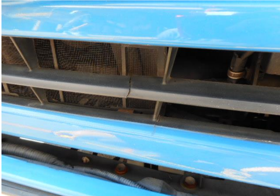
Photo 12 shows a general view of the Lorry front portion. We observed multiple groups of crack marks on the front grille.
