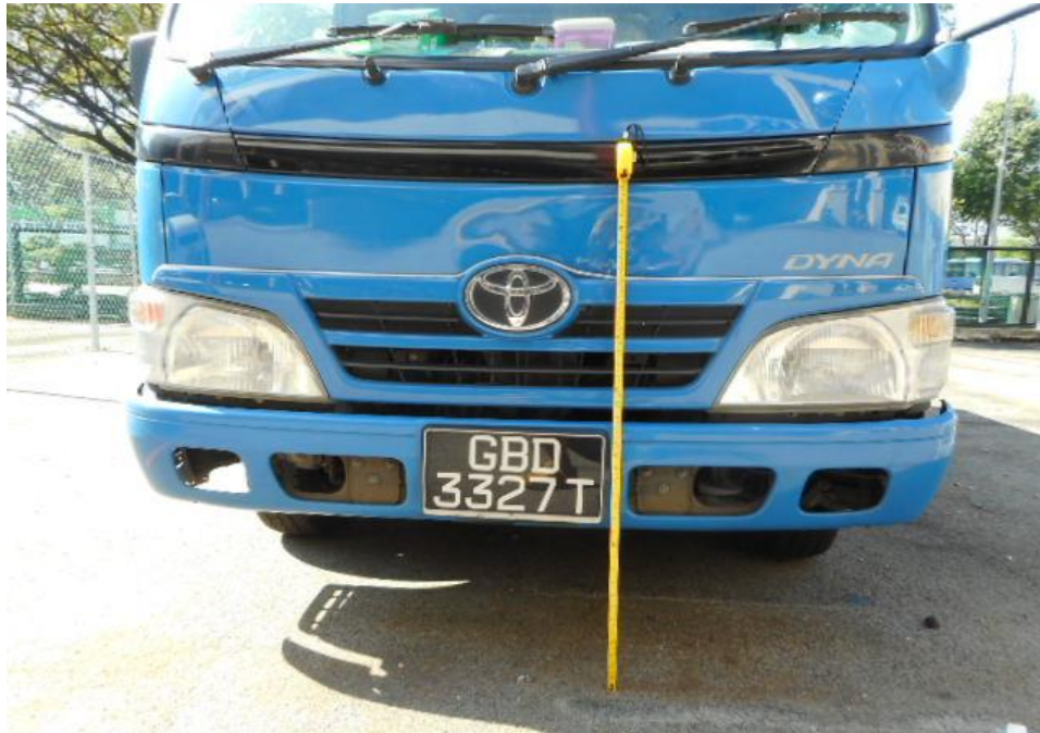
Photo 15 shows a general view of the height measurement being conducted on the front portion of Lorry. The bent and scratched marks on the front left bumper, was measured to be at 55cm to 43cm above ground level.
