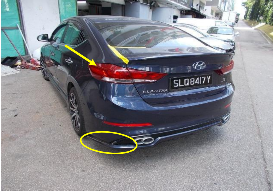
Photo 1 shows the general view of the rear portion of Car at the time of inspection. The rear bumper skirting (yellow circle) had been damaged and dislodged. Also the rear left brake lamp (arrowed) was found to be misaligned.
