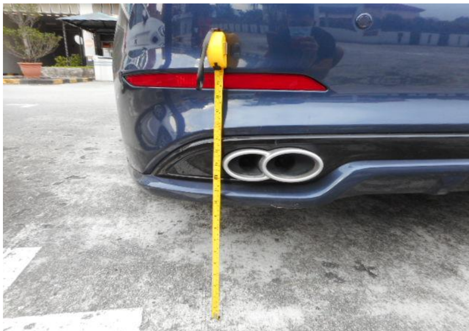
Photo 16 shows the general up view of the height measurement being conducted on the rear portion of Car. The height above ground level of where the damaged and dislodgment were found on the rear bumper skirting of the Car was at 37cm to 27cm.
