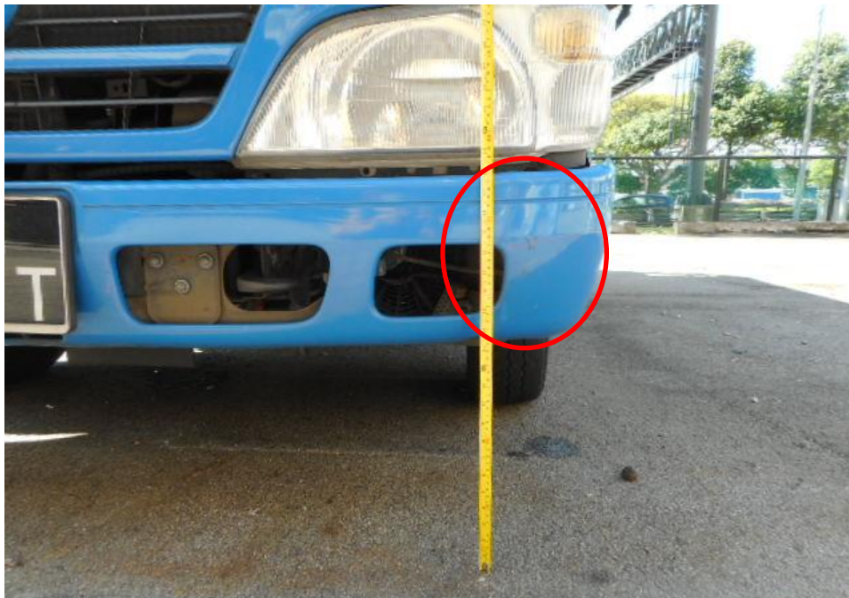
Photo 7 shows a close up view of the Lorry front left bumper portion. There were damages observed on the front bumper there when bent mark and scratch marks (circled).
