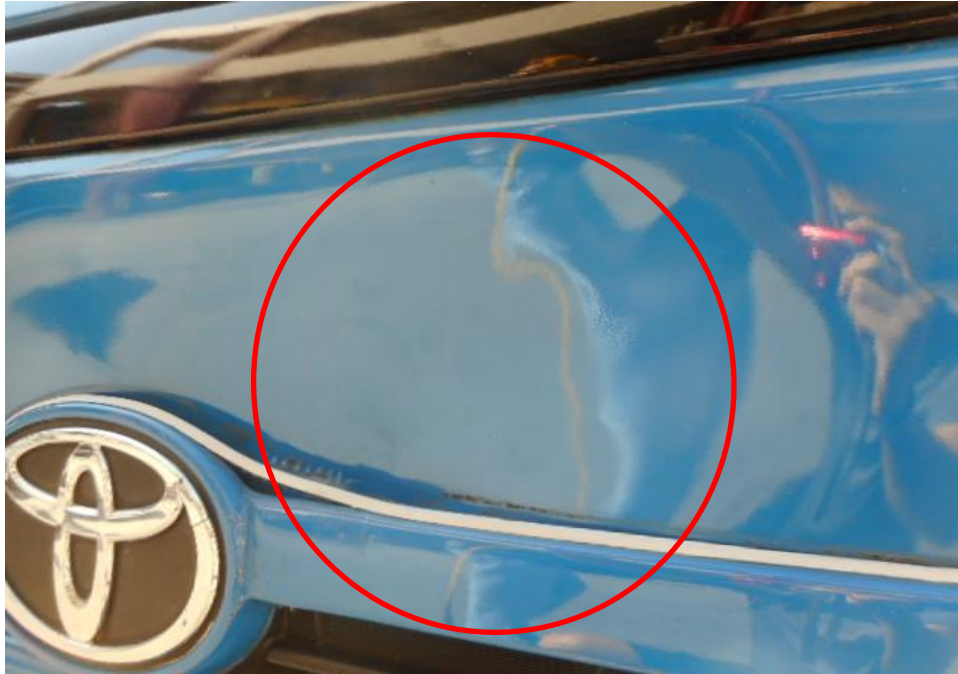
Photo 10 shows a close up view of the Lorry front portion. We observed dent on its front body panel (circled).
