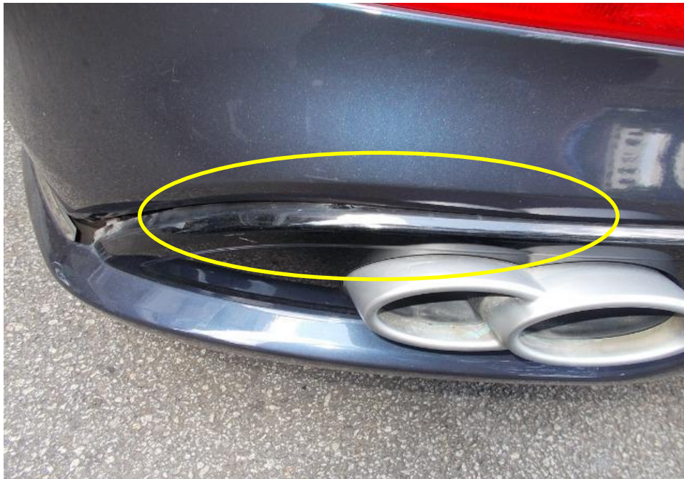
Photo 2 shows the close up view of the rear left portion of Car at the time of inspection. The rear bumper skirting had been damaged. It was also noted that it was dislodged (circled) from the rear bumper of Car.
