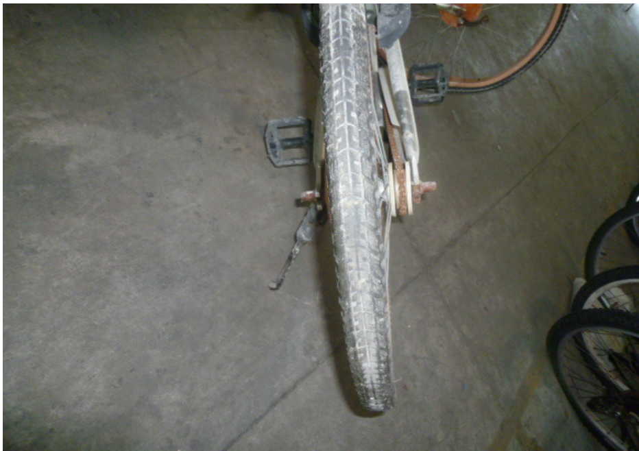
Photo 12 shows the rear tyre of the Bicycle. The pattern of the tread was clearly visible. There was no tear, burst mark(s) and/or punctured hole(s) on the sidewalls as well as across the tread of the front tyre. The rear tyre was also observed to be sufficiently inflated for vehicular operation.
