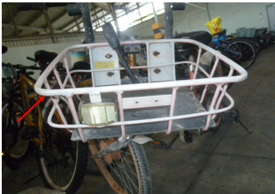
Photo 6 shows the damaged front basket (arrowed) of the Bicycle at the time of our inspection.
