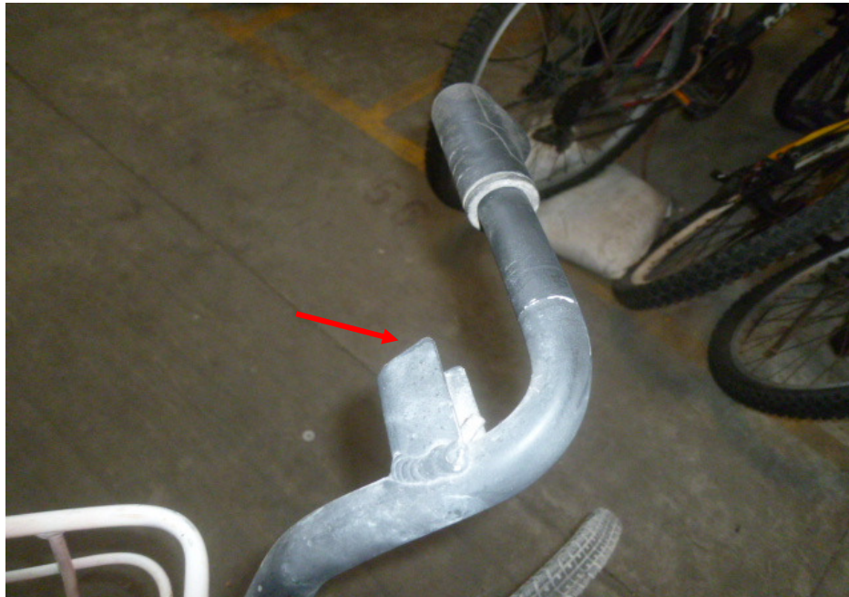
Photo 17 shows the right handlebar of the Bicycle. Upon closer inspection, we observed that there was no hand brake lever fitted on the right handlebar of the Bicycle (arrowed).
