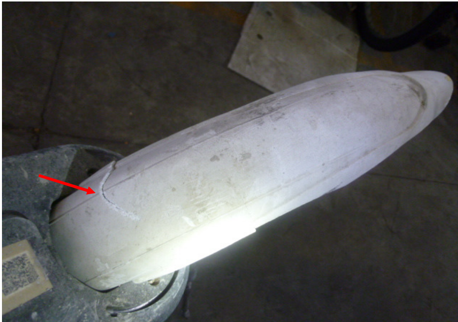
Photo 9 shows the cracked rear mudguard (arrowed) of the Bicycle at the time of our inspection.
