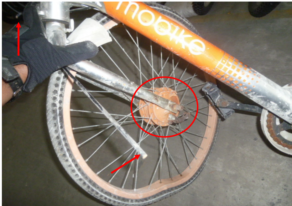
Photo 18 shows the front wheel of the Bicycle. The type of brake system for the front wheel was of a mechanical type, controlled by the left hand lever of the Bicycle. Our checks on the spring and drum (circled), which are all part of the components in the front brake system of the Bicycle reveal all to be intact and without damage. However we also found that the brake cables for the front and rear braking system of the Bicycle were cut (arrowed).
