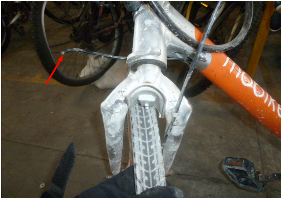
Photo 19 shows a closer view of the brake cable for the rear braking system of the Bicycle which was observed to be cut (arrowed).
