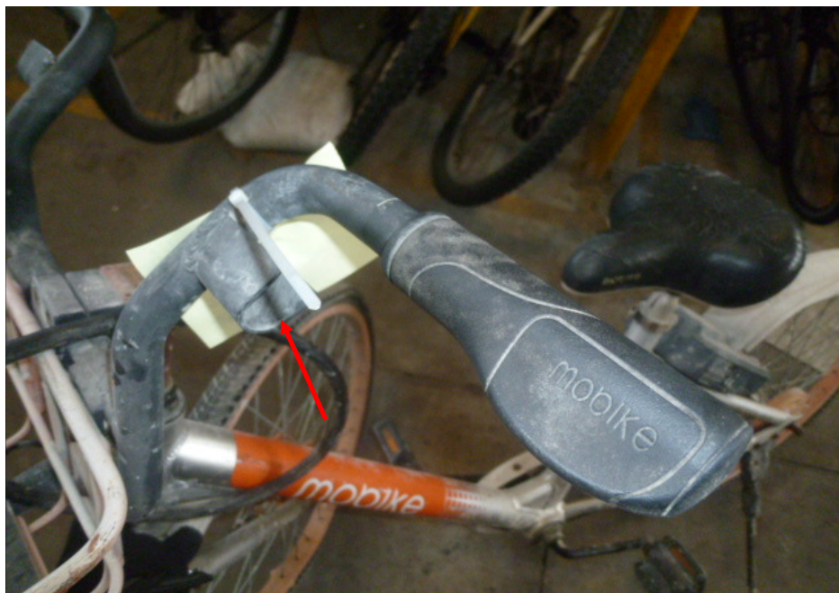
Photo 16 shows the left handlebar of the Bicycle. Upon closer inspection, we observed that there was no hand brake lever fitted on the left handlebar of the Bicycle (arrowed).
