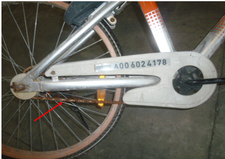
Photo 13 shows the general view of the gear train of the Bicycle, which was observed to be intact with no misalignment. However it was observed not to be adequately lubricated for operating purposes (arrowed).
