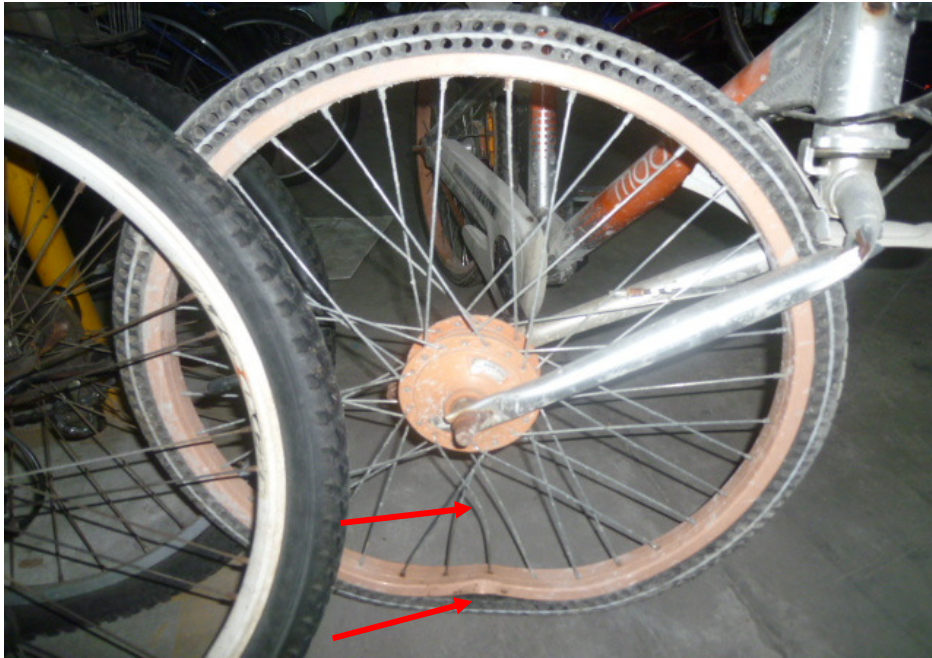
Photo 11 shows the bent spokes and front wheel rim of the Bicycle at the time of our inspection (arrowed).
