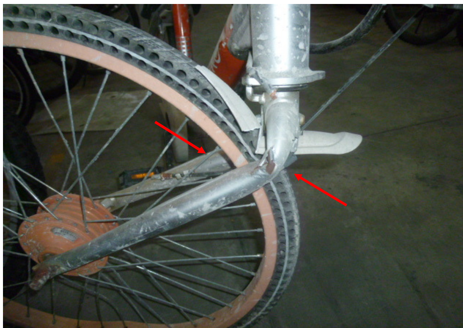
Photo 15 shows the front fork assembly (arrowed) of the Bicycle. The front forks of the Bicycle were both found to be bent as a result of the accident, hence causing the whole steering system to be out of alignment and rendering the Bicycle immobile for any static or operational tests.
