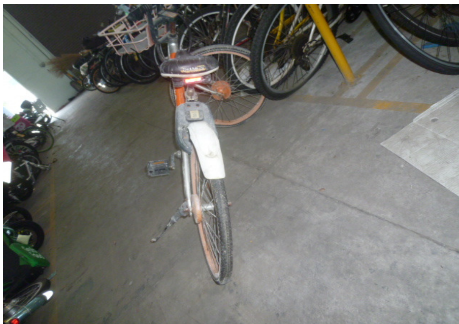
Photo 4 shows the rear portion of the Bicycle at the time of our inspection. The Bicycle had sustained damages all around. The body parts that were found to have been damaged include its front basket, front fork assembly, front mudguard, left pedal and rear mudguard, amongst others as a result of the accident.
