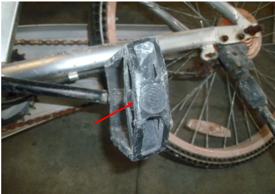
Photo 8 shows the damaged right pedal of the Bicycle (arrowed) at the time of our inspection.
