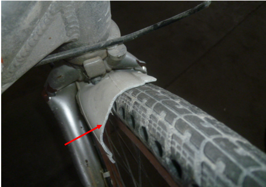
Photo 7 shows the broken front mudguard (arrowed) of the Bicycle at the time of our inspection.
