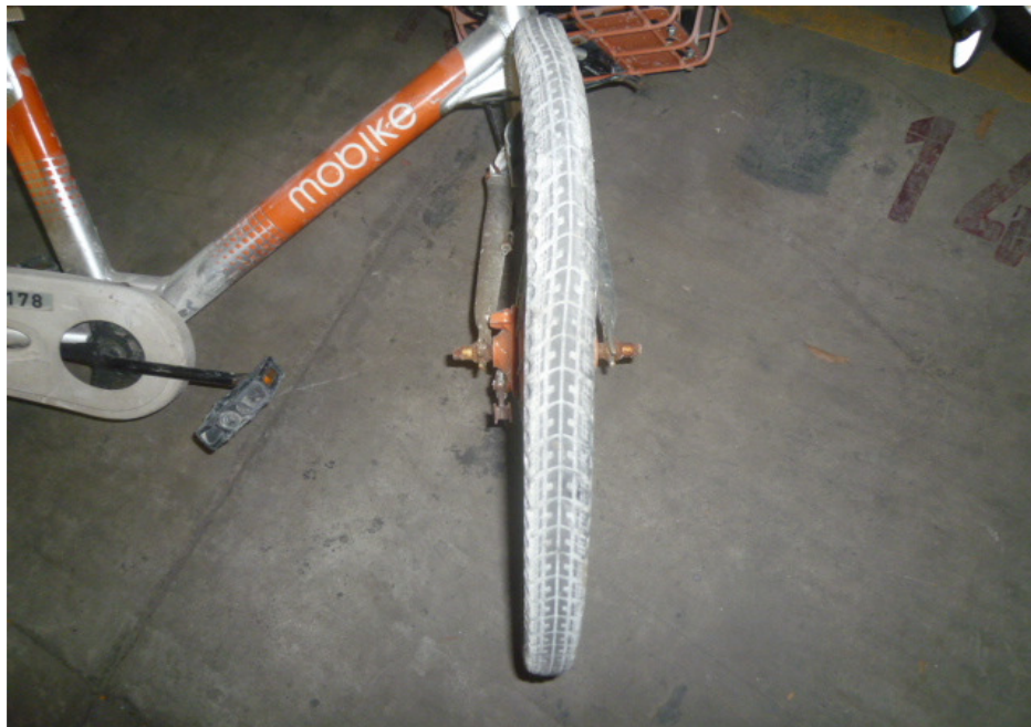
Photo 10 shows the front tyre of the Bicycle. The pattern of the tread was clearly visible. There was no tear, burst mark(s) and/or punctured hole(s) on the sidewalls as well as across the tread of the front tyre. The front tyre was also observed to be sufficiently inflated for vehicular operation.
