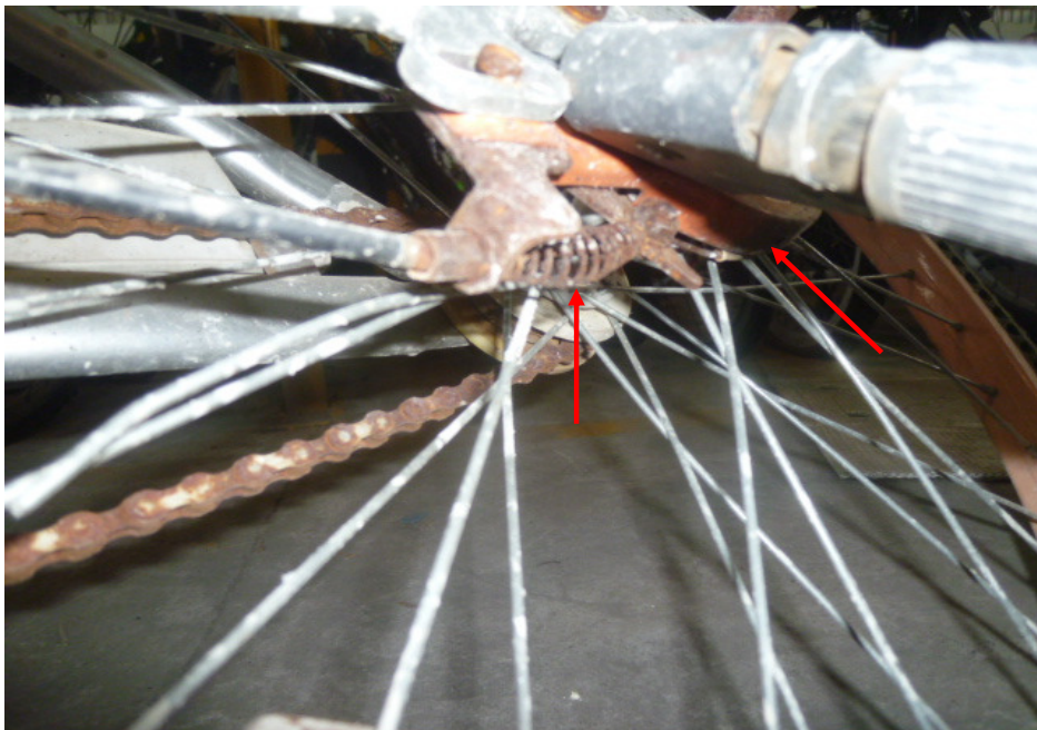
Photo 20 shows the rear wheel of the Bicycle. The type of brake system for the rear wheel was of a mechanical type, controlled by the right hand lever of the Bicycle. Our checks on the spring and drum (circled), which are all part of the components in the rear brake system of the Bicycle reveal all to be intact and without damage (arrowed).
