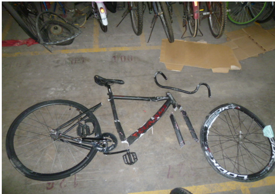
Photo 2 shows the right body of the Bicycle at the time of our inspection. The Bicycle had sustained damages all around. The body parts that were found to have been damaged include its front fork assembly, handlebar, frame, seat and pedals, amongst others as a result of the accident.
