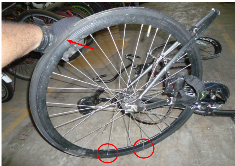
Photo 11 shows the bent rear wheel rim (circled) and deflated rear tyre of the Bicycle most likely as a result of the accident (arrowed). The pattern of the tread was clearly visible.
