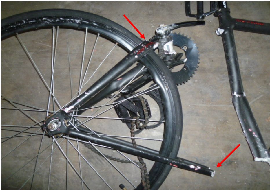
Photo 8 shows the dislodged rear frame of the Bicycle as a result of the accident (arrowed).
