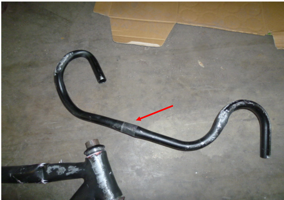
Photo 16 shows the dislodged handlebar (arrowed) of the Bicycle. The Bicycle was found not to be fitted with a braking system. Hence we were unable to conduct any static or operational tests of the braking system.
