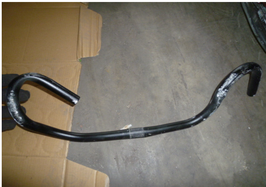
Photo 3 shows the deformed handlebar of the Bicycle at the time of our inspection.
