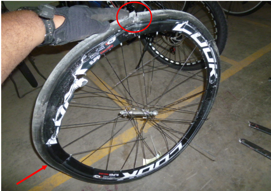
Photo 9 shows the bent front wheel rim and deflated front tyre of the Bicycle most likely as a result of the accident (arrowed). The pattern of the tread was clearly visible. However we also observed a cut/tear on the front tyre (circled).
