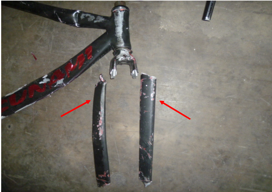
Photo 15 shows the front fork assembly (arrowed) of the Bicycle. The front forks and fork bracket of the Bicycle were both found to be broken and dislodged as a result of the accident, hence causing the whole steering system to be out of alignment and rendering the Bicycle immobile for any static or operational tests.
