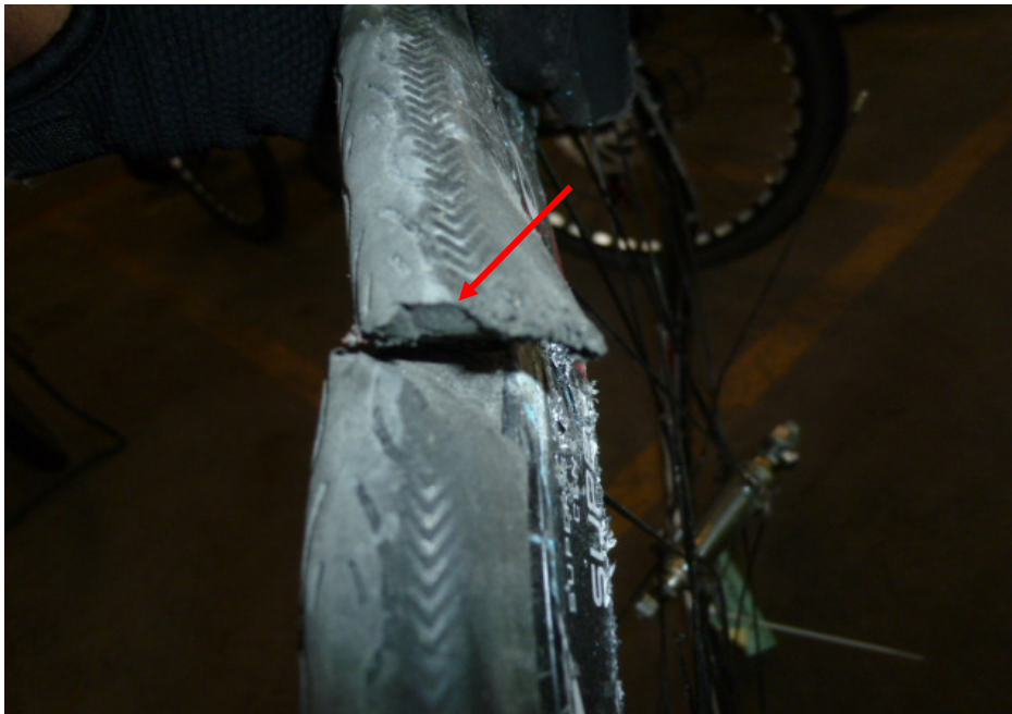
Photo 10 shows a close up view of the cut/tear on the front tyre of the Bicycle most likely as a result of the accident (arrowed).
