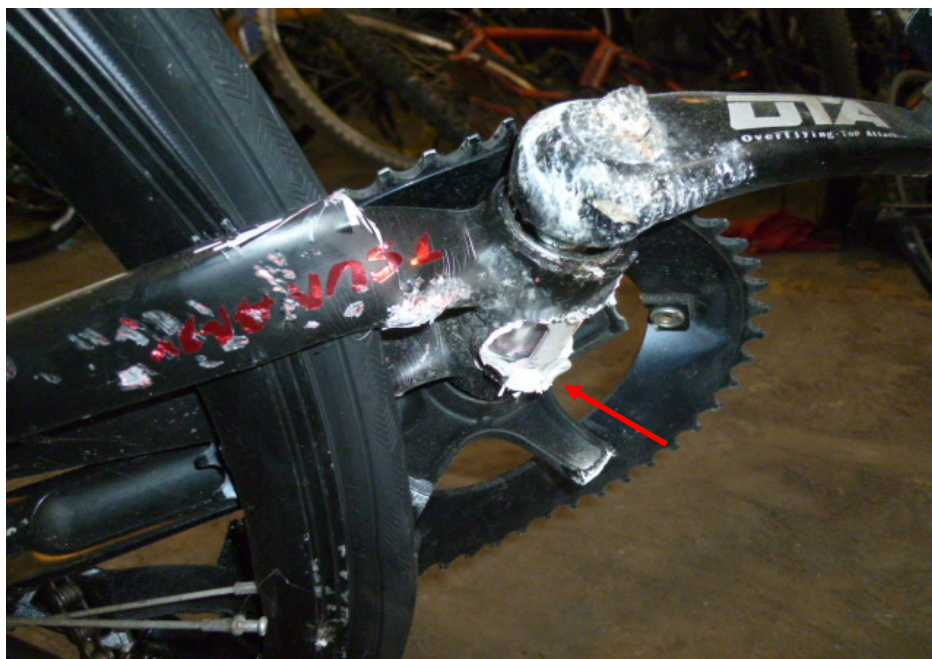
Photo 6 shows the broken left pedal of the Bicycle as a result of the accident (arrowed).
