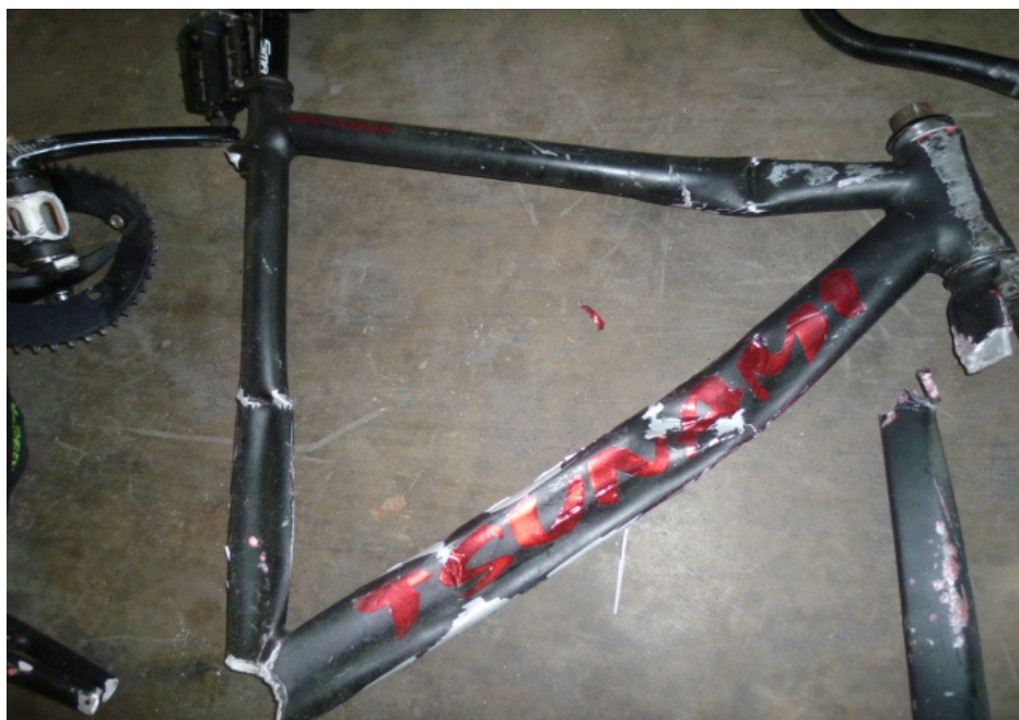
Photo 4 shows the bent frame of the Bicycle as a result of the accident.
