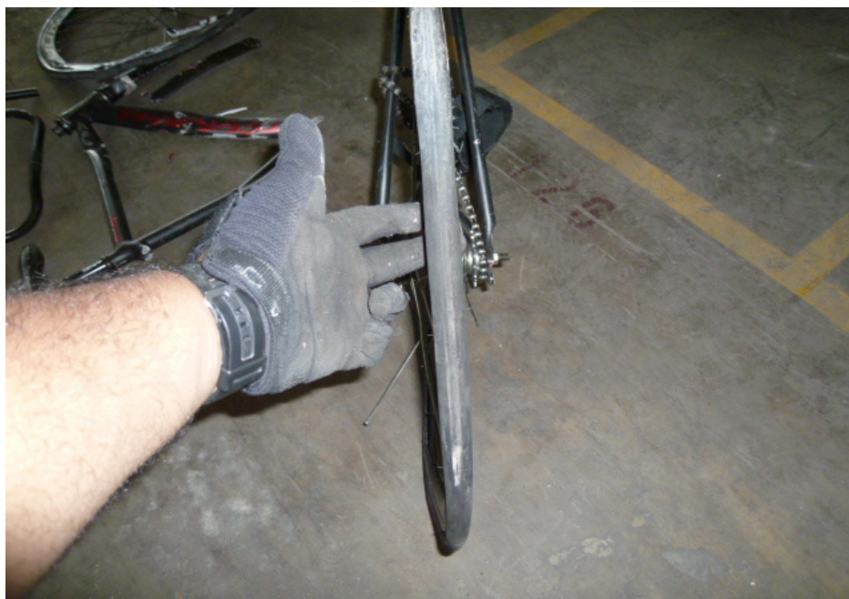
Photo 12 shows the deflated rear tyre of the Bicycle. The pattern of the tread was clearly visible. There was no tear, burst mark(s) and/or punctured hole(s) on the sidewalls as well as across the tread of the rear tyre.
