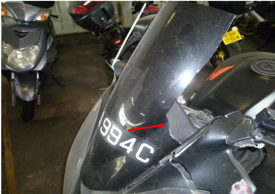
Photo 5 shows a close up view of the cracked windshield which was amongst the body parts of the Motorcycle that had sustained damage as a result of the accident (arrowed).
