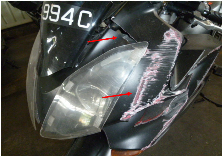
Photo 6 shows a closer view of the cracked and grazed head cowling which was amongst the body parts at the front body of the Motorcycle that had sustained damage as a result of the accident (arrowed).
