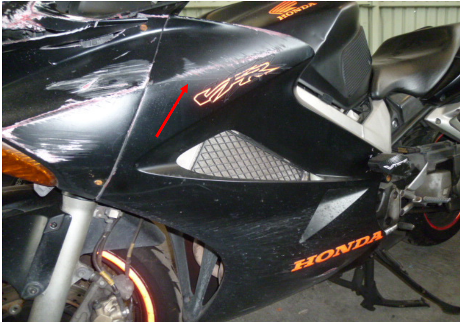
Photo 7 shows a closer view of the left cowling of the Motorcycle that had sustained damages of grazing nature as a result of the accident (arrowed).
