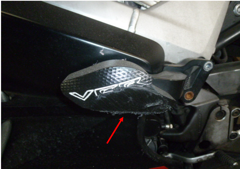
Photo 10 shows a closer view of the left frame slider which was amongst the body parts of the Motorcycle that had sustained damages of grazing nature as a result of the accident (arrowed).
