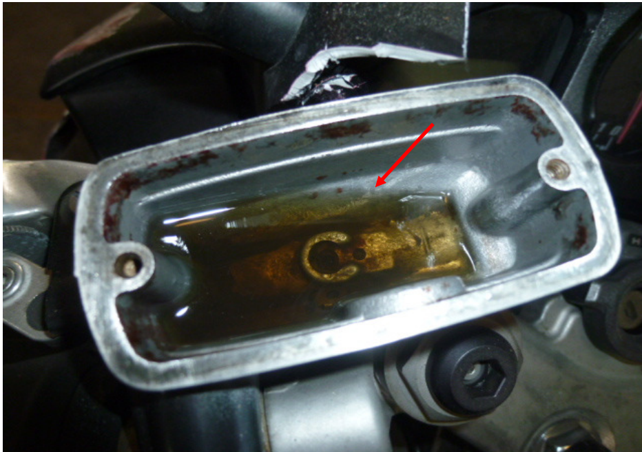
Photo 24 shows the hydraulic clutch fluid reservoir for the hydraulic clutch system of the Motorcycle. The hydraulic clutch fluid was observed to be of insufficient level for operational purposes. It was also found to be slightly contaminated (arrowed).
