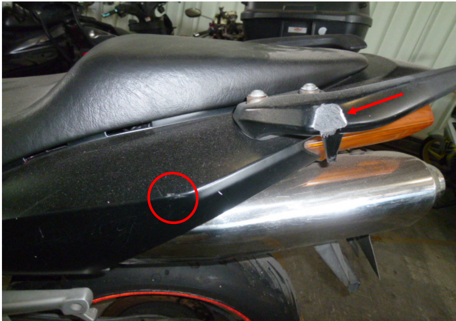
Photo 12 shows a closer view of the grazed left rear side cover (circled) and left pillion grab rail (arrowed) of the Motorcycle as a result of the accident.
