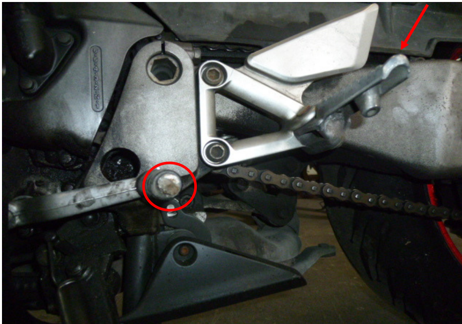
Photo 9 shows a closer view of the gear shift pedal (circled) and left front footrest (arrowed) which were amongst the body parts of the Motorcycle that had sustained damage as a result of the accident.
