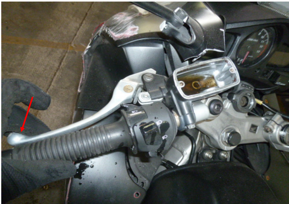
Photo 25 shows the clutch lever being depressed. There was some resistance felt (spongy like feel) upon pressing the clutch lever (arrowed). This would indicate that there is no leakage of pressure/vacuum in the hydraulic clutch system.
