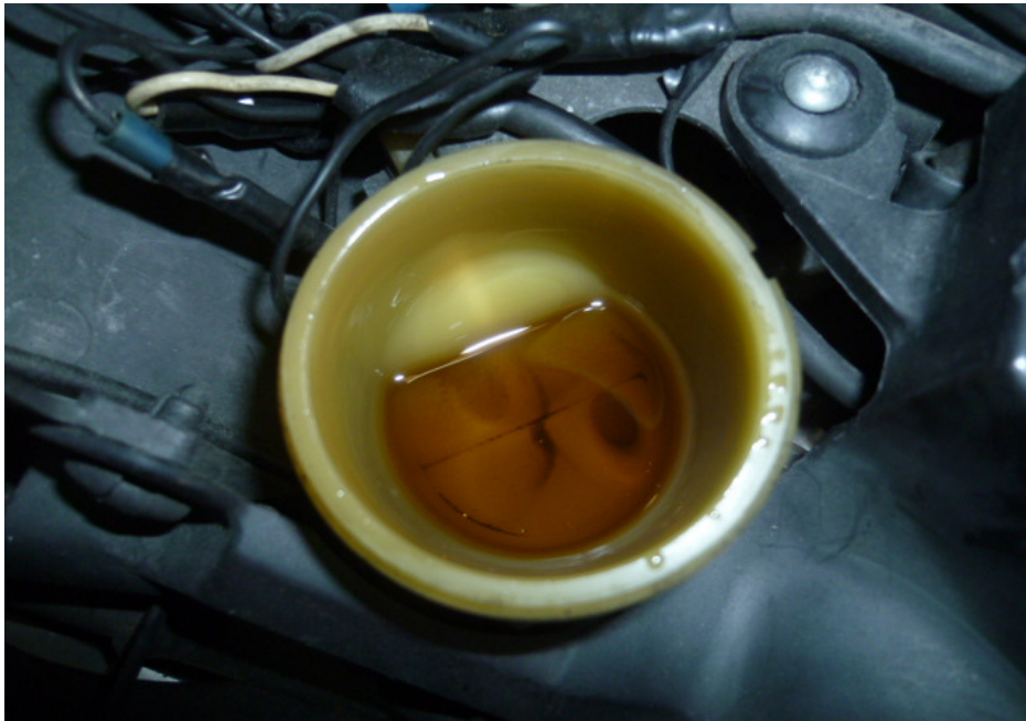
Photo 24 shows the brake fluid reservoir for the rear brake of the Motorcycle. The brake fluid was observed to be of sufficient level for operational purposes and without contamination.
