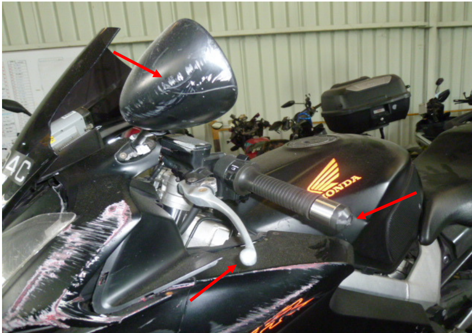
Photo 8 shows a closer view of the clutch lever, left handlebar end and left side mirror (arrowed) which were amongst the body parts of the Motorcycle that had sustained damage as a result of the accident.
