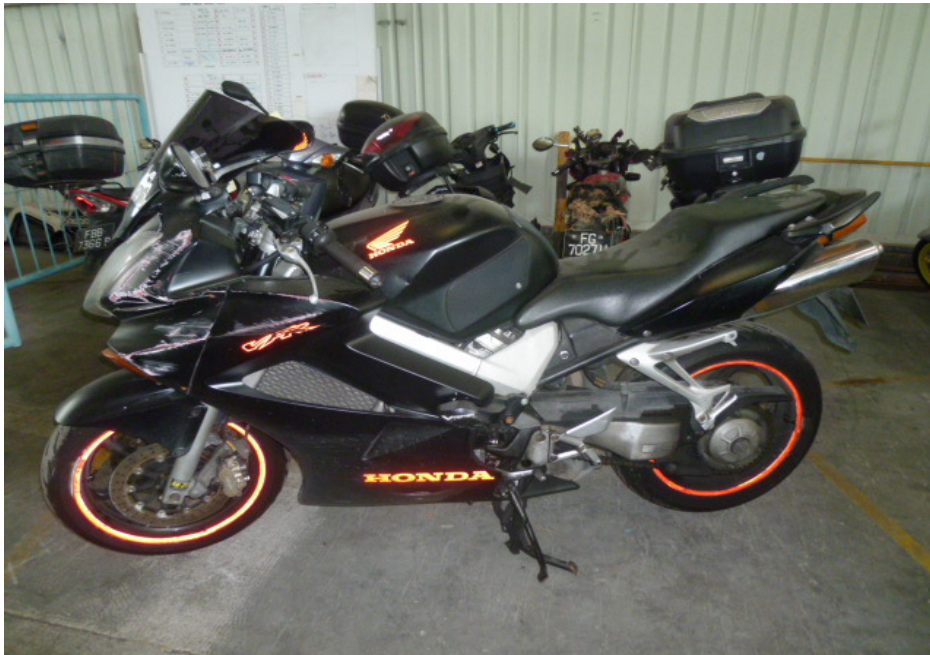
Photo 4 shows a general view of the left body of the Motorcycle at the time of our inspection. The Motorcycle was observed to have sustained at its frontal portion and left body. The body parts that were found to have been damaged include its windshield, head cowl, left cowl, left frame slider, left handlebar end, left side mirror, gear shift pedal, left front footrest, left pillion foot peg, left rear side cover and left pillion grab rail, amongst others.
