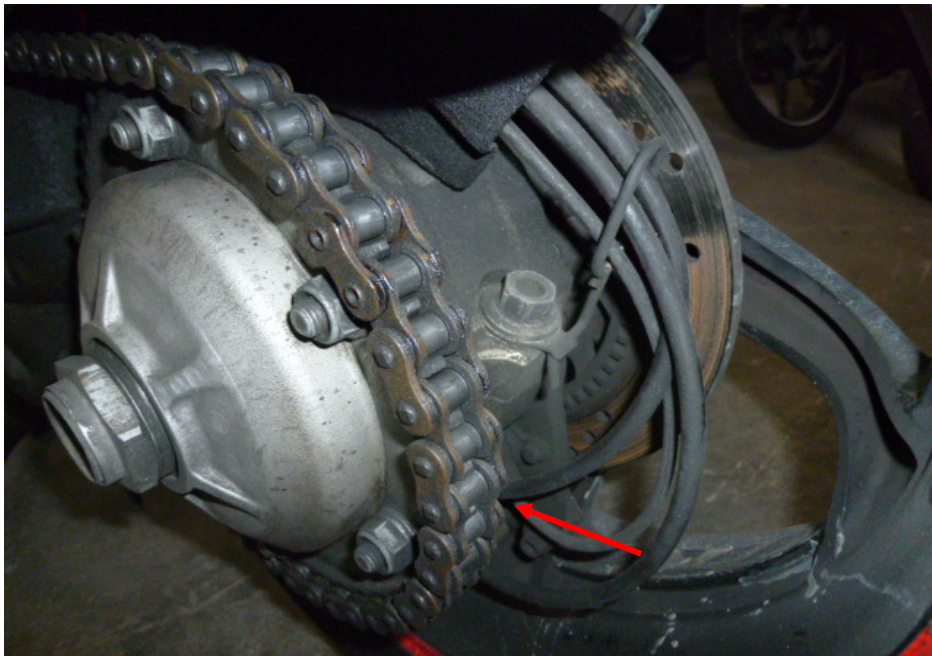
Photo 18 shows a closer view of the gear train (arrowed) of the Motorcycle, which was observed to be intact with no misalignment. It was also adequately lubricated for operating purposes.
