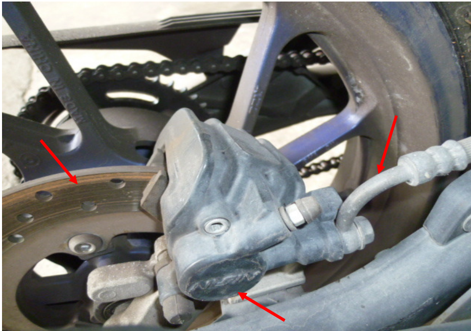
Photo 25 shows a close up view of the rear brake caliper, rear brake disc and rear brake hose (arrowed) of the Motorcycle, which are all part of the components in the hydraulic rear brake system of the Motorcycle. Our visual checks of these various components had revealed all to be intact with no visible damage. No leakage of brake fluid was also observed.
