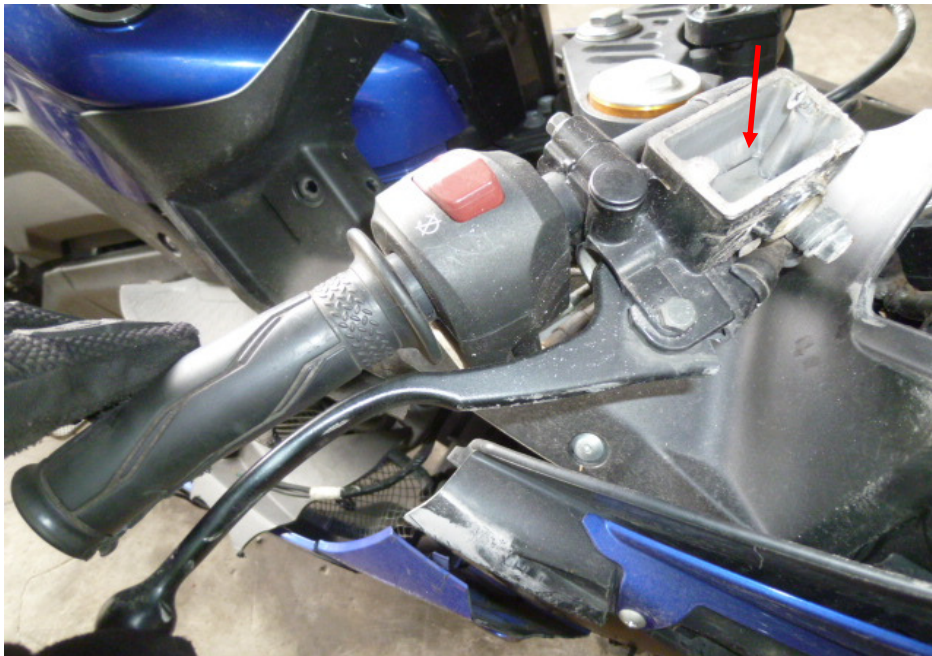
Photo 24 shows the front brake lever being depressed. The front brake reservoir cover was observed to be missing as a result of the accident. The front brake reservoir was also found to be empty (arrowed). Hence we were unable to indicate if there was any leakage of pressure/vacuum in the front brake system of the Motorcycle.
