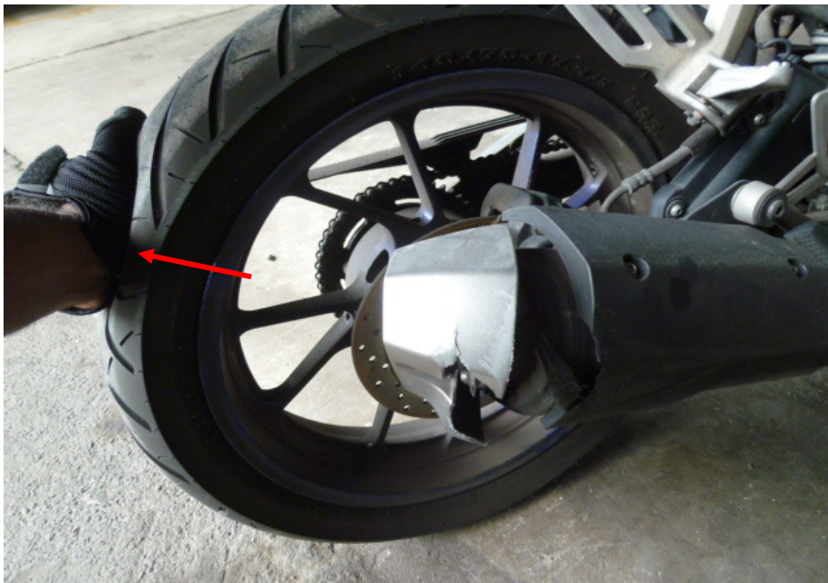
Photo 15 shows the condition of the Motorcycle's rear tyre. The rear tyre was observed to be in serviceable condition with remaining tread depth of approximately 3mm. We did not observe any tear, burst mark(s) and/or punctured hole(s) on the sidewalls as well as across the tread of the rear tyre. However the tyre was also observed to be deflated (arrowed).
