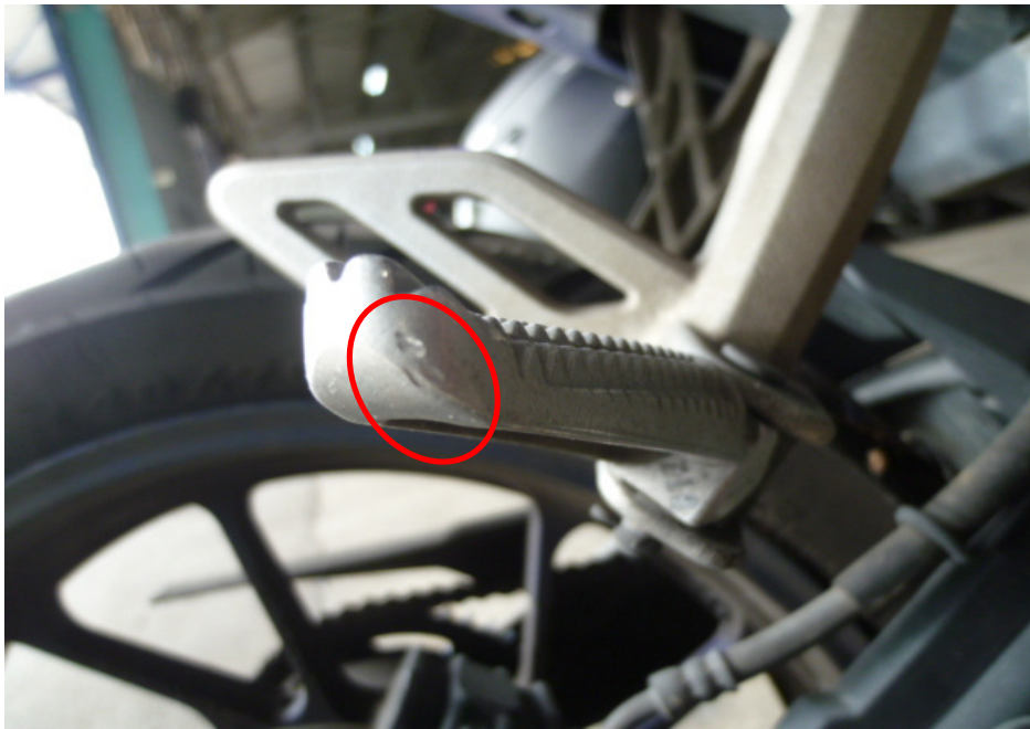
Photo 10 shows a closer view of the left pillion foot peg (circled) which was amongst the body parts of the Motorcycle that had sustained damage as a result of the accident.
