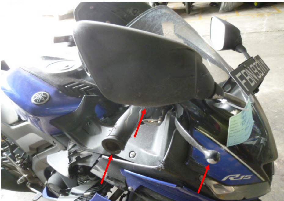
Photo 7 shows a closer view of the right handlebar grip, right side mirror and front brake lever which was amongst the body parts of the Motorcycle that had sustained damage as a result of the accident (arrowed).
