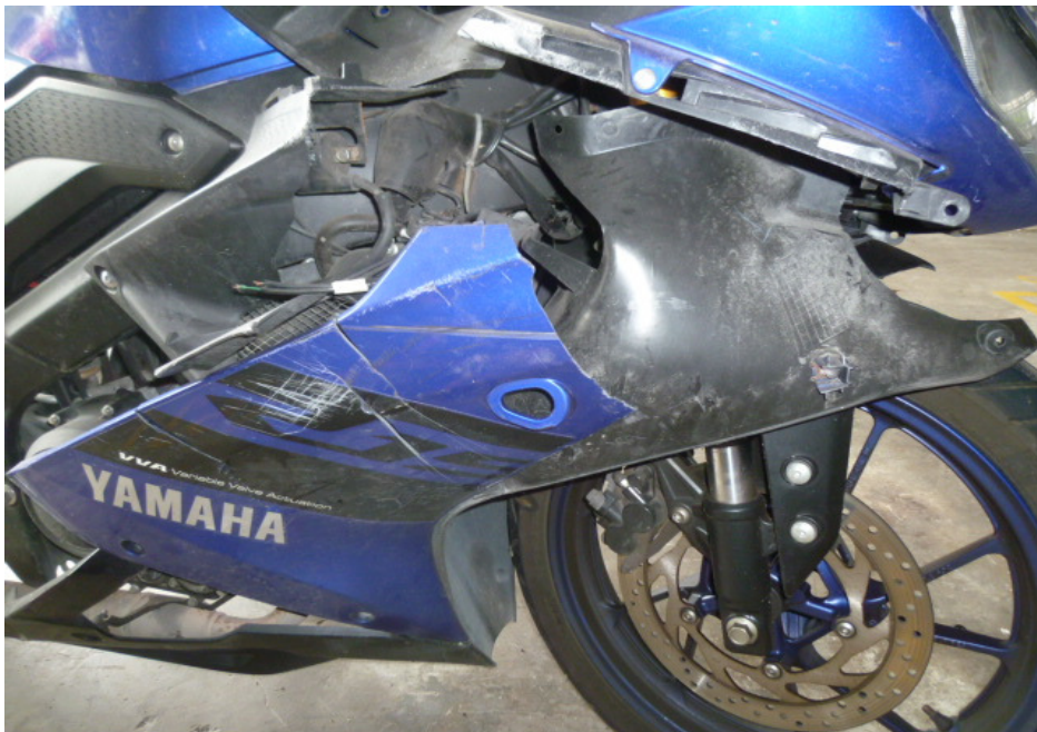
Photo 9 shows a closer view of the cracked right cowling of the Motorcycle as a result of the accident.
