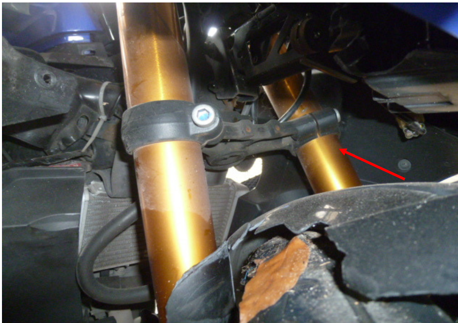
Photo 20 shows the front forks of the Motorcycle. The left front fork was observed to be bent (arrowed) as a result of the accident. Hence we were unable to turn the handle bar towards the left or right.
