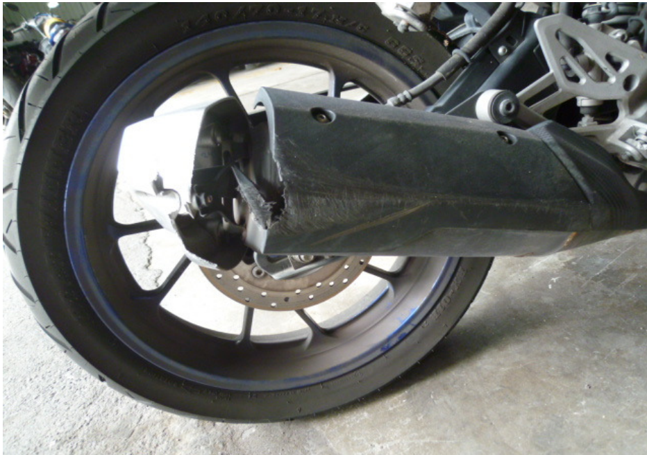
Photo 12 shows a closer view of the cracked exhaust muffler heat shield of the Motorcycle as a result of the accident.
