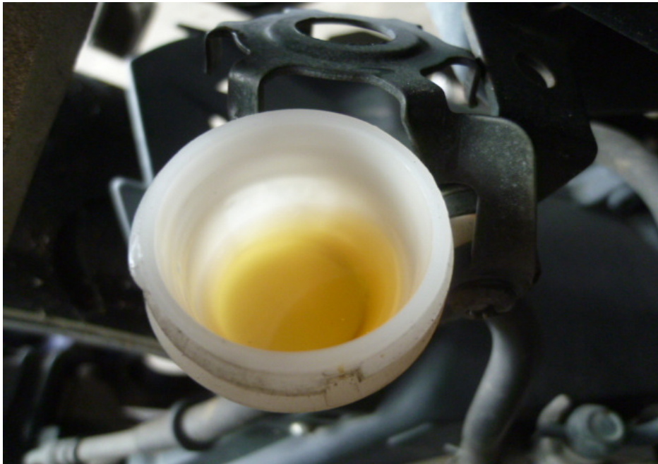
Photo 26 shows the brake fluid reservoir for the rear brake of the Motorcycle. The brake fluid was observed to be of sufficient level for operational purposes and without contamination.
