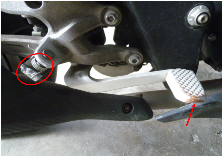
Photo 13 shows the broken right front footrest (circled) and grazed rear brake pedal (arrowed) of the Motorcycle as a result of the accident.
