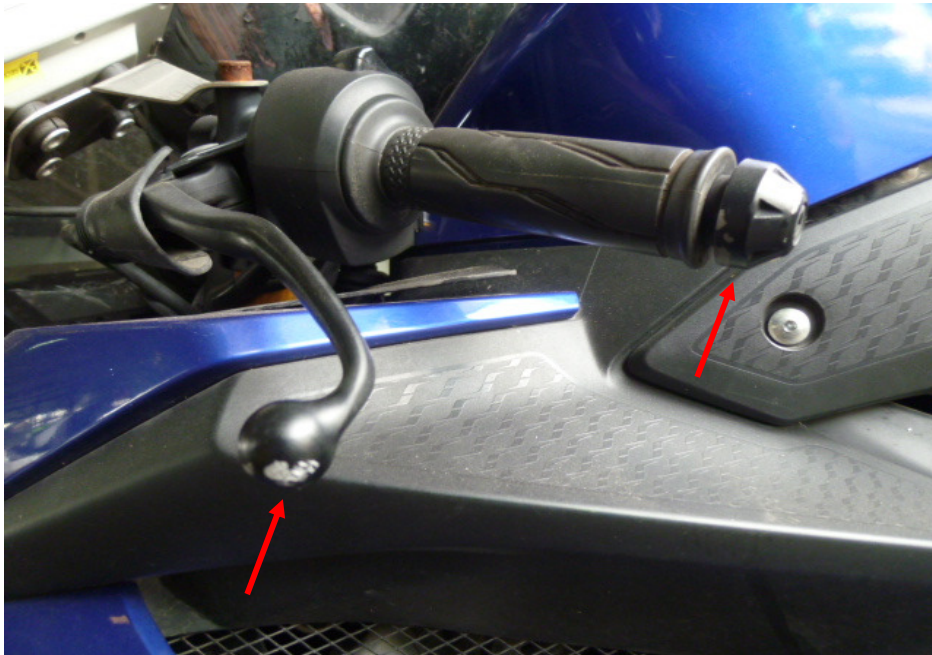
Photo 8 shows a closer view of the grazed left handlebar and bent clutch lever of the Motorcycle as a result of the accident (arrowed).
