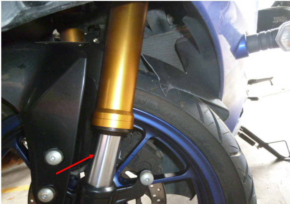
Photo 21 shows a closer view of the bent left front fork of the Motorcycle as a result of the accident (arrowed). Hence we were not able to conduct any test(s) on the steering system of the Motorcycle
