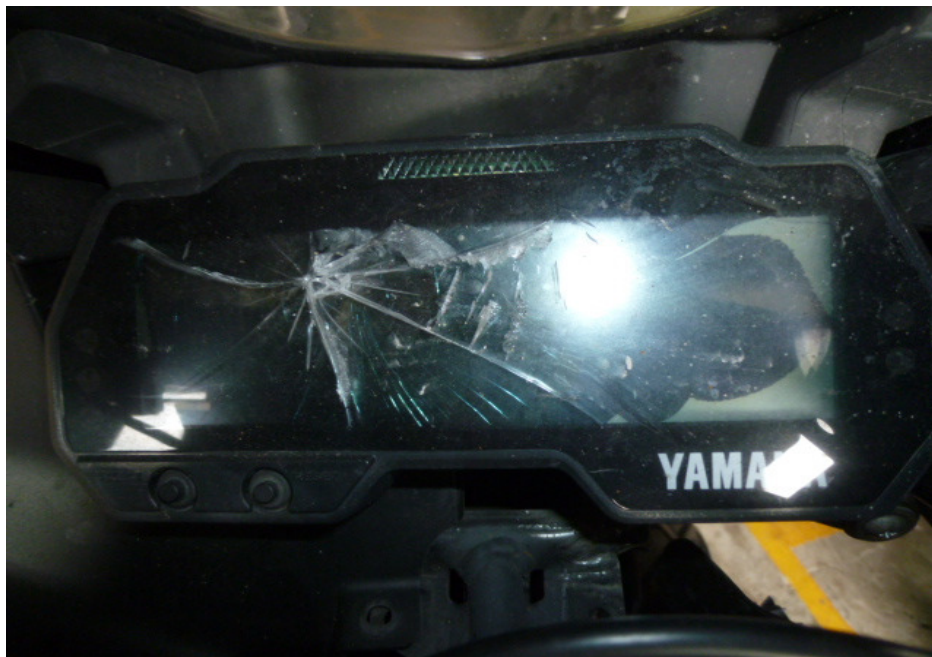
Photo 1 shows the damaged speedometer gauge of the Motorcycle as a result of the accident. Hence, we were unable to record the mileage of the Motorcycle at the time of our inspection.
