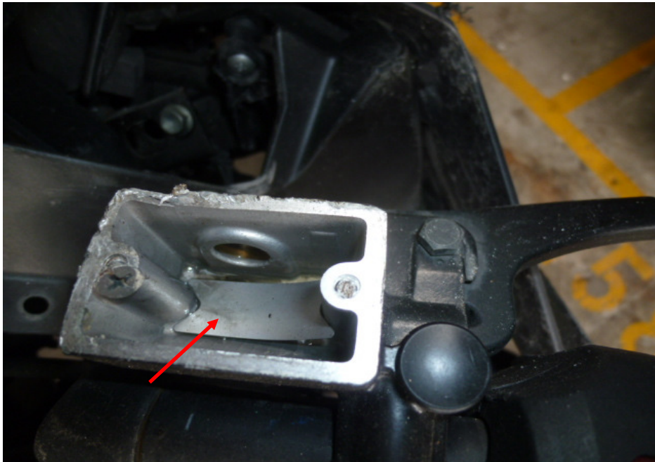
Photo 23 shows the front brake reservoir of the Motorcycle. The front brake reservoir cover was missing as a result of the accident. The front brake reservoir was also found to be empty (arrowed).
