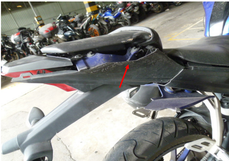
Photo 11 shows the cracked right rear side cover of the Motorcycle as a result of the accident (arrowed).
