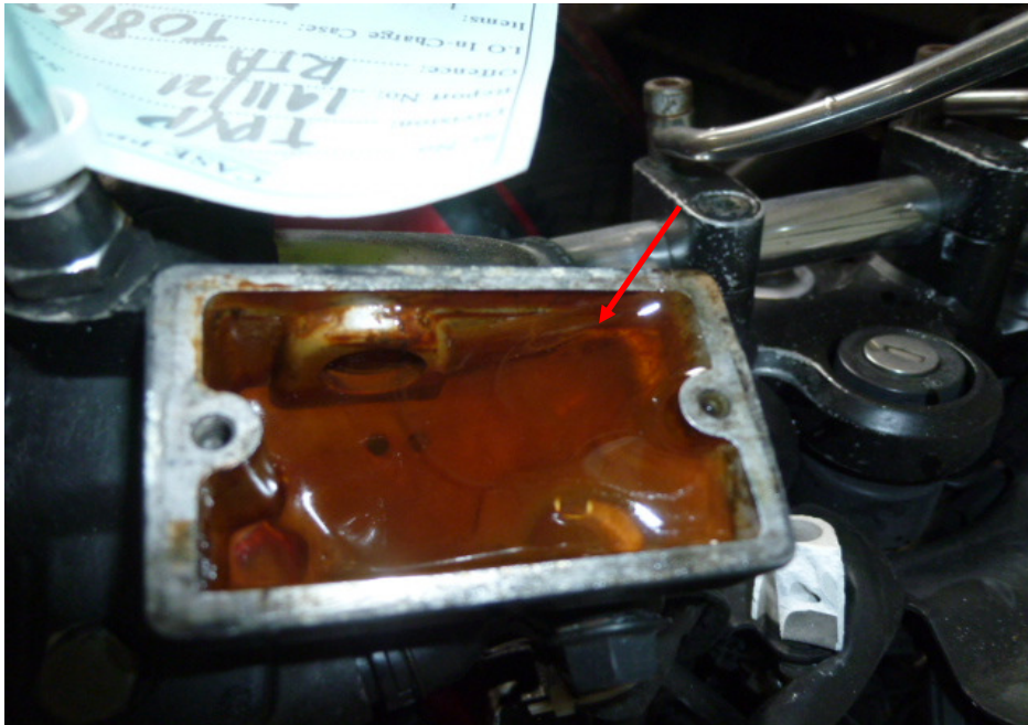
Photo 25 shows the brake fluid reservoir for the front brake of the Motorcycle. The brake fluid was found to be of sufficient level for operating purposes. However the brake fluid was found to be slightly contaminated (arrowed).
