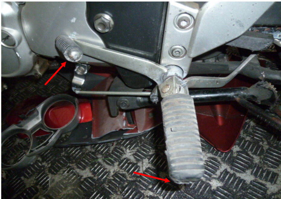
Photo 14 shows a closer view of the gear shift pedal and left front footrest which were amongst the body parts of the Motorcycle that had sustained damage as a result of the accident (arrowed).
