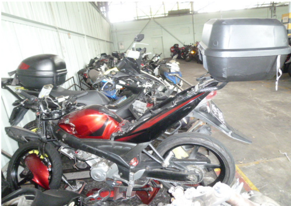
Photo 4 shows a general view of the left body of the Motorcycle at the time of our inspection. The Motorcycle had sustained damages all around. Body parts that were found to have been damaged include its headlight assembly, speedometer gauge, front fork assembly, front mudguard, right front signal lamp, right handlebar end, right side mirror, front brake lever, petrol tank, radiator, left rear side cover, rear brake pedal, gear shift pedal, left front footrest, top box and rear mudguard, amongst others.
