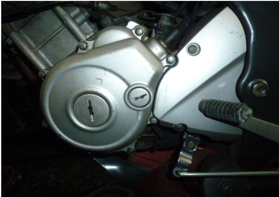
Photo 19 shows the left side of the engine of the Motorcycle at the time of our inspection. The various engine related parts and components were found to be intact with no visible damage. There was also no sign(s) or indication(s) of fluid leak observed around the left engine area of the Motorcycle.
