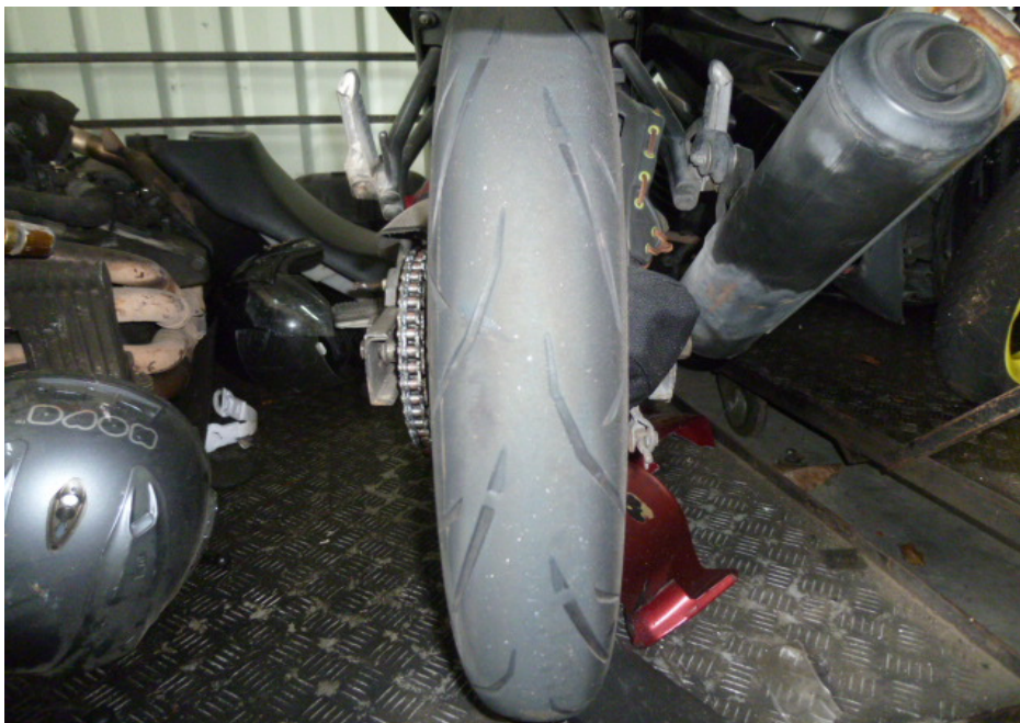
Photo 18 shows the condition of the Motorcycle's rear tyre. The pattern of the tread was clearly visible with remaining tread depth of approximately 3mm. We did not observe any tear, burst mark(s) and/or punctured hole(s) on the sidewalls as well as across the tread of the rear tyre.
