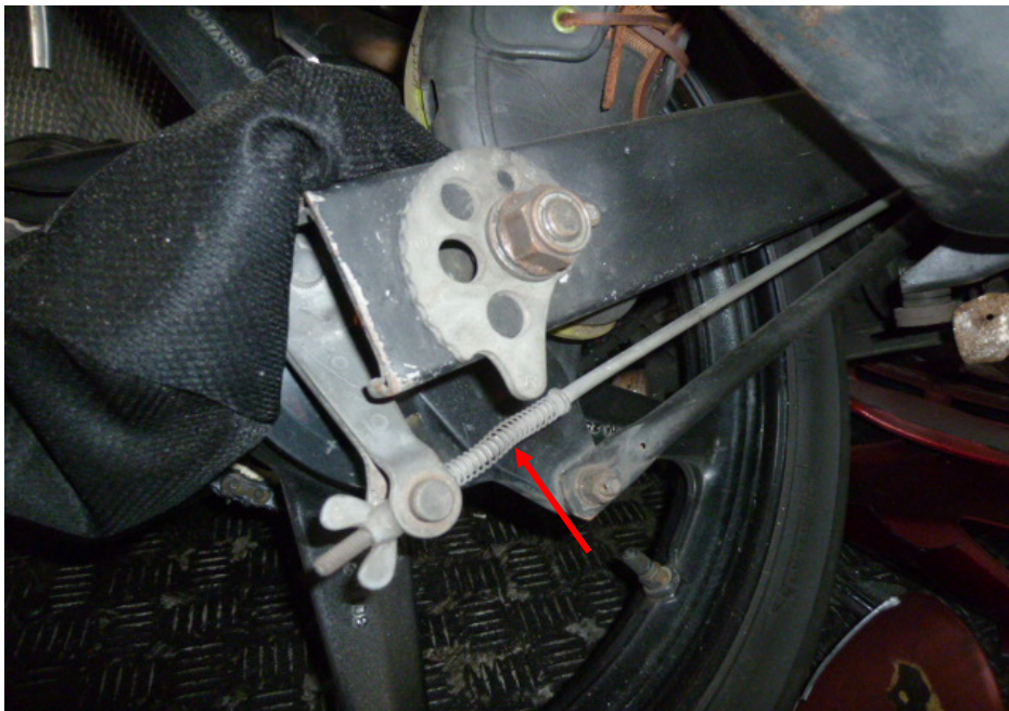
Photo 27 shows the rear wheel of the Motorcycle. The type of brake system for the rear wheel was of a mechanical type, controlled by the brake foot pedal of the Motorcycle. Our checks of the cable (arrowed), spring and drum which are all part of the components in the rear brake system of the Motorcycle reveal all to be intact and without damage.
