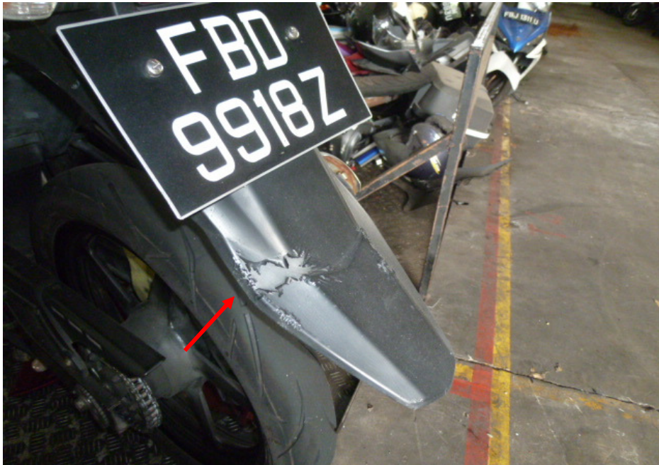
Photo 13 shows a closer view of the deformed rear mudguard of the Motorcycle as a result of the accident (arrowed).
