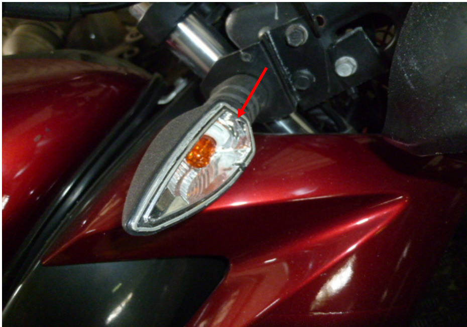
Photo 10 shows a closer view of the cracked right front signal lamp which was amongst the body parts of the Motorcycle that had sustained damage as a result of the accident (arrowed).
