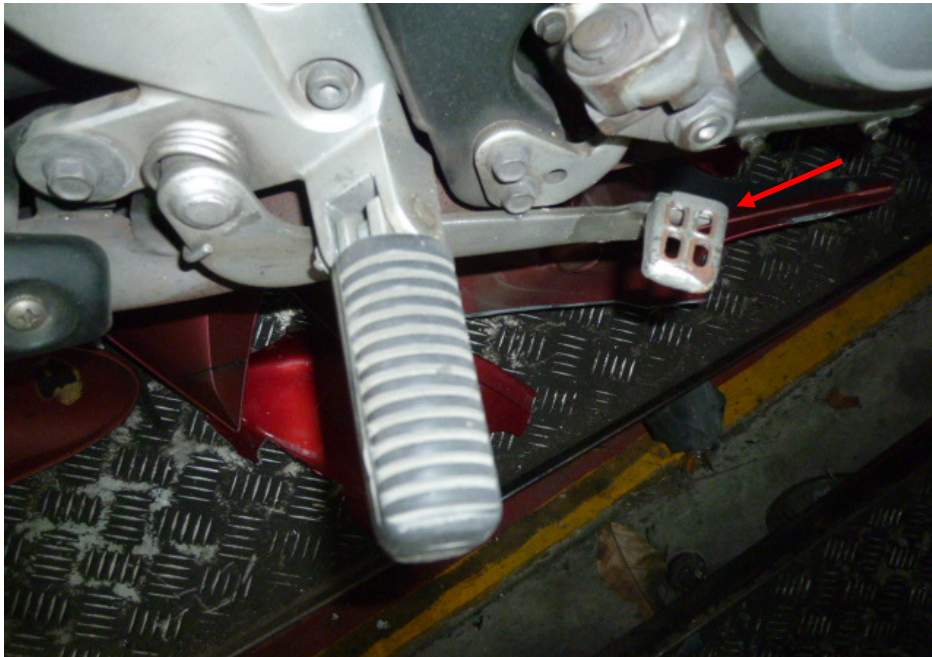
Photo 12 shows a closer view of the bent rear brake pedal of the Motorcycle that as a result of the accident (arrowed).
