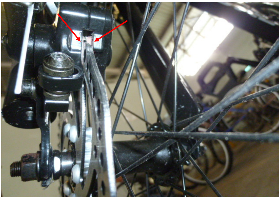
Photo 21 shows a close up view of the front brake pads responding to the gripping action. The front brake pads pressed against the front brake disc (arrowed) upon depressing the right hand brake lever. This had appeared to indicate that the front brake of the Bicycle was in serviceable condition.
