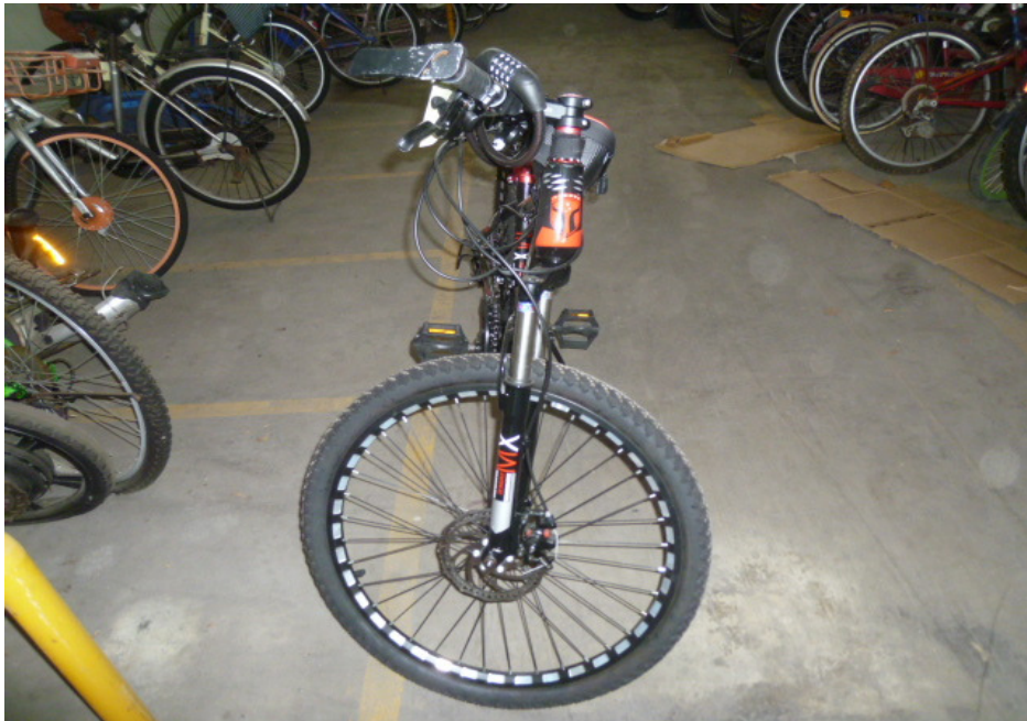
Photo 18 shows the front wheel of the Bicycle turned towards its full right. Turning the Bicycle's handle bar towards the right did not produce any abnormal free play and/or resistance. This would indicate that the steering system of the Bicycle was in serviceable condition at the time of our inspection.
