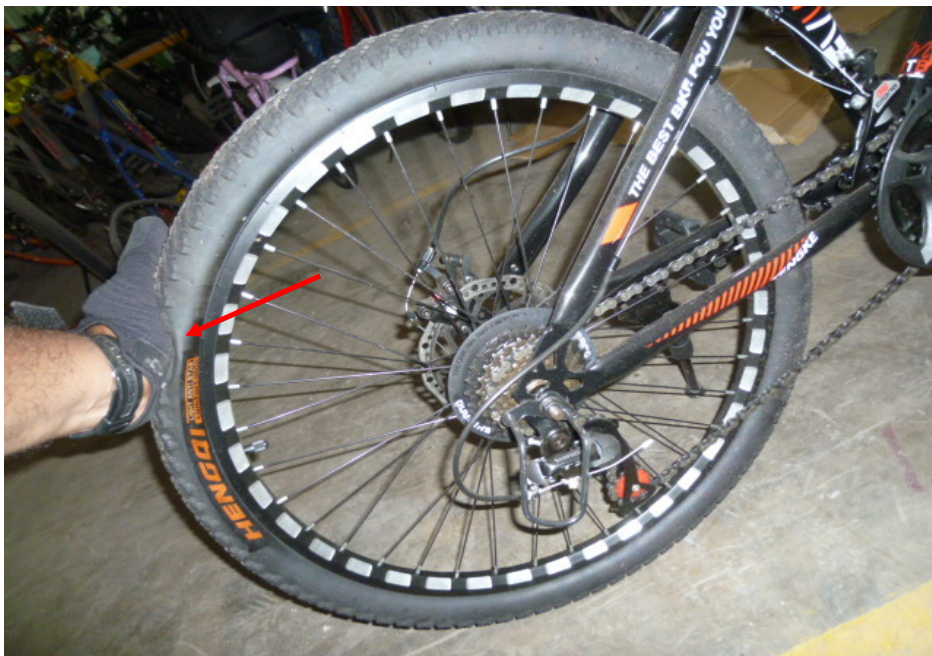
Photo 14 shows the deflated rear tyre of the Bicycle (arrowed).
