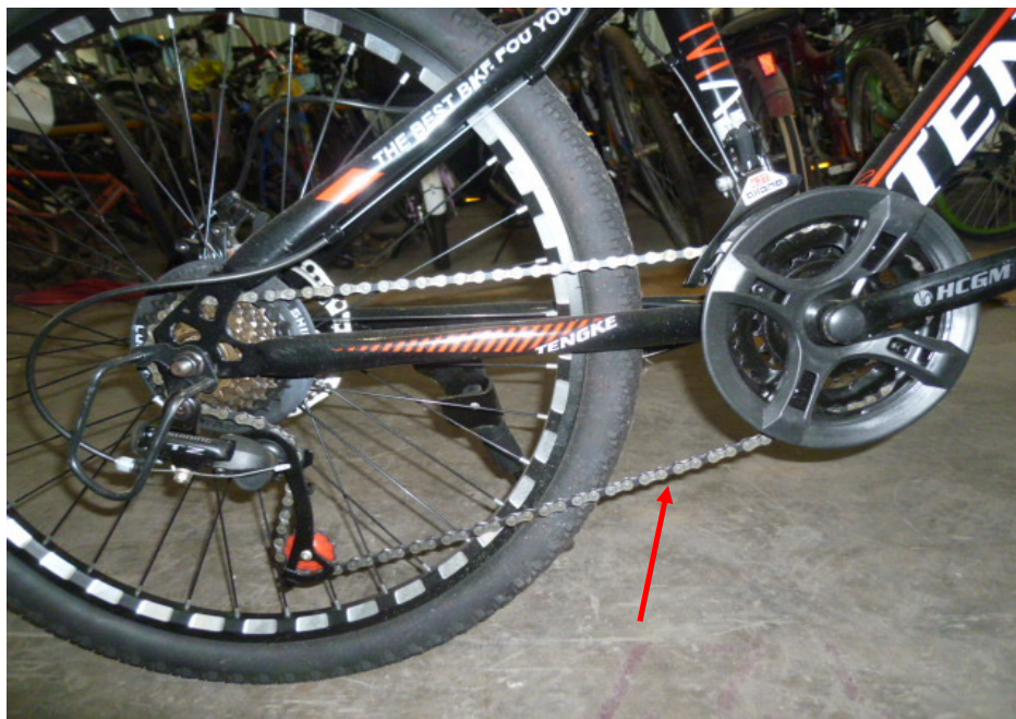
Photo 15 shows the general view of the gear train of the Bicycle, which was observed to be intact with no misalignment (arrowed). It was also adequately lubricated for operating purposes.
