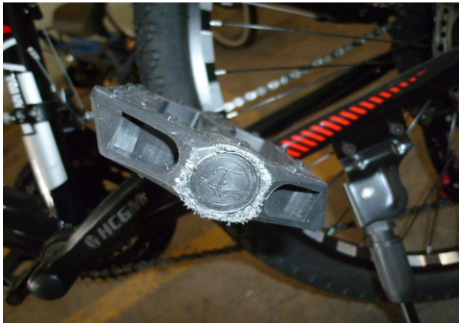
Photo 8 shows the damages of grazing nature on the left pedal of the Bicycle at the time of our inspection.
