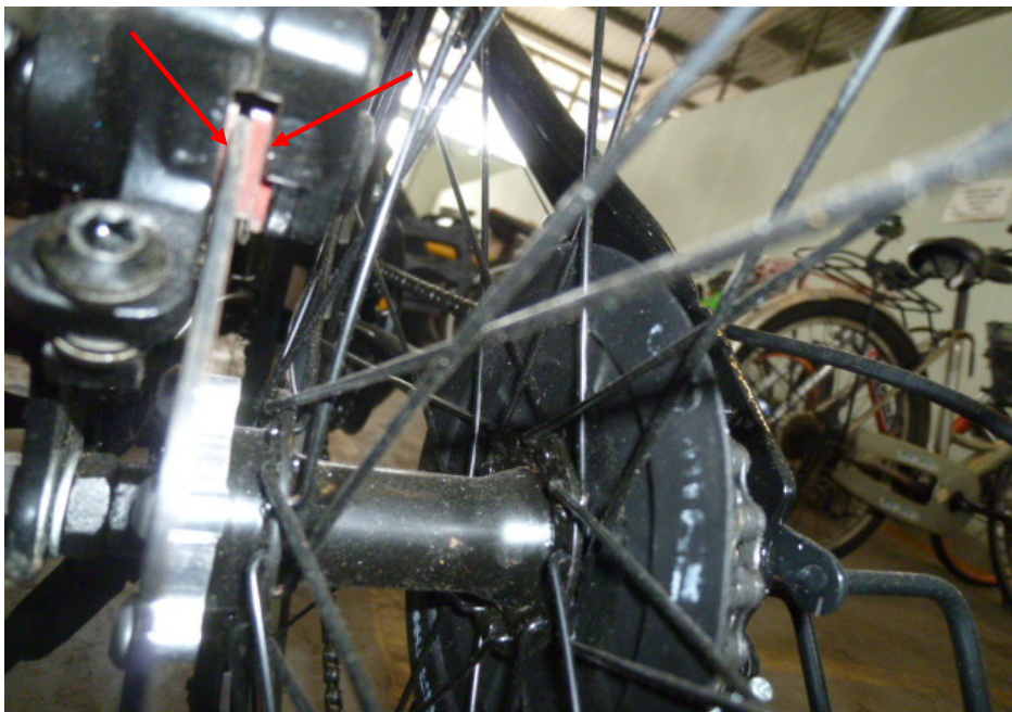
Photo 23 shows a close up view of the rear brake pads responding to the gripping action. The rear brake pads pressed against the rear brake disc (arrowed) upon depressing the left hand brake lever. This had appeared to indicate that the rear brake of the Bicycle was in serviceable condition.
