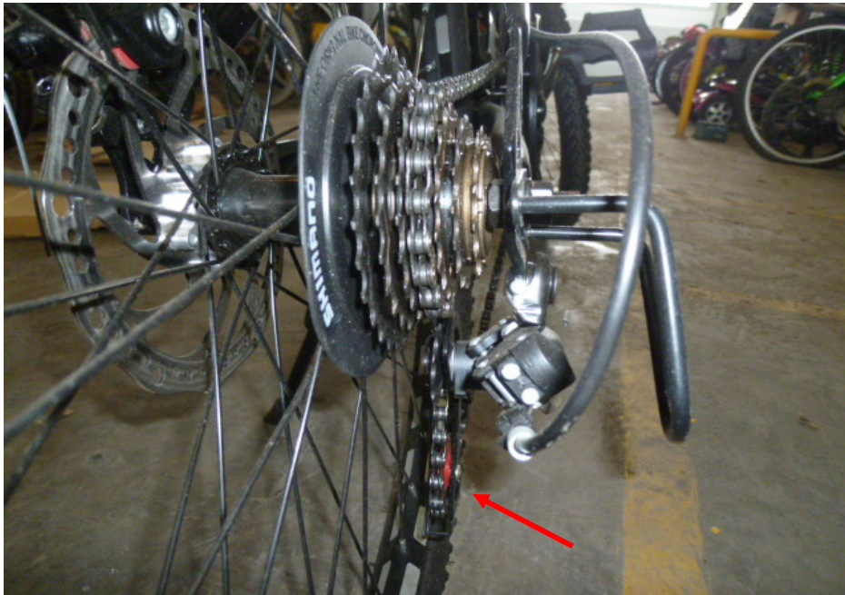
Photo 16 shows a closer view of the gear train of the Bicycle, which was observed to be intact with no misalignment (arrowed). It was also adequately lubricated for operating purposes.
