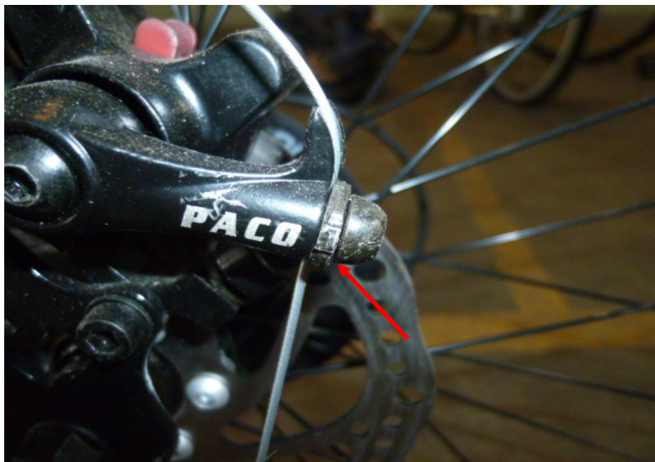
Photo 9 shows the damages of grazing nature on the rear brake caliper nut of the Bicycle at the time of our inspection (arrowed).
