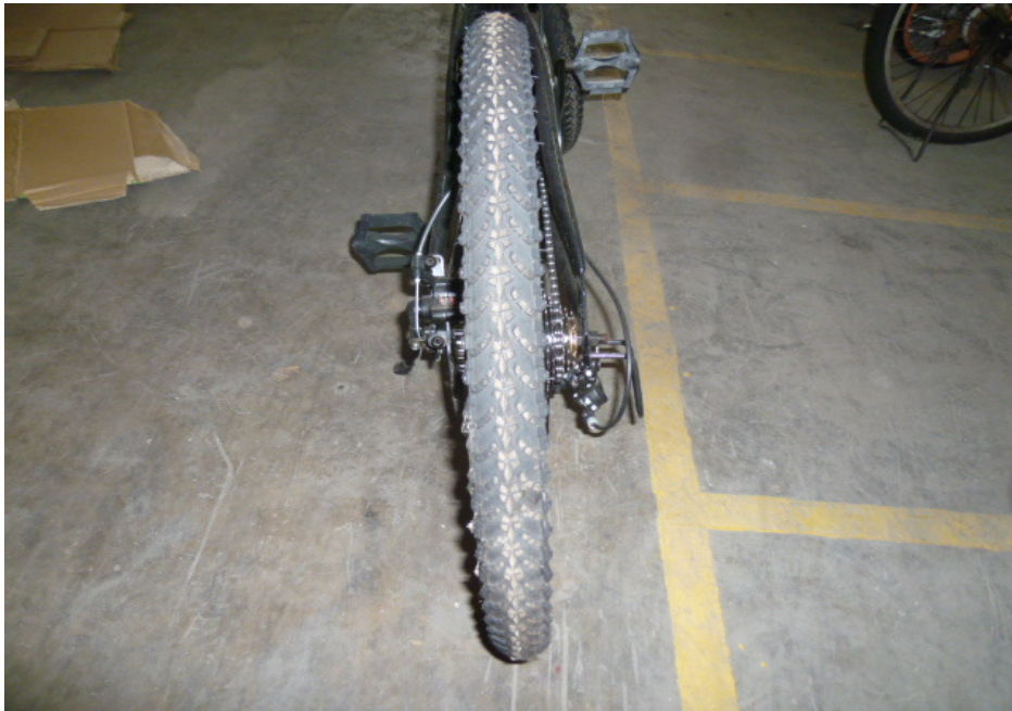
Photo 13 shows the rear tyre of the Bicycle. The pattern of the tread was clearly visible. There was no tear, burst mark(s) and/or punctured hole(s) on the sidewalls as well as across the tread of the front tyre. However the rear tyre was observed to be deflated.
