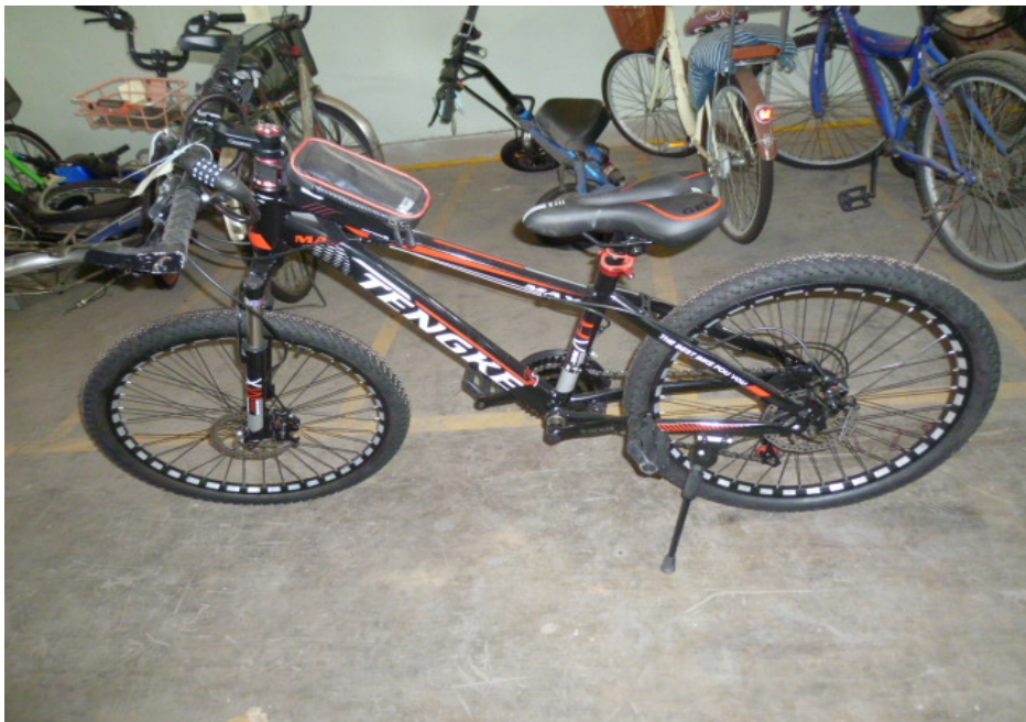
Photo 4 shows the left body of the Bicycle at time of our inspection. The Bicycle had sustained damages at its left body. The body parts that were found to have been damaged include its left hand brake lever guard, left fork stem, left pedal, seat and rear brake caliper nut, amongst others as a result of the accident.
