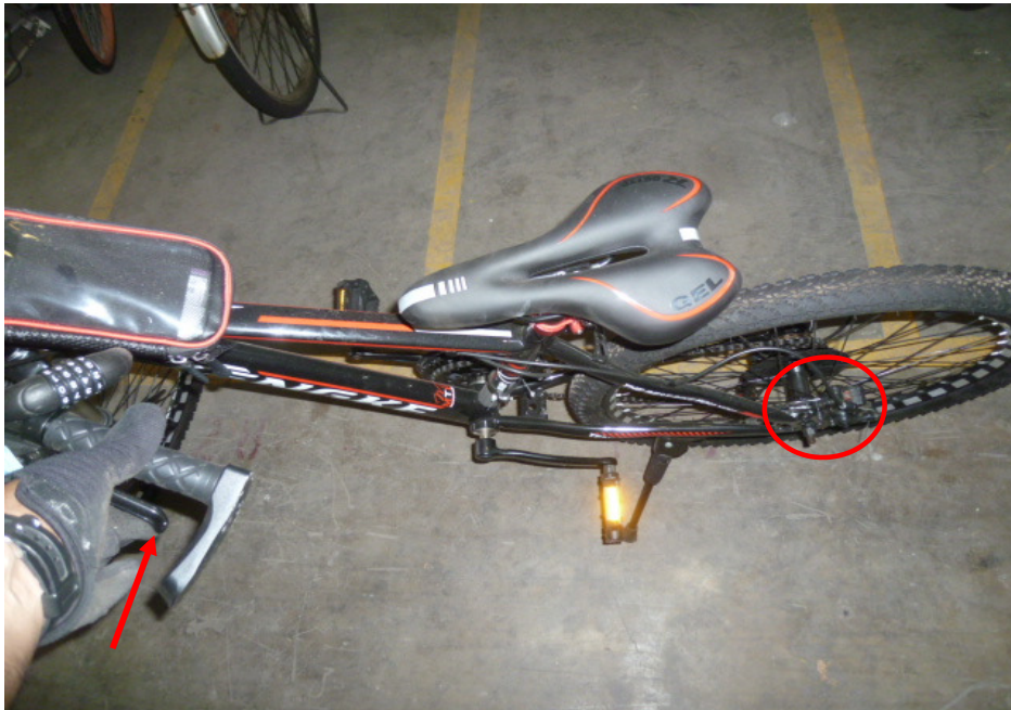
Photo 22 shows a static brake test conducted on the Bicycle's rear brake. There was some resistance felt upon pressing the left hand brake lever (arrowed). It also shows that the rear brake pads responded to the gripping action (circled) after depressing the left hand brake lever.
