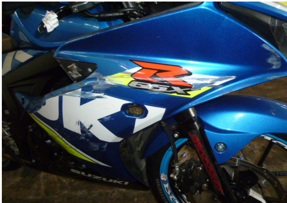
Photo 7 shows a closer view of the right cowling which was amongst the body parts of the Motorcycle that had sustained damage as a result of the accident.
