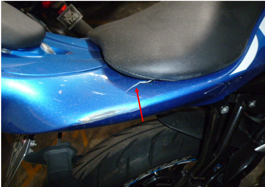
Photo 10 shows a closer view of the cracked right rear side cover of the Motorcycle as a result of the accident (arrowed).
