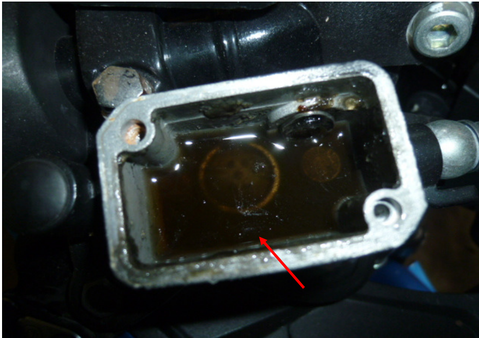
Photo 24 shows the brake fluid reservoir for the front brake of the Motorcycle. The brake fluid was found to be of sufficient level for operating purposes. However the brake fluid was observed to be slightly contaminated (arrowed).
