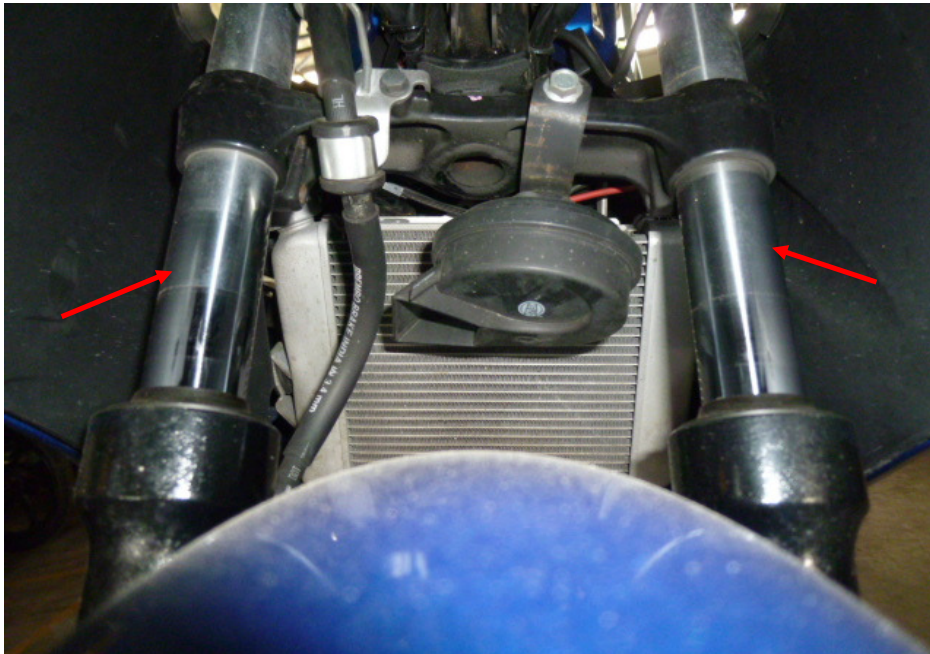
Photo 20 shows the front fork (arrowed) of the Motorcycle. The front fork and fork bracket of the Motorcycle were both found to be intact and undamaged. Turning the Motorcycle's handle bar towards the left and right did not produce any abnormal free play. The steering system of the Motorcycle was in serviceable condition at the time of our inspection.
