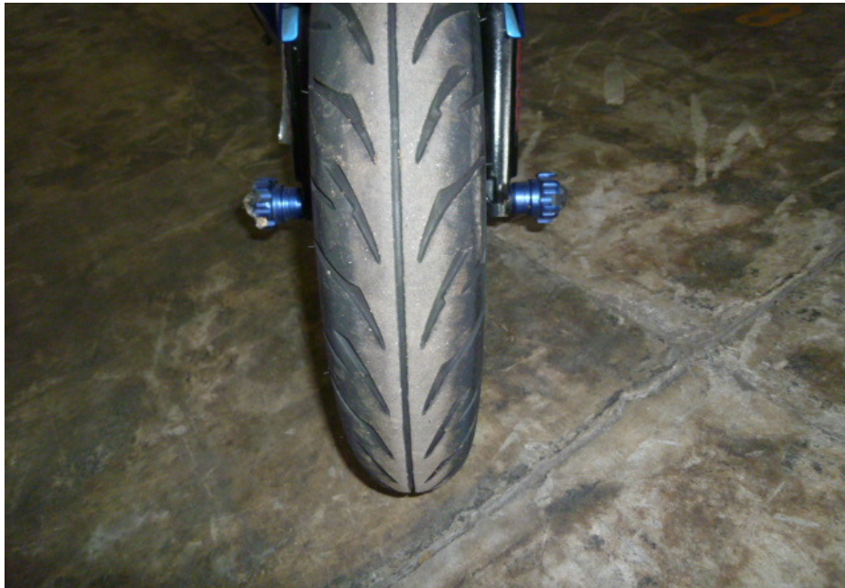
Photo 14 shows the front tyre of the Motorcycle at the time of our inspection. The front tyre was observed to be in serviceable condition with remaining tread depth of approximately 3mm. The pattern of the tread was also clearly visible. There was no tear, burst mark(s) and/or punctured hole(s) on the sidewalls as well as across the tread of the front tyre.
