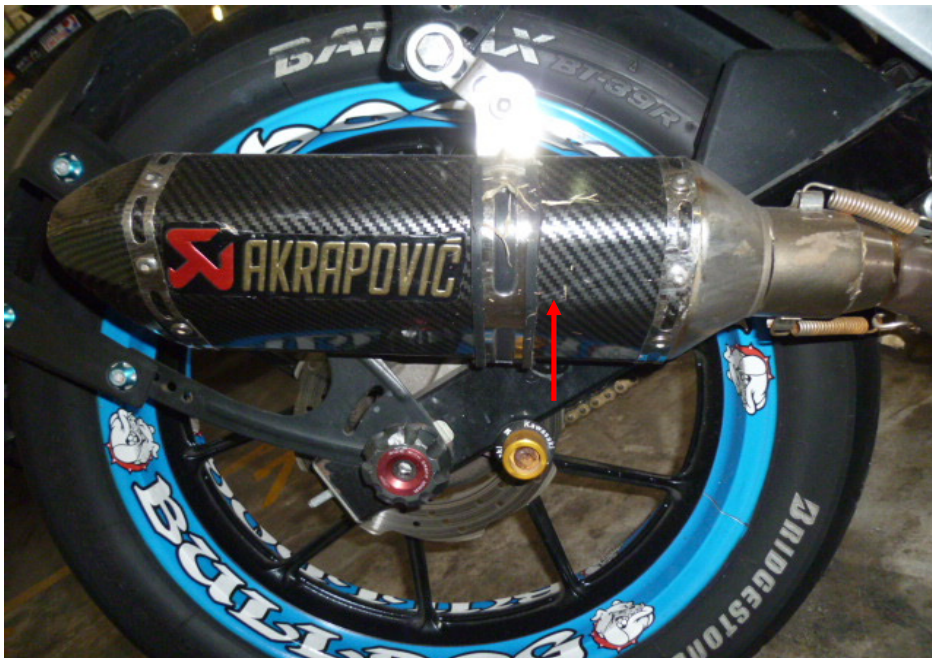
Photo 13 shows the grazed exhaust muffler of the Motorcycle as a result of the accident (arrowed).
