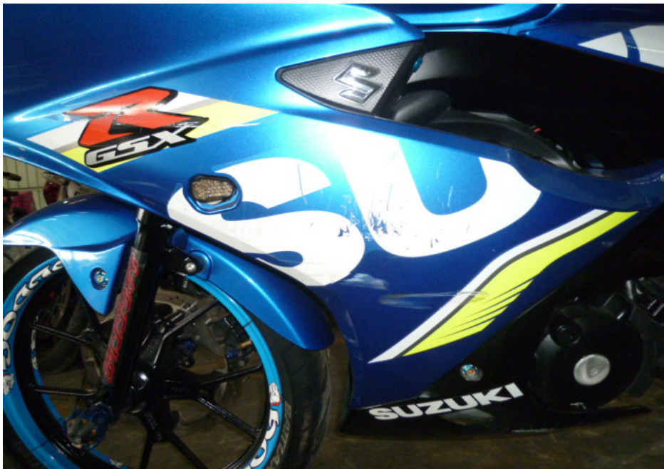
Photo 11 shows a closer view of the left cowling which was amongst the body parts of the Motorcycle that had sustained damages of grazing nature as a result of the accident.
