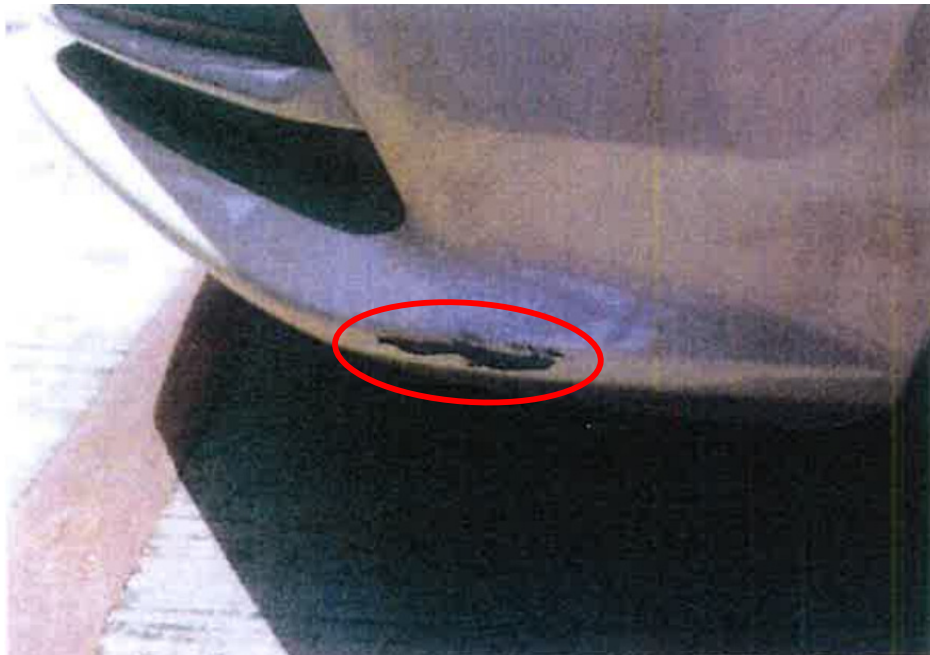
Photo 6 shows the damage to left side lower area of PMC's front bumper. Black coloured marks that appear to be of grazing nature (circled) were seen on the left lower corner of the front bumper. Refer to photograph 7 below for a general view of PMC showing its left side front profile.
