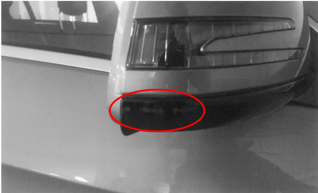
Photo 12 shows a close up view of DMC's right wing mirror (photograph taken on 01 October 2018 or thereabouts). Scratch/grazed marks (circled) were observed on the outer cover at the side surface area of the right wing mirror (refer to photograph 13 below for a general view of DMC showing its side profile). Note that the right wing mirror was seen to be shifted inwards in the photographs that were taken at the incident location. Refer to yellow arrow in photograph 8 above.
