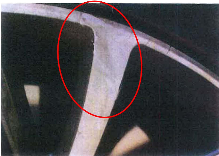
Photo 3 shows a close up view of the damage to the front left wheel rim of PMC. What appear to be black coloured marks were seen on the outer spoke of the front left wheel rim (circled).
