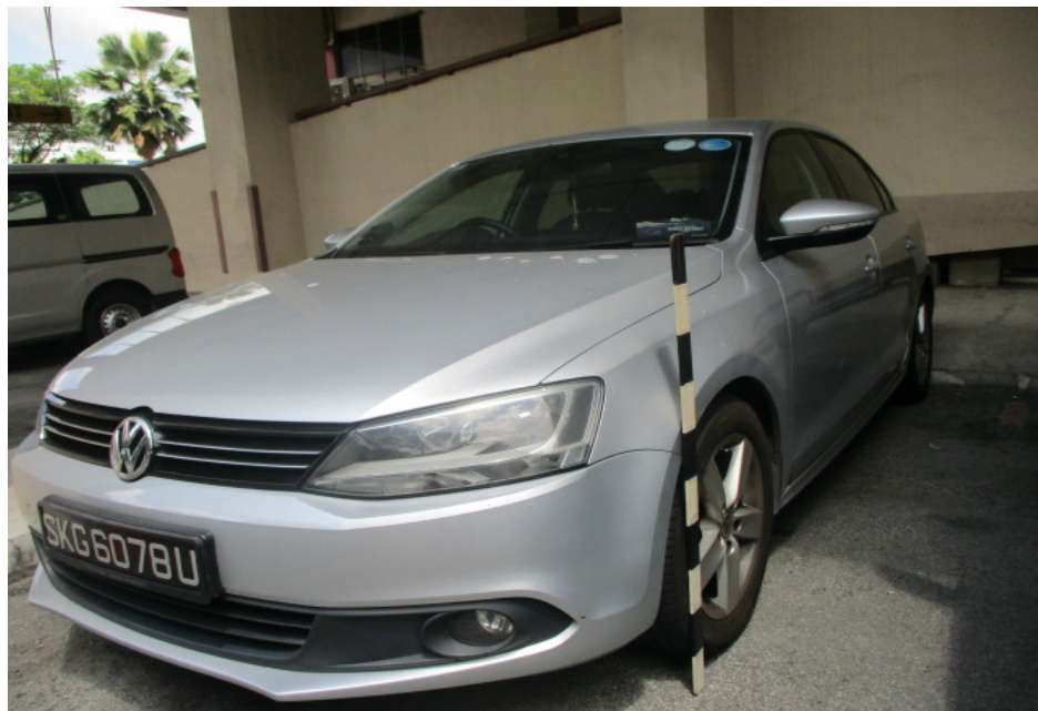
Photo 17 shows height measurement being carried out to a similar make and model vehicle as PMC, in particular to the height above ground level of the damage at the front left headlamp, front left fender and left wing mirror of PMC.
