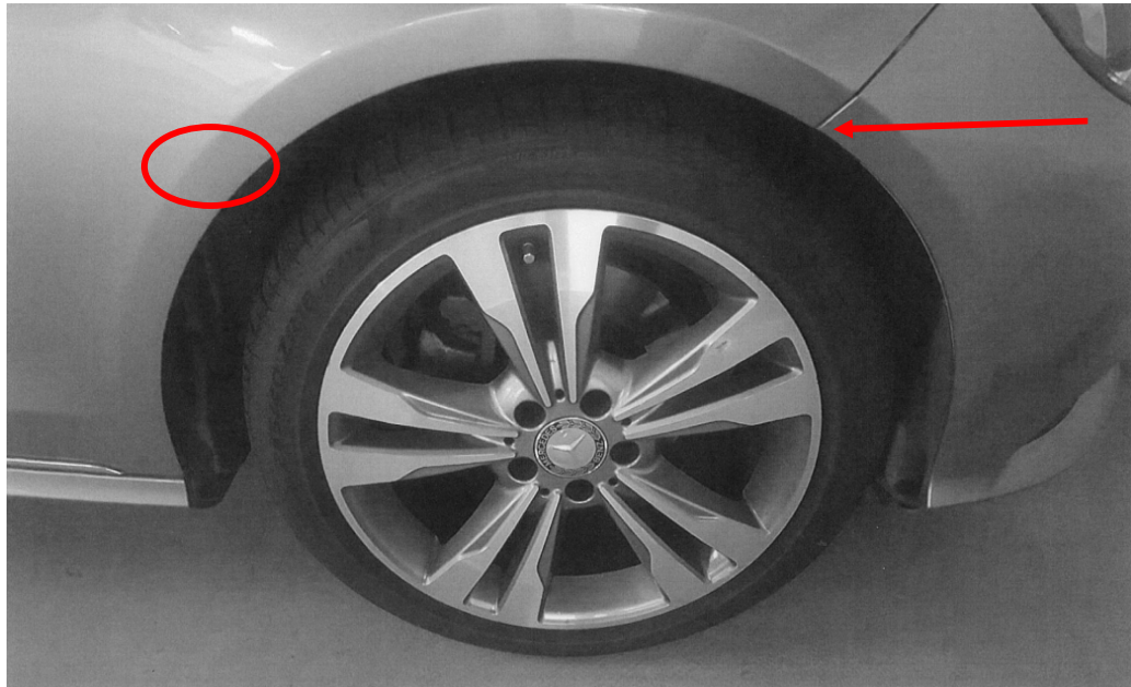
Photo 10 shows a general view of the front right wheel rim and front right fender of DMC (photograph taken on 01 October 2018 or thereabouts). The grazed marks on the front right fender of DMC that were seen in the set of photographs taken at the incident location (refer to red circle in photograph 8 above) were not seen on the same area of the front right fender (circled). This area was determined by taking reference from the edge of DMC's front bumper as highlighted by the red arrow (refer to the set of photographs taken at the incident location that were contained in PAEIC).
