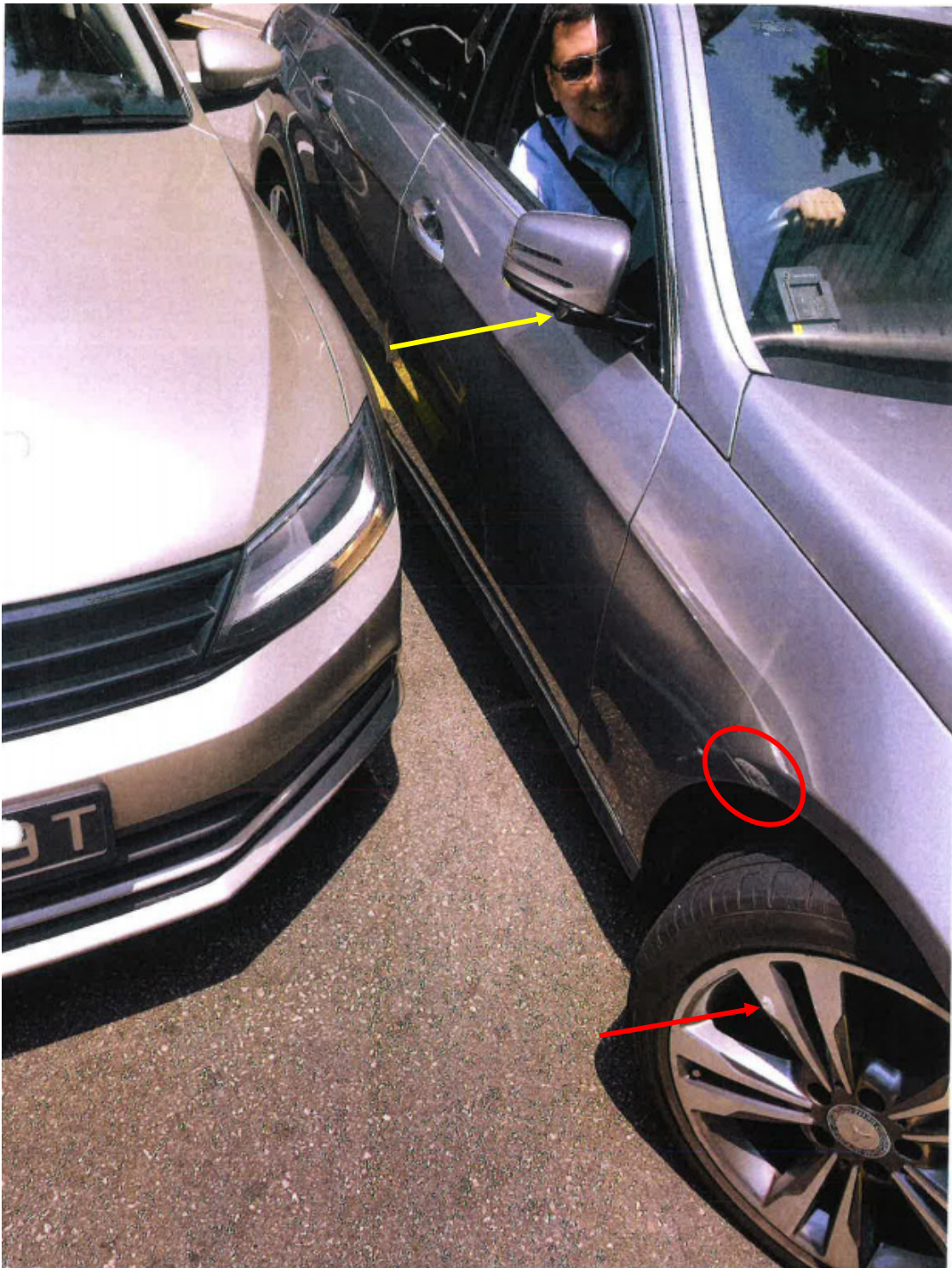
Photo 8 shows DMC at the incident location. Basing on the photographs contained in DAEIC, it was observed that the front right wheel rim of DMC had sustained scratches on its outer spoke (red arrow). What appears to be marks of grazing nature was also observed on the front right fender (red circle). DMC's right wing mirror was further seen to be shifted inwards (yellow arrow). Note that these damages were along the side body of DMC.
