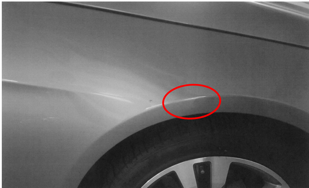
Photo 11 shows the distortion (circled) on the front right fender of DMC that I had observed from the set of photographs that were taken on 01 October 2018 or thereabouts. The distorted area was noted to be near the grazed marks that were seen on the front right fender of DMC at the incident location (refer to red circle in photograph 8 above).
