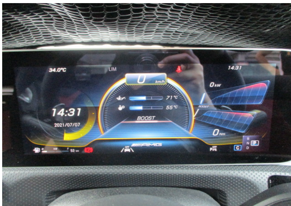
Photo 15 shows the respective warning lights no longer illuminated, indicating that there is no fault detected to the ABS, SRS, EPS, TPM and TCS systems of the Motor Car during the self-test. These electronic systems were hence in working condition at the time of my inspection.
