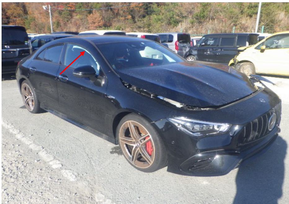
Photo 3 shows the front right body of the Motor Car (photograph provided to me). Apart for the front left portion, there was no physical damage seen to other areas of the Motor Car. I had however observed that the right curtain airbag (arrowed) was activated.
