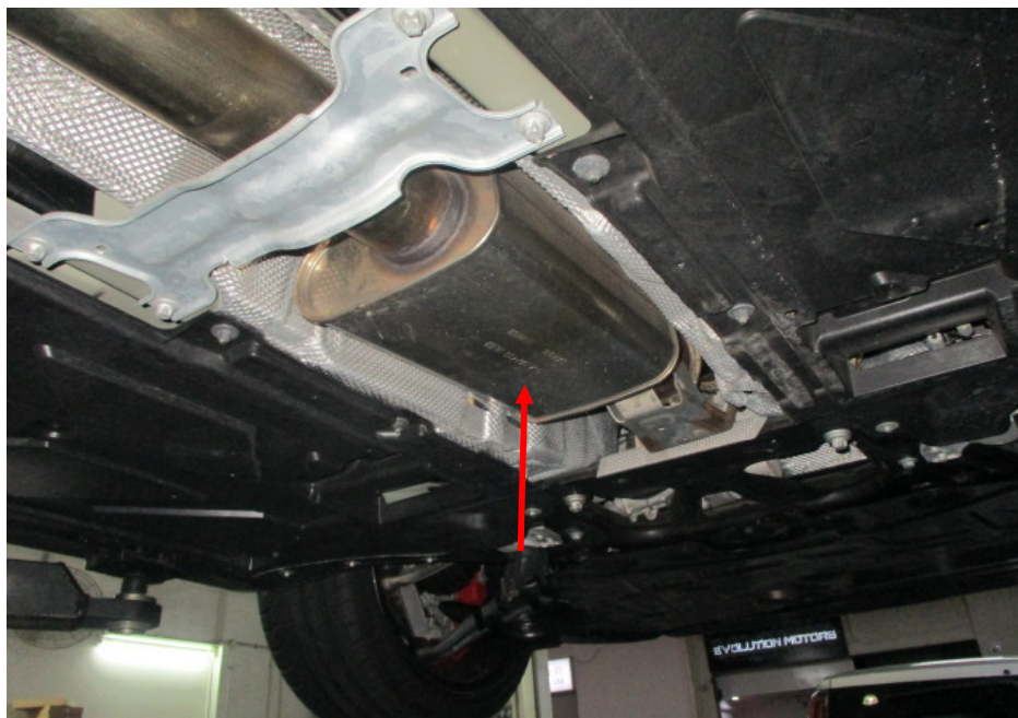
Photo 20 shows the front section of the Motor Car's exhaust system. My examination of the Motor Car's exhaust system revealed no sign(s) or indication(s) of any cut or weld marks along its exhaust pipes, on its catalytic converter, centre resonator box (arrowed) and on its rear muffler.
