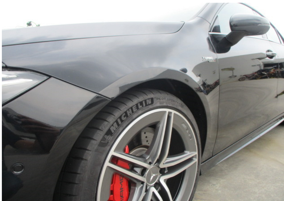
Photo 7 shows a closer view of the front bumper and front left fender of the Motor Car. The body parts at the front left portion of the Motor Car were visually examined and it was observed that the repair/restoration works carried out to the damaged area of the Motor Car (refer to photograph 1 & 2 above) were reasonably adequate and in order.
