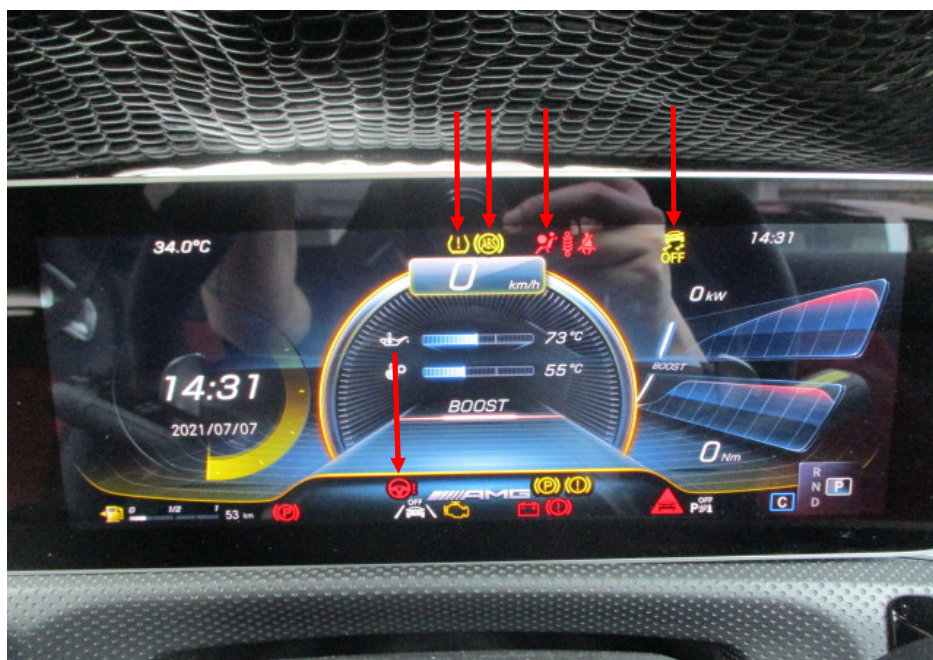
Photo 14 shows the warning lights for the various electronic safety features appearing on the instrument panel of the Motor Car during its self-test when the engine is cranked, in particular the ABS, SRS, EPS, TPM and TCS lights (arrowed).
