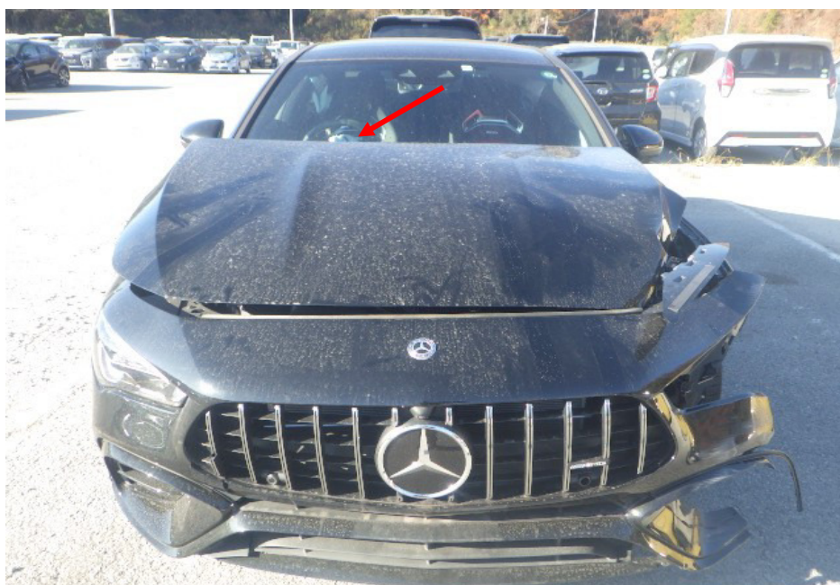
Photo 2 shows the frontal body of the Motor Car (photograph provided to me). The Motor Car was observed to have sustained damages at its front left portion. Body parts damaged include the front bumper, front bumper centre lower grille, front left headlamp and front bonnet amongst others. The driver's airbag (arrowed) was observed to be deployed.
