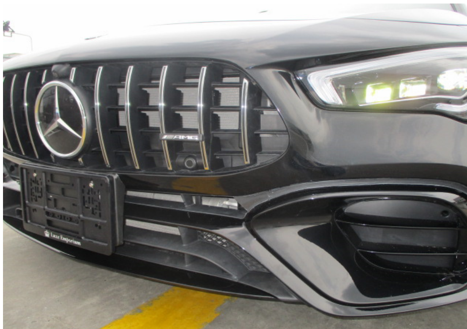
Photo 6 shows a closer view of the front bumper, front bumper centre lower grille, front bumper left lower grille and front left headlamp of the Motor Car. The body parts at the front left portion of the Motor Car were visually examined and it was observed that the repair/restoration works carried out to the damaged area of the Motor Car (refer to photograph 1 & 2 above) were reasonably adequate and in order.
