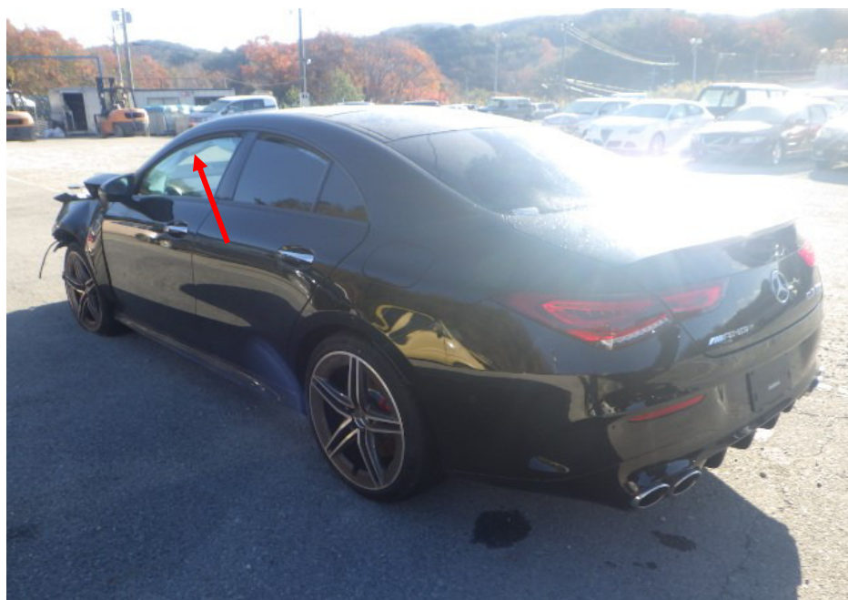
Photo 4 shows the rear left body of the Motor Car (photograph provided to me). Apart for the front left portion, there was no physical damage seen to other areas of the Motor Car. I had however observed that the left curtain airbag (arrowed) was activated.
