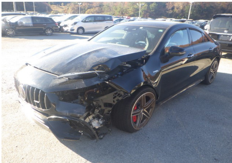
Photo 1 shows the front left body of the Motor Car (photograph provided to me). The Motor Car was observed to have sustained damages at its front left portion. Body parts damaged include the front bumper, front bumper left bracket, front bumper left lower grille, front left headlamp, front left fender and front left fender inner shield amongst others.
