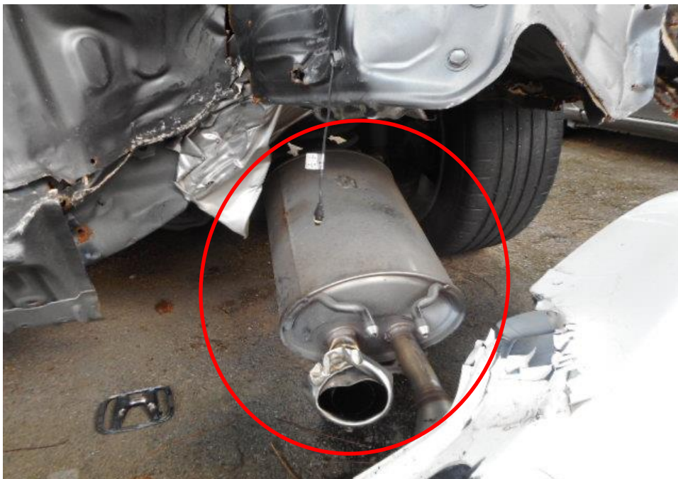
Photo 7 shows a close up view of the Motor Car's rear body at the time of my inspection. The rear portion of the Motor Car was observed to have sustained damage. Its rear exhaust pipe (circled) was the body parts that were damaged as a result of the accident
