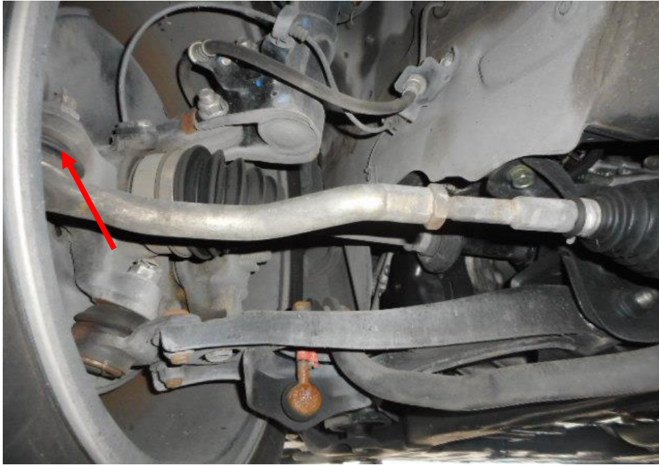
Photo 26 shows the various undercarriage components at the front left wheel of the Motor Car, which had included the steering tie rod (red arrow). The various undercarriage components of the Motor Car were all found to be intact without any visible damage.
