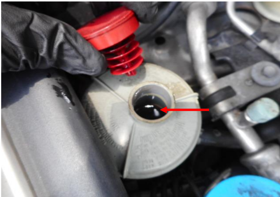
Photo 16 shows the power steering fluid reservoir of the Motor Car at the time of my inspection. The steering fluid was observed to be of sufficient level (arrowed) and without any visible contamination.
