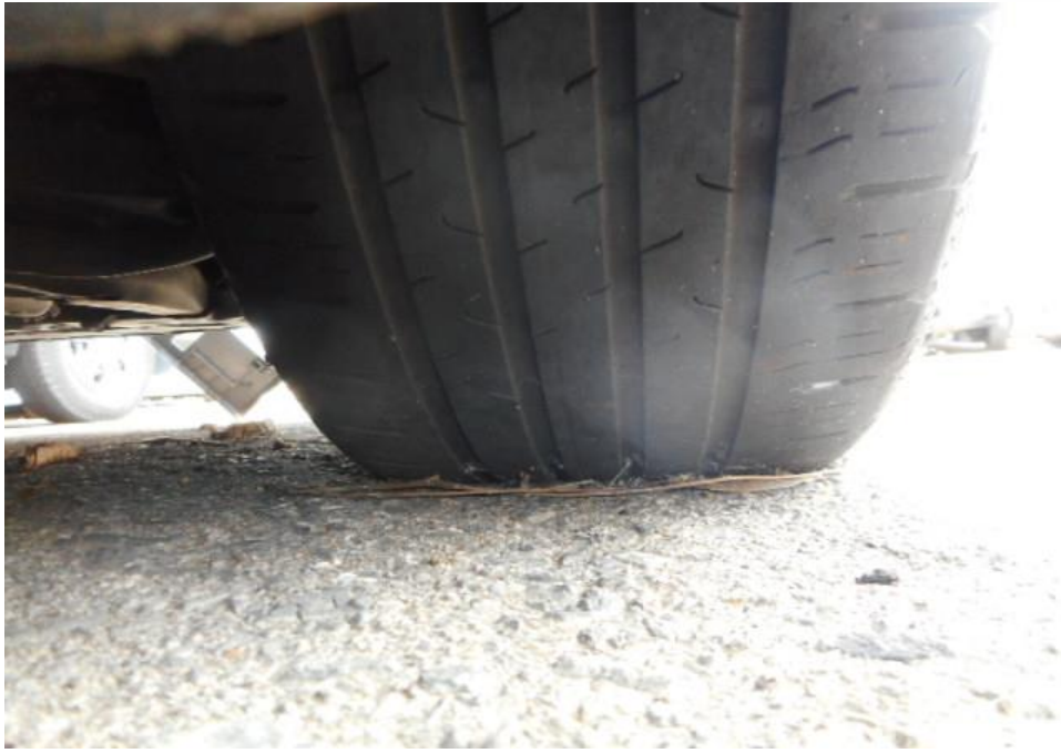
Photo 10 shows the condition of the front right tyre of the Motor Car, which was observed to be in serviceable condition with remaining tread depth of approximately 3.4mm. The tyre was sufficiently inflated for vehicular operation with no tear, cut or burst mark(s) on the outer and the inner sidewalls as well as across the tread. The 4 tyres of the Motor Car were wrapped around standard steel wheel rims without any damage.
