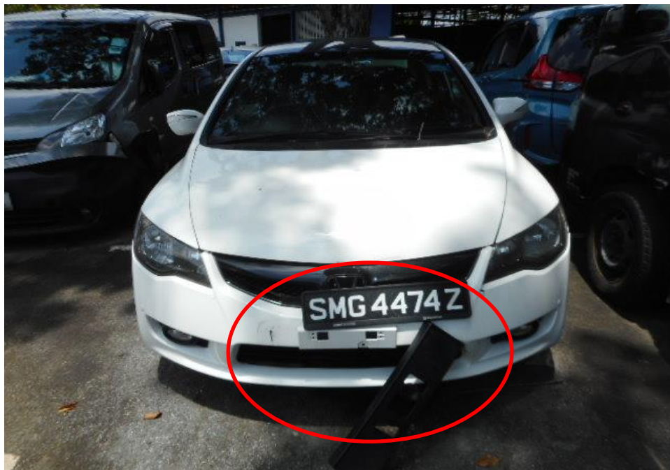
Photo 3 shows a close up view of the Motor Car's front body at the time of my inspection. The front portion of the Motor Car was observed to have sustained damage. Its front bumper and front number plate (circled) was the body parts that were damaged as a result of the accident.
