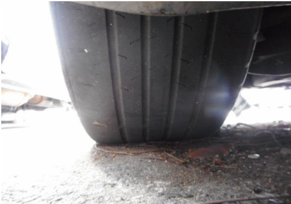
Photo 13 shows the condition of the front left tyre of the Motor Car, which was observed to be in serviceable condition with remaining tread depth of approximately 2.5mm. There was also no tear, cut or burst mark(s) on the outer and the inner sidewalls as well as across the tread of the Motor Car's 4 tyres.
