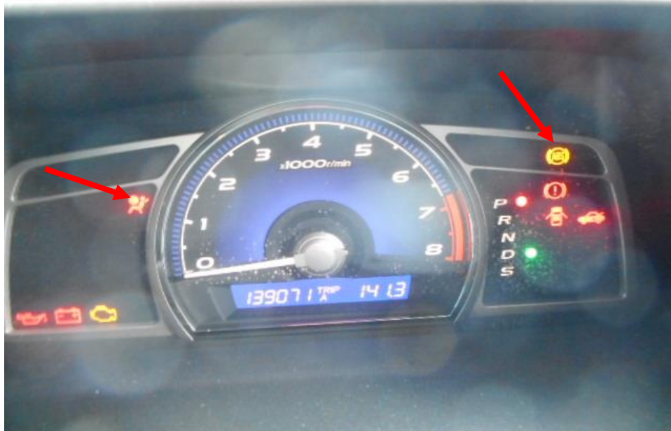
Photo 27 shows the warning light for Anti-Lock Brake System (ABS), and Supplemental Restraint System (SRS) (arrowed) appearing on the instrument panel of the Motor Car during the self-test of its various electronic operating systems when its engine was cranked.
