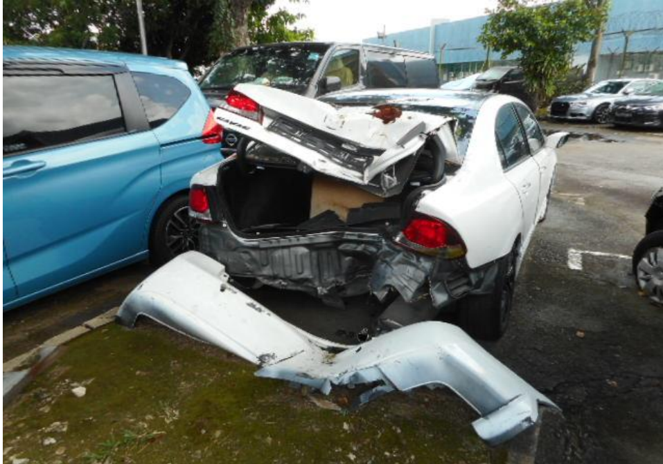
Photo 4 shows a general view of the Motor Car's front body at the time of my inspection. The front and rear portion. Its front bumper, front number plate, rear bonnet, rear bumper and rear exhaust pipe was the body parts that were damaged as a result of the accident.
