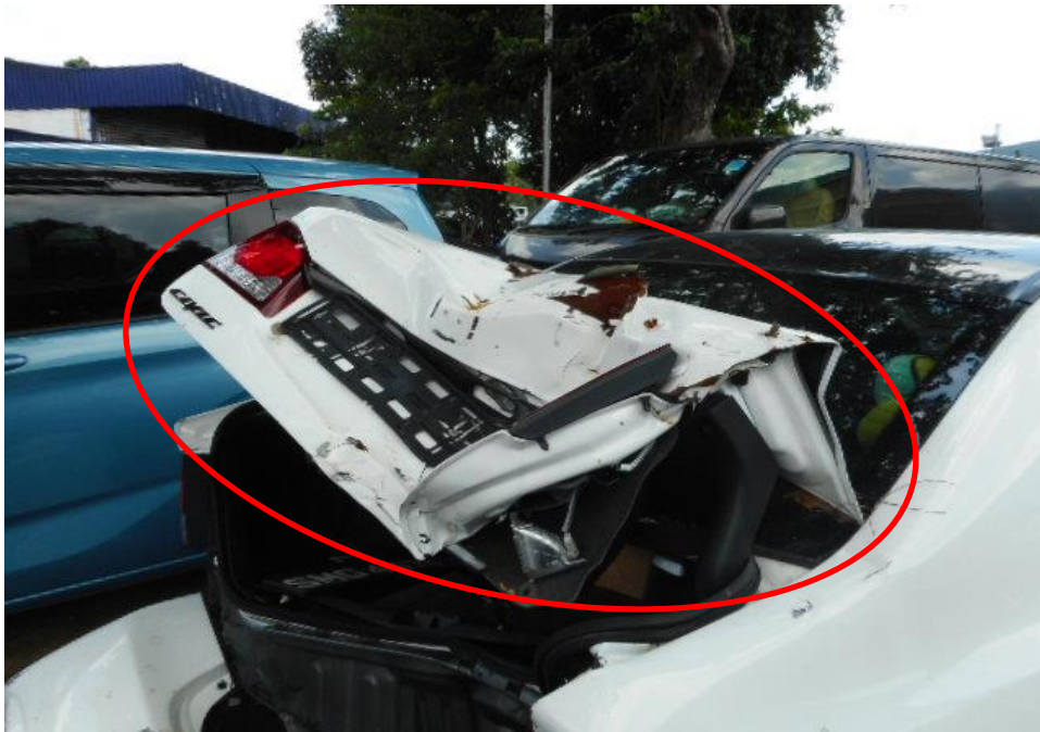
Photo 5 shows a close up view of the Motor Car's rear body at the time of my inspection. The rear portion of the Motor Car was observed to have sustained damage. Its rear bonnet and rear number plate (circled) was the body parts that were damaged as a result of the accident.
