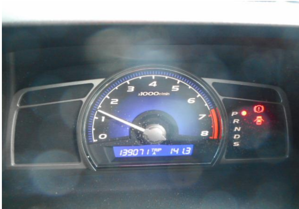
Photo 28 shows no warning lights illuminated on the instrument panel of the Motor Car after the engine was cranked. This would suggest that there was no abnormality to the electronic operating system of the Motor Car, like the ABS, and SRS etc.
