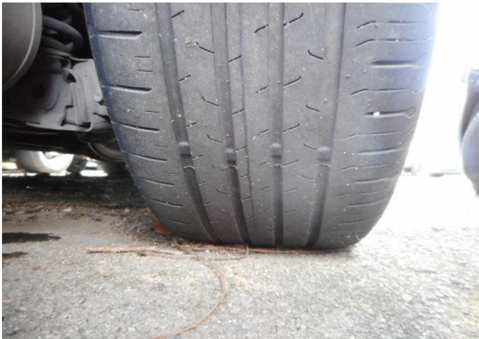
Photo 11 shows the condition of the rear right tyre of the Motor Car, which was observed to be in serviceable condition with remaining tread depth of approximately 3.5mm. The tyre was also observed to be sufficiently inflated for vehicular operation with no tear, cut or burst mark(s).
