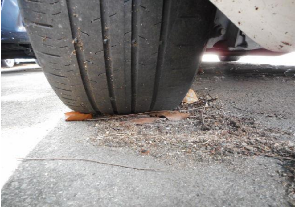
Photo 12 shows the condition of the rear left tyre of the Motor Car, which was observed to be in serviceable condition with remaining tread depth of approximately 2.9mm. The tyre, which was wrapped around steel wheel rim, was also observed to be sufficiently inflated for vehicular operation. The 4 tyres of the Motor Car were wrapped around standard steel wheel rims.
