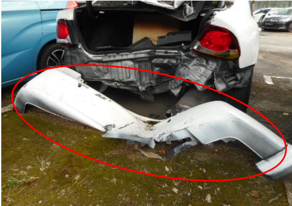
Photo 6 shows a close up view of the Motor Car's rear body at the time of my inspection. The rear portion of the Motor Car was observed to have sustained damage. Its rear bonnet and rear number plate (circled) was the body parts that were damaged as a result of the accident
