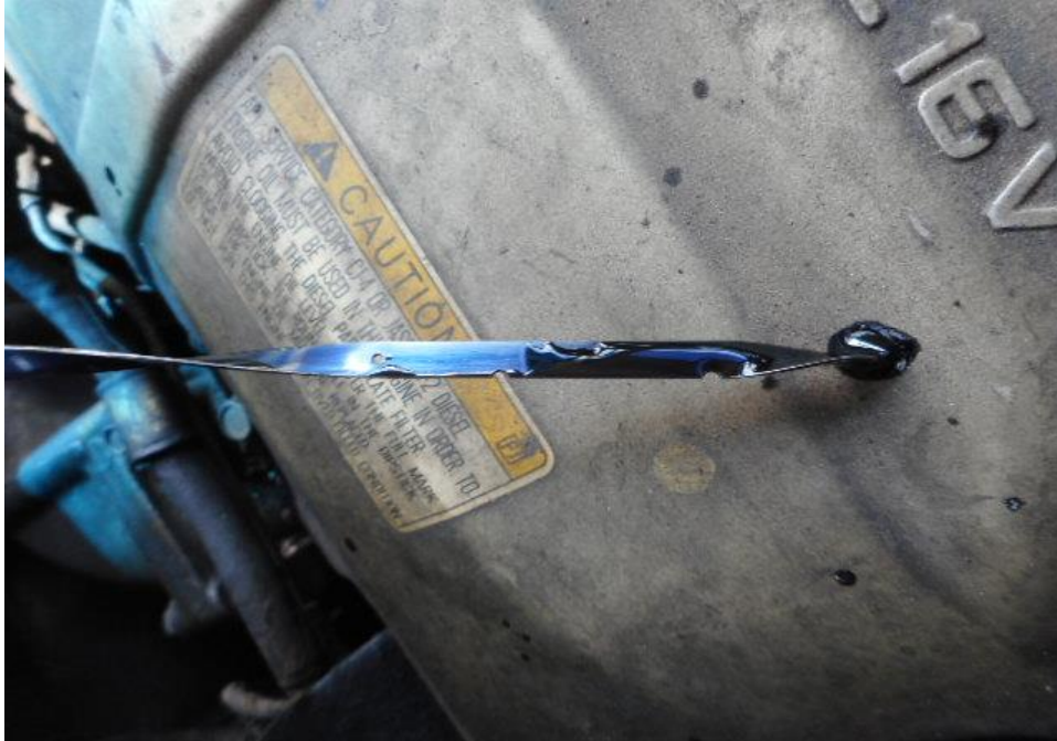
Photo 13 shows the engine oil dip stick of the Bus at the time of my inspection. The engine oil was observed to be of sufficient level and without any visible contamination.
