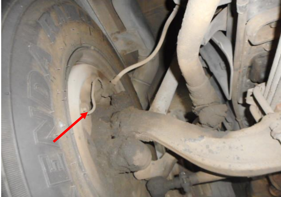
Photo 20 shows the brake hose/pipe (arrowed) at the front right wheel of the Bus. No leakage of brake fluid was observed. Visual examination of the various components of the braking system like the brake drum, brake booster, brake pedal etc had revealed all to be intact and without visible damage at the time of accident. There was also no sign of fluid stain(s) observed on the various undercarriage components.
