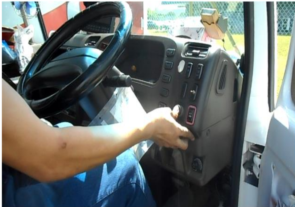
Photo 15 shows the jumpstarting process of the Bus's engine. The engine of the Bus was unable to be jumpstarted up despite multiple attempts in starting it.
