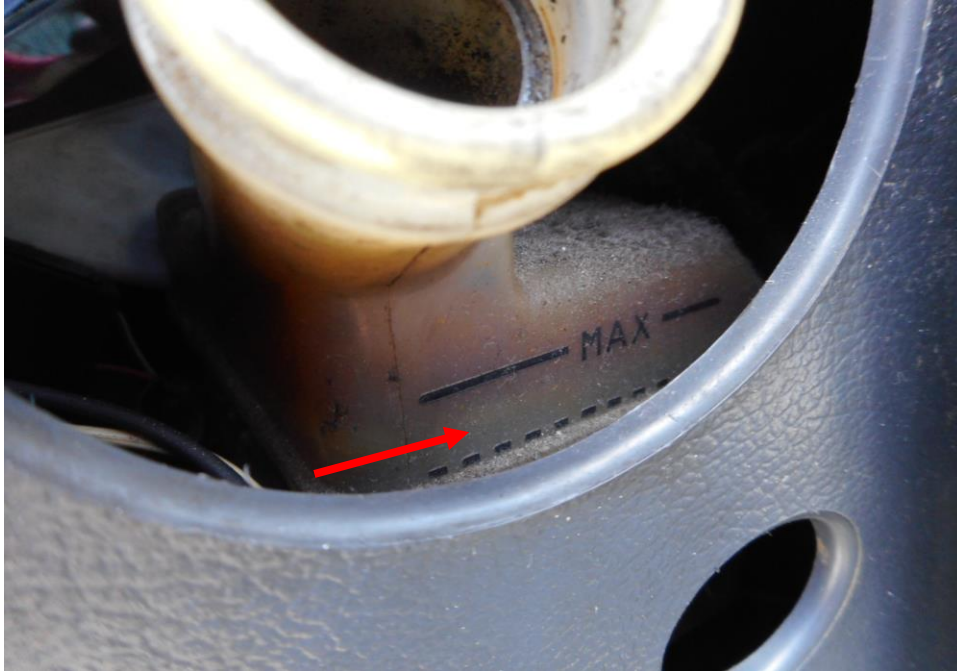
Photo 11 shows the brake fluid reservoir of the Bus at the time of my inspection. The brake fluid was observed to be of sufficient level (arrowed) and without any visible contamination.
