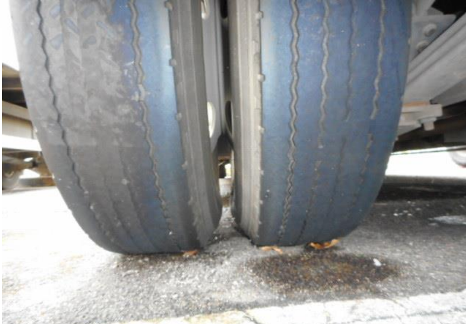
Photo 8 shows the condition of the rear left tyres of the Bus, which was observed to be in serviceable condition with remaining tread depth of approximately 1.9mm. The tyres, which were wrapped around standard steel wheel rim, were also observed to be sufficiently inflated for vehicular operation. There was also no damage found on all 6 steel wheel rims of the Bus.
