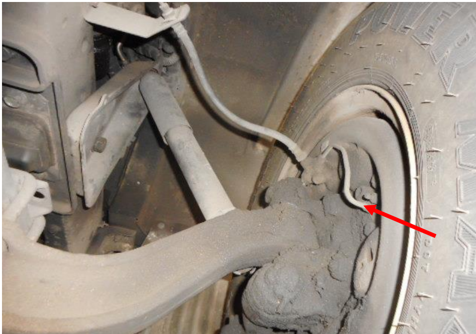
Photo 21 shows the brake hose/pipe (arrowed) at the front left wheel of the Bus. No leakage of brake fluid was observed. Visual examination of the various components of the braking system like the brake drum, brake booster, brake pedal etc had revealed all to be intact and without visible damage at the time of accident. There was also no sign of fluid stain(s) observed on the various undercarriage components.
