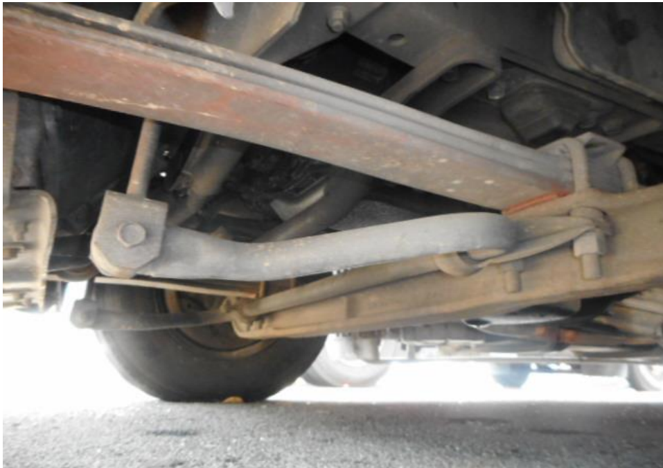
Photo 14 shows the undercarriage of the Bus, at the area where the engine housing and transmission housing are located. I did not find any sign(s) or indication(s) of fluid leak and/or fluid stain(s) on the underside of the Bus.
