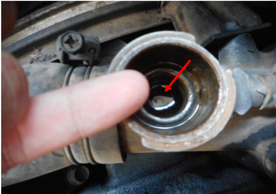
Photo 12 shows the engine coolant reservoir of the Bus at the time of my inspection. The engine coolant was observed to be of sufficient level (arrowed) and without any visible contamination.
