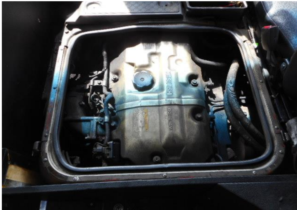
Photo 10 shows a general view of the Bus's engine compartment, which was accessed by lifting the front cabin of the Bus. The various parts and components inside the engine compartment were unaffected by the accident. There was also no sign(s) or indication(s) of fresh fluid leakage and/or fluid stain within the engine compartment
