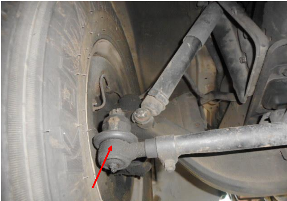
Photo 17 shows the various undercarriage components at the front left wheel of the Bus, in particular the steering tie rod end (arrowed). The various undercarriage components of the Bus were all found to be intact without any visible damage. There was also no sign of fluid stain(s) observed on the various undercarriage components.
