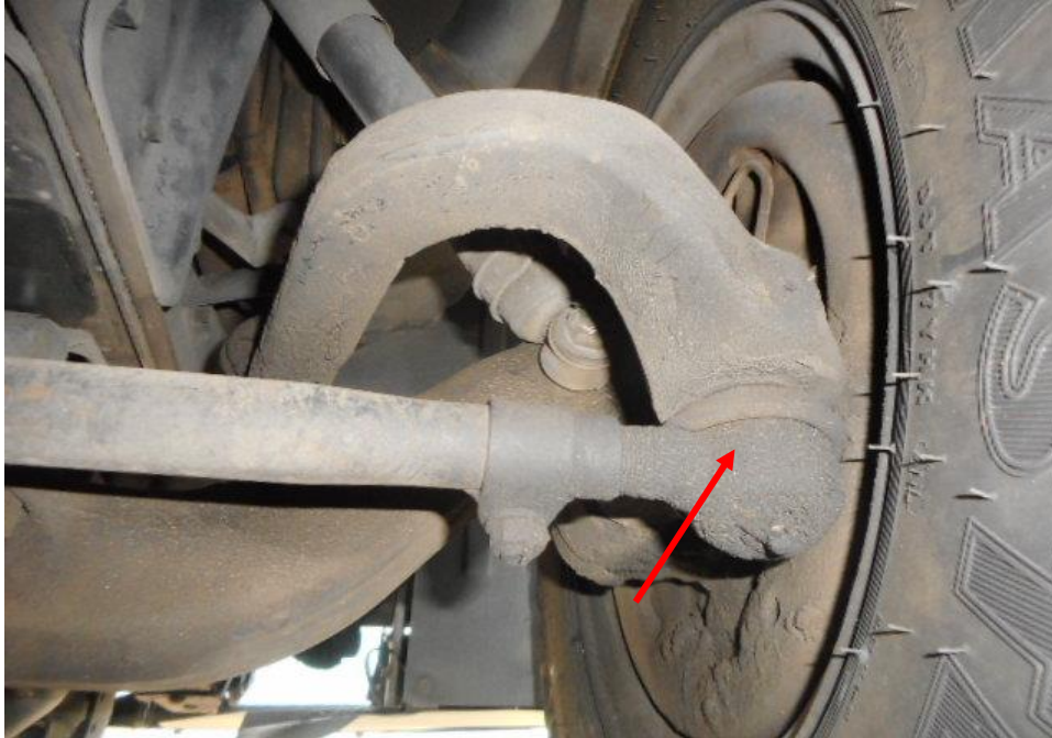
Photo 16 shows the various undercarriage components at the front right wheel of the Bus, in particular the steering tie rod end (arrowed). The various steering components were all found to be intact, suggesting that the steering system of the Bus was likely to be in serviceable condition at the material time of accident. There was also no sign of fluid stain(s) observed on the various undercarriage components.
