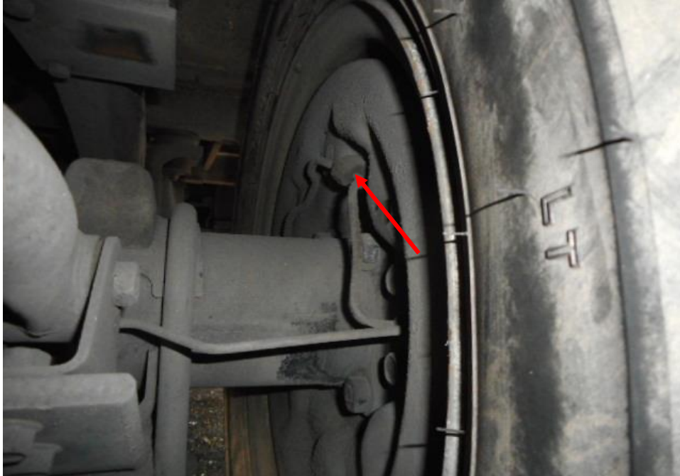
Photo 18 shows the brake pipe (arrowed) at the rear right wheel of the Bus. I did not observe any leakage of brake fluid at the time of my inspection of the Bus. My static tests of the Bus's braking system, along with my visual examination of the various mechanical components in the braking system, had indicated that there was no internal leakage of pressure/vacuum. Hence the braking system of the Bus was likely to be in serviceable condition at the material time of accident.
