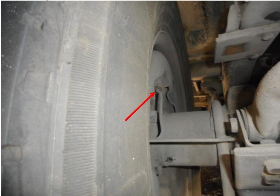
Photo 19 shows the brake pipe (arrowed) at the rear left wheel of the Bus. I did not observe any leakage of brake fluid at the time of my inspection of the Bus. My static tests of the Bus's braking system, along with my visual examination of the various mechanical components in the braking system had indicated that there was no internal leakage of pressure/vacuum. Hence the braking system of the Bus was likely to be in serviceable condition at the material time of accident.
