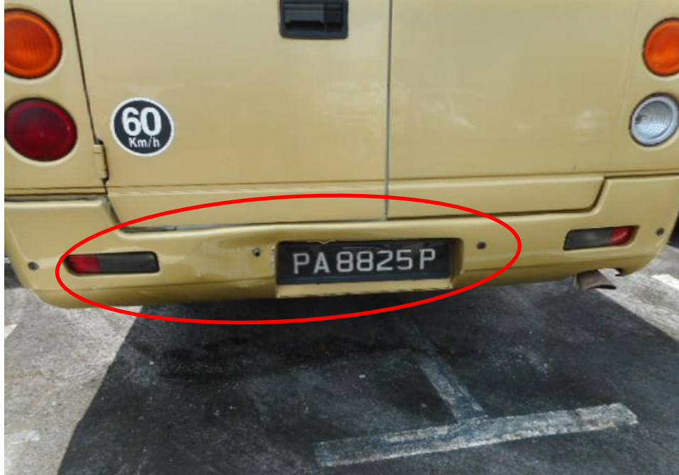
Photo 2 shows a close up view of the Bus's rear portion at the time of my inspection. The Bus rear portion was observed to have sustained damage at its rear bumper (circled) at the time of my inspection as result of the accident.
