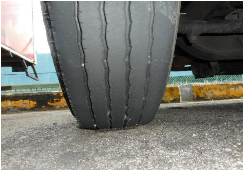
Photo 9 shows the condition of the rear right tyres of the Bus, which were observed to be in serviceable condition with remaining, tread depth of approximately 4.6mm. There was also no tear, cut or burst mark(s) on the outer and the inner sidewalls as well as across the tread of the 6 tyres that were fitted on the Bus.
