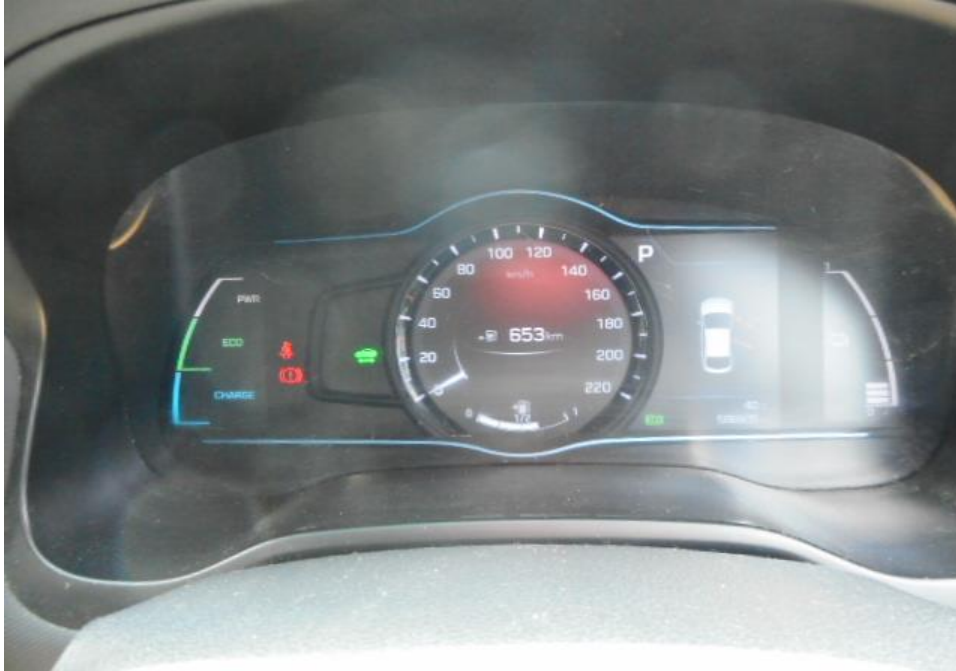
Photo 25 shows no warning lights illuminated on the instrument panel of the Motor Taxi after the engine was cranked. This would suggest that there was no abnormality to the electronic operating system of the Motor Taxi, like the ABS, EPS, TCS and SRS etc.
