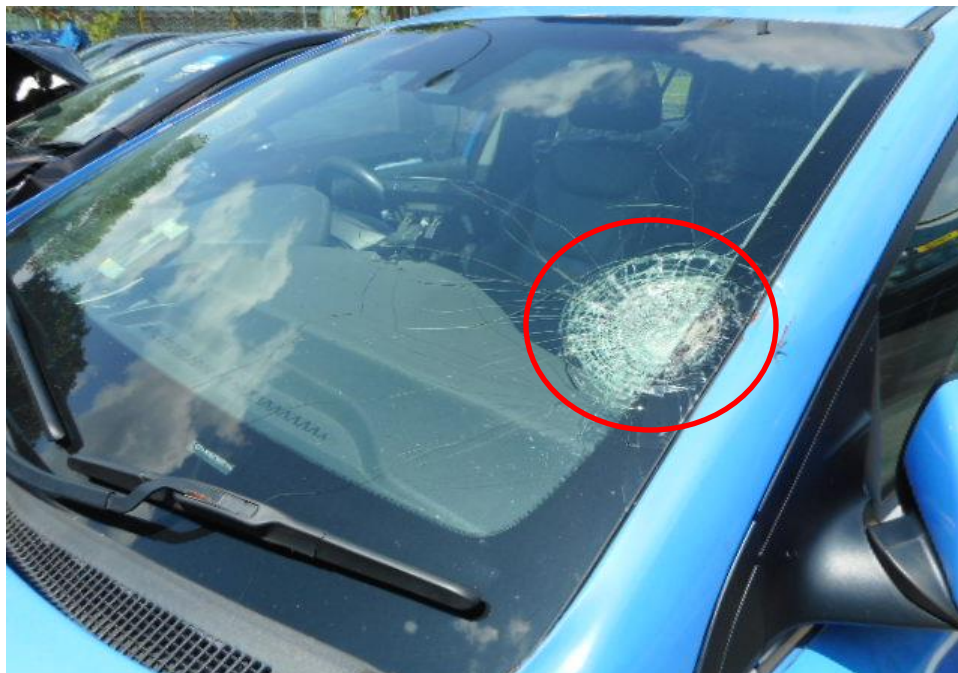
Photo 3 shows a close up view of the Motor Taxi's front body at the time of my inspection. The front portion of the Motor Taxi was observed to have sustained damage. Its front windscreen (circled) was the body part that were damaged as a result of the accident.
