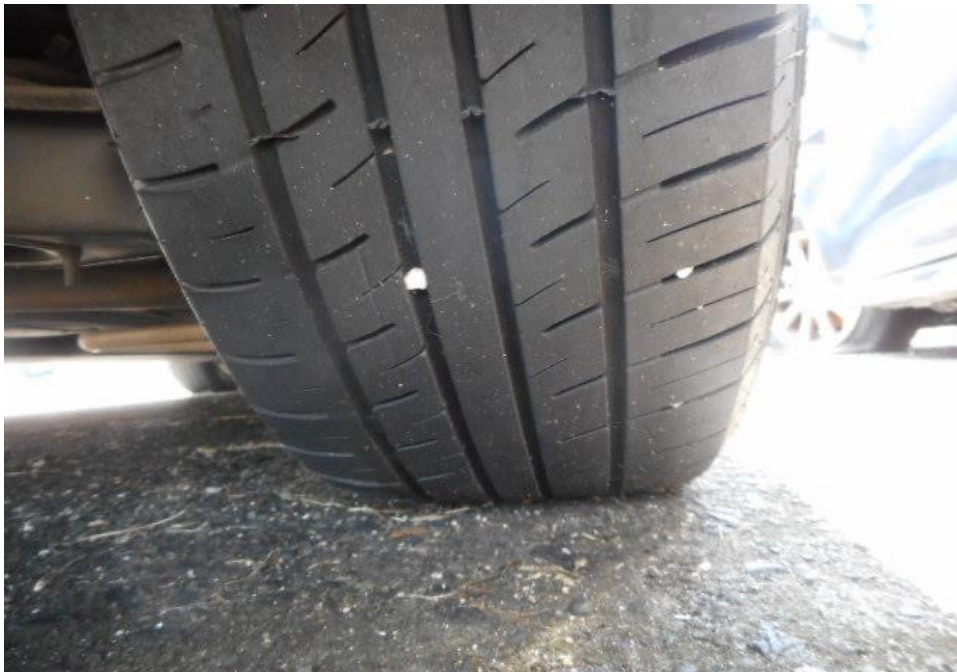
Photo 9 shows the condition of the rear right tyre of the Motor Taxi, which was observed to be in serviceable condition with remaining tread depth of approximately 4.8mm. The tyre was also observed to be sufficiently inflated for vehicular operation with no tear, cut or burst mark(s).
