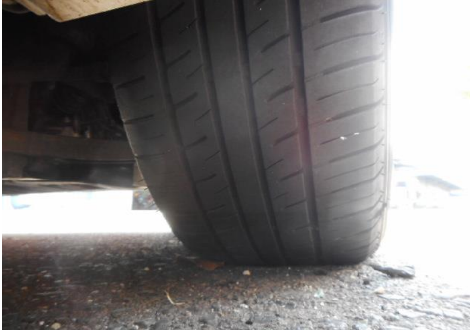
Photo 8 shows the condition of the front right tyre of the Motor Taxi, which was observed to be in serviceable condition with remaining tread depth of approximately 3.8mm. The tyre was sufficiently inflated for vehicular operation with no tear, cut or burst mark(s) on the outer and the inner sidewalls as well as across the tread. The 4 tyres of the Motor Taxi were wrapped around standard steel wheel rims without any damage.
