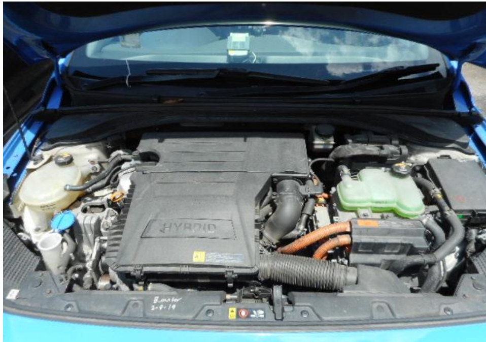
Photo 12 shows a general view of the Motor Taxi's engine compartment. The various parts and components inside the engine compartment were unaffected by the accident. There was also no sign(s) or indication(s) of fluid leakage and/or fluid stain within the engine compartment.
