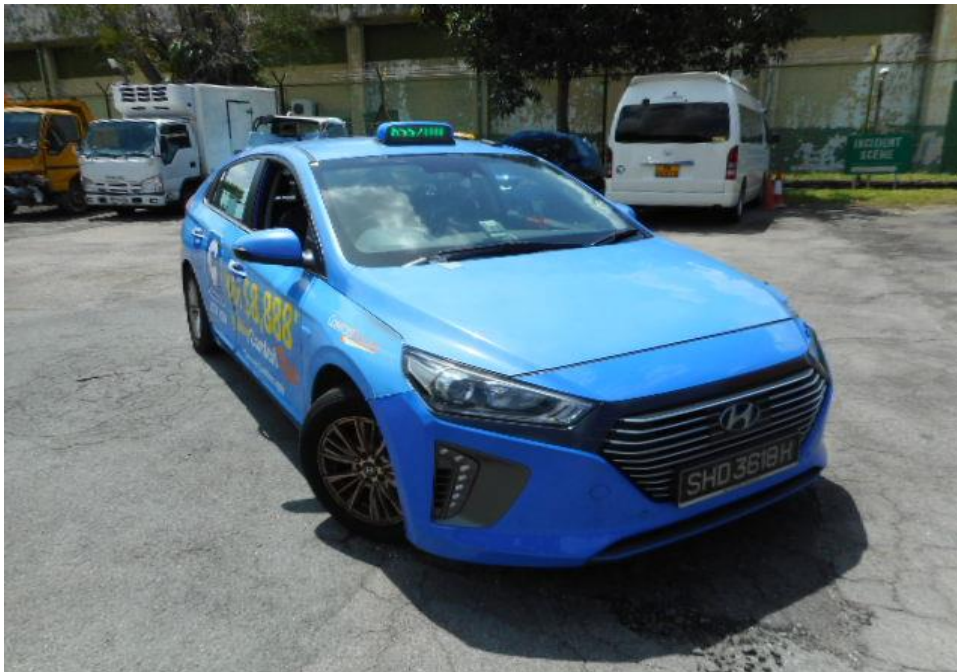
Photo 21 shows the front right wheel of the Motor Taxi turned to its full left. During my steering system test, I did not experience any abnormal free play and/or resistance when I had turned the steering wheel towards the left and right. This would suggest that the steering system of the Motor Taxi was likely to be in serviceable condition at the material time of accident.
