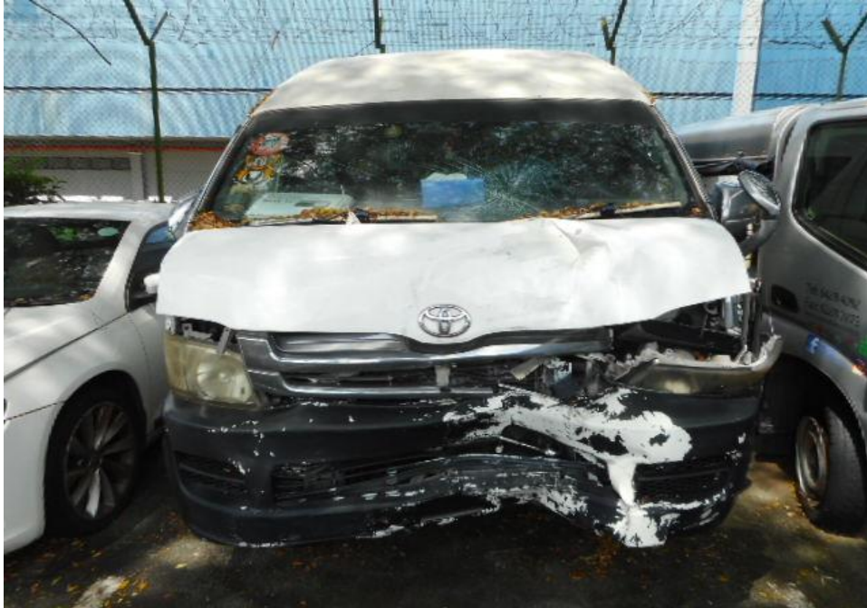
Photo 2 shows a general view of the Mini Bus's frontal portion at the time of my inspection. The Mini Bus front portion was observed to have sustained damage at its front windscreen, front body panel, front bumper, front left headlamp and engine components were damage at the time of my inspection as result of the accident.
