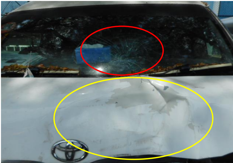
Photo 3 shows a close up view of the Mini Bus's frontal portion at the time of my inspection. The Mini Bus front portion was observed to have sustained damage at its front windscreen (red circle) and front body panel (yellow circle) at the time of my inspection as result of the accident.
