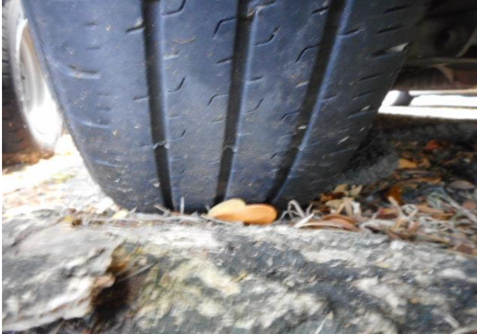
Photo 10 shows the condition of the rear left tyres of the Mini Bus, which was observed to be in serviceable condition with remaining tread depth of approximately 3.5mm. The tyres, which were wrapped around standard steel wheel rim, were also observed to be sufficiently inflated for vehicular operation. There was also no damage found on all 4 steel wheel rims of the Mini Bus.
