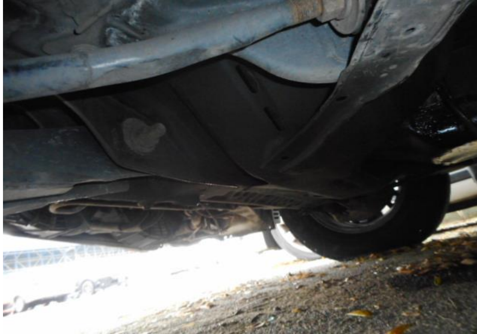
Photo 17 shows the undercarriage of the Mini Bus, at the area where the engine housing and transmission housing are located. I did not find any sign(s) or indication(s) of fluid leak and/or fluid stain(s) on the underside of the Mini Bus.
