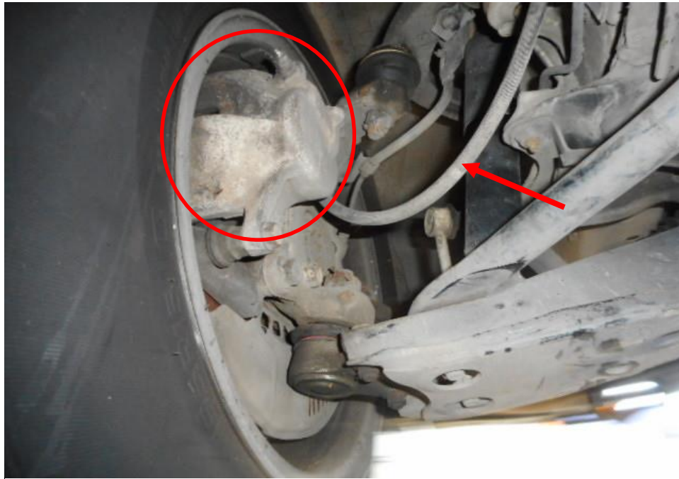
Photo 24 shows the brake hose/pipe (arrowed) at the front left wheel of the Mini Bus. No leakage of brake fluid was observed. Visual examination of the various components of the braking system like the brake caliper (circled), brake booster, brake pedal etc had revealed all to be intact and without visible damage at the time of accident. There was also no sign of fluid stain(s) observed on the various undercarriage components.
