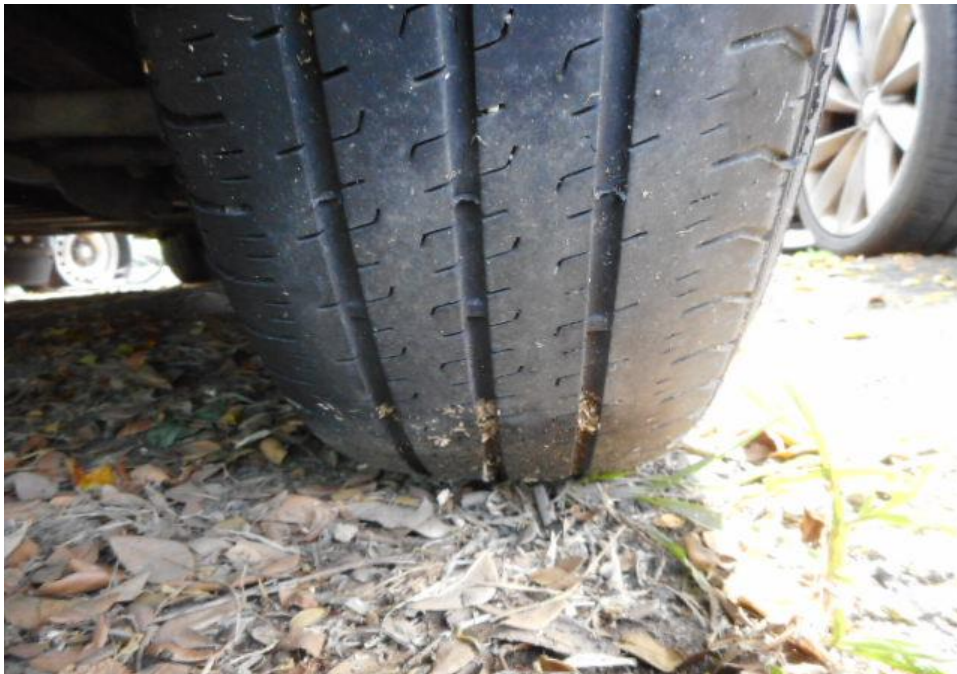
Photo 9 shows the condition of the rear right tyre of the Mini Bus, which was observed to be in serviceable condition with remaining tread depth of approximately 3.4mm. The tyre, which was wrapped around standard steel wheel rim, it was observed to be sufficiently inflated for vehicular operation.
