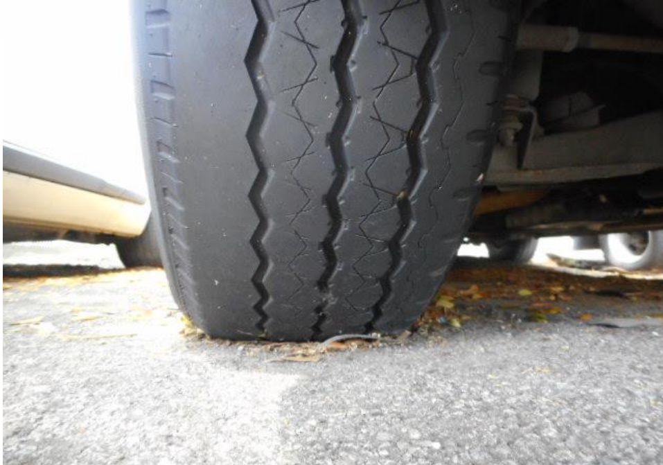
Photo 8 shows the condition of the front right tyre of the Mini Bus, which was observed to be in serviceable condition with remaining tread depth of approximately 6mm. The tyre, which was wrapped around standard steel wheel rim, was also observed to be sufficiently inflated for vehicular operation. There was no tear, cut or burst mark(s) on the outer and the inner sidewalls as well as across the tread of the 4 tyres that were fitted on the Mini Bus.
