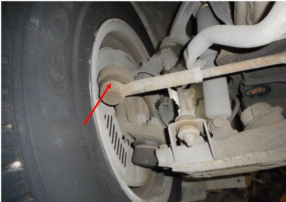
Photo 19 shows the various undercarriage components at the front right wheel of the Mini Bus, in particular the steering tie rod end (arrowed). The various steering components were all found to be intact, suggesting that the steering system of the Mini Bus was likely to be in serviceable condition at the material time of accident. There was also no sign of fluid stain(s) observed on the various undercarriage components.
