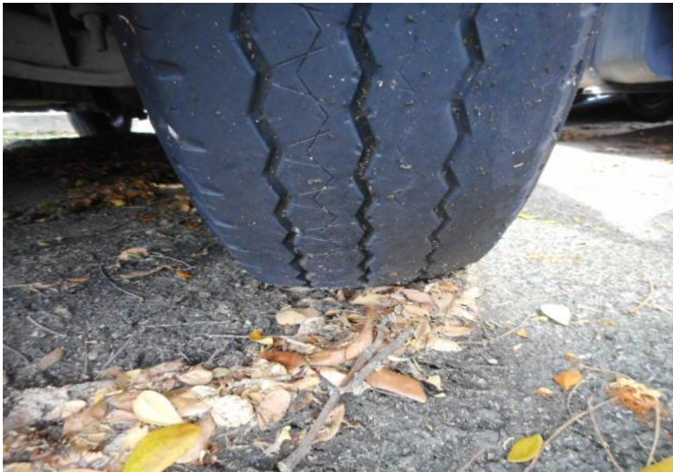
Photo 11 shows the condition of the rear right tyres of the Mini Bus, which were observed to be in serviceable condition with remaining, tread depth of approximately 5.3mm. There was also no tear, cut or burst mark(s) on the outer and the inner sidewalls as well as across the tread of the 4 tyres that were fitted on the Mini Bus.
