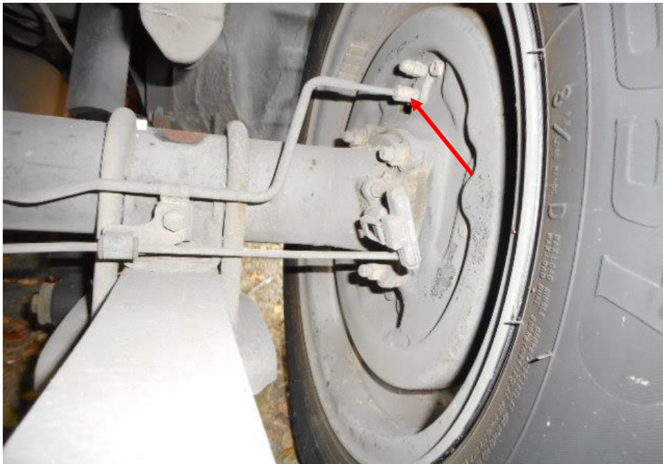
Photo 21 shows the brake pipe (arrowed) at the rear right wheel of the Mini Bus. I did not observe any leakage of brake fluid at the time of my inspection of the Mini Bus. My static tests of the Mini Bus's braking system, along with my visual examination of the various mechanical components in the braking system, had indicated that there was no internal leakage of pressure/vacuum. Hence the braking system of the Mini Bus was likely to be in serviceable condition at the material time of accident.
