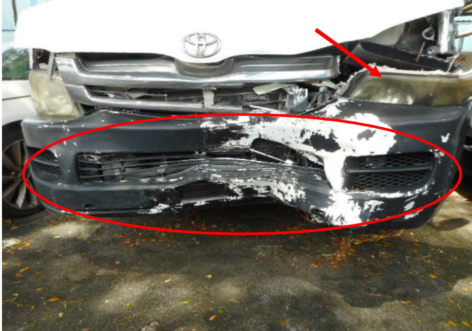
Photo 4 shows a close up view of the Mini Bus's frontal portion at the time of my inspection. The Mini Bus front portion was observed to have sustained damage at its front bumper (circled) and front left headlamp (arrowed) at the time of my inspection as result of the accident.
