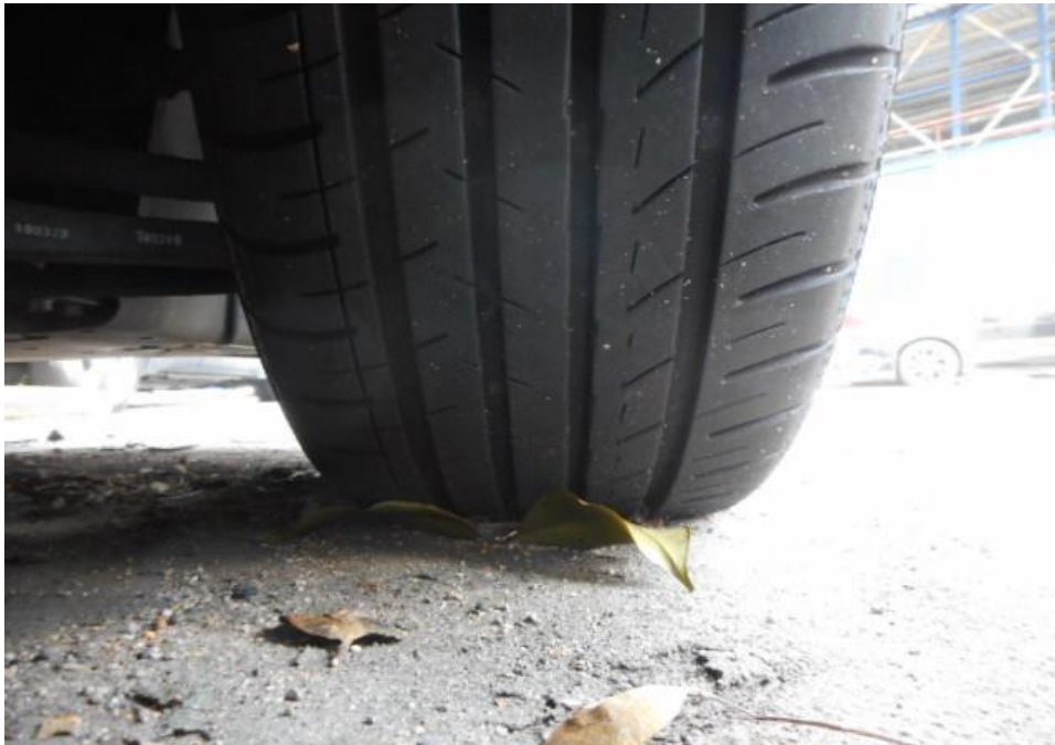
Photo 7 shows the condition of the front right tyre of the Motor Car, which was observed to be in serviceable condition with remaining tread depth of approximately 6.1mm. The tyre was sufficiently inflated for vehicular operation with no tear, cut or burst mark(s) on the outer and the inner sidewalls as well as across the tread. The 4 tyres of the Motor Car were wrapped around standard steel wheel rims without any damage.
