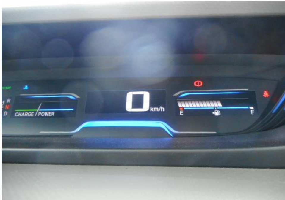
Photo 24 shows no warning lights illuminated on the instrument panel of the Motor Car after the engine was cranked. This would suggest that there was no abnormality to the electronic operating system of the Motor Car, like the ABS, EPS, TCS and SRS etc.
