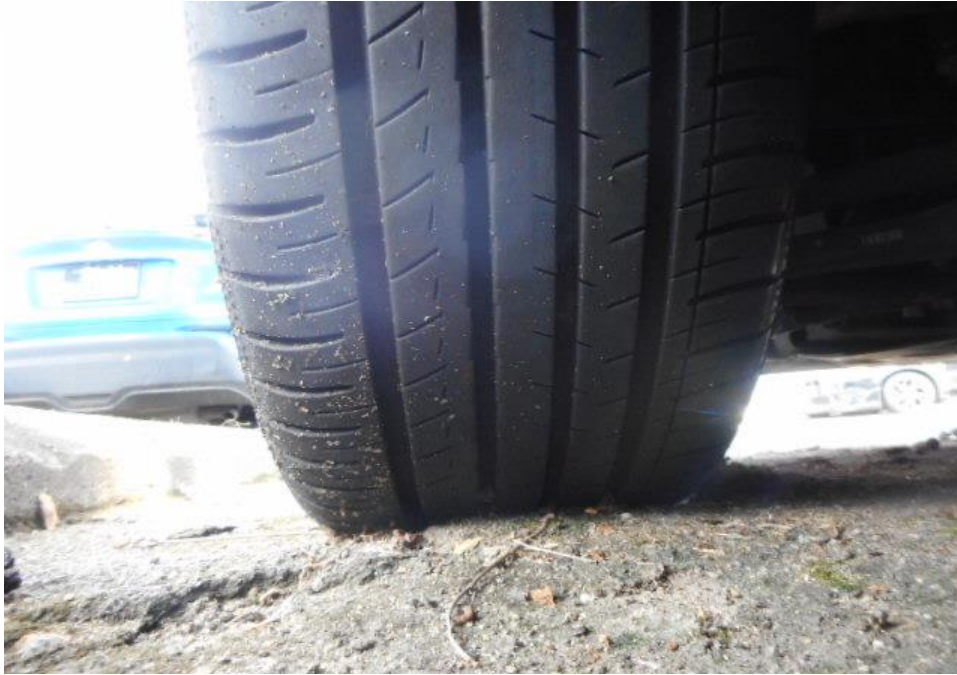
Photo 10 shows the condition of the front left tyre of the Motor Car, which was observed to be in serviceable condition with remaining tread depth of approximately 5.9mm. There was also no tear, cut or burst mark(s) on the outer and the inner sidewalls as well as across the tread of the Motor Car's 4 tyres.
