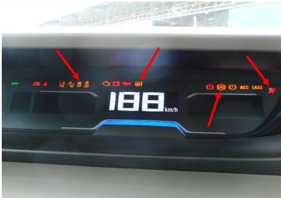
Photo 23 shows the warning light for Anti-Lock Brake System (ABS), Electric Power Steering System (EPS), Traction Control System (TCS) and Supplemental Restraint System (SRS) (arrowed) appearing on the instrument panel of the Motor Car during the self-test of its various electronic operating systems when its engine was cranked.
