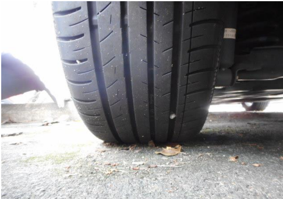
Photo 9 shows the condition of the rear left tyre of the Motor Car, which was observed to be in serviceable condition with remaining tread depth of approximately 5.9mm. The tyre, which was wrapped around steel wheel rim, was also observed to be sufficiently inflated for vehicular operation. The 4 tyres of the Motor Car were wrapped around standard steel wheel rims.
