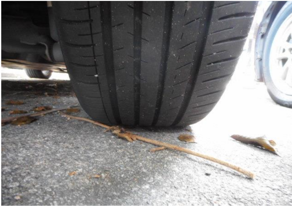
Photo 8 shows the condition of the rear right tyre of the Motor Car, which was observed to be in serviceable condition with remaining tread depth of approximately 5.9mm. The tyre was also observed to be sufficiently inflated for vehicular operation with no tear, cut or burst mark(s).
