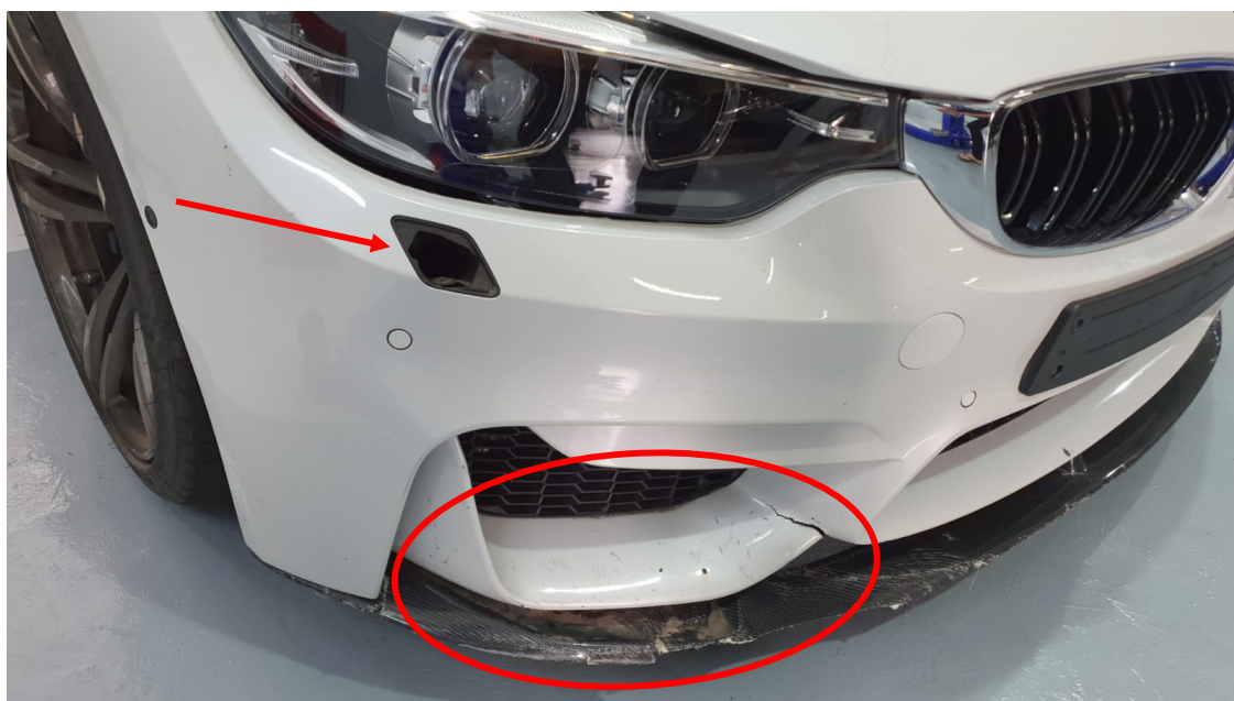
Photo 2 shows a closer view of the damage to the front bumper and front bumper lower lip of the Motor Car (photograph provided to me). The front right headlamp washer cover (arrowed) was also observed to be missing.
