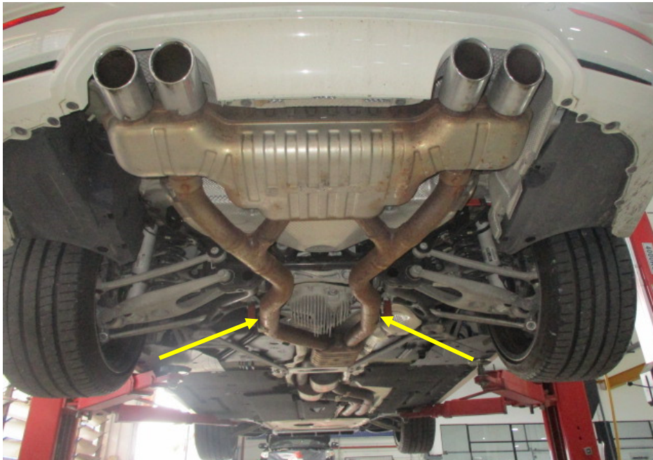
Photo 20 shows a general view of the rear section of the Motor Car's exhaust system. My examination of the Motor Car's exhaust system revealed no sign(s) or indication(s) of any cut or weld marks along its exhaust pipes (arrowed), on its catalytic converters, centre resonator boxes and on its rear mufflers.
