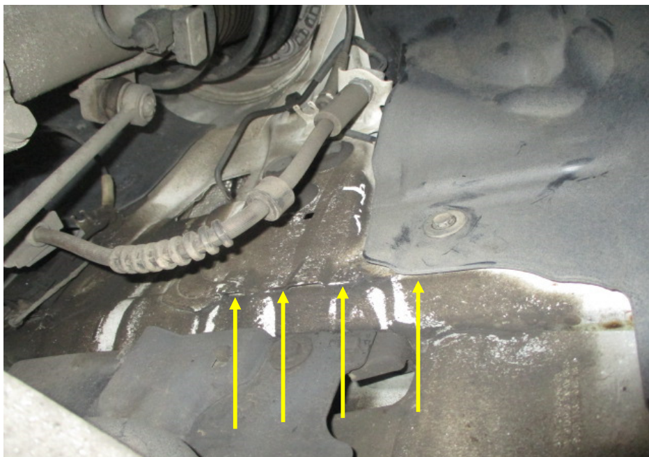
Photo 22 shows the chassis/structural body at the underside front right of the Motor Car. I did not find any weld marks other than original spot weld marks on the chassis/structural body of the Motor Car. The original factory sealant (arrowed) at the joints along the chassis/structural body was untouched, indicating no work was done on the chassis/structural body of the Motor Car and that the chassis/structural body was originally fitted.
