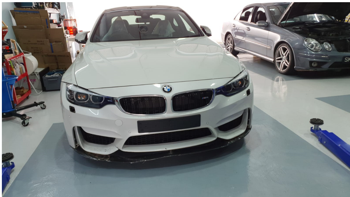
Photo 1 shows the frontal body of the Motor Car (photograph provided to me). The photographs provided to me had showed damage to the frontal portion of the Motor Car. Body parts observed to be damaged were the front bumper and front bumper lower lip. The front left headlamp washer cover and front right headlamp washer cover were both observed to be missing.
