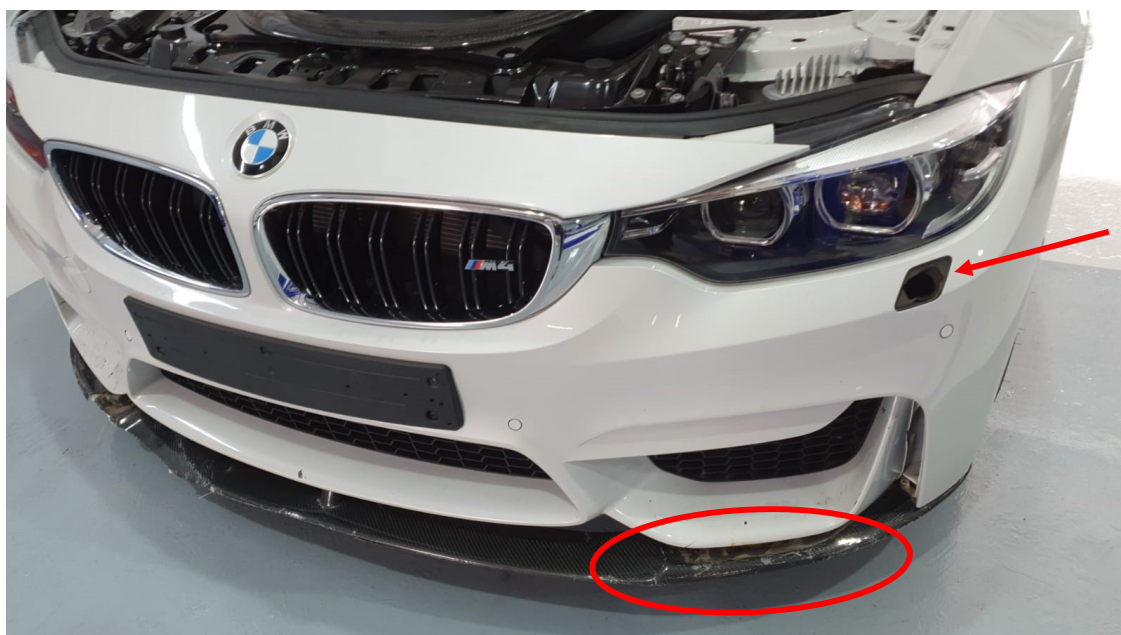
Photo 3 shows a closer view of the damage to the front bumper and front bumper lower lip of the Motor Car (photograph provided to me). The front left headlamp washer cover (arrowed) was also observed to be missing.
