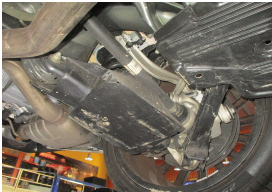
Photo 17 shows a general view of the control arms and linkages at the rear left wheel of the Motor Car. I did not observe any fluid leak and/or fluid stain on the underside of the Motor Car. All of the Motor Car's undercarriage components were observed to be intact and secured in an appropriate manner.
