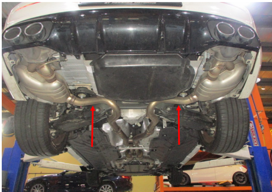
Photo 20 shows a general view of the Motor Car's exhaust system (rear section). My examination of the Motor Car's exhaust system revealed no sign(s) or indication(s) of any cut or weld marks along its exhaust pipes (arrowed), on its centre resonator boxes, catalytic converters and on its rear mufflers.
