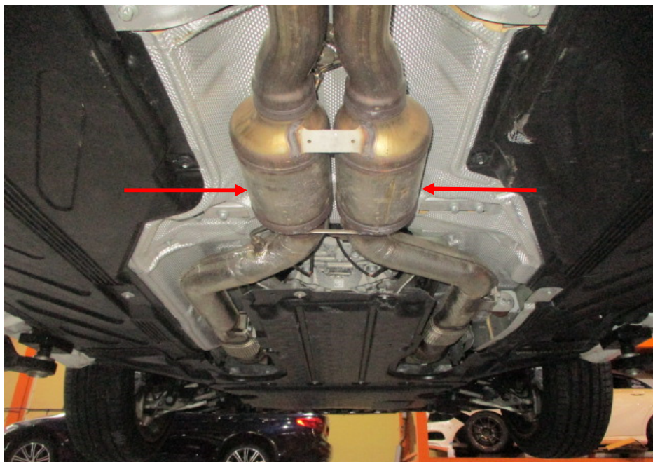
Photo 21 shows a general view of the Motor Car's exhaust system (front section). My examination of the Motor Car's exhaust system revealed no sign(s) or indication(s) of any cut or weld marks along its exhaust pipes, on its centre resonator boxes (arrowed), catalytic converters and on its rear mufflers.
