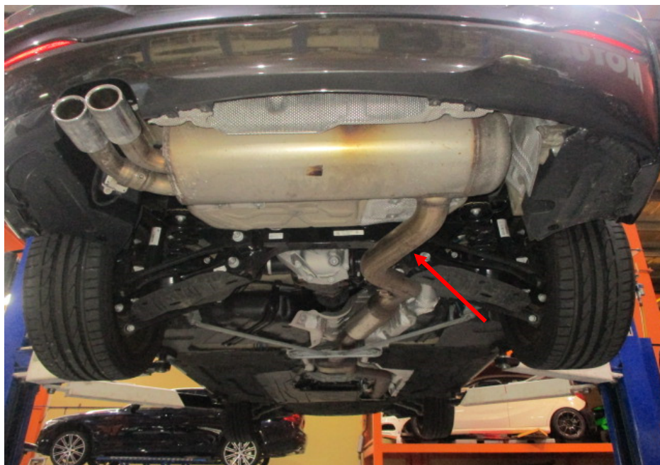
Photo 18 shows a general view of the Motor Car's exhaust system (rear section). My examination of the Motor Car's exhaust system revealed no sign(s) or indication(s) of any cut or weld marks along its exhaust pipes (arrowed), centre resonator boxes, rear muffler and on its catalytic converter.
