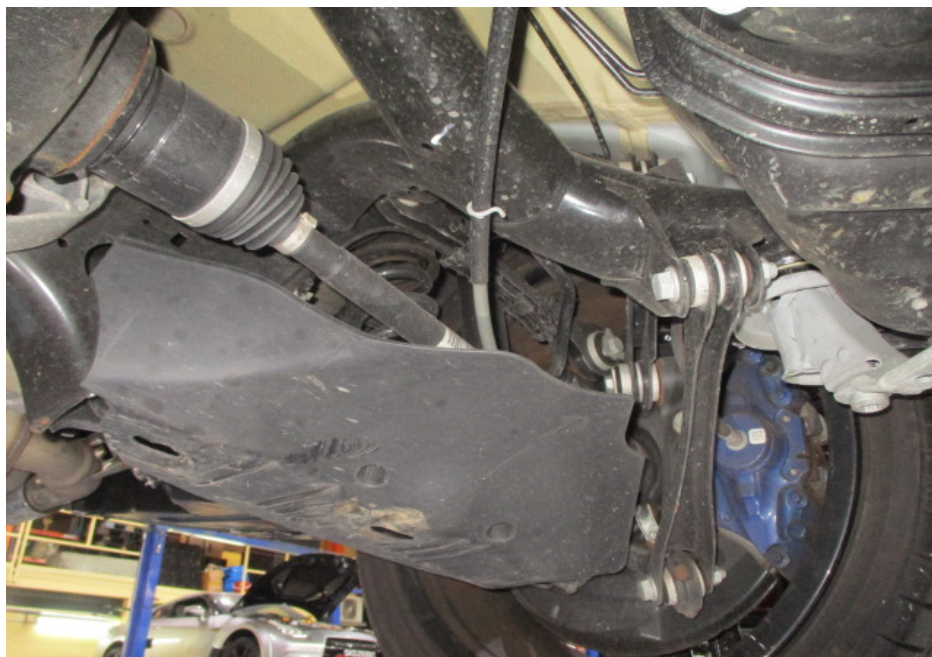
Photo 16 shows the various undercarriage components at the rear left wheel of the Motor Car. The mechanical components, control arms and linkages were all found to be intact and secured in an appropriate manner.
