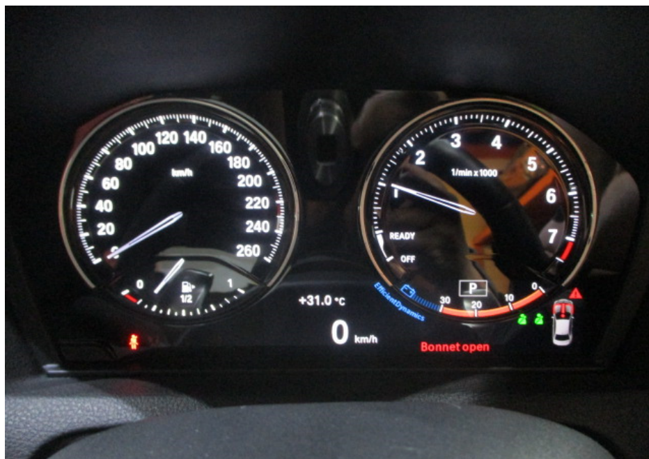
Photo 13 shows the respective warning lights no longer illuminated, indicating that there is no fault detected to the ABS, SRS, IAS, TPM and DSC systems of the Motor Car during the self-test. These electronic systems were hence in working condition at the time of my inspection.
