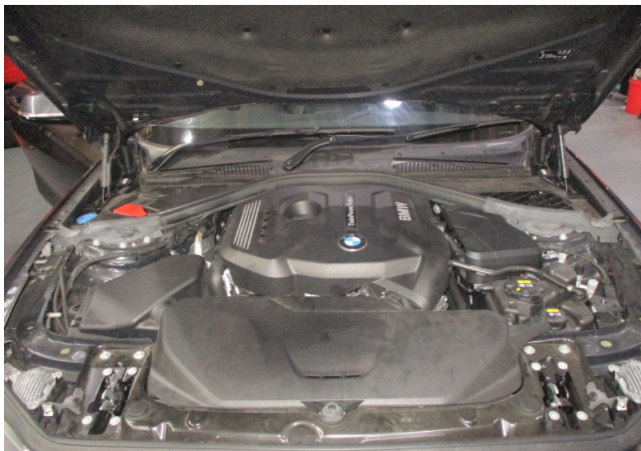
Photo 10 shows a general view of the Motor Car's engine compartment at the time of my inspection. The various parts and components inside the engine compartment were all observed to be intact and properly fitted. There was also no sign(s) or indication(s) of fluid leak and/or fluid stain found within the engine compartment.
