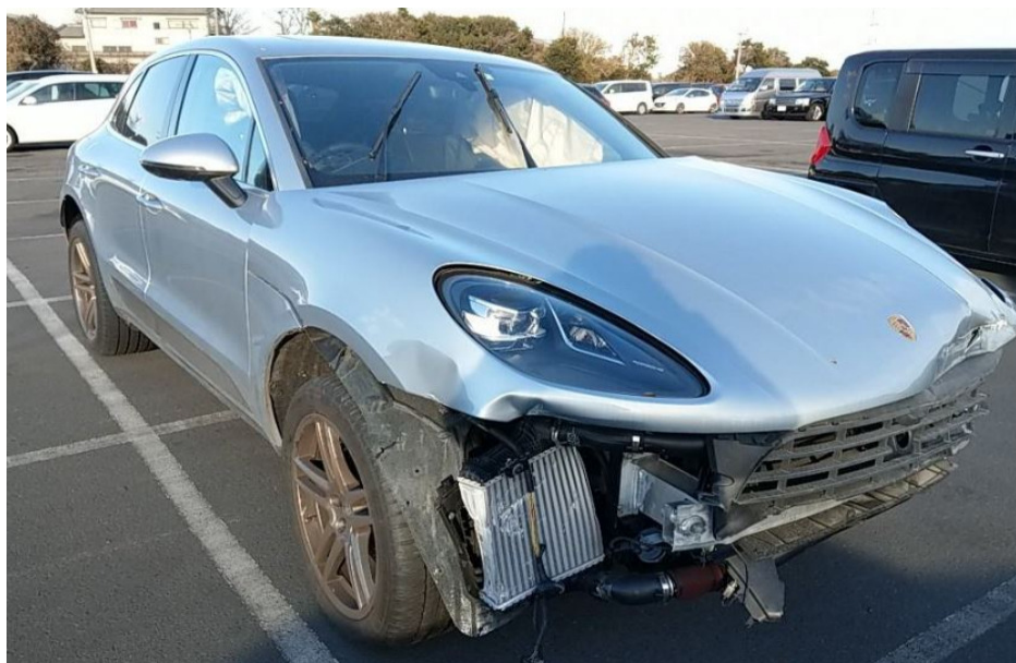
Photo 1 shows the front right body of the Motor Car prior to any repairs being carried out (photograph provided to me). The Motor Car was observed to have sustained damages at its frontal portion. The front bumper, front bumper right grille, front bumper centre lower grille, front bumper right lower grille, front bumper reinforcement, front radiator grille, front right day running light, front right intercooler, front bonnet and front right fender inner shield were amongst the body parts that were observed to be damaged.
