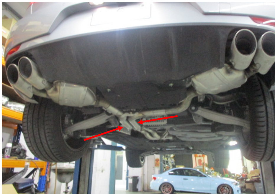
Photo 21 shows a general view of the Motor Car's exhaust system. My examination of the Motor Car's exhaust system revealed no sign(s) or indication(s) of any cut or weld marks along its exhaust pipes (arrowed), on its catalytic converters and on its rear mufflers.
