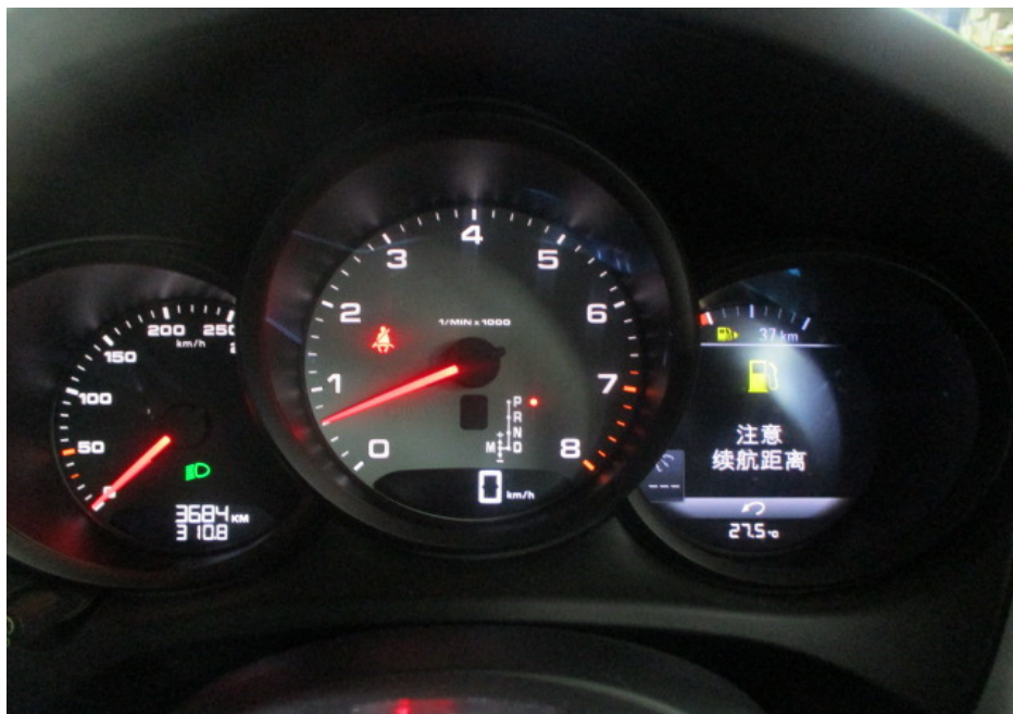
Photo 16 shows the respective warning lights no longer illuminated, indicating that there is no fault detected to the ABS, SRS, TPM and TCS systems of the Motor Car during the self-test. These electronic systems were hence in working condition at the time of my inspection.
