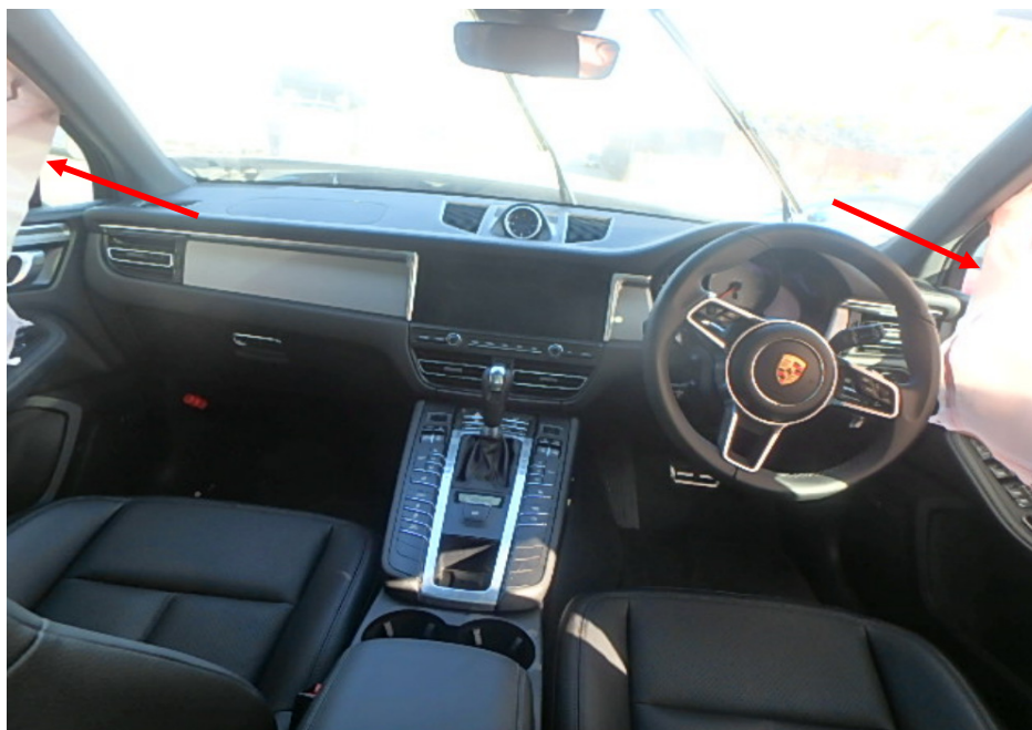
Photo 4 shows the interior compartment of the Motor Car prior to any repairs being carried out (photograph provided to me). The right side curtain airbag and left side curtain airbag were deployed (arrowed).
