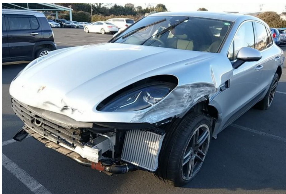
Photo 2 shows the front left body of the Motor Car prior to any repairs being carried out (photograph provided to me). The Motor Car was observed to have sustained damages at its frontal portion. The front bumper, front bumper left grille, front bumper centre lower grille, front bonnet, front left day running light, front left intercooler, front left headlamp and front left wheel rim were amongst the body parts that were observed to be damaged.
