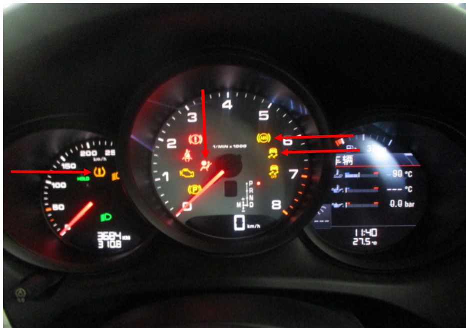
Photo 15 shows the warning lights for the various electronic safety features appearing on the instrument panel of the Motor Car during its self-test when the engine is cranked, in particular the ABS, SRS, TPM and TCS lights (arrowed).
