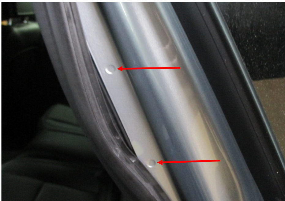
Photo 25 shows the left side "C" pillar of the Motor Car. I did not find any weld marks other than original spot weld marks (arrowed) on the left side "C" pillar of the Motor Car which, indicates that there was no re-welding works carried out. In general, I had found all the non-detachable body panels of the Motor Car to be originally fitted at the time of my inspection.
