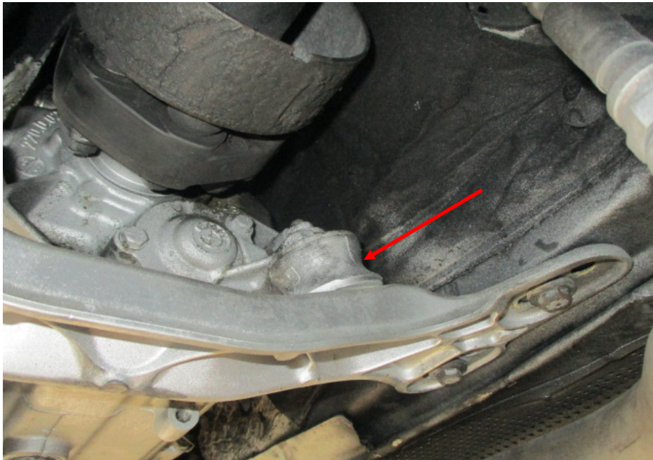
Photo 6 shows a closer view of the other rubber bushing (arrowed). The rubber bushing sits between the transmission and the bracket, absorbing any vibrations arising from the rotation of the transmission gears. This minimises any stress to the bracket.
