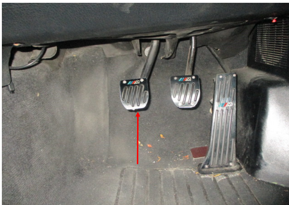
Photo 9 shows the clutch pedal (arrowed) for engaging and disengaging the transmission gears.
