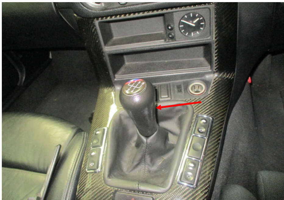
Photo 8 shows the gear shifter (arrowed) that was fitted on the Motor Car, for manually selecting the transmission gear to be engaged. The gear selector fork from the underside of the Motor Car (refer to photograph 7 above) connects to this gear shifter through the floorboard.
