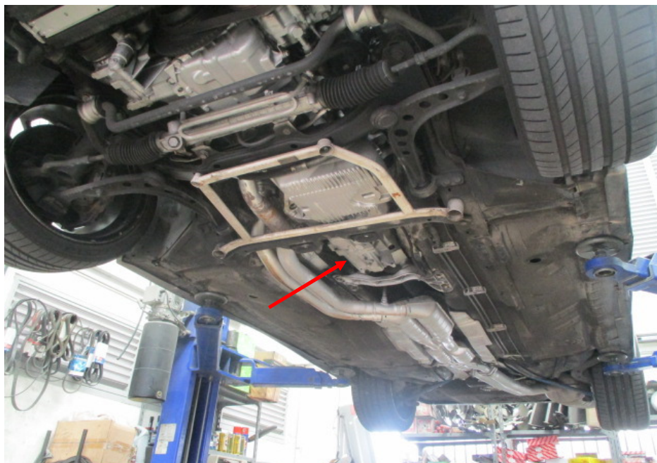
Photo 2 shows a general view of the transmission (arrowed) that was fitted on the Motor Car. The front (input) side of the transmission is bolted to the crankshaft side of the engine block while the rear (output) side of the transmission was connected to the propeller shaft, which links to the rear axle of the Motor Car.
