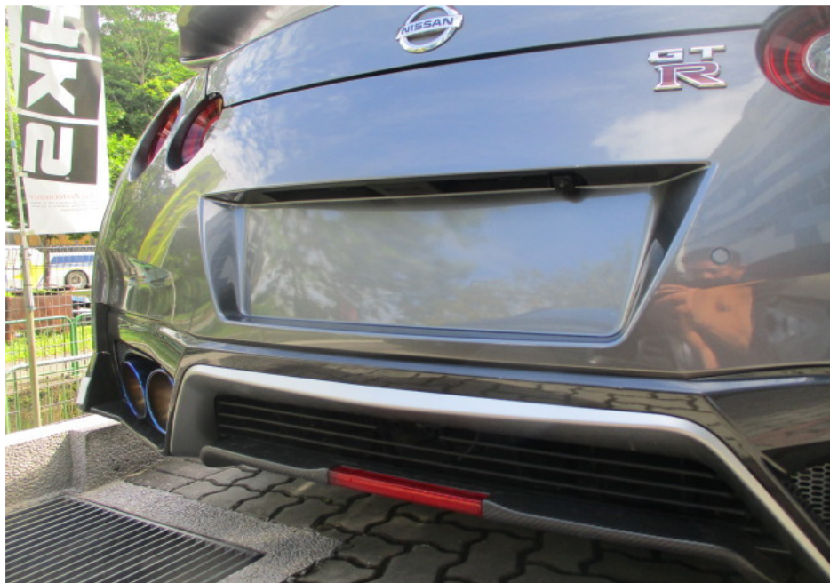
Photo 9 shows a closer view of the Motor Car's rear bumper, rear bumper lower cover, rear bumper lower cover garnish and rear bumper diffuser at the time of my inspection. The rear portion of the Motor Car were visually examined, and it was observed that the repair/restoration works carried out to the damaged area of the Motor Car (refer to photograph 1 & 2 above) were reasonably adequate and in order.
