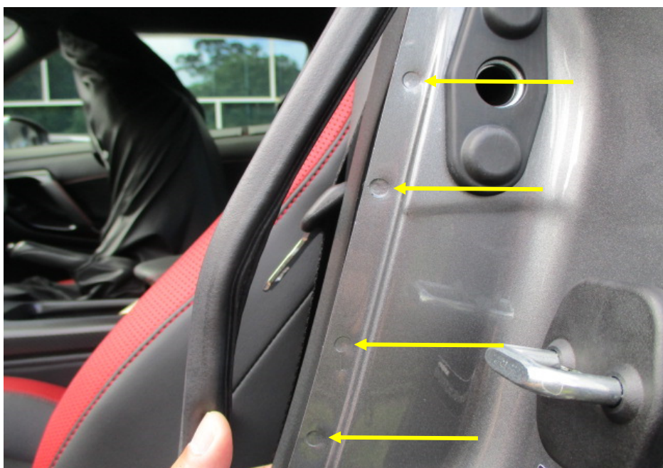
Photo 25 shows the left side rear body panel of the Motor Car. I did not find any weld marks other than original spot weld marks (arrowed) on the left side rear body panel of the Motor Car, which indicates that there was no re-welding works carried out. In general, I had found all the non-detachable body panels of the Motor Car to be originally fitted at the time of my inspection.
