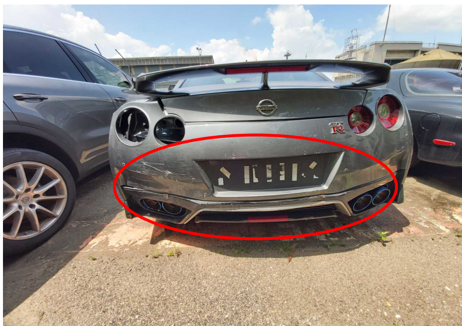
Photo 2 shows the rear body of the Motor Car (photograph provided to me). The Motor Car was observed to have sustained damage at its rear portion (circled). From the photographs provided, I had observed damage to the rear bumper, rear bumper lower cover, rear bumper lower cover garnish, rear bumper diffuser and rear left taillamp.
