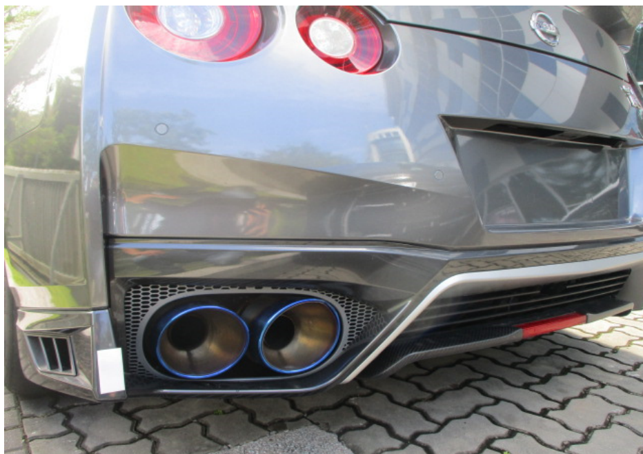
Photo 7 shows a closer view of the Motor Car's rear bumper, rear bumper lower cover, rear bumper lower cover garnish, rear bumper diffuser and rear left taillamp at the time of my inspection. The rear portion of the Motor Car were visually examined, and it was observed that the repair/restoration works carried out to the damaged area of the Motor Car (refer to photograph 1 & 2 above) were reasonably adequate and in order.
