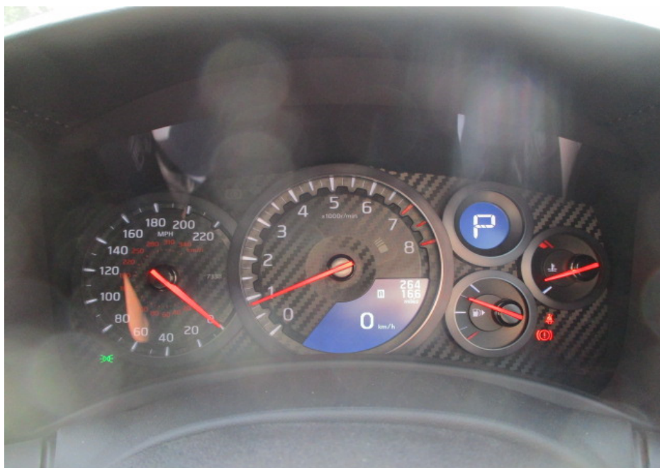
Photo 15 shows the respective warning lights no longer illuminated, indicating that there is no fault detected to the ABS, SRS, TPM and VDC systems of the Motor Car during the self-test. These electronic systems were hence in working condition at the time of my inspection.
