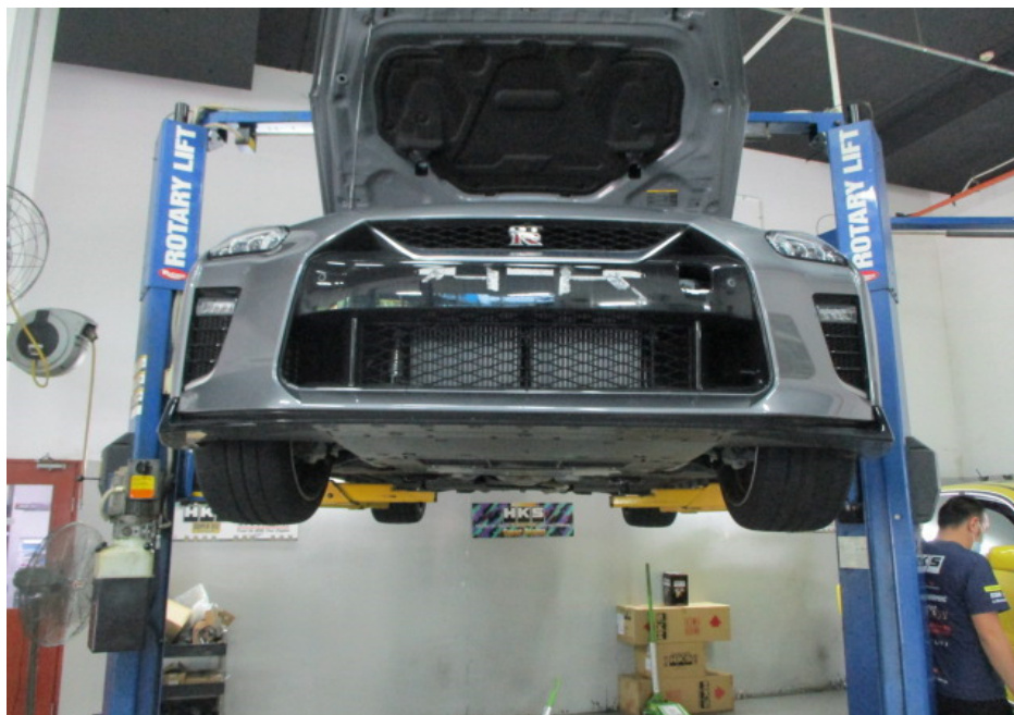
Photo 16 shows the Motor Car hoisted up for checks on its undercarriage. There was no sign(s) or indication(s) of fluid leakage and/or fluid stain(s) on the underside of the Motor Car. The undercarriage components of the Motor Car were also all observed to be intact and secured in an appropriate manner.
