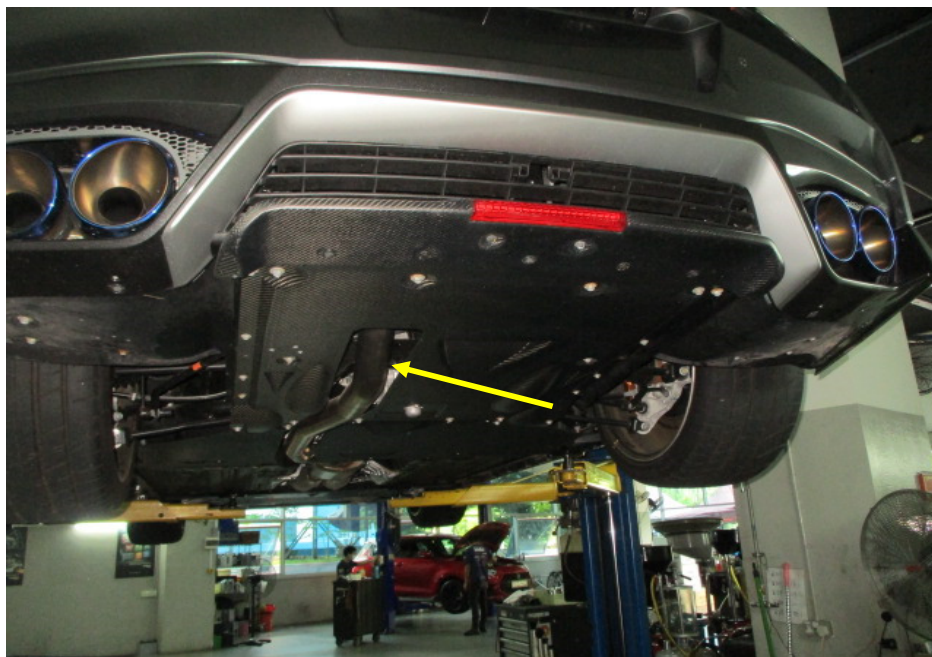
Photo 20 shows a general view of the rear section of the Motor Car's exhaust system. My examination of the Motor Car's exhaust system revealed no sign(s) or indication(s) of any cut or weld marks along its exhaust pipes (arrowed), on its catalytic converters, centre resonator box and its rear mufflers.
