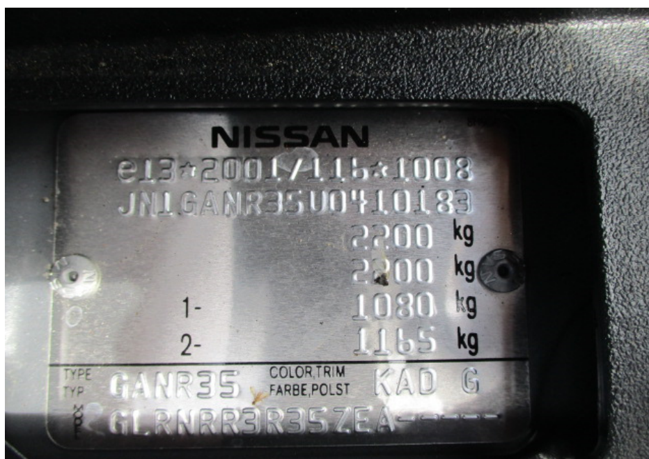
Photo 11 shows the chassis number of the Motor Car. The chassis number recorded was JN1GANR35U0410183.
