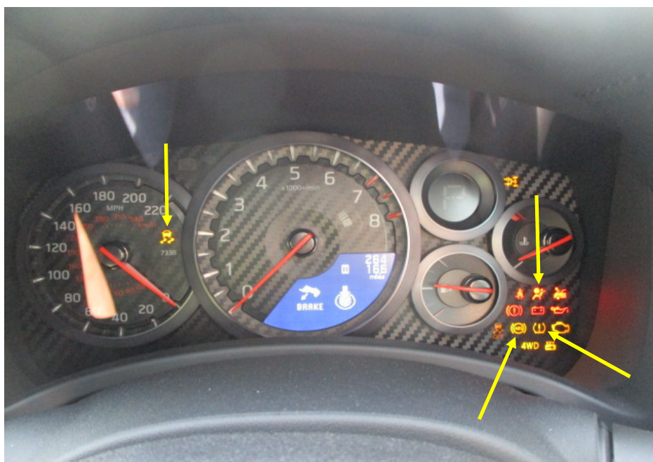
Photo 14 shows the warning lights for the various electronic safety features appearing on the instrument panel of the Motor Car during its self-test when the engine is cranked, in particular the ABS, SRS, TPM and VDC lights (arrowed).
