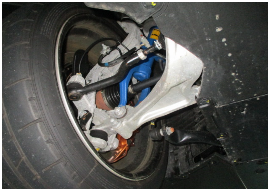
Photo 19 shows the various undercarriage components at the front left wheel of the Motor Car. The mechanical components, control arms and linkages were all found to be intact and secured in an appropriate manner. I also did not observe any fluid leak and/or fluid stain on the underside of the Motor Car.
