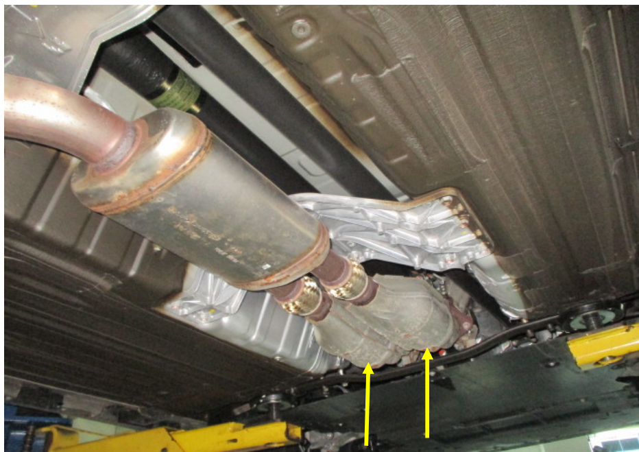
Photo 21 shows the front section of the Motor Car's exhaust system. My examination of the Motor Car's exhaust system revealed no sign(s) or indication(s) of any cut or weld marks along its exhaust pipes, on its catalytic converters (arrowed), centre resonator box and its rear mufflers.
