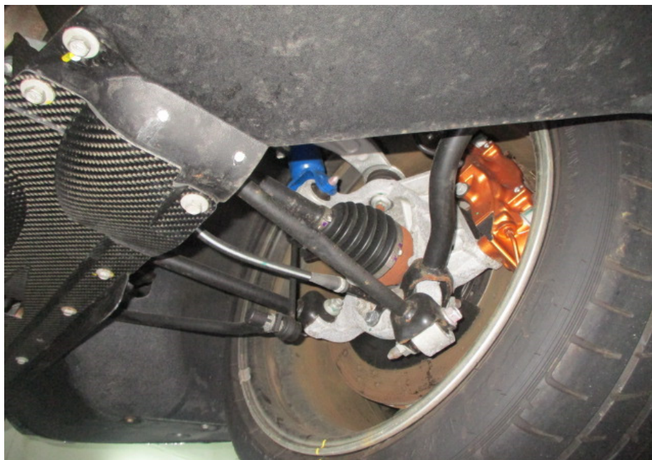
Photo 18 shows the various undercarriage components at the rear left wheel of the Motor Car. The mechanical components, control arms and linkages were all found to be intact and secured in an appropriate manner.
