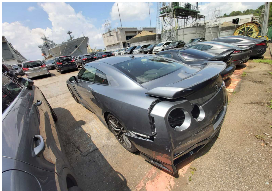
Photo 1 shows the rear left body of the Motor Car (photograph provided to me). The Motor Car was observed to have sustained damage at its rear portion. From the photographs provided, I had observed damage to rear bumper and rear left taillamp amongst others.
