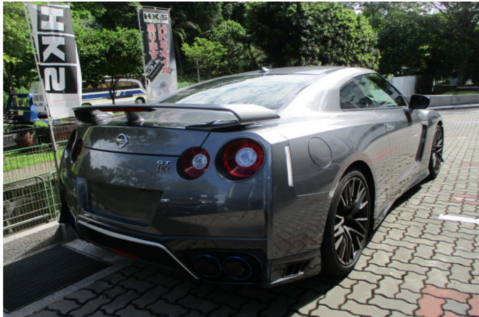
Photo 8 shows a general view of the rear right body of the Motor Car at the time of my inspection. The Motor Car was observed to be in a relatively good general condition with no loose exterior fittings observed. The rear portion of the Motor Car were visually examined, and it was observed that the repair/restoration works carried out to the damaged area of the Motor Car (refer to photograph 1 & 2 above) were reasonably adequate and in order.
