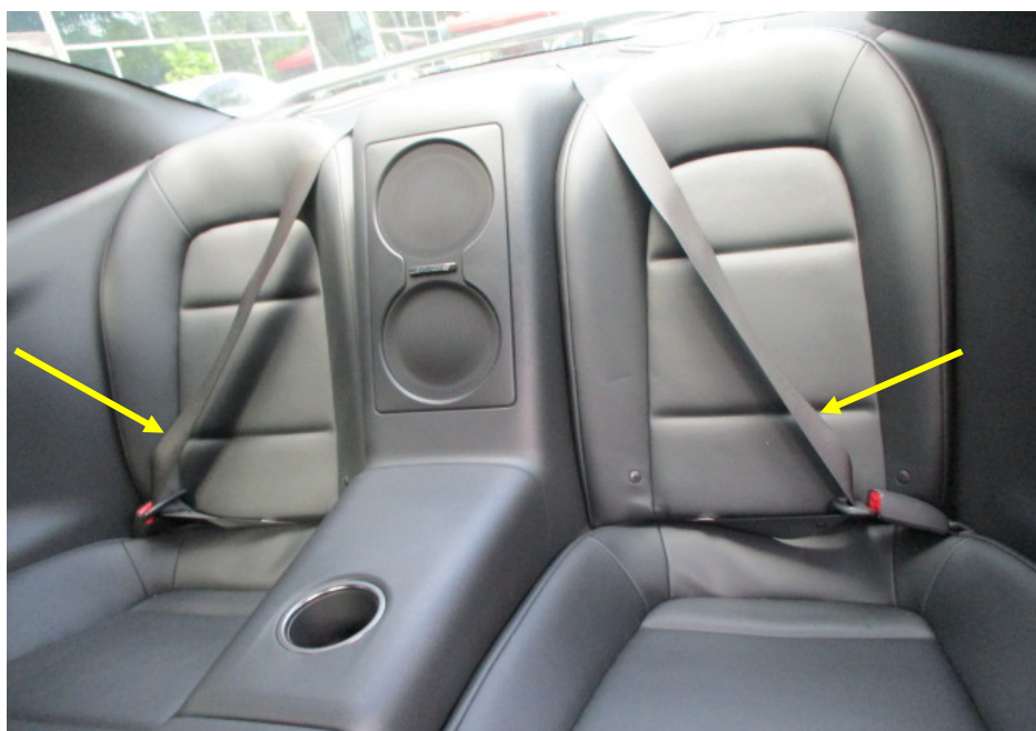
Photo 13 shows the rear seats of the Motor Car. All the seats of the Motor Car were secured via seat rails to the floorboard. They were also fitted with a retractable seat belt reel and a pre-tensioner. The seat belts (arrowed) were tested and were able to be fastened into the respective pre-tensions that were fitted on the side of each individual seat.
