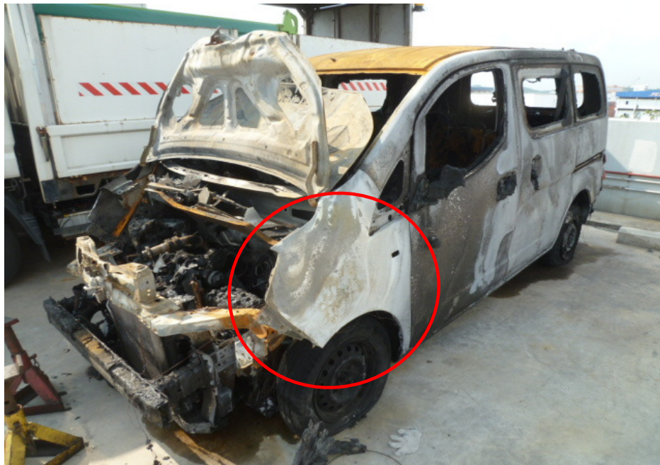
Photo 19 shows the burn pattern and whitish burn marks that were found on the left front fender of the Insured Vehicle (circled). Such whitish burn marks are a result of exposure to prolonged heat intensity, which may indicate where the fire had started.
