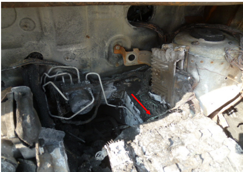
Photo 10 shows a closer view of the burnt wirings leading from the ECM around the left portion of the engine compartment, which is in the immediate vicinity where the fire to the Insured Vehicle had likely started. We noticed greenish residue on several stretches of burnt wirings (arrowed). The presence of greenish residue indicates internal heating of copper wires, a sign of an electrical short circuit occurring. The greenish residue is normally left behind from oxidation as a result of chemical reaction involving the copper wires.
