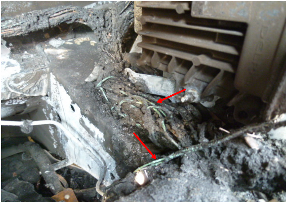
Photo 11 shows a closer view of the greenish residue found on several stretches of burnt wirings leading from the ECM (red arrows). The presence of such greenish residue suggests occurrence of an electrical short circuit.
