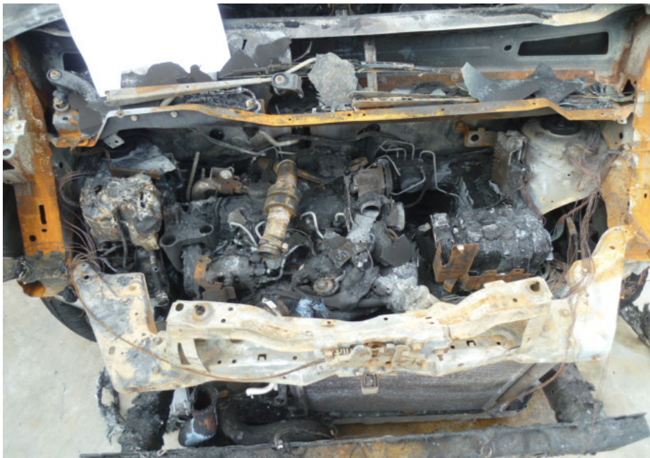
Photo 4 shows the engine compartment of the Insured Vehicle at the time of our inspection. The entire engine compartment of the Insured Vehicle was observed to be severely burnt. Most of the parts inside the engine compartment were found to be burnt and/or melted as a result of the fire.
