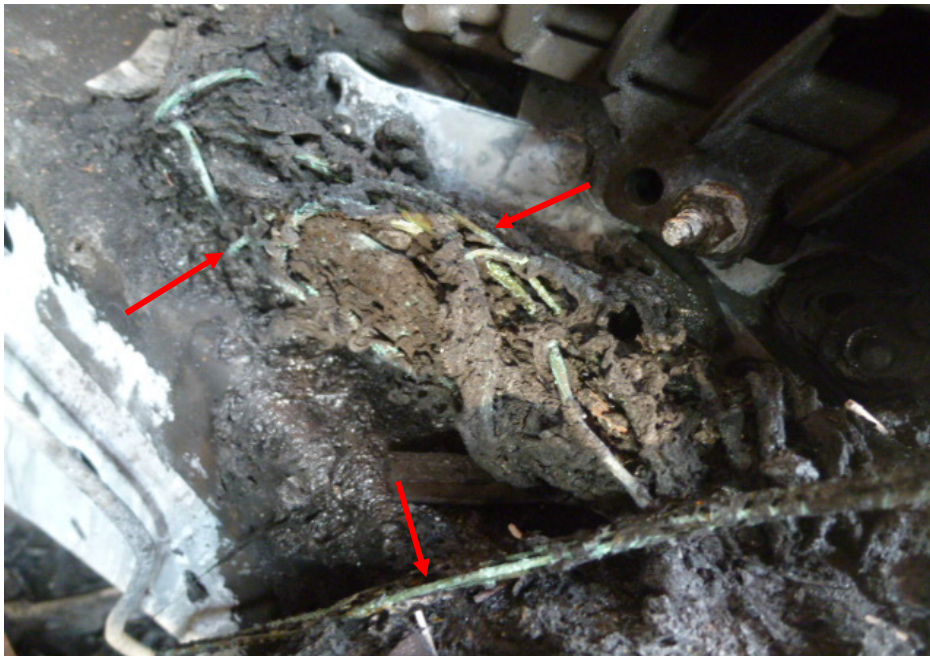
Photo 12 shows a close up view of the greenish residue found on several stretches of burnt wirings leading from the ECM (red arrows). The presence of such greenish residue suggests occurrence of an electrical short circuit.
