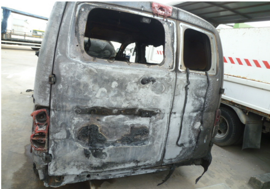
Photo 2 shows the general view of the rear portion of the Insured Vehicle at the time of our inspection. The Insured Vehicle was observed to have sustained extensive fire damage all around. Rust had accumulated all over the Insured Vehicle as a result of exposure to environmental condition for a period of time.
