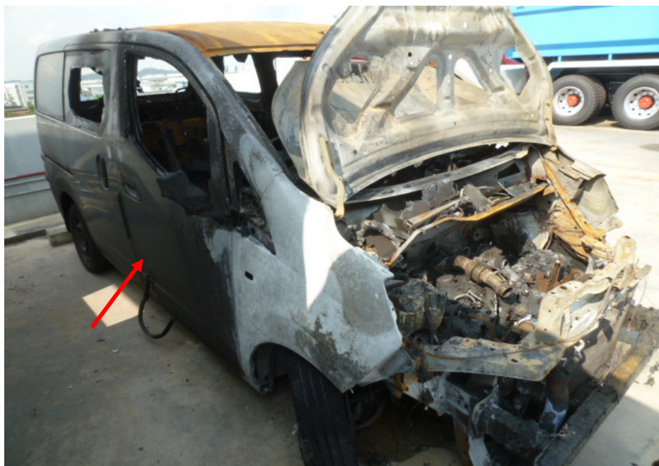
Photo 7 shows the right body of the Insured Vehicle. The nature of the fire damage was less extensive at the right portion (arrowed).
