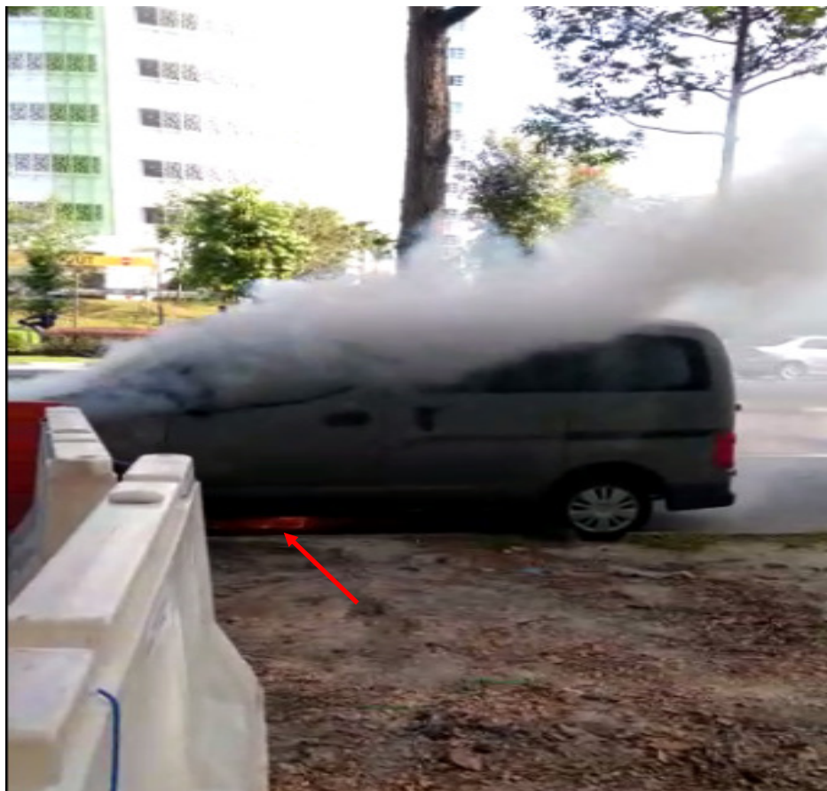
Photo 13 shows the Insured Vehicle on fire before the arrival of the SCDF. In general, the information that could be gathered from this photograph had corresponded to the events that were related to us by Mr Yong which is the fire had started from the left bottom portion of the Insured Vehicle (arrowed).
