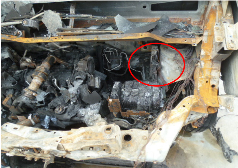
Photo 9 shows the burnt wirings leading from the ECM around the left portion of the engine compartment (circled), which is in the immediate vicinity where the fire to the Insured Vehicle had likely started.
