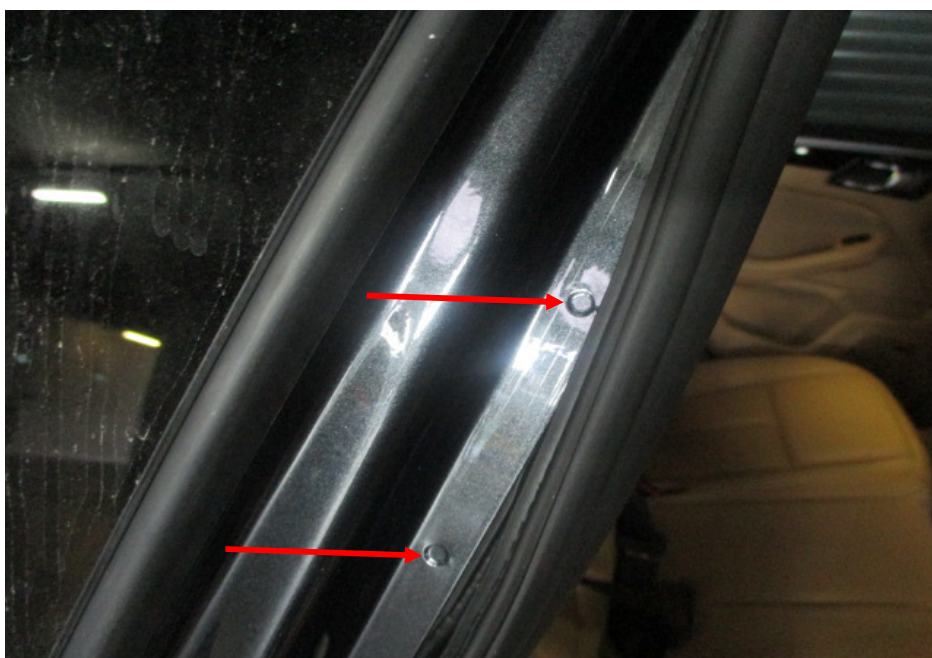
Photo 27 shows the right side "C" pillar of the Motor Car. I did not find any weld marks other than original spot weld marks (arrowed) on the right side "C" pillar of the Motor Car which, indicates that there was no re-welding works carried out. In general, I had found all the non-detachable body panels of the Motor Car to be originally fitted at the time of my inspection.
