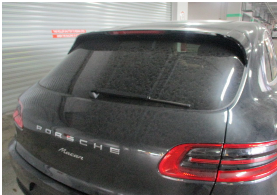
Photo 11 shows a closer view of the Motor Car's rear tailgate, rear tailgate right side lamp, rear right taillamp and rear windscreen. The body parts at the rear portion of the Motor Car were visually examined and it was observed that the repair/restoration works carried out to the damaged area of the Motor Car (refer to photograph 3 above) were reasonably adequate and in order.
