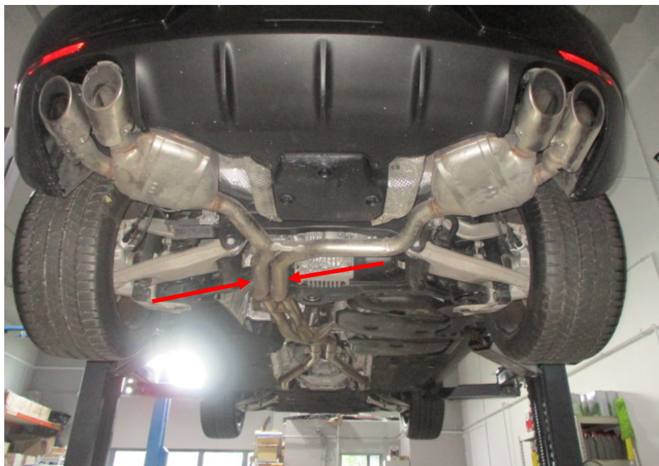
Photo 23 shows a general view of the Motor Car's exhaust system. My examination of the Motor Car's exhaust system revealed no sign(s) or indication(s) of any cut or weld marks along its exhaust pipes (arrowed), on its catalytic converters and on its rear mufflers.
