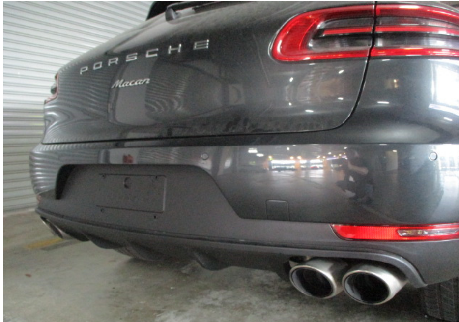
Photo 10 shows a closer view of the Motor Car's rear bumper, rear bumper right reflector, rear bumper lower garnish and rear tailgate. The body parts at the rear portion of the Motor Car were visually examined and it was observed that the repair/restoration works carried out to the damaged area of the Motor Car (refer to photograph 3 above) were reasonably adequate and in order.
