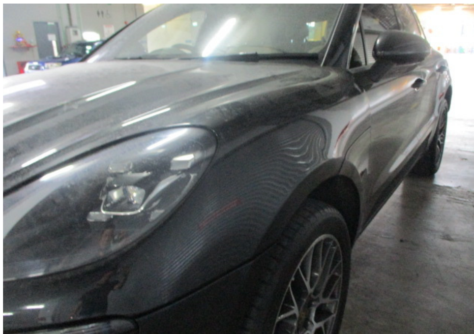
Photo 6 shows a closer view of the Motor Car's front bonnet and front left headlamp. The body parts at the frontal portion of the Motor Car were visually examined and it was observed that the repair/restoration works carried out to the damaged area of the Motor Car (refer to photograph 1 above) were reasonably adequate and in order.
