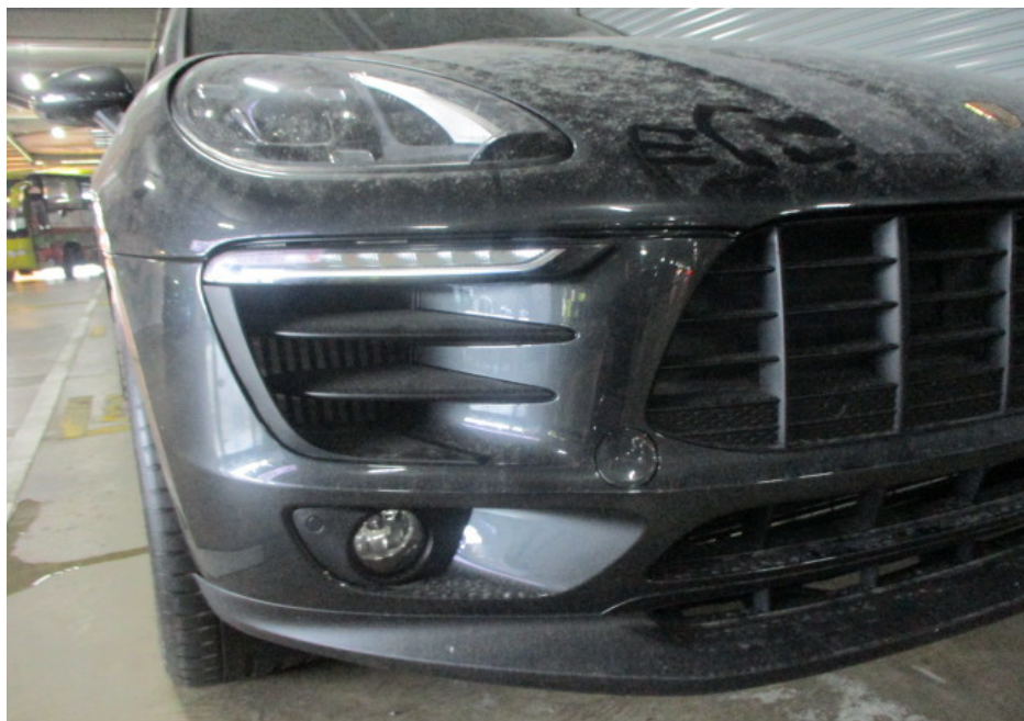
Photo 8 shows a closer view of the Motor Car's front bumper, front bumper right lower grille, front right headlamp, front right day running light, front right fog lamp and front radiator grille. The body parts at the frontal portion of the Motor Car were visually examined and it was observed that the repair/restoration works carried out to the damaged area of the Motor Car (refer to photograph 2 above) were reasonably adequate and in order.
