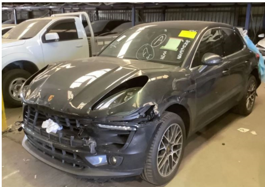
Photo 2 shows the front left body of the Motor Car prior to any repairs being carried out (photograph provided to me). The Motor Car was observed to have sustained damages at its frontal portion. The front bumper, front radiator grille, front left headlamp and front bonnet were amongst the parts that were observed to be damaged. Given the extent of damage seen to the frontal portion, it is likely that the front bumper reinforcement, front support panel, front support panel top garnish and front bonnet lock amongst others, were also damaged.
