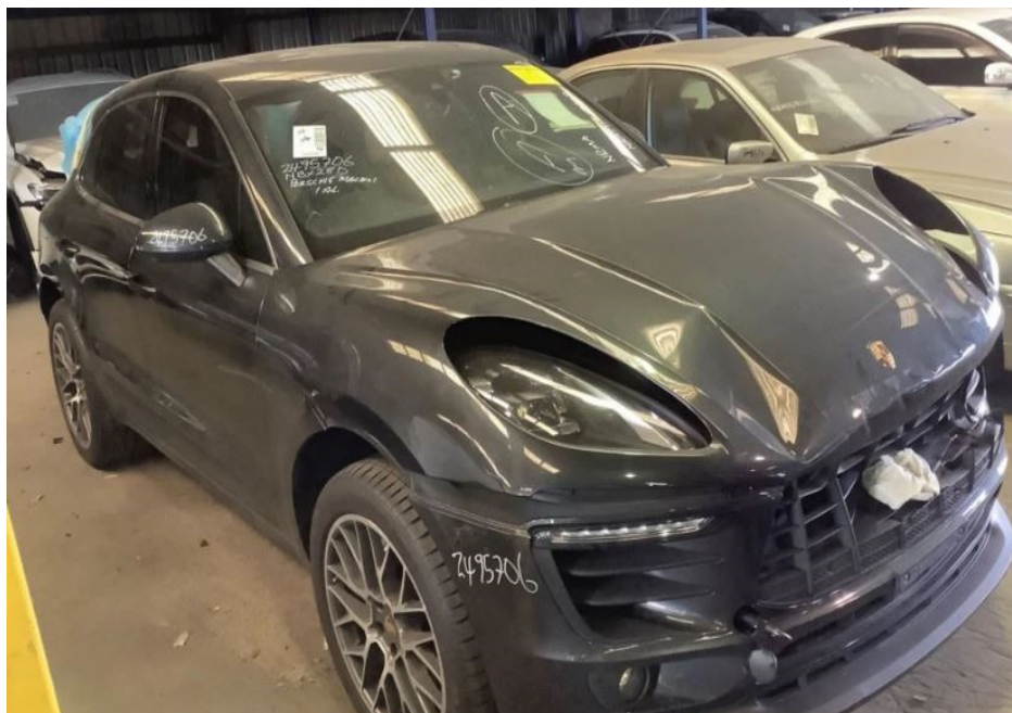
Photo 1 shows the front right body of the Motor Car prior to any repairs being carried out (photograph provided to me). The Motor Car was observed to have sustained damages at its frontal portion. The front bumper, front radiator grille and front bonnet were amongst the parts that were observed to be damaged.
