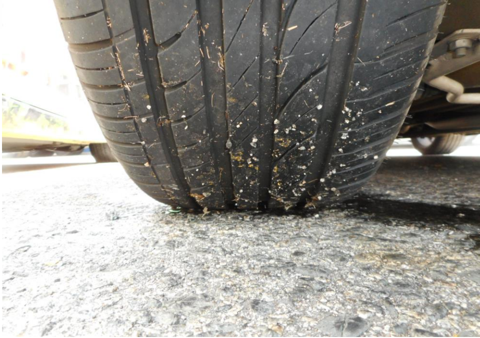
Photo 10 shows the condition of the rear left tyre of the Motor Car, which was observed to be in serviceable condition with remaining tread depth of approximately 6.1mm. The tyre, which was wrapped around steel wheel rim, was also observed to be sufficiently inflated for vehicular operation. The 4 tyres of the Motor Car were wrapped around standard steel wheel rims.
