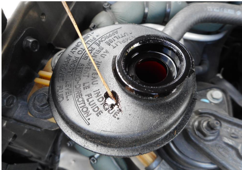
Photo 16 shows the power steering fluid of the Motor Car at the time of my inspection. The steering fluid was observed to be of sufficient level and without any visible contamination.
