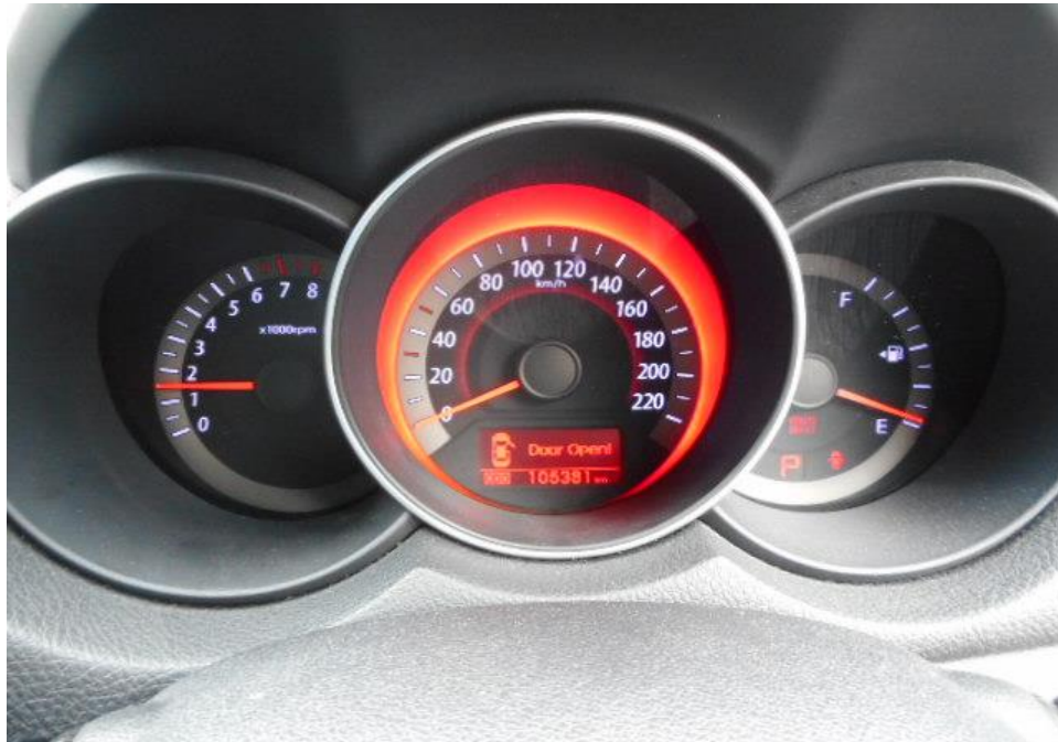
Photo 26 shows no warning lights illuminated on the instrument panel of the Motor Car after the engine was cranked. This would suggest that there was no abnormality to the electronic operating system of the Motor Car, like the ABS, SRS, TCS and etc.
