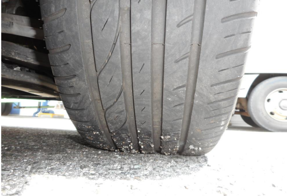
Photo 8 shows the condition of the front right tyre of the Motor Car, which was observed to be in serviceable condition with remaining tread depth of approximately 4.6mm. The tyre was sufficiently inflated for vehicular operation with no tear, cut or burst mark(s) on the outer and the inner sidewalls as well as across the tread. The 4 tyres of the Motor Car were wrapped around standard steel wheel rims without any damage.
