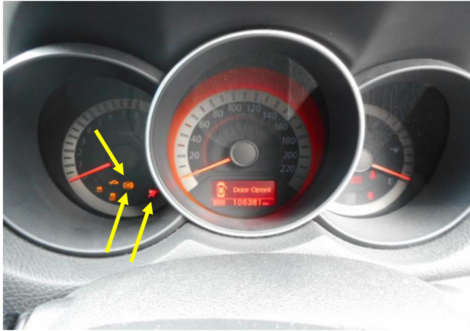
Photo 25 shows the warning light for Anti-Lock Brake System (ABS), Supplemental Restraint System (SRS) and Traction Control System (TCS) (arrowed) appearing on the instrument panel of the Motor Car during the self-test of its various electronic operating systems when its engine was cranked.
