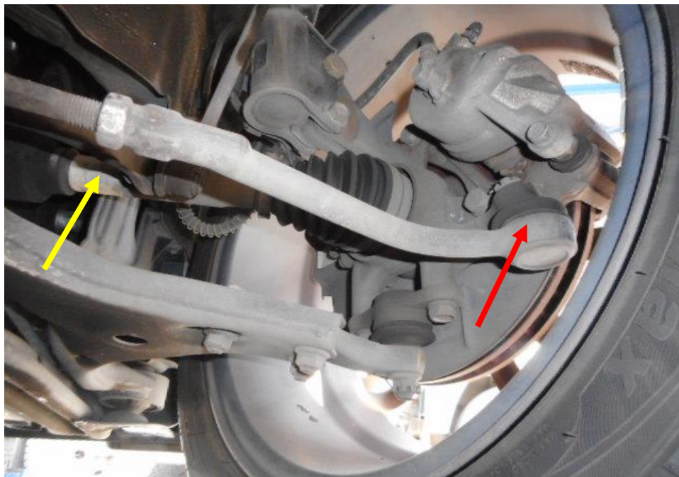
Photo 23 shows the various undercarriage components at the front right wheel of the Motor Car, in particular the steering tie rod (red arrow) and drive shaft (yellow arrow). The various steering components were all found to be intact, suggesting that the steering system of the Motor Car was likely to be in serviceable condition at the material time of accident. There was also no sign of fluid stain observed on the various undercarriage components at the front right wheel of the Motor Car.
