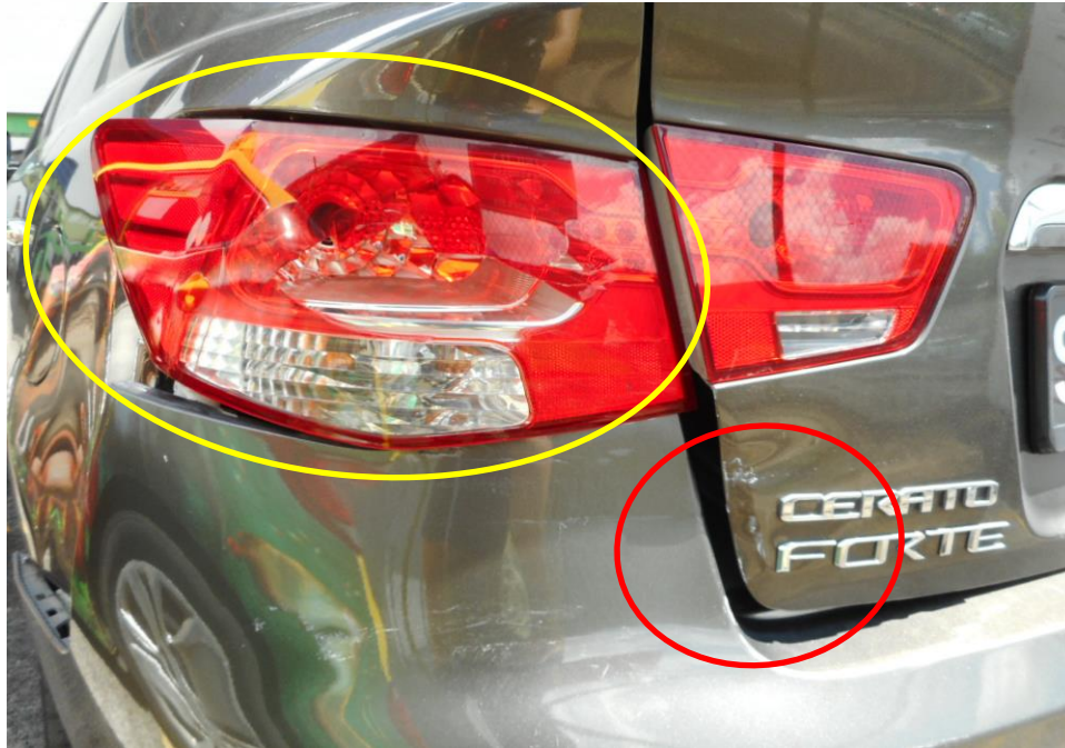
Photo 4 shows a close up view of the Motor Car's rear body at the time of my inspection. The rear portion of the Motor Car was observed to have sustained damage. Its rear left brake lamp (yellow circle) and rear bonnet (red circle) was the body parts that were damaged as a result of the accident.
