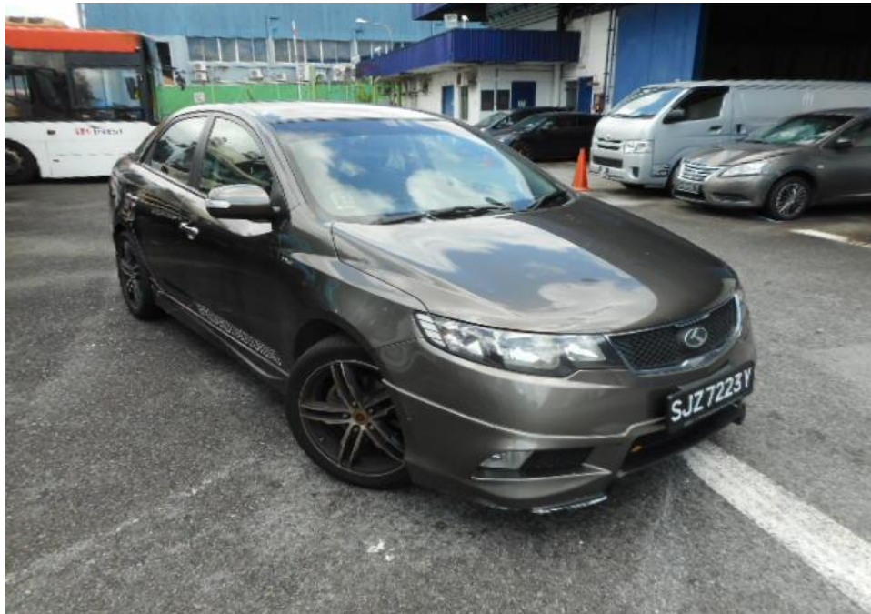
Photo 22 shows the front right wheel of the Motor Car turned to its full left. During my steering system test, I did not experience any abnormal free play and/or resistance when I had turned the steering wheel towards the left and right. This would suggest that the steering system of the Motor Car was likely to be in serviceable condition at the material time of accident.
