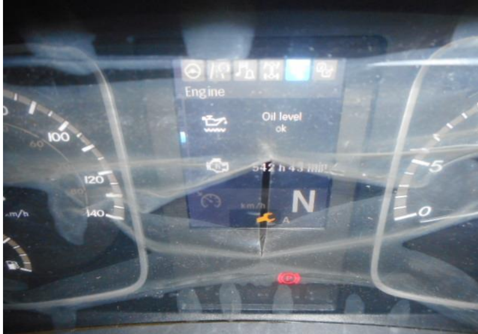
Photo 15 shows the engine oil display of the Police Truck at the time of my inspection. The engine oil was observed to be of sufficient level at the time of our inspection.
