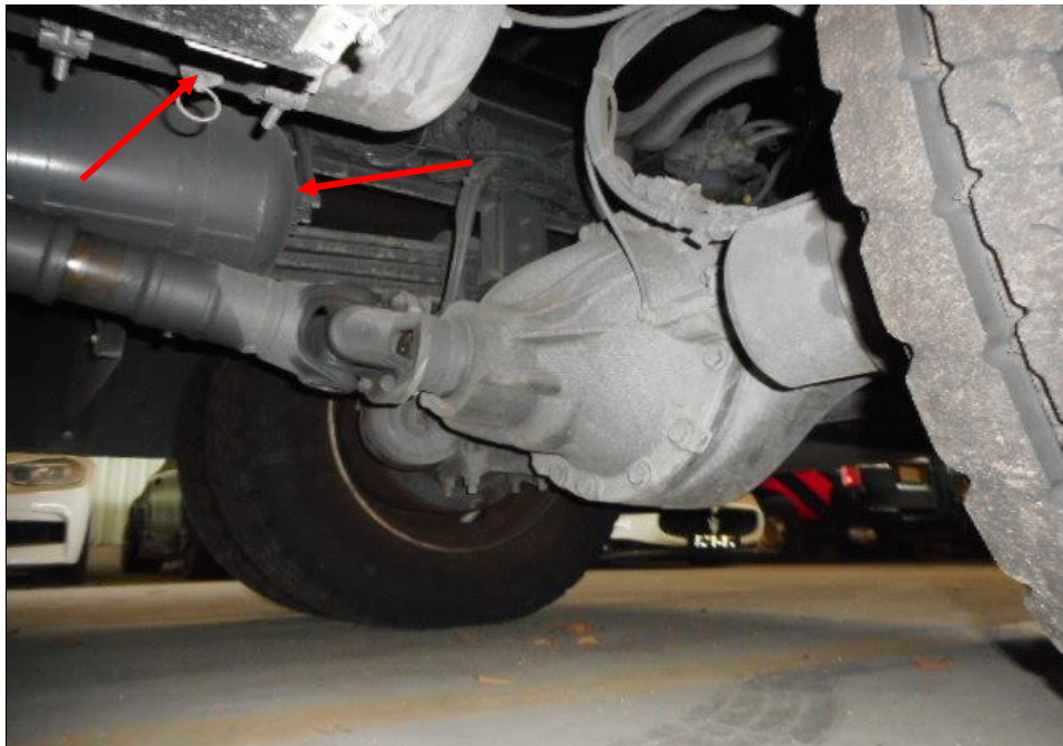
Photo 21 shows the air brake cylinders (arrowed) at the undercarriage of the Police Truck. I did not observe any leakage of air brake fluid at the time of my inspection of the Police Truck. My static tests of the Police Truck's braking system, along with my visual examination of the various mechanical components in the braking system had indicated that there was no internal leakage of pressure/vacuum. Hence the braking system of the Police Truck was likely to be in serviceable condition at the material time of accident.
