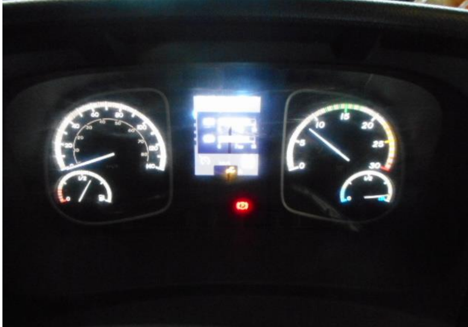
Photo 27 shows no warning lights illuminated on the instrument panel of the Police Truck after the engine was cranked. This would suggest that there was no abnormality to the electronic operating system of the Police Truck, like the ABS and etc.
