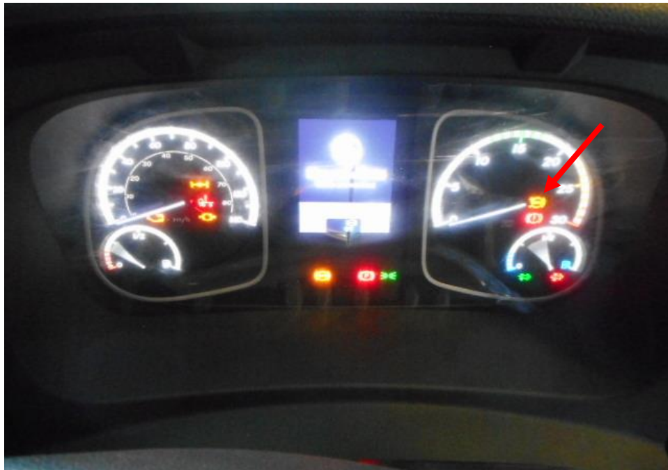
Photo 26 shows the warning light for Anti-Lock Brake System (ABS) (arrowed) appearing on the instrument panel of the Police Truck during the self-test of its various electronic operating systems when its engine was cranked.
