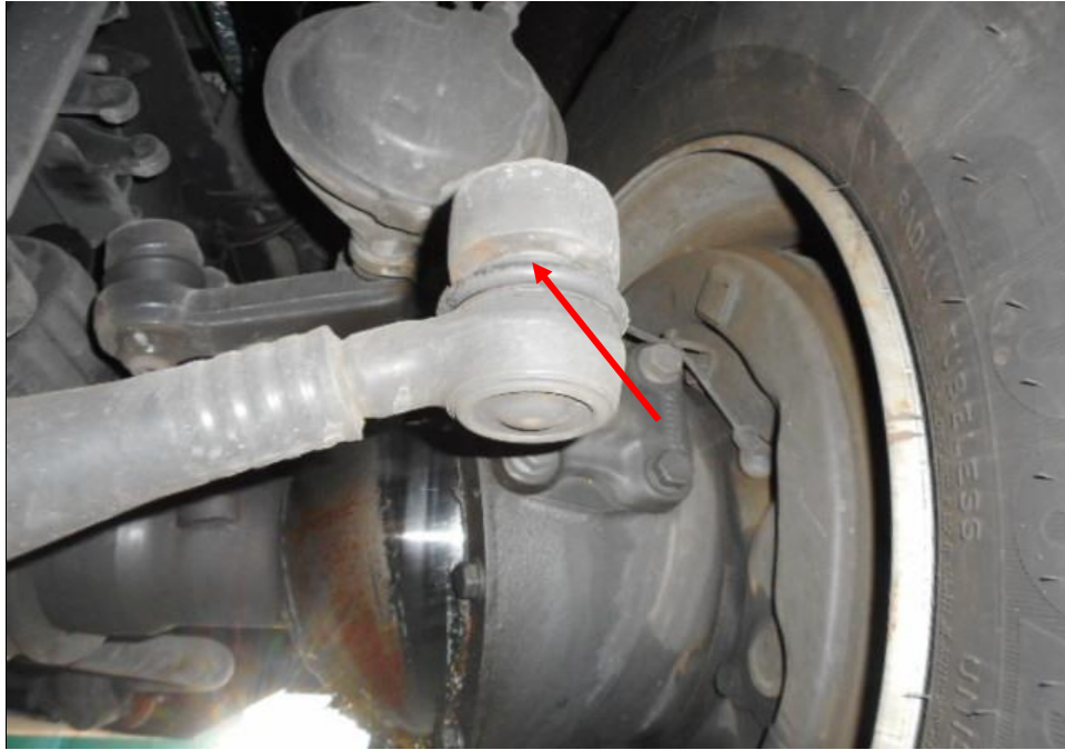
Photo 22 shows the various undercarriage components at the front right wheel of the Police Truck, in particular the steering tie rod end (arrowed). The various steering components were all found to be intact, suggesting that the steering system of the Police Truck was likely to be in serviceable condition at the material time of accident. There was also no sign of fluid stain(s) observed on the various undercarriage components.
