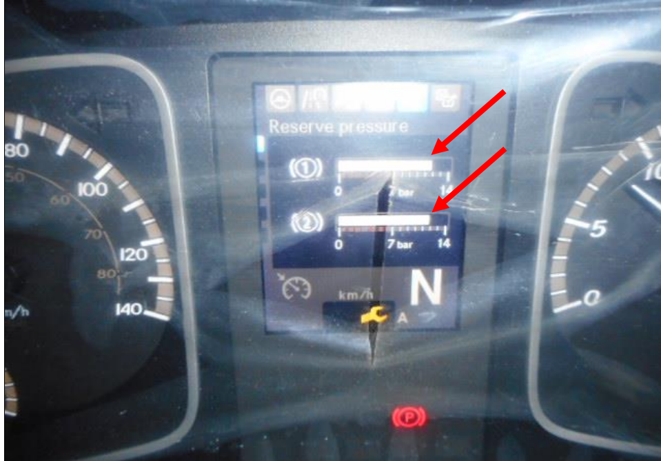
Photo 13 shows the air in the air brake cylinders of the Police Truck at the time of my inspection. The air in the cylinder was observed to be of sufficient level & serviceable at the time of the accident.
