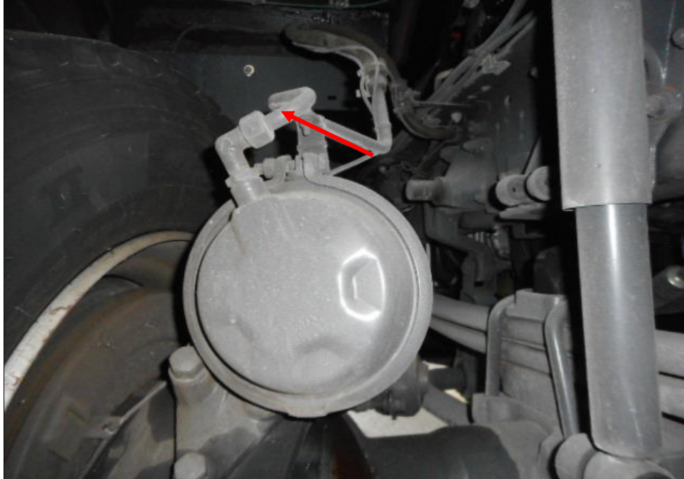
Photo 20 shows the brake pipe (arrowed) at the front left wheel of the Police Truck. I did not observe any leakage of brake fluid at the time of my inspection of the Police Truck. My static tests of the Police Truck's braking system, along with my visual examination of the various mechanical components in the braking system had indicated that there was no internal leakage of pressure/vacuum. Hence the braking system of the Police Truck was likely to be in serviceable condition at the material time of accident.
