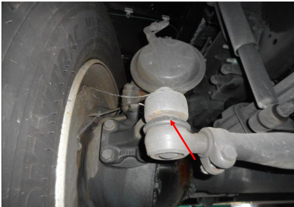
Photo 23 shows the various undercarriage components at the front left wheel of the Police Truck, in particular the steering tie rod end (arrowed). The various undercarriage components of the Police Truck were all found to be intact without any visible damage. There was also no sign of fluid stain(s) observed on the various undercarriage components.
