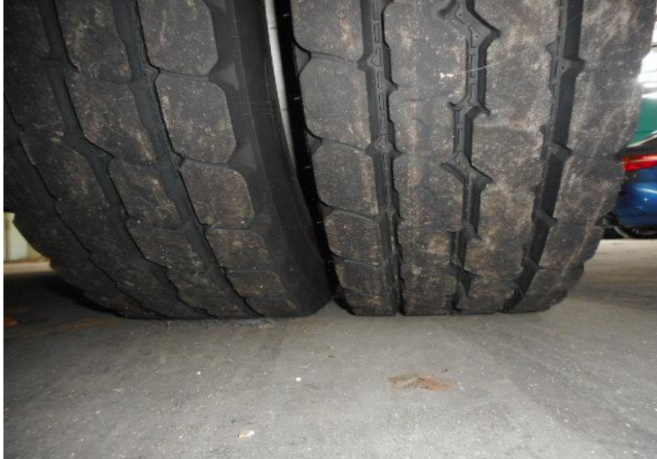
Photo 10 shows the condition of the rear right tyre of the Police Truck, which was observed to be in serviceable condition with remaining tread depth of approximately 14.5mm. The tyre, which was wrapped around standard steel wheel rim, was also observed to be sufficiently inflated for vehicular operation.
