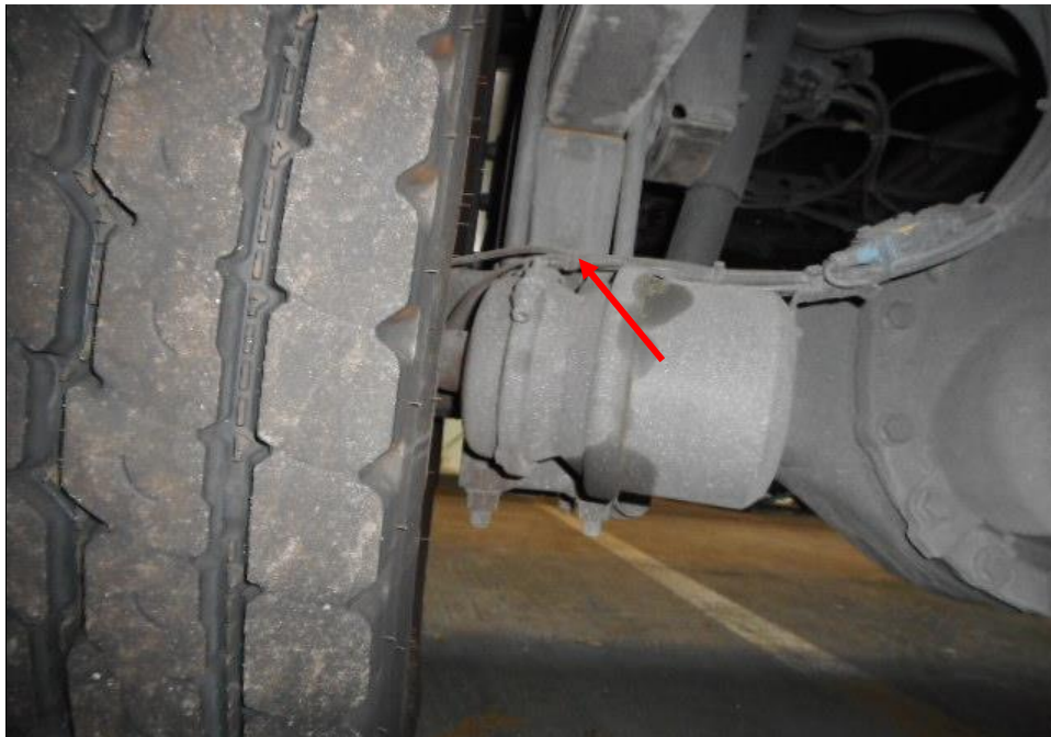
Photo 17 shows the brake pipe (arrowed) at the rear right wheel of the Police Truck. I did not observe any leakage of brake fluid at the time of my inspection of the Police Truck. My static tests of the Police Truck's braking system, along with my visual examination of the various mechanical components in the braking system, had indicated that there was no internal leakage of pressure/vacuum. Hence the braking system of the Police Truck was likely to be in serviceable condition at the material time of accident.
