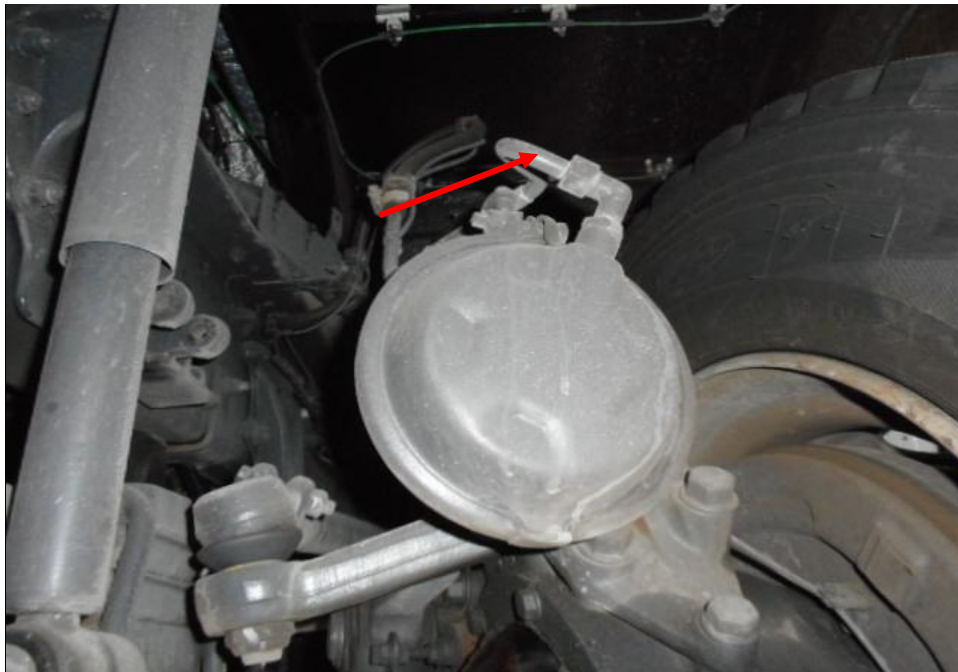
Photo 19 shows the brake pipe (arrowed) at the front right wheel of the Police Truck. I did not observe any leakage of brake fluid at the time of my inspection of the Police Truck. My static tests of the Police Truck's braking system, along with my visual examination of the various mechanical components in the braking system, had indicated that there was no internal leakage of pressure/vacuum. Hence the braking system of the Police Truck was likely to be in serviceable condition at the material time of accident.
