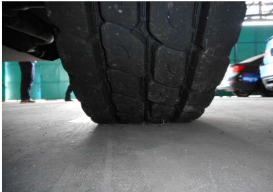
Photo 9 shows the condition of the front right tyre of the Police Truck, which was observed to be in serviceable condition with remaining tread depth of approximately 14.1mm. The tyre, which was wrapped around standard steel wheel rim, was also observed to be sufficiently inflated for vehicular operation. There was no tear, cut or burst mark(s) on the outer and the inner sidewalls as well as across the tread of the 6 tyres that were fitted on the Police Truck.
