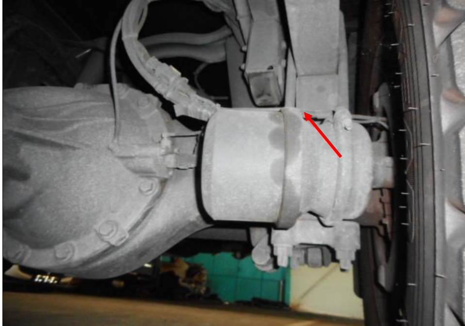
Photo 18 shows the brake pipe (arrowed) at the rear left wheel of the Police Truck. I did not observe any leakage of brake fluid at the time of my inspection of the Police Truck. My static tests of the Police Truck's braking system, along with my visual examination of the various mechanical components in the braking system, had indicated that there was no internal leakage of pressure/vacuum. Hence the braking system of the Police Truck was likely to be in serviceable condition at the material time of accident.
