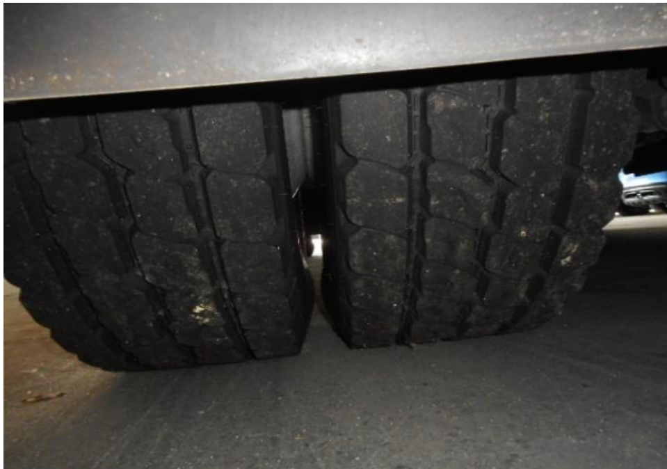
Photo 11 shows the condition of the rear left tyres of the Police Truck, which was observed to be in serviceable condition with remaining tread depth of approximately 14.2mm. The tyres, which were wrapped around standard steel wheel rim, were also observed to be sufficiently inflated for vehicular operation. There was also no damage found on all 6 steel wheel rims of the Police Truck.
