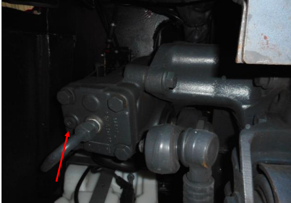
Photo 24 shows the steering box component (arrowed) at the undercarriage of the Police Truck was found to be intact without any visible damage. There was also no sign of fluid stain(s) observed on the various undercarriage components.
