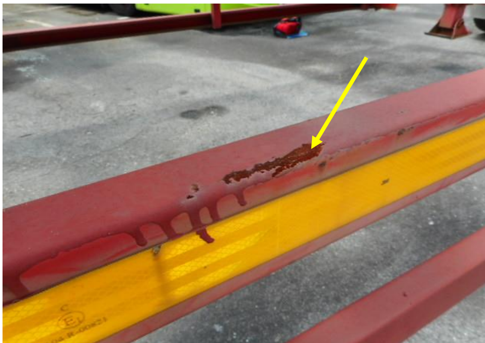
Photo 10 shows a close up view of the trailer's right body at the time of my inspection. The Motor Truck was observed to sustain damaged on its Trailer's right portion. Its right body panel (arrowed) was damaged at the time of my inspection.
