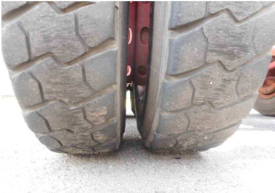
Photo 16 shows the condition of the right tyres of the trailer, which was observed to be in serviceable condition with remaining, tread depth of approximately 7.1mm. There was also no tear, cut or burst mark(s) on the outer and the inner sidewalls as well as across the tread of the 8 tyres that were fitted on the trailer.
