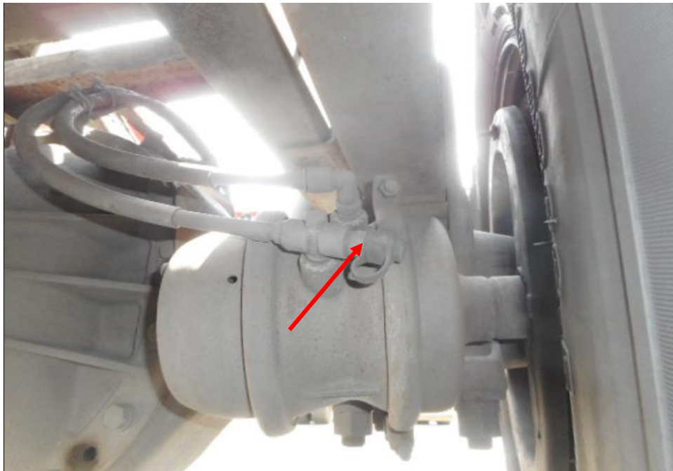
Photo 25 shows the brake pipe (arrowed) at the rear left wheel of the Motor Truck. I did not observe any leakage of brake fluid at the time of my inspection of the Motor Truck. My static tests of the Motor Truck's braking system, along with my visual examination of the various mechanical components in the braking system, had indicated that there was no internal leakage of pressure/vacuum. Hence the braking system of the Motor Truck was likely to be in serviceable condition at the material time of accident.
