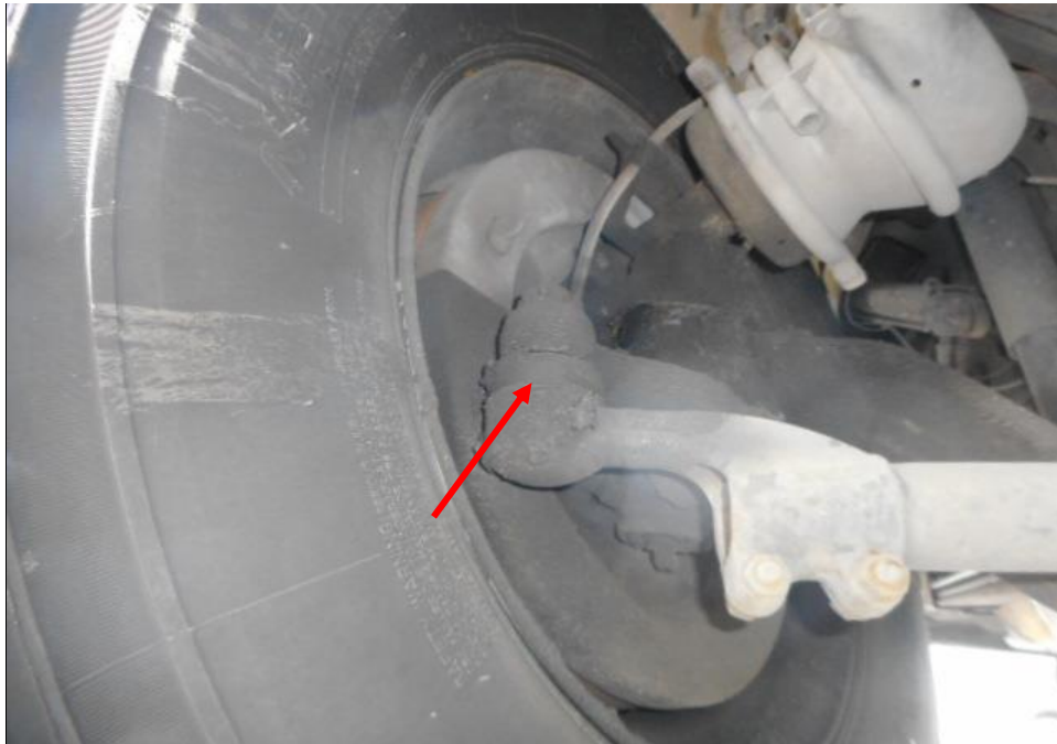
Photo 30 shows the various undercarriage components at the front left wheel of the Motor Truck, in particular the steering tie rod end (arrowed). The various undercarriage components of the Motor Truck were all found to be intact without any visible damage. There was also no sign of fluid stain(s) observed on the various undercarriage components.
