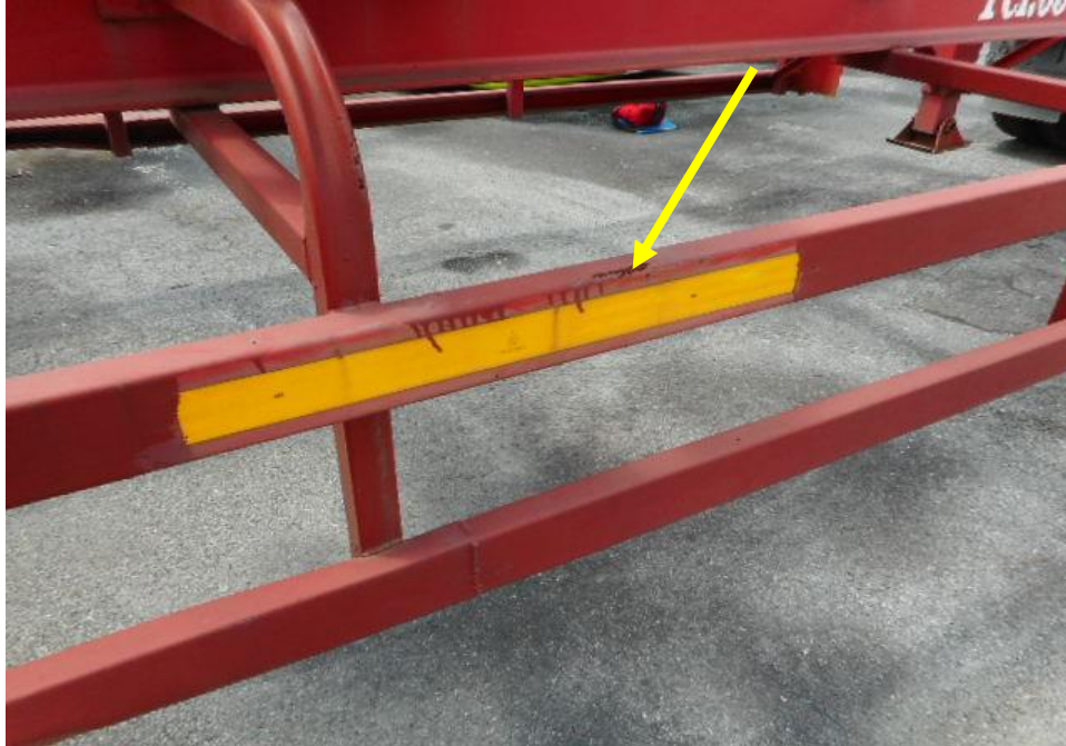
Photo 9 shows a close up view of the trailer's right body at the time of my inspection. The Motor Truck was observed to sustain damaged on its Trailer's right portion. Its right body panel (arrowed) was damaged at the time of my inspection.
