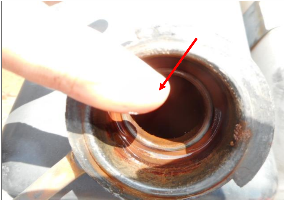
Photo 20 shows the engine coolant reservoir of the Motor Truck at the time of my inspection. The engine coolant was observed to be of sufficient level (arrowed) and without any visible contamination.
