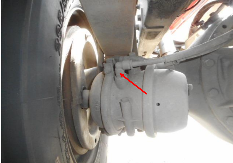
Photo 24 shows the brake pipe (arrowed) at the rear right wheel of the Motor Truck. I did not observe any leakage of brake fluid at the time of my inspection of the Motor Truck. My static tests of the Motor Truck's braking system, along with my visual examination of the various mechanical components in the braking system, had indicated that there was no internal leakage of pressure/vacuum. Hence the braking system of the Motor Truck was likely to be in serviceable condition at the material time of accident.
