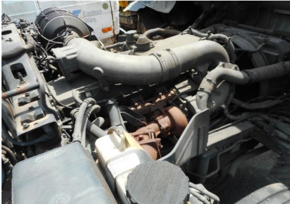
Photo 18 shows a general view of the Motor Truck's engine compartment, which was accessed by lifting the front cabin of the Motor Truck. The various parts and components inside the engine compartment were unaffected by the accident. There was also no sign(s) or indication(s) of fresh fluid leakage and/or fluid stain within the engine compartment
