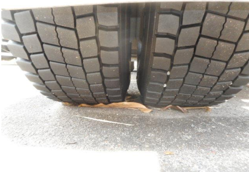
Photo 14 shows the condition of the rear left tyres of the Motor Truck, which was observed to be in serviceable condition with remaining tread depth of approximately 13.7mm. The tyres, which were wrapped around standard steel wheel rim, were also observed to be sufficiently inflated for vehicular operation. There was also no damage found on all 6 steel wheel rims of the Motor Truck.
