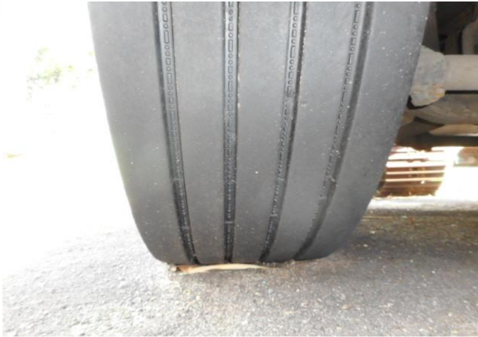
Photo 15 shows the condition of the front left tyres of the Motor Truck, which were observed to be in serviceable condition with remaining tread depth of approximately 9.4mm. There was also no tear, cut or burst mark(s) on the outer and the inner sidewalls as well as across the tread of the 6 tyres that were fitted on the Motor Truck.
