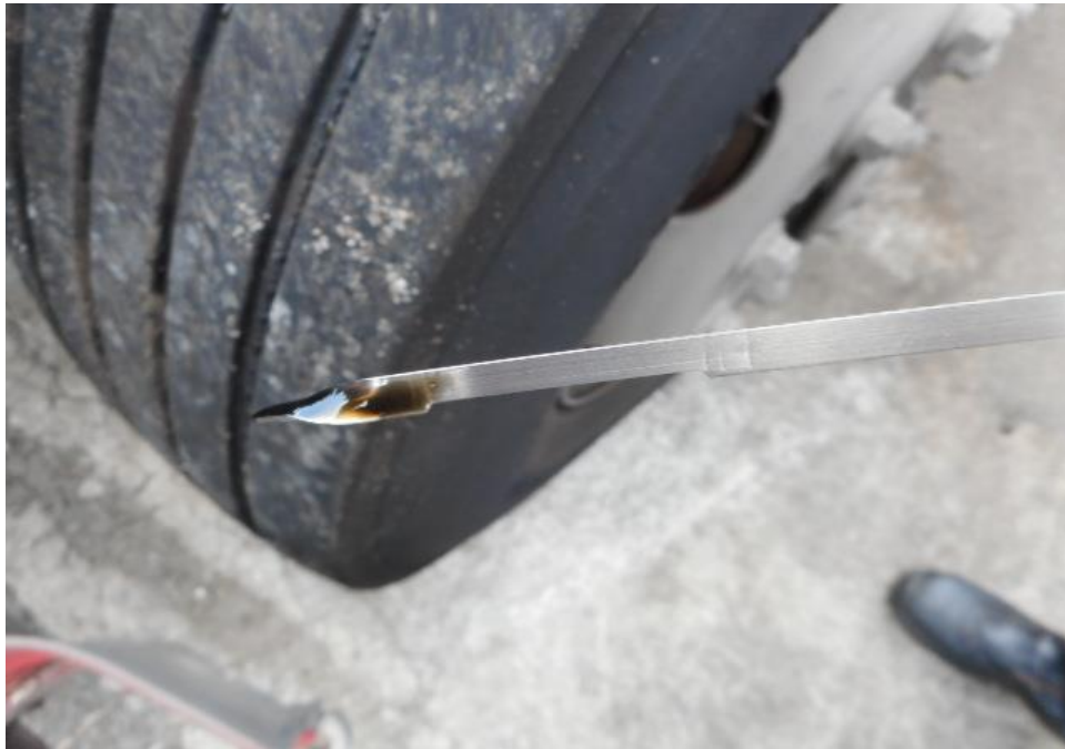
Photo 22 shows the engine oil dip stick of the Motor Truck at the time of my inspection. The engine oil was observed to be of insufficient level at the time of our inspection.
