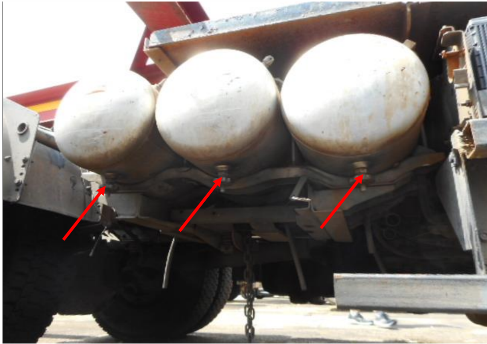
Photo 28 shows the air brake cylinders (arrowed) at the undercarriage of the Motor Truck. I did not observe any leakage of air brake fluid at the time of my inspection of the Motor Truck. My static tests of the Motor Truck's braking system, along with my visual examination of the various mechanical components in the braking system had indicated that there was no internal leakage of pressure/vacuum. Hence the braking system of the Motor Truck was likely to be in serviceable condition at the material time of accident.
