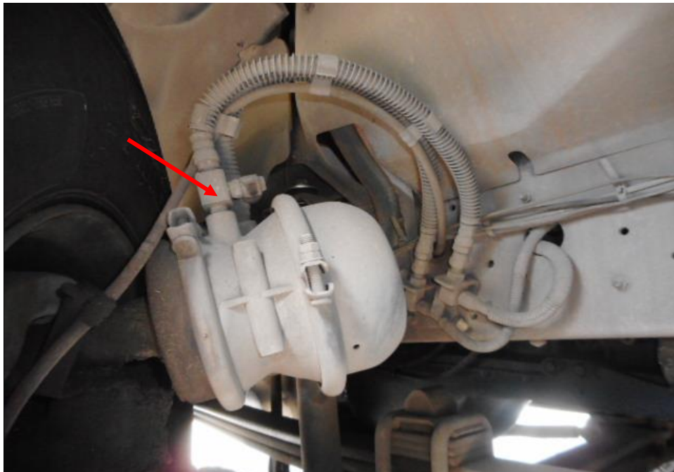
Photo 27 shows the brake pipe (arrowed) at the front left wheel of the Motor Truck. I did not observe any leakage of brake fluid at the time of my inspection of the Motor Truck. My static tests of the Motor Truck's braking system, along with my visual examination of the various mechanical components in the braking system had indicated that there was no internal leakage of pressure/vacuum. Hence the braking system of the Motor Truck was likely to be in serviceable condition at the material time of accident.
