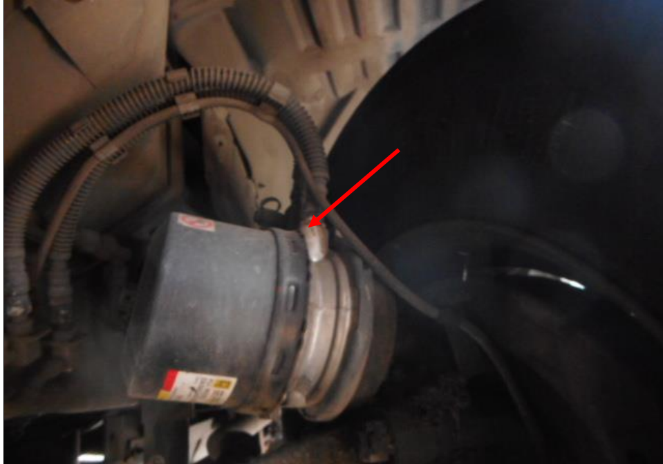
Photo 26 shows the brake pipe (arrowed) at the front right wheel of the Motor Truck. I did not observe any leakage of brake fluid at the time of my inspection of the Motor Truck. My static tests of the Motor Truck's braking system, along with my visual examination of the various mechanical components in the braking system, had indicated that there was no internal leakage of pressure/vacuum. Hence the braking system of the Motor Truck was likely to be in serviceable condition at the material time of accident.
