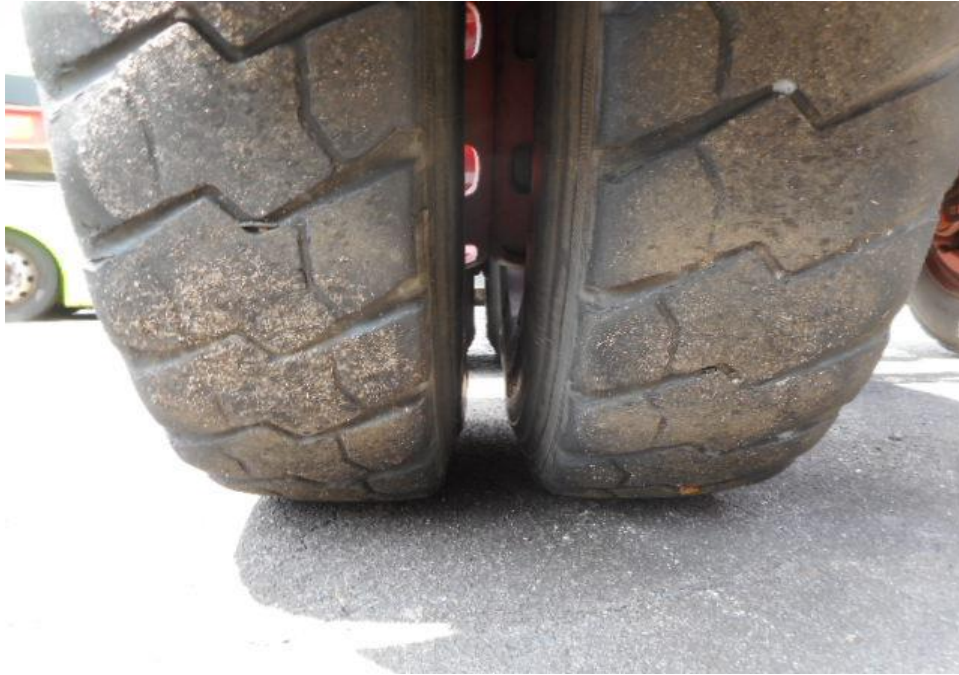
Photo 17 shows the condition of the left tyres of the trailer, which was observed to be in serviceable condition with remaining tread depth of approximately 4.2mm. There was also no tear, cut or burst mark(s) on the outer and the inner sidewalls as well as across the tread of the 8 tyres that were fitted on the trailer.
