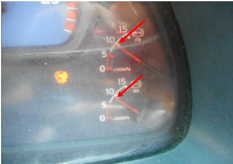
Photo 19 shows the air in the air brake cylinders of the Motor Truck at the time of my inspection. The air in the cylinder was observed to be of sufficient level & serviceable at the time of the accident.
