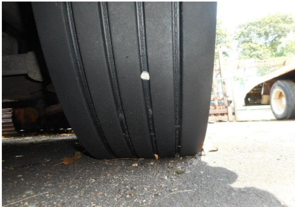
Photo 12 shows the condition of the front right tyre of the Motor Truck, which was observed to be in serviceable condition with remaining tread depth of approximately 9.2mm. The tyre, which was wrapped around standard steel wheel rim, was also observed to be sufficiently inflated for vehicular operation. There was no tear, cut or burst mark(s) on the outer and the inner sidewalls as well as across the tread of the 6 tyres that were fitted on the Motor Truck.
