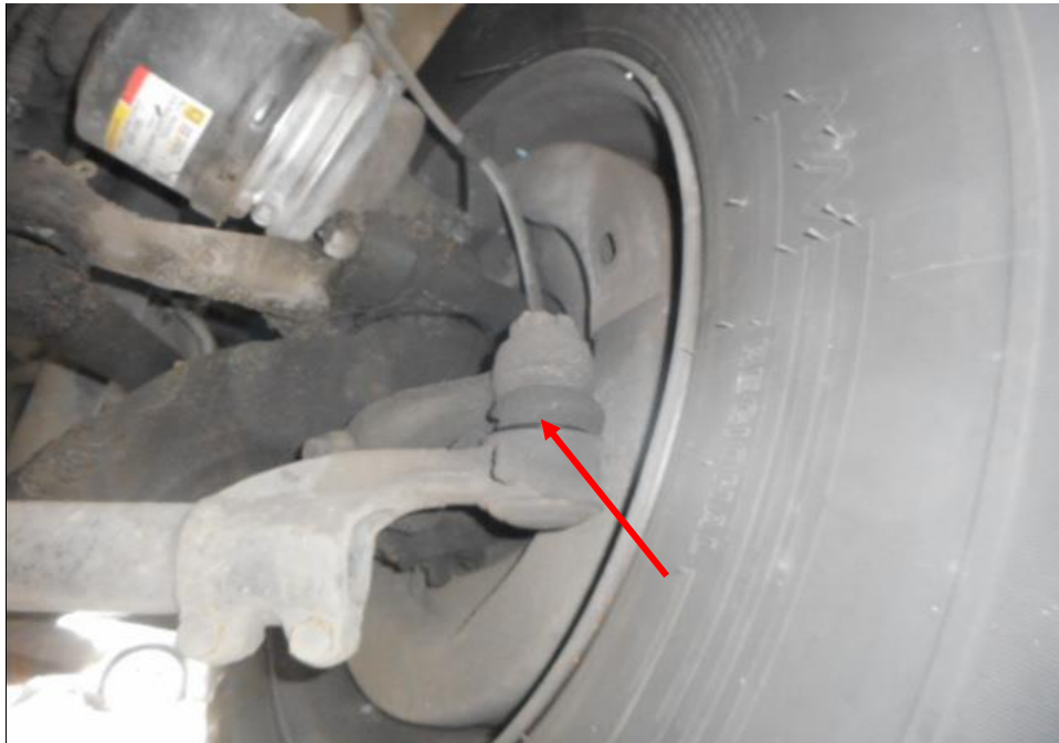
Photo 29 shows the various undercarriage components at the front right wheel of the Motor Truck, in particular the steering tie rod end (arrowed). The various steering components were all found to be intact, suggesting that the steering system of the Motor Truck was likely to be in serviceable condition at the material time of accident. There was also no sign of fluid stain(s) observed on the various undercarriage components.
