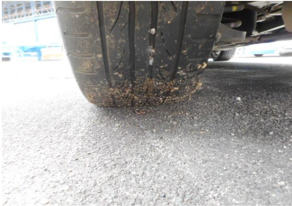
Photo 8 shows the condition of the rear left tyres of the Motor Car, which was observed to be in serviceable condition with remaining tread depth of approximately 3.7mm. The tyres, which were wrapped around standard alloy wheel rim, were also observed to be sufficiently inflated for vehicular operation. There was also no damage found on all 4 alloy wheel rims of the Motor Car.
