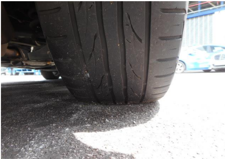
Photo 7 shows the condition of the rear right tyre of the Motor Car, which was observed to be in serviceable condition with remaining tread depth of approximately 3.7mm. The tyre, which was wrapped around standard alloy wheel rim, was also observed to be sufficiently inflated for vehicular operation.
