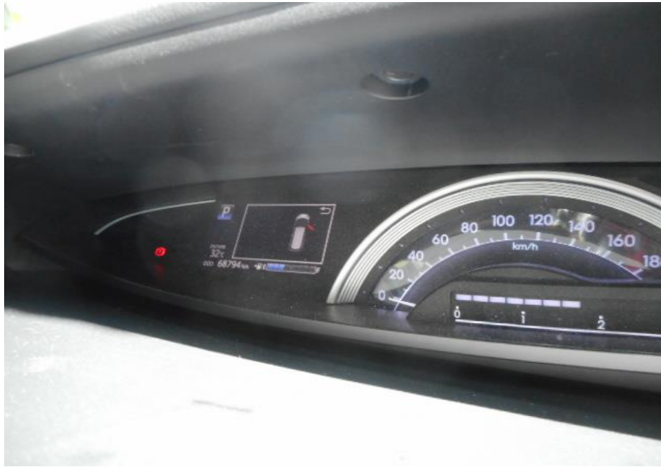
Photo 23 shows no warning lights illuminated on the instrument panel of the Motor Car after the engine was cranked. This would suggest that there was no abnormality to the various electronic operating systems of the Motor Car, like the ABS, TCS, SRS and EPS.
