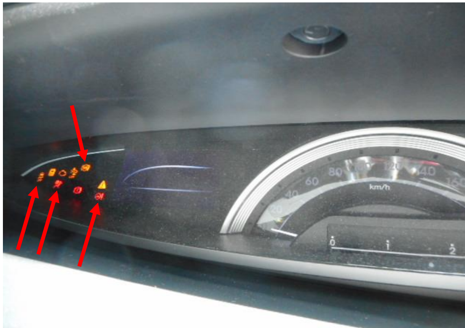
Photo 22 shows the warning light for Anti-Lock Brake System (ABS), Traction Control System (TCS), Supplemental Restraint System (SRS) and Electric Power Steering System (EPS) appearing on the instrument panel of the Motor Car during the self-test of its various electronic operating systems when its engine was cranked.
