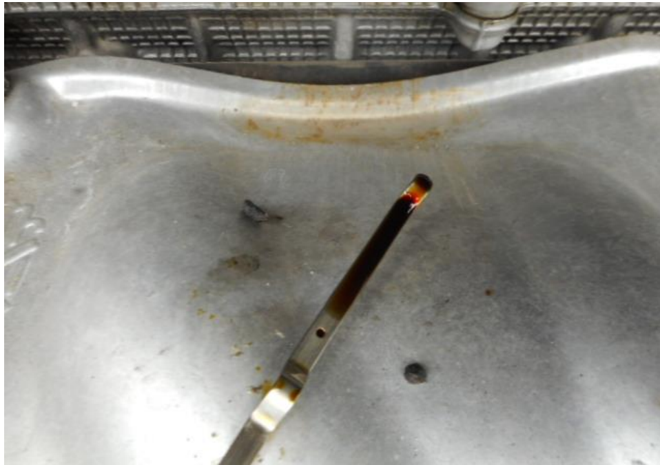
Photo 13 shows the engine oil dip stick of the Motor Car at the time of my inspection. The engine oil was observed to be of sufficient level and without any visible contamination.
