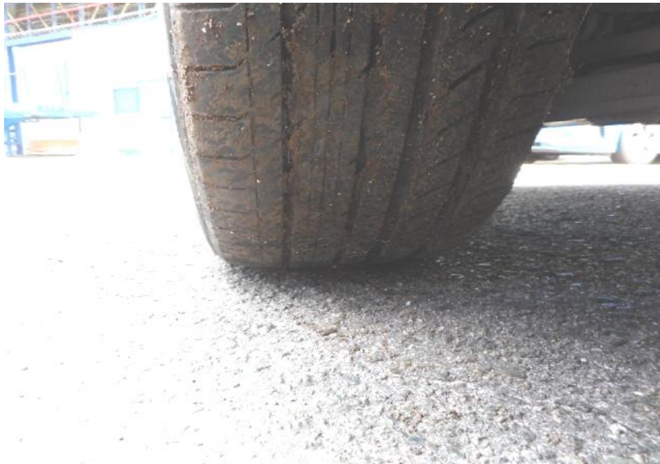
Photo 9 shows the condition of the rear right tyres of the Motor Car, which were observed to be in serviceable condition with remaining, tread depth of approximately 4.5mm. There was also no tear, cut or burst mark(s) on the outer and the inner sidewalls as well as across the tread of the 4 tyres that were fitted on the Motor Car.
