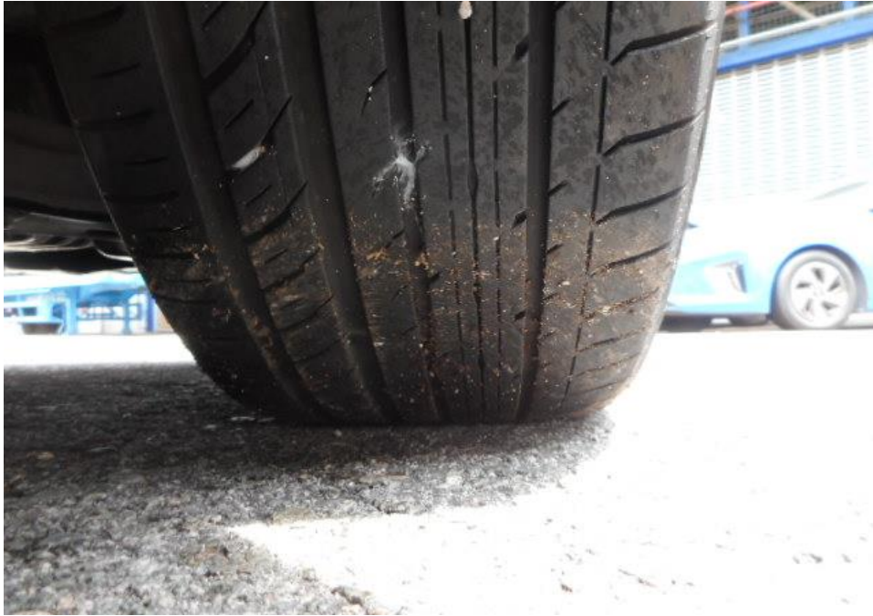
Photo 6 shows the condition of the front right tyre of the Motor Car, which was observed to be in serviceable condition with remaining tread depth of approximately 4.4mm. The tyre, which was wrapped around standard alloy wheel rim, was also observed to be sufficiently inflated for vehicular operation. There was no tear, cut or burst mark(s) on the outer and the inner sidewalls as well as across the tread of the 4 tyres that were fitted on the Motor Car.
