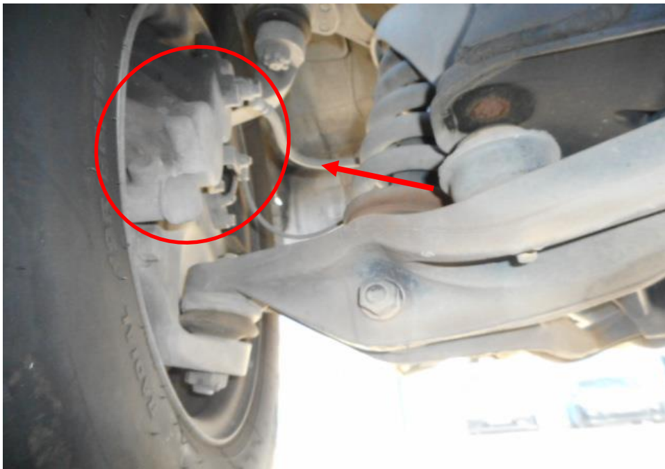
Photo 19 shows the various undercarriage components at the front left wheel of the Motor Lorry, in particular the brake hose (arrowed) and callipers (circled). The various undercarriage components of the Motor Lorry were all found to be intact without any visible damage. There was also no sign of fluid stain(s) observed on the various undercarriage components.
