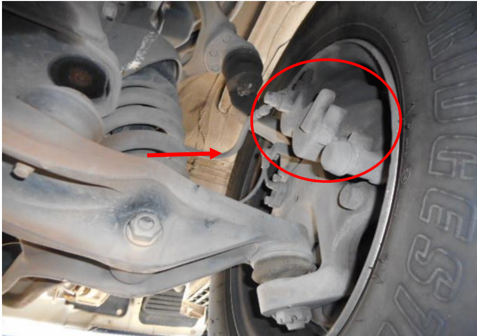
Photo 18 shows the various undercarriage components at the front right wheel of the Motor Lorry, in particular the brake hose (arrowed) and callipers (circled). The various undercarriage components of the Motor Lorry were all found to be intact without any visible damage. There was also no sign of fluid stain(s) observed on the various undercarriage components.
