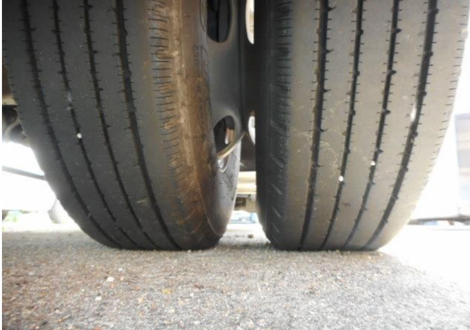
Photo 10 shows the condition of the rear right tyres of the Motor Lorry, which observed to be in serviceable condition with remaining tread depth of approximately 4mm. The tyres, which were wrapped around standard steel wheel rim, were also observed to be sufficiently inflated for vehicular operation.
