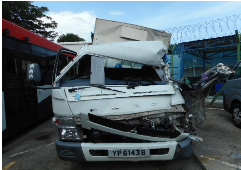
Photo 1 shows a general view of the front windscreen and body panel of the Motor Lorry at the time of our inspection. The Motor Lorry was observed sustained major damages at its front and rear cabin portion as well as its left door as a result of the accident.
