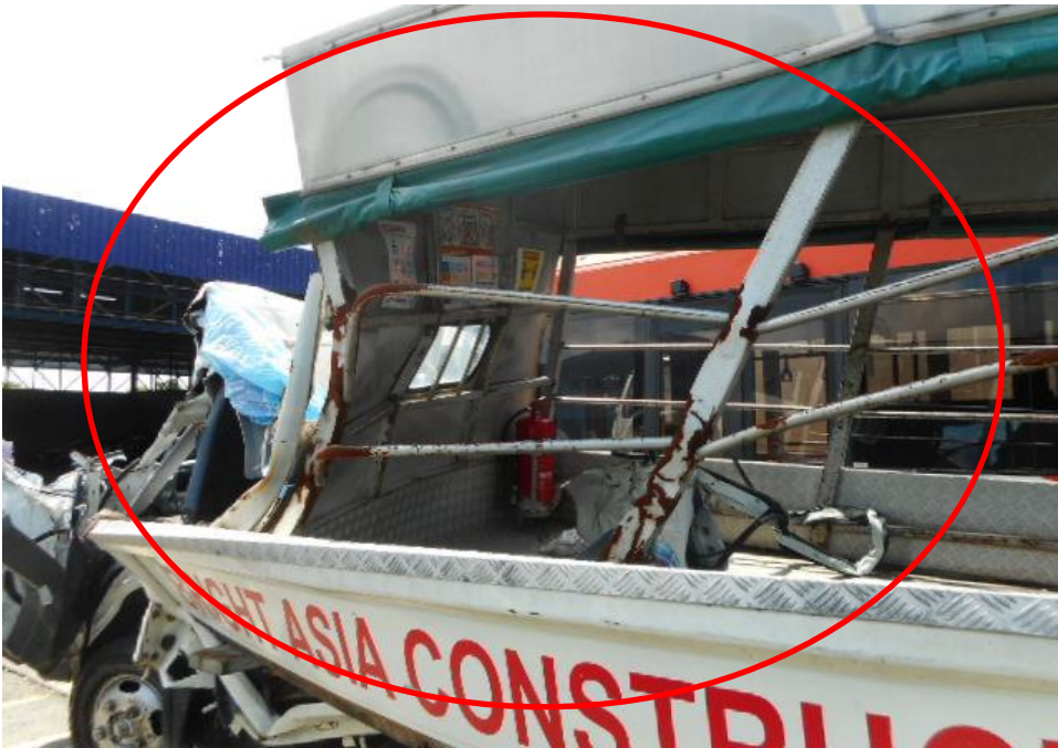
Photo 5 shows a left general view of the rear cabin portion of the Motor Lorry at the time of my inspection, its rear cabin body panel (circled) was observed to have been damaged as a result of the accident's impact.
