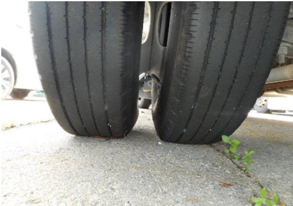
Photo 11 shows the condition of the rear left tyres of the Motor Lorry, which were observed to be in serviceable condition with remaining, tread depth of approximately 2.5mm. See above.
