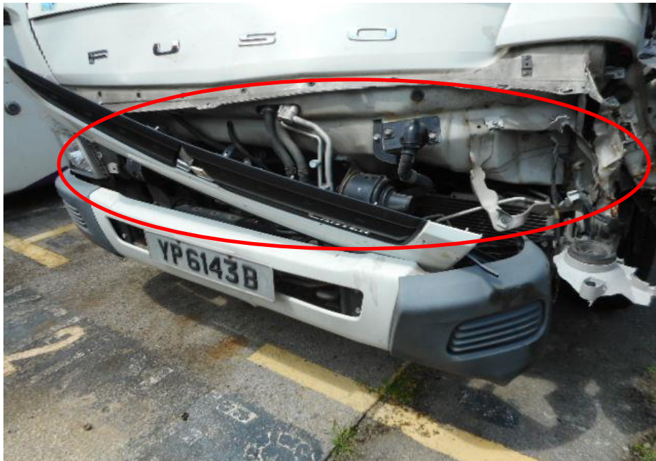
Photo 3 shows the close up view of the front portion of the Motor Lorry at the time of our inspection. The Motor Lorry was observed to have sustained major damages to its front body panel (circled) that was damaged as a result of the accident's impact.
