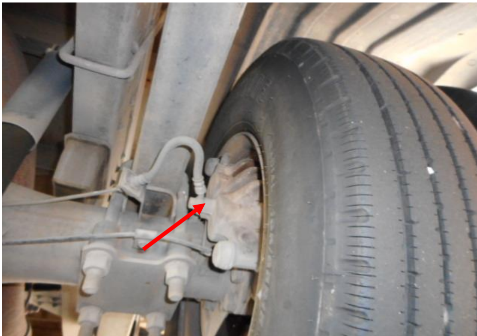
Photo 21 shows the various undercarriage components at the rear right wheel of the Motor Lorry, in particular the brake hose and drum brake (arrowed). The various undercarriage components of the Motor Lorry were all found to be intact without any visible damage. There was also no sign of fluid stain(s) observed on the various undercarriage components.
