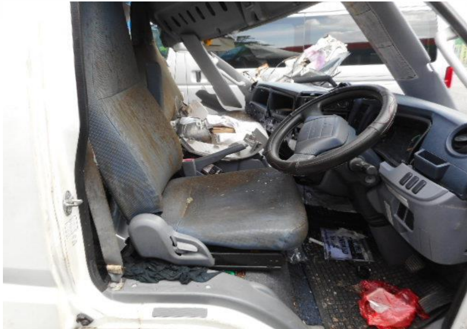
Photo 8 shows the close up view of the front interior cabin of the Motor Lorry. It was observed to have sustained extensive induced damages to the dashboard as a result of the accident.
