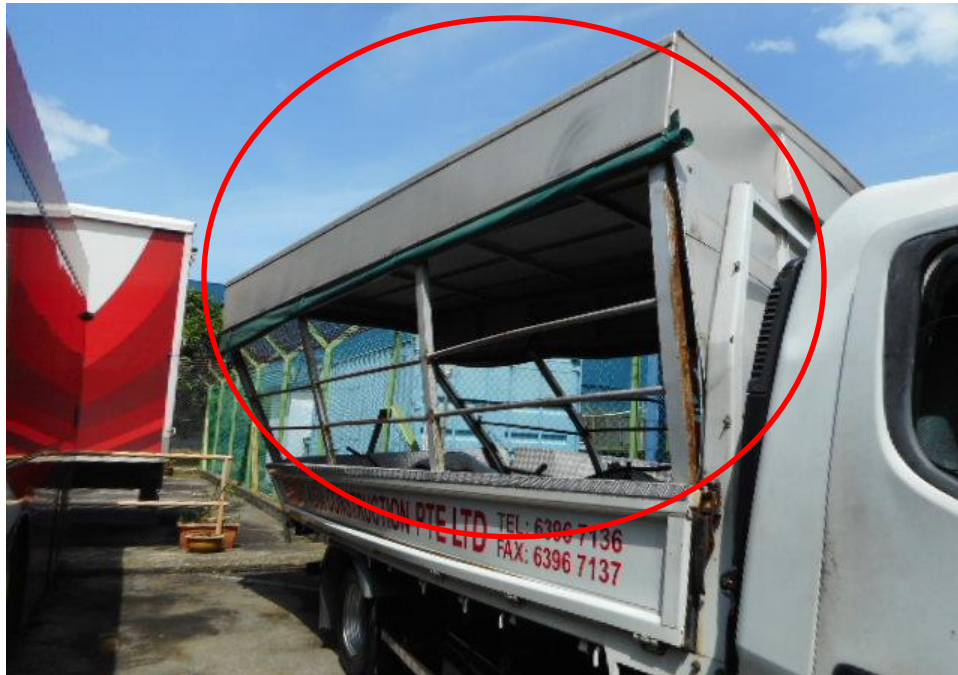
Photo 6 shows a right general view of the rear cabin portion of the Motor Lorry at the time of my inspection, its rear cabin body panel (circled) was observed to have been damaged as a result of the accident's impact.
