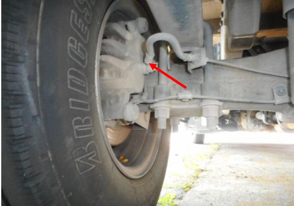
Photo 20 shows the various undercarriage components at the rear left wheel of the Motor Lorry, in particular the brake hose and drum brake (arrowed). The various undercarriage components of the Motor Lorry were all found to be intact without any visible damage. There was also no sign of fluid stain(s) observed on the various undercarriage components.
