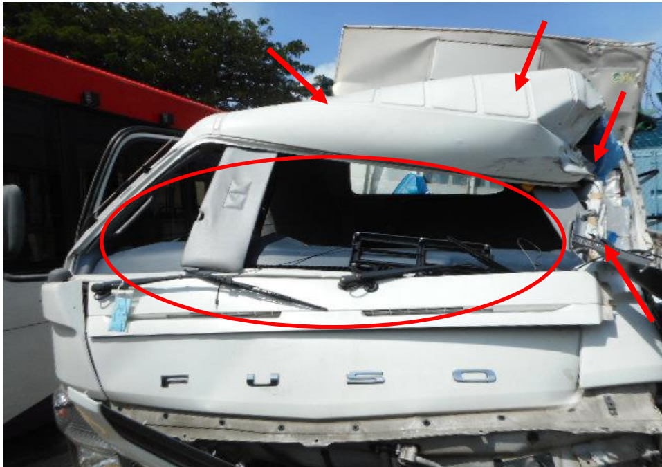
Photo 2 shows the close up view of the front portion of the Motor Lorry at the time of our inspection. The Motor Lorry was observed to have sustained major damages to its front windscreen (circled) and its front cabin (arrowed) that was crushed due to the accident's impact.
