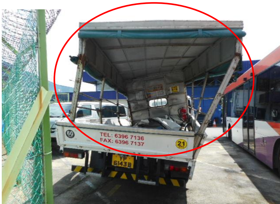
Photo 7 shows a rear general view of the rear cabin portion of the Motor Lorry at the time of my inspection, its rear cabin body panel (circled) was observed to have been damaged as a result of the accident's impact.
