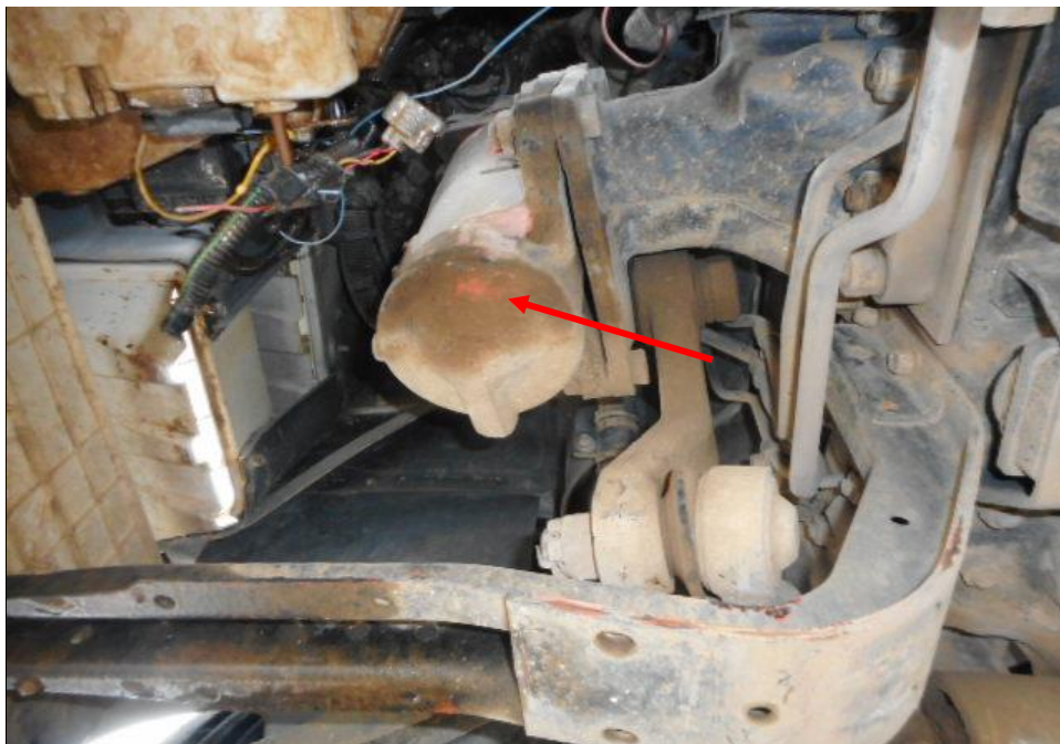
Photo 19 shows the steering box component (arrowed) at the undercarriage of the Motor Truck was found to be intact without any visible damage. There was also no sign of fluid stain(s) observed on the various undercarriage components.
