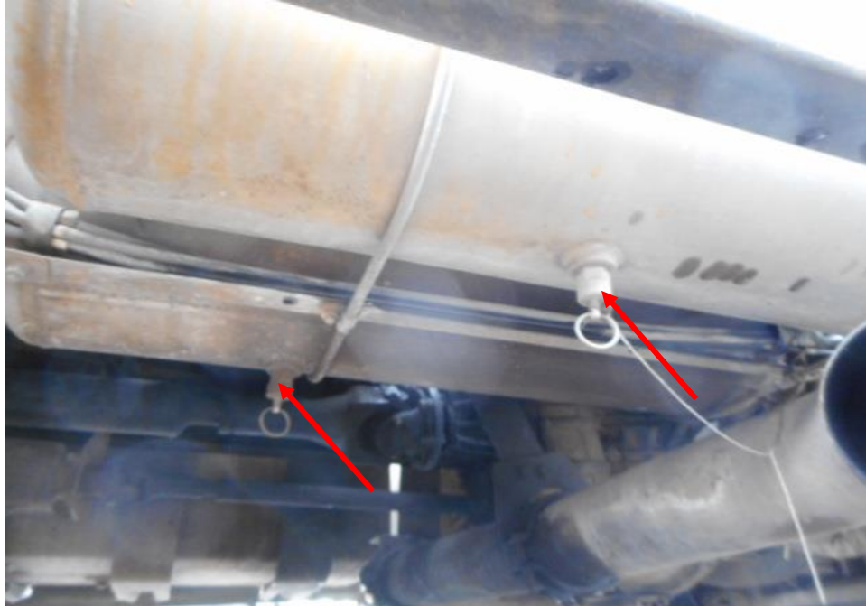
Photo 16 shows the air brake cylinders (arrowed) at the undercarriage of the Motor Truck. I did not observe any leakage of air brake fluid at the time of my inspection of the Motor Truck. My visual examination of the various mechanical components in the braking system had indicated that these was no internal leakage of pressure/vacuum and these components were generally in good condition.
