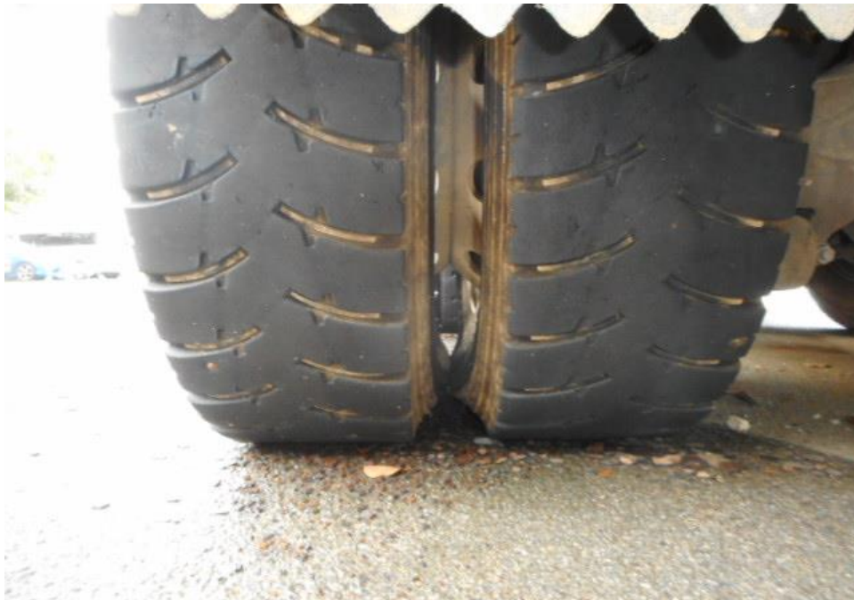
Photo 8 shows the condition of the rear right tyre of the Motor Truck, which was observed to be in serviceable condition with remaining tread depth of approximately 6.5mm. The tyre, which was wrapped around standard steel wheel rim, was also observed to be sufficiently inflated for vehicular operation.
