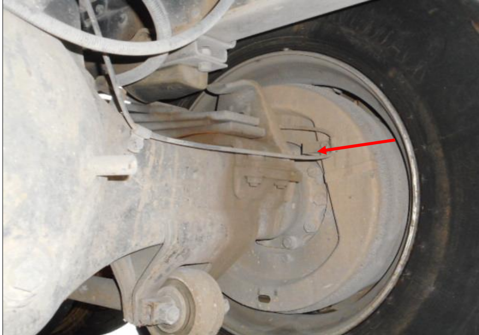
Photo 12 shows the brake pipe (arrowed) at the rear right wheel of the Motor Truck. I did not observe any leakage of brake fluid at the time of my inspection of the Motor Truck. My visual examination of the various mechanical components in the braking system, had indicated that these was no internal leakage of pressure/vacuum and these components were generally in good condition.
