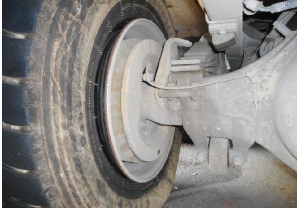
Photo 9 shows the close up view of the rear left inner tyre of the Motor Truck, which was observed to be deflated and slipped off the wheel rim.
