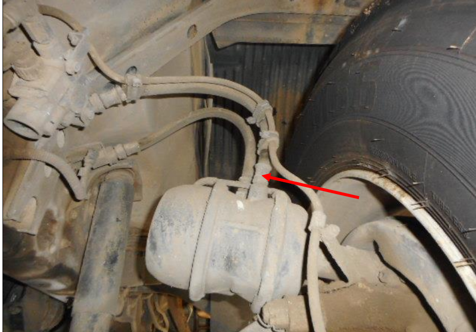
Photo 14 shows the brake pipe (arrowed) at the front right wheel of the Motor Truck. I did not observe any leakage of brake fluid at the time of my inspection of the Motor Truck. My static tests of the Motor Truck's braking system, along with my visual examination of the various mechanical components in the braking system, had indicated that there was no internal leakage of pressure/vacuum and these components were generally in good condition.
