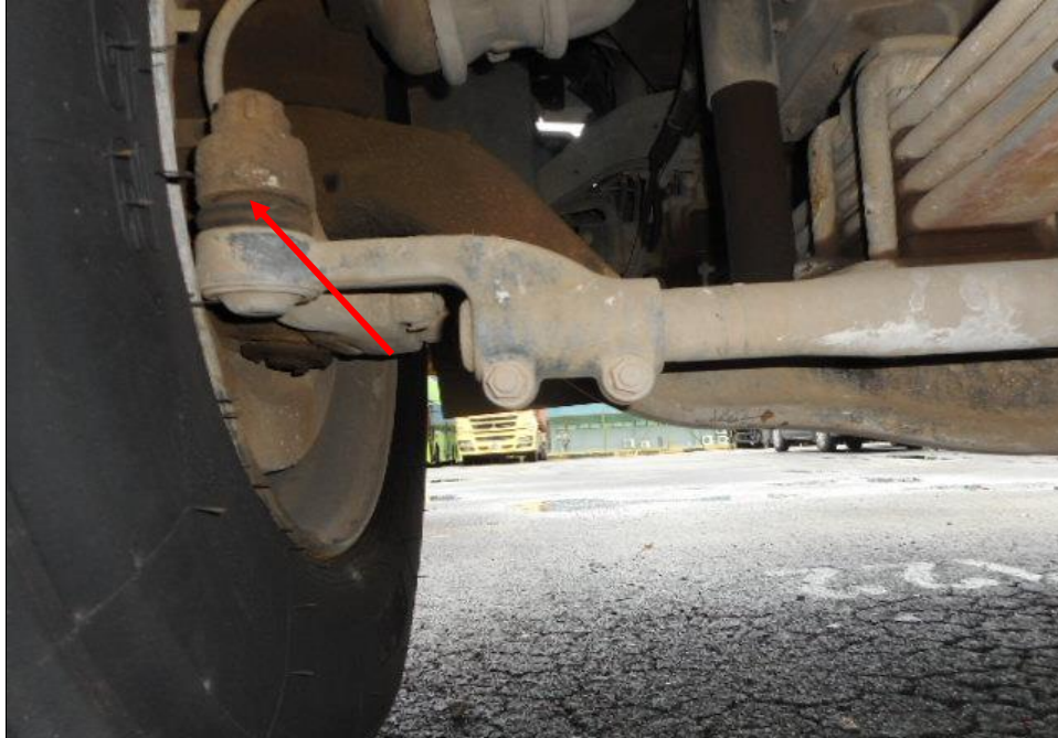
Photo 18 shows the various undercarriage components at the front left wheel of the Motor Truck, in particular the steering tie rod end (arrowed). The various undercarriage components of the Motor Truck were all found to be intact without any visible damage. There was also no sign of fluid stain(s) observed on the various undercarriage components.
