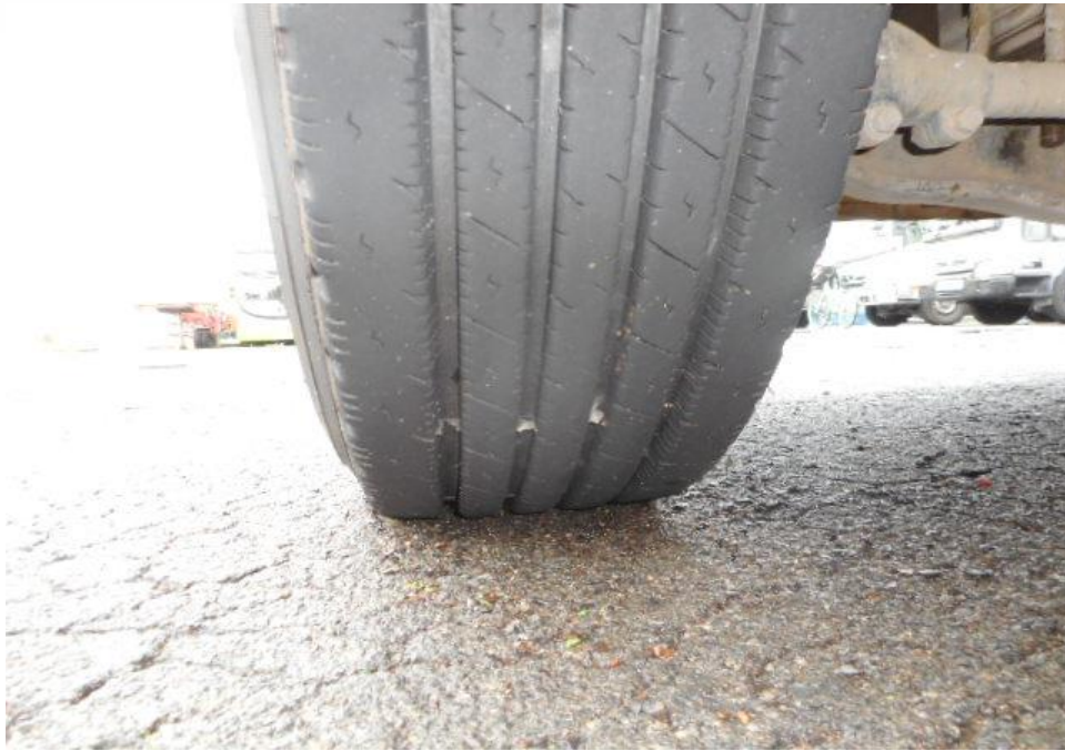
Photo 11 shows the condition of the front left tyres of the Motor Truck, which were observed to be in serviceable condition with remaining tread depth of approximately 12.4mm. There was also no tear, cut or burst mark(s) on the outer and the inner sidewalls as well as across the tread of the 10 tyres that were fitted on the Truck.
