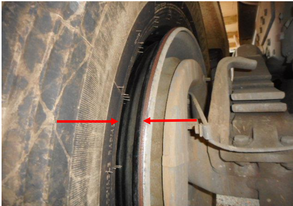
Photo 10 shows the close up view of the rear left inner tyre of the Motor Truck, which was observed to be deflated and slipped off the wheel rim (arrowed).
