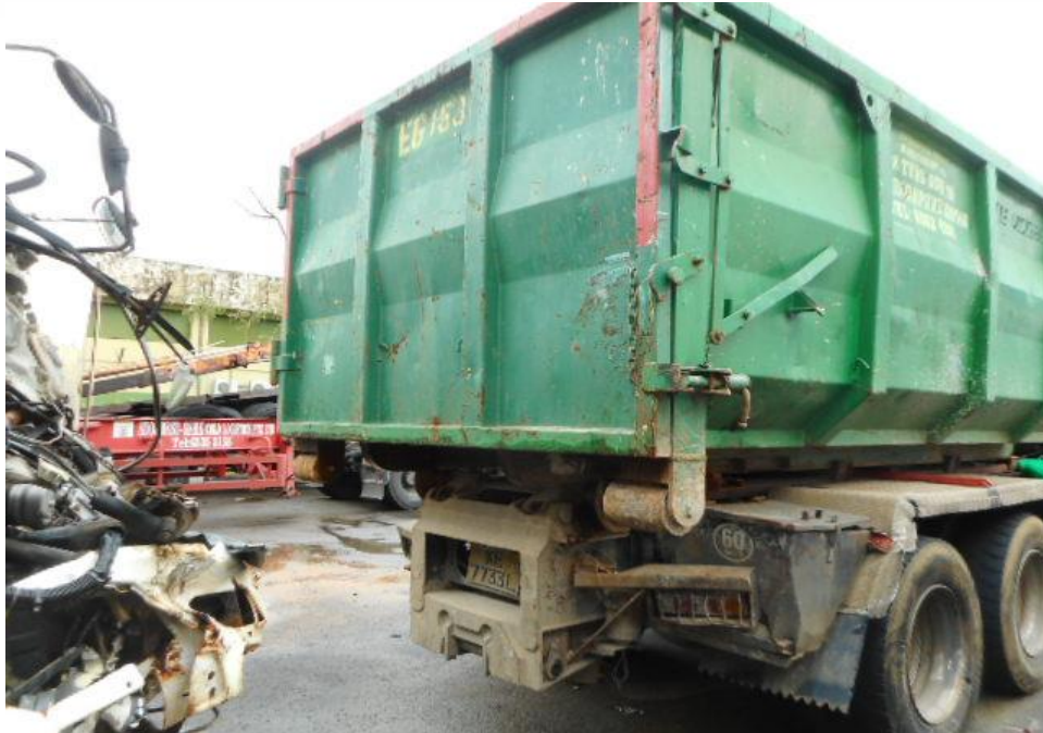
Photo 1 shows a general view of the Motor Truck's rear body at the time of my inspection. The Motor Truck was observed to sustained damage at its rear portion. Its rear right brake lamp were damage at the time of my inspection as a result of the accident.
