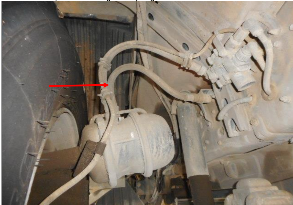
Photo 15 shows the brake pipe (arrowed) at the front left wheel of the Motor Truck. I did not observe any leakage of brake fluid at the time of my inspection of the Motor Truck. My visual examination of the various mechanical components in the braking system had indicated that there was no internal leakage of pressure/vacuum and these components were generally in good condition.
