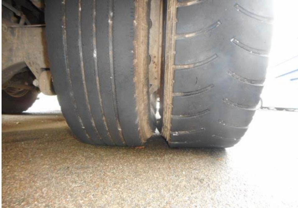
Photo 7 shows the condition of the rear right tyre of the Motor Truck, which was observed to be in serviceable condition with remaining tread depth of approximately 6.5mm. The tyre, which was wrapped around standard steel wheel rim, was also observed to be sufficiently inflated for vehicular operation.
