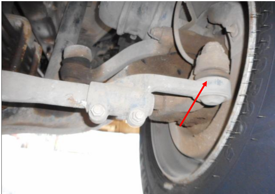
Photo 17 shows the various undercarriage components at the front right wheel of the Motor Truck, in particular the steering tie rod end (arrowed). The various steering components were all found to be intact, suggesting that the steering system of the Motor Truck was likely to be in serviceable condition at the material time of accident. There was also no sign of fluid stain(s) observed on the various undercarriage components.
