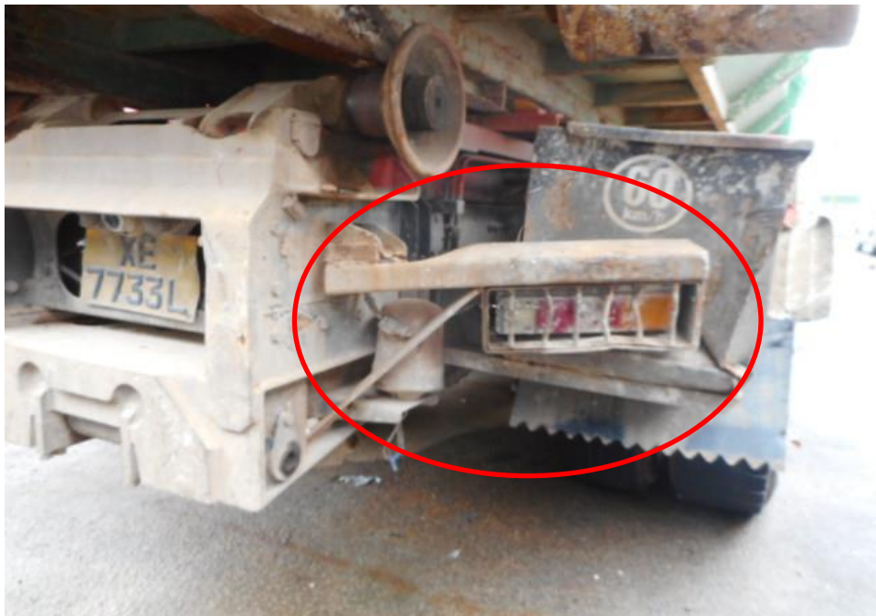
Photo 2 shows a close up view of the Motor Truck's rear body at the time of my inspection. The Motor Truck was observed to sustained damage at its rear portion. Its rear right brake lamp (circled) were damage at the time of my inspection as a result of the accident.
